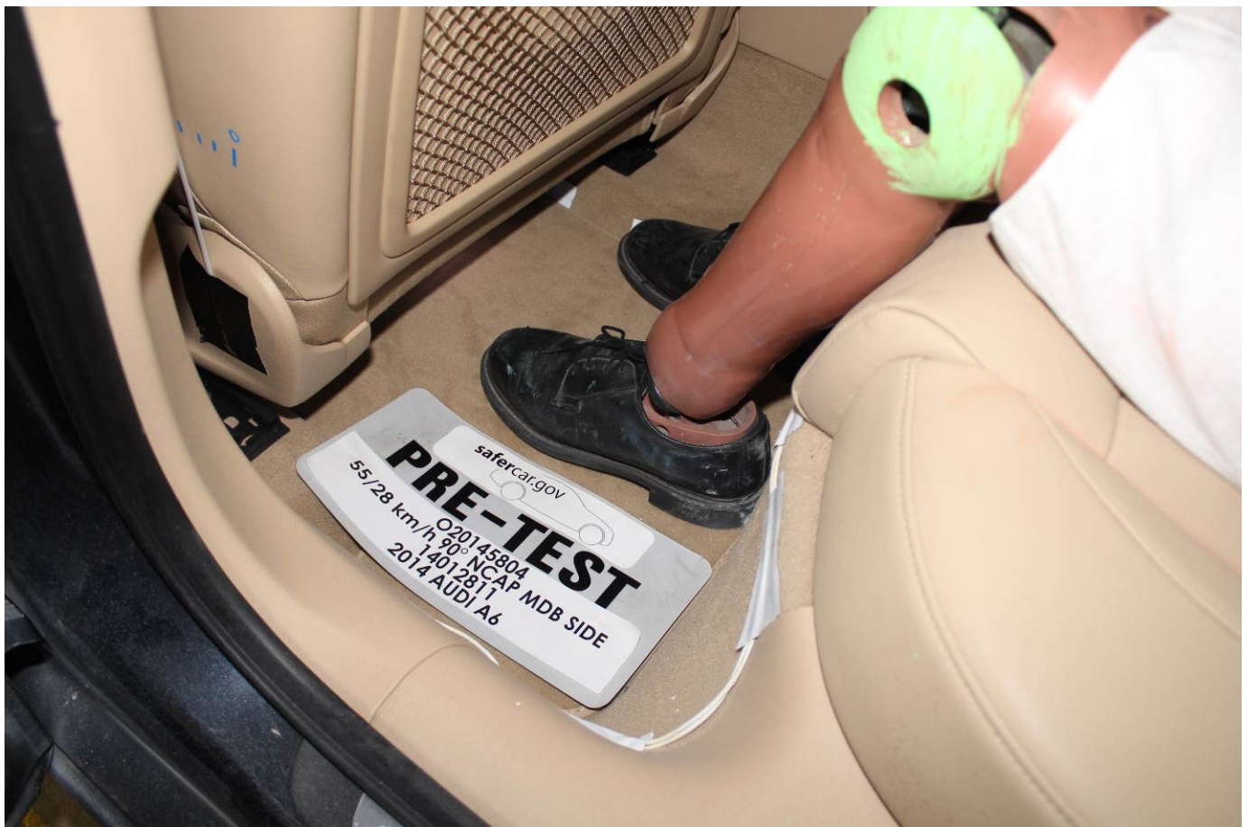
Pre-Test Placement of Rear Passenger Dummy's Feet
