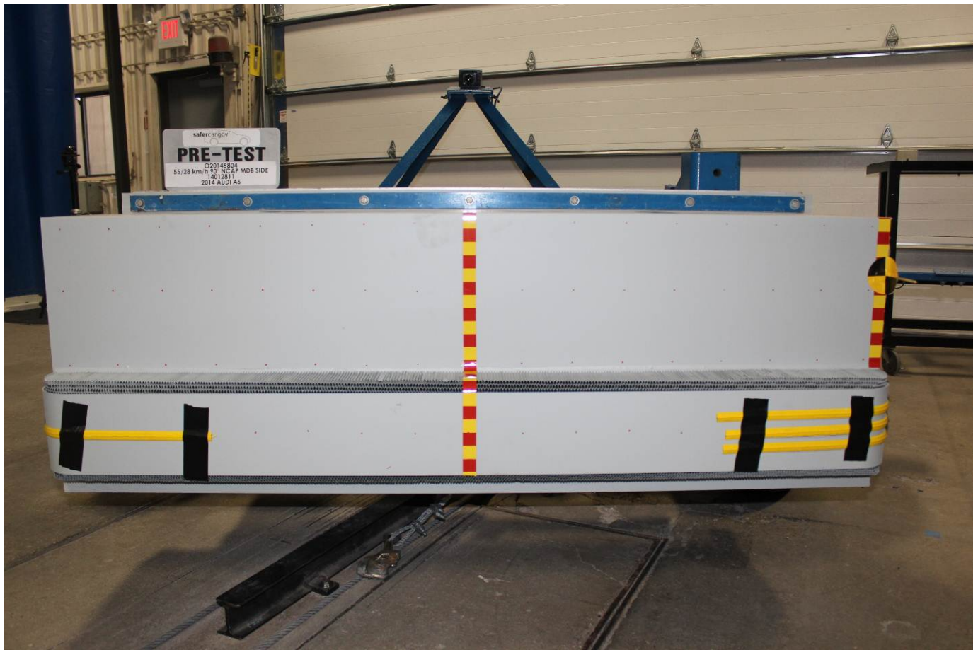
Pre-Test Front View of MDB Impactor Face
