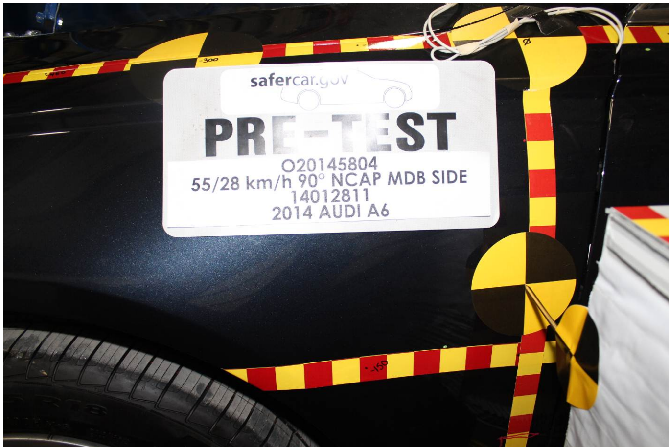
Pre-Test Close-Up View of Impact Point Target
