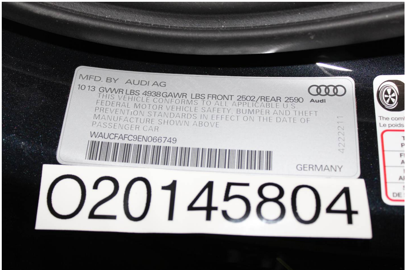
Close-Up View of Vehicle's Certification Label
