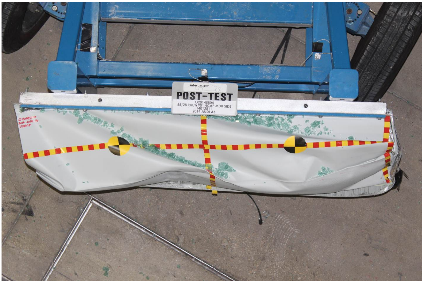
Post-Test Top View of MDB Impactor Face
