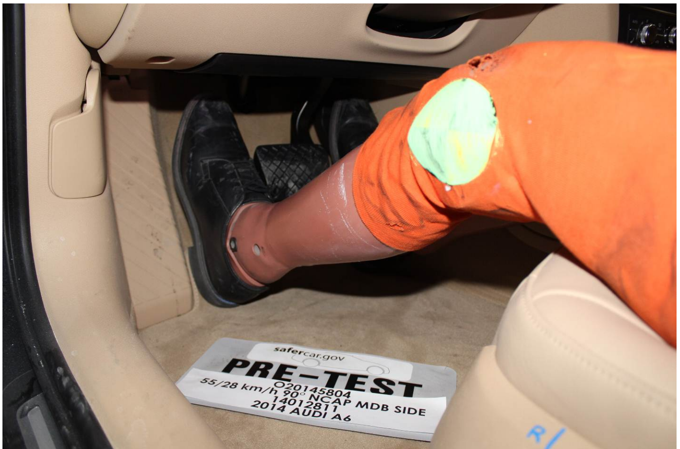
Pre-Test Placement of Driver Dummy's Feet
