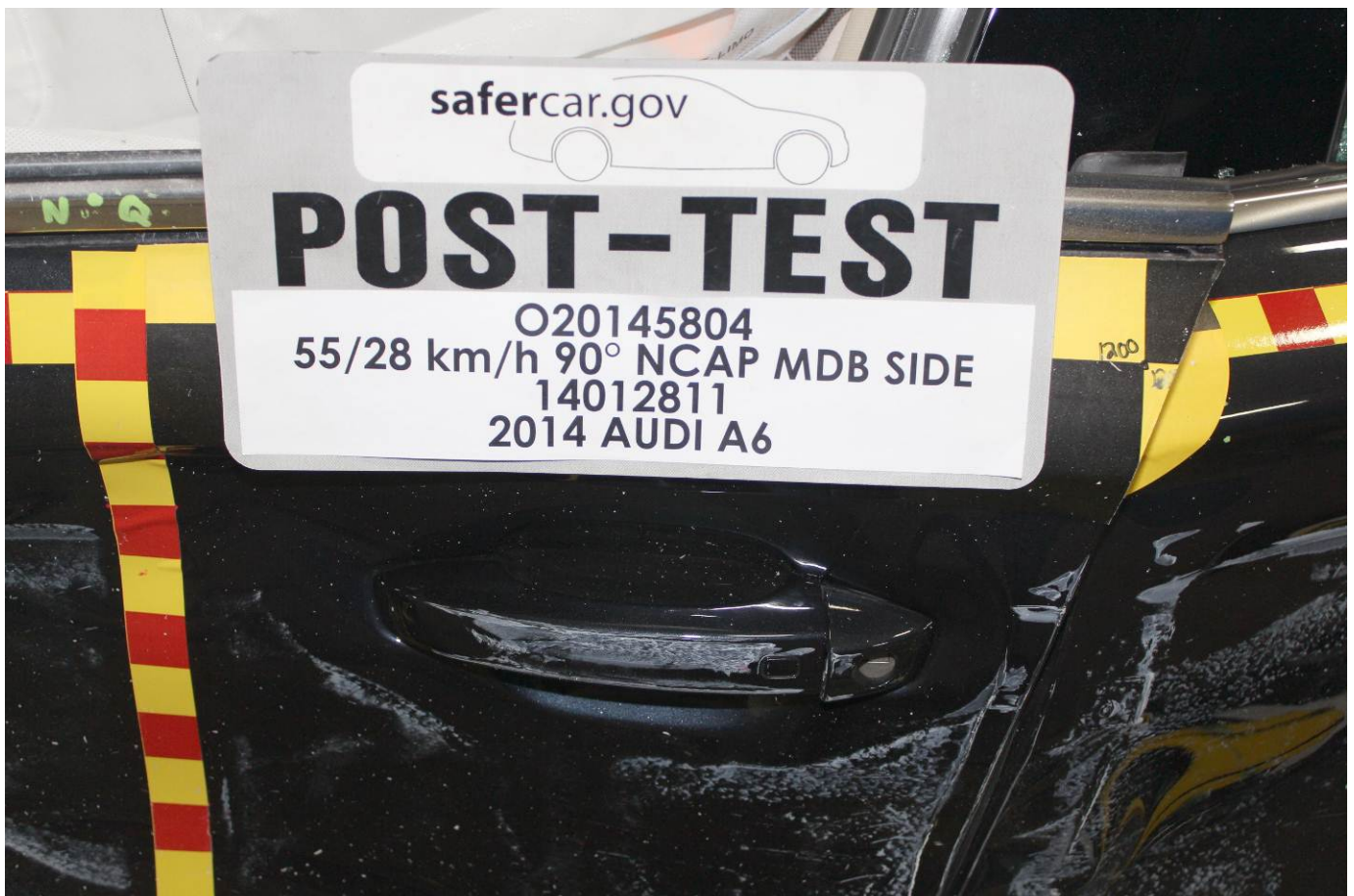
Post-Test Left Front Door Latch Close-Up
