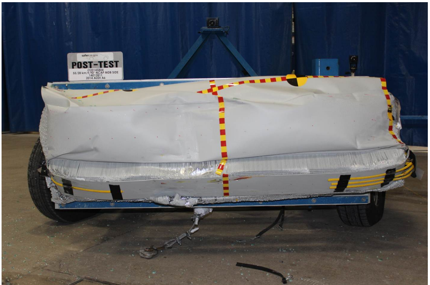
Post-Test Front View of MDB Impactor Face
