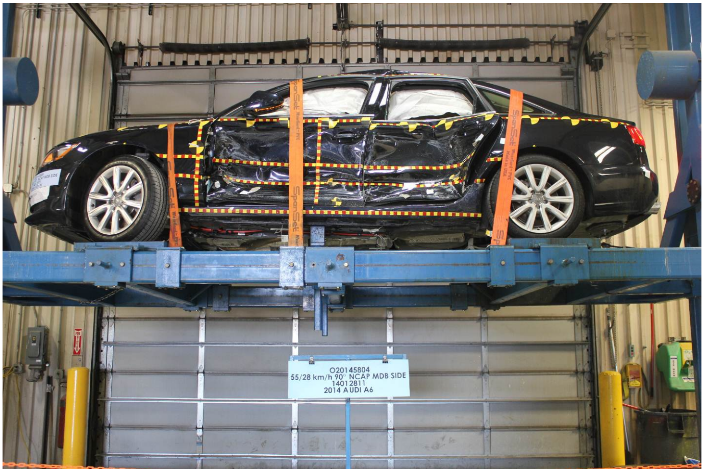
FMVSS No. 301 Static Rollover 360 Degrees
