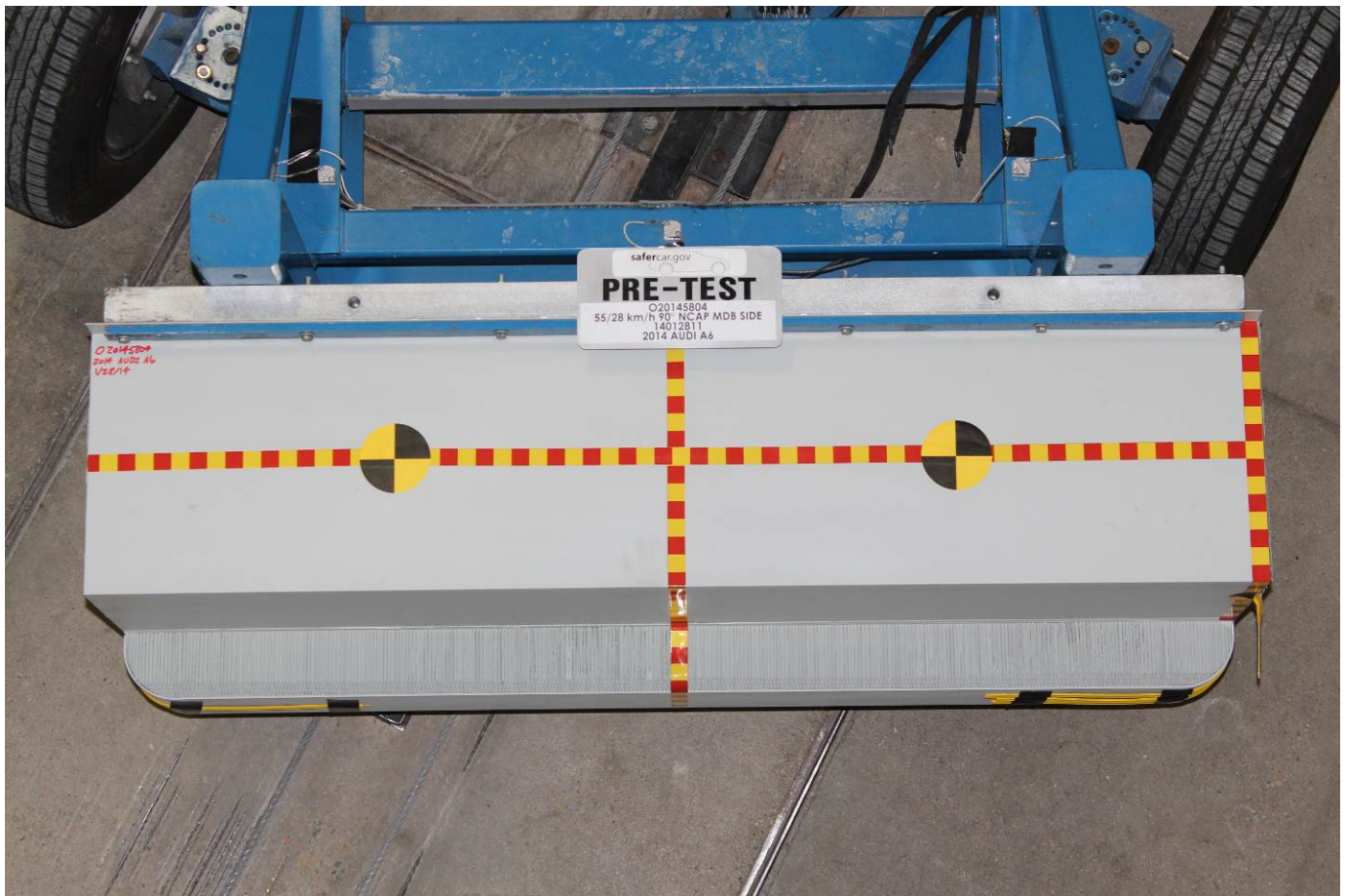
Pre-Test Top View of MDB Impactor Face
