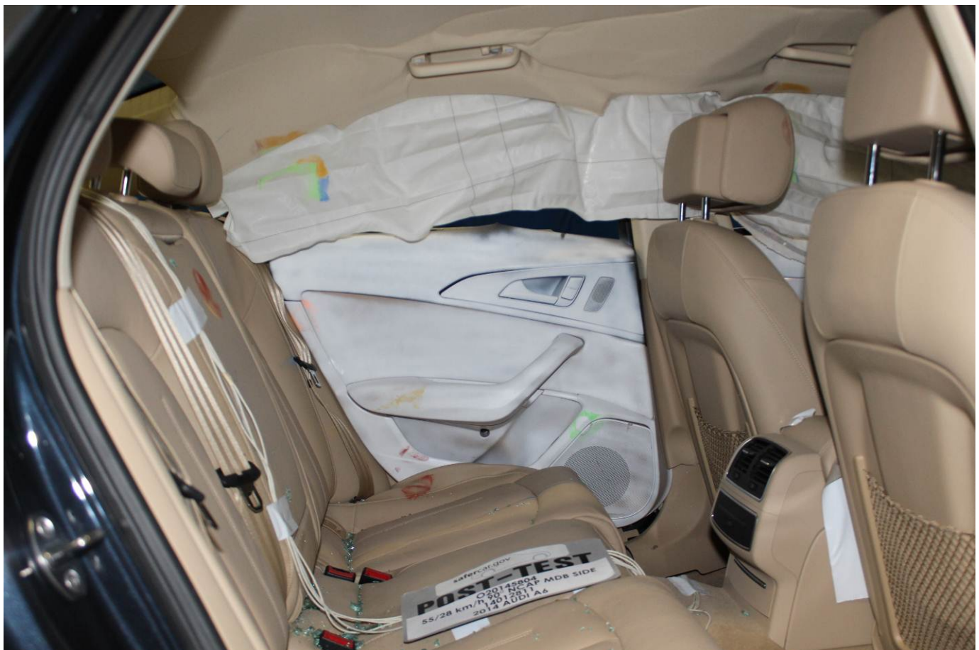
Post-Test Rear Passenger Inner Door Panel View
