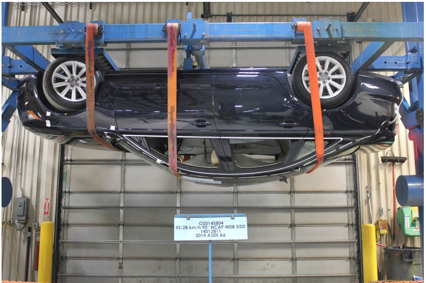
FMVSS No. 301 Static Rollover 180 Degrees
