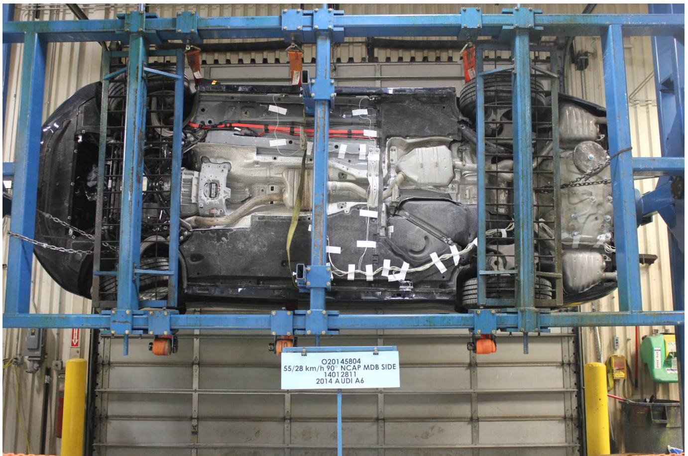
FMVSS No. 301 Static Rollover 90 Degrees
