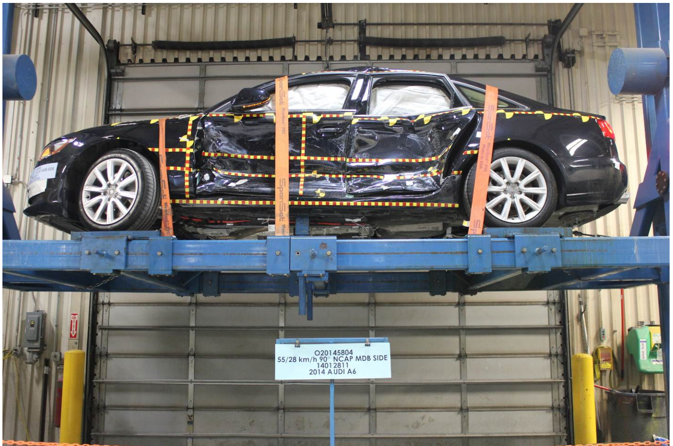
FMVSS No. 301 Static Rollover 0 Degrees
