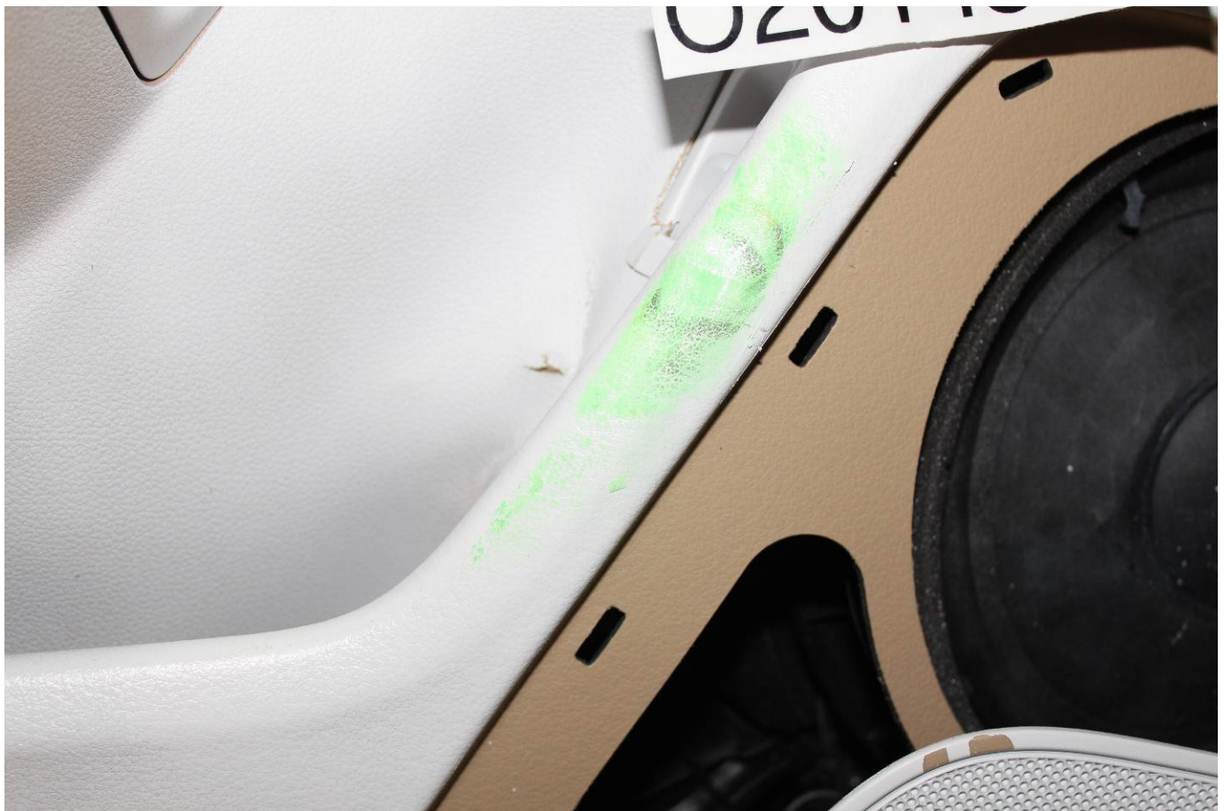
Post-Test Driver Dummy Close-up Knee Contact View
