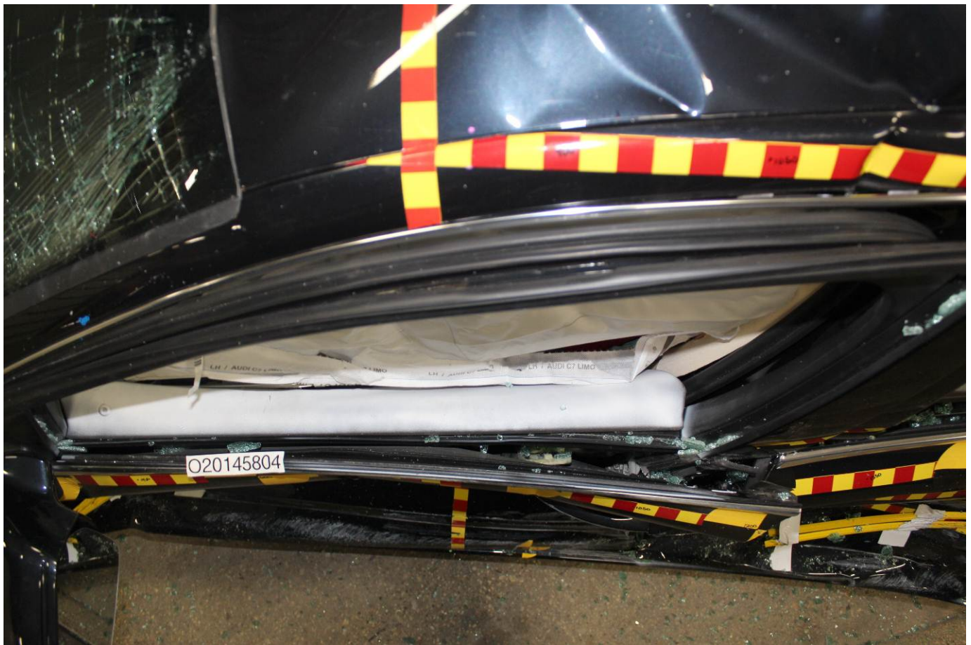
Post-Test Driver Dummy and Door Clearance View
