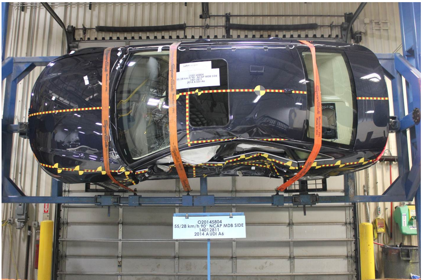
FMVSS No. 301 Static Rollover 270 Degrees
