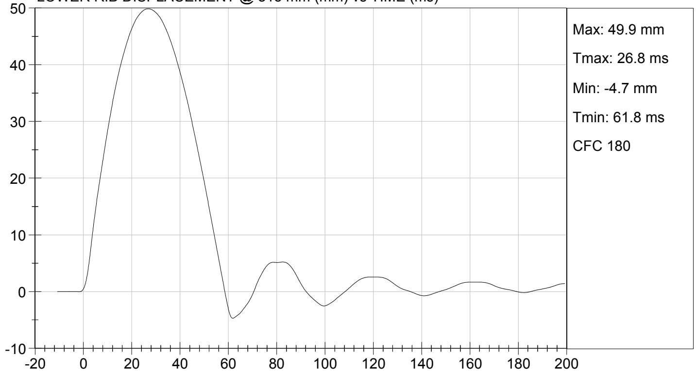
LOWER RIB DISPLACEMENT @ 815 mm (mm) vs TIME (ms)
