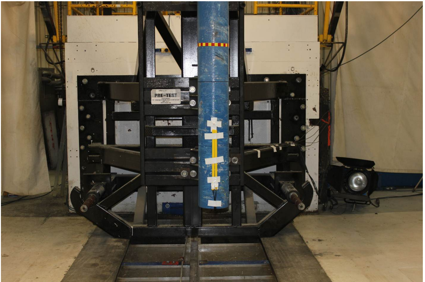
Pre-Test Pole Barrier Front View
