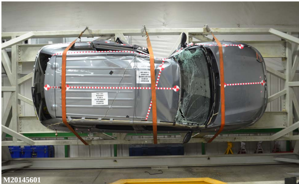
Figure 066: FMVSS No. 301 Static Rollover 270 Degrees
