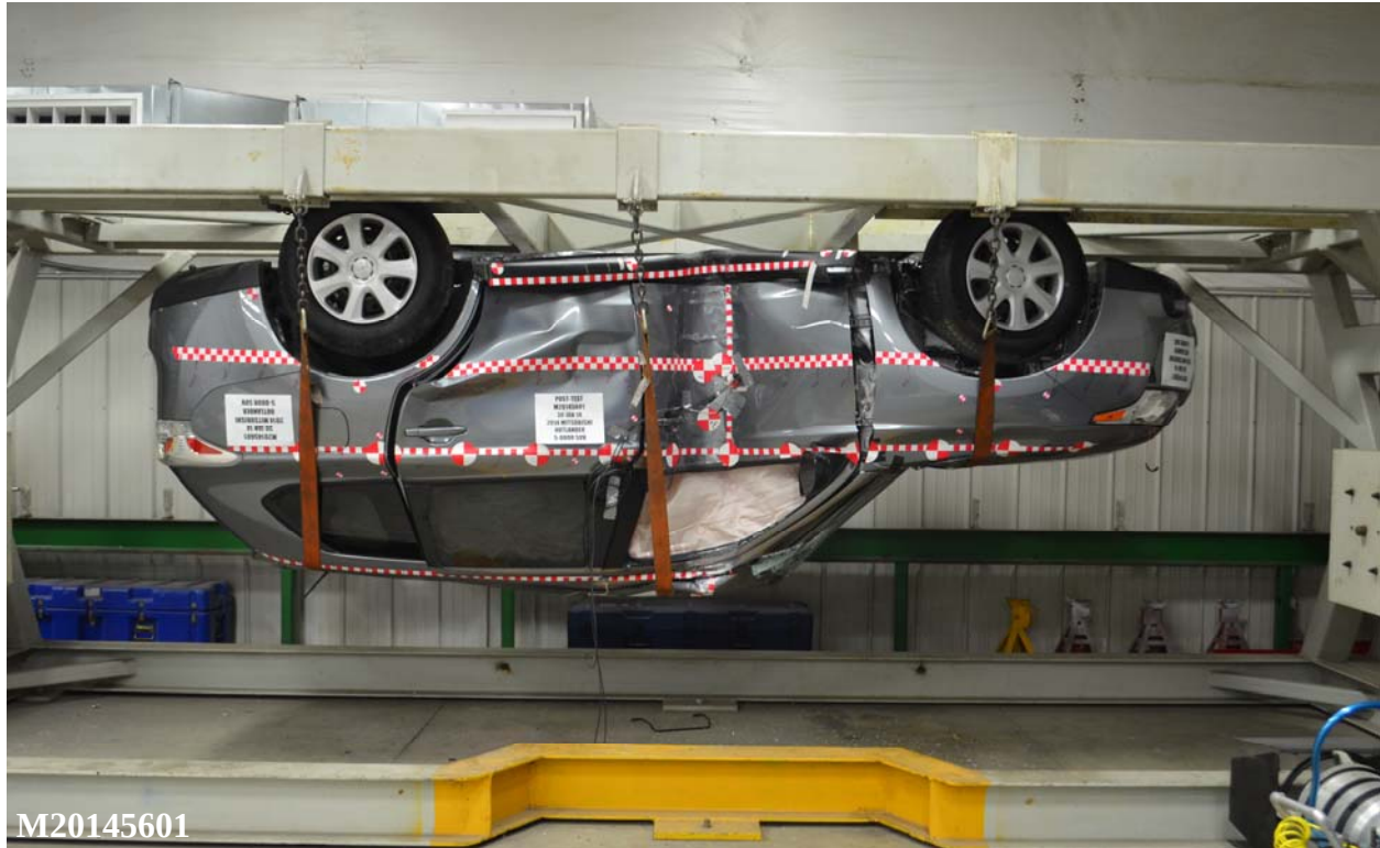
Figure 065: FMVSS No. 301 Static Rollover 180 Degrees
