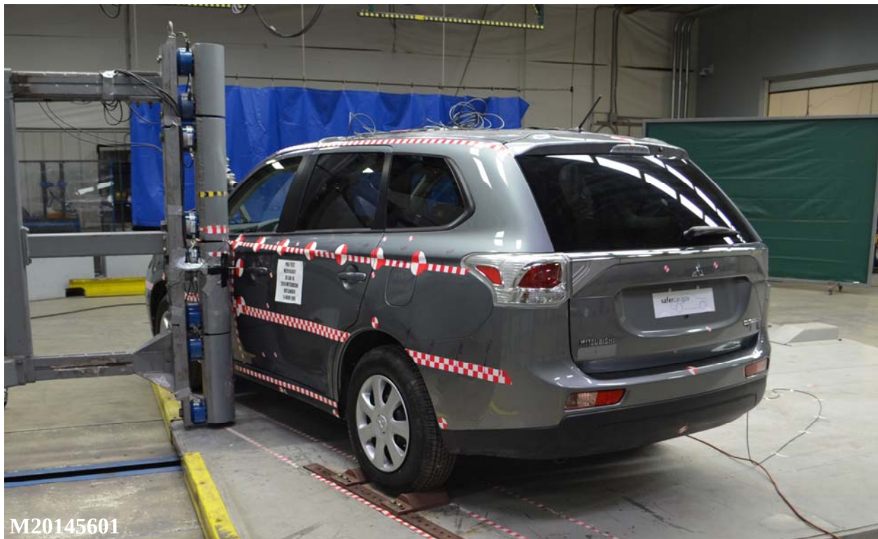
Figure 018: Pre-Test Right Side View of Pole Positioned Against Side of Vehicle
