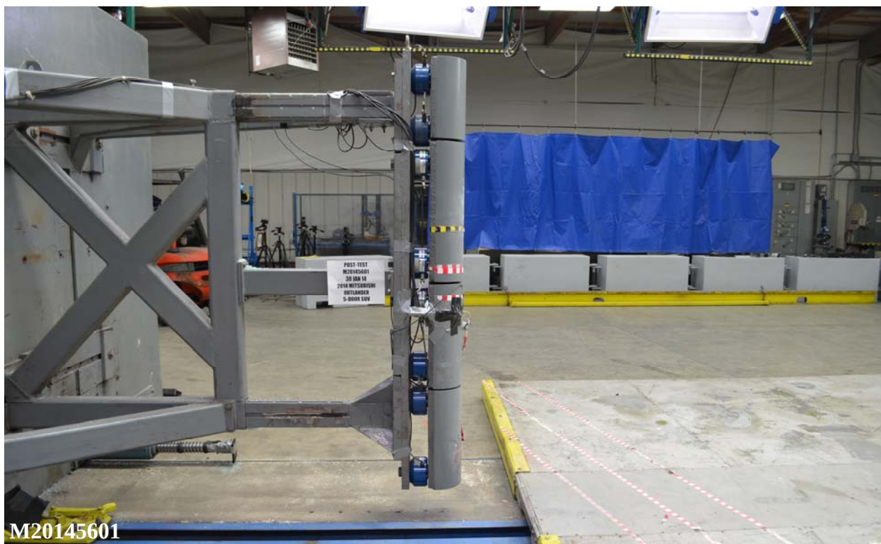
Figure 060: Post-Test Pole Barrier Side View
