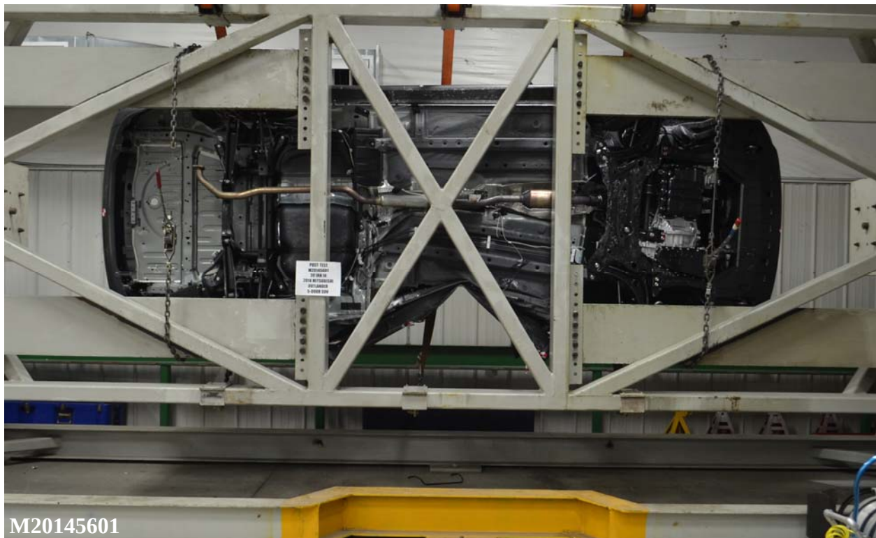
Figure 064: FMVSS No. 301 Static Rollover 90 Degrees
