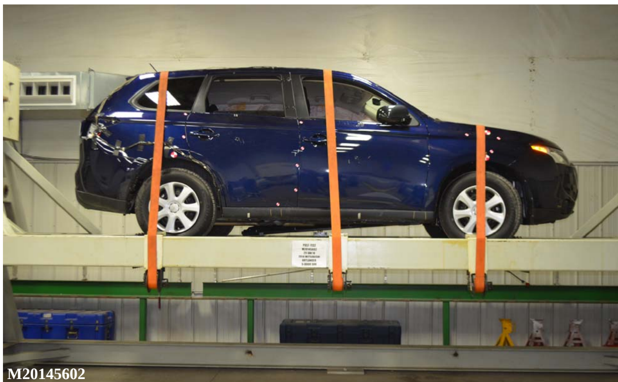
Figure A-96: FMVSS No. 301 Static Rollover 0 Degrees
