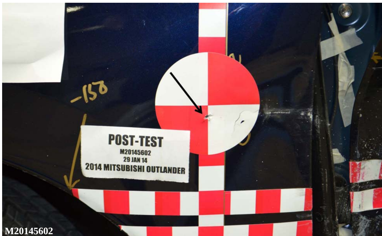
Figure A-20: Post-Test Close-Up View of Impact Point Target
