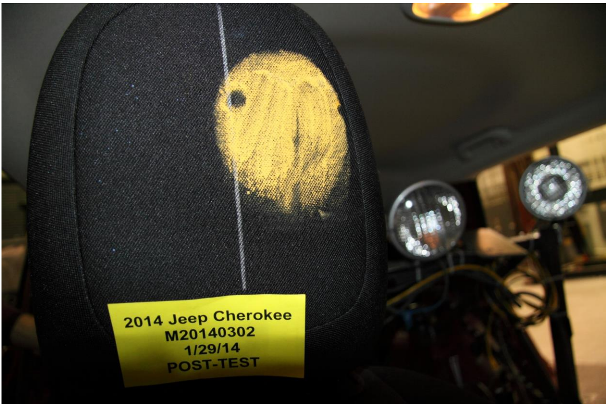
066 Post Test Passenger Dummy Contact With Headrest
