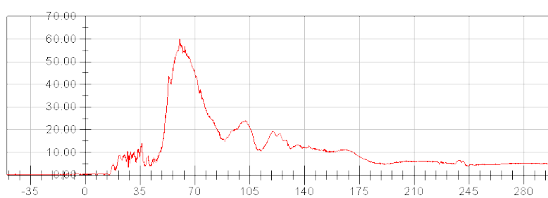
Passenger Head Resultant Acceleration vs. Time Primary (g) vs. Time [ms]
