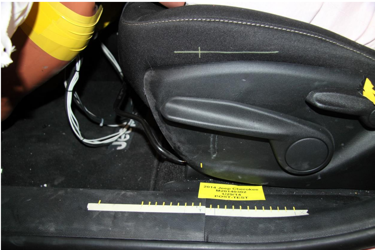
036 Post-Test Driver's Seat Fore-Aft Markings
