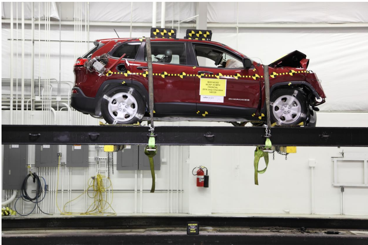
074 Vehicle at 360° on Static Rollover Device
