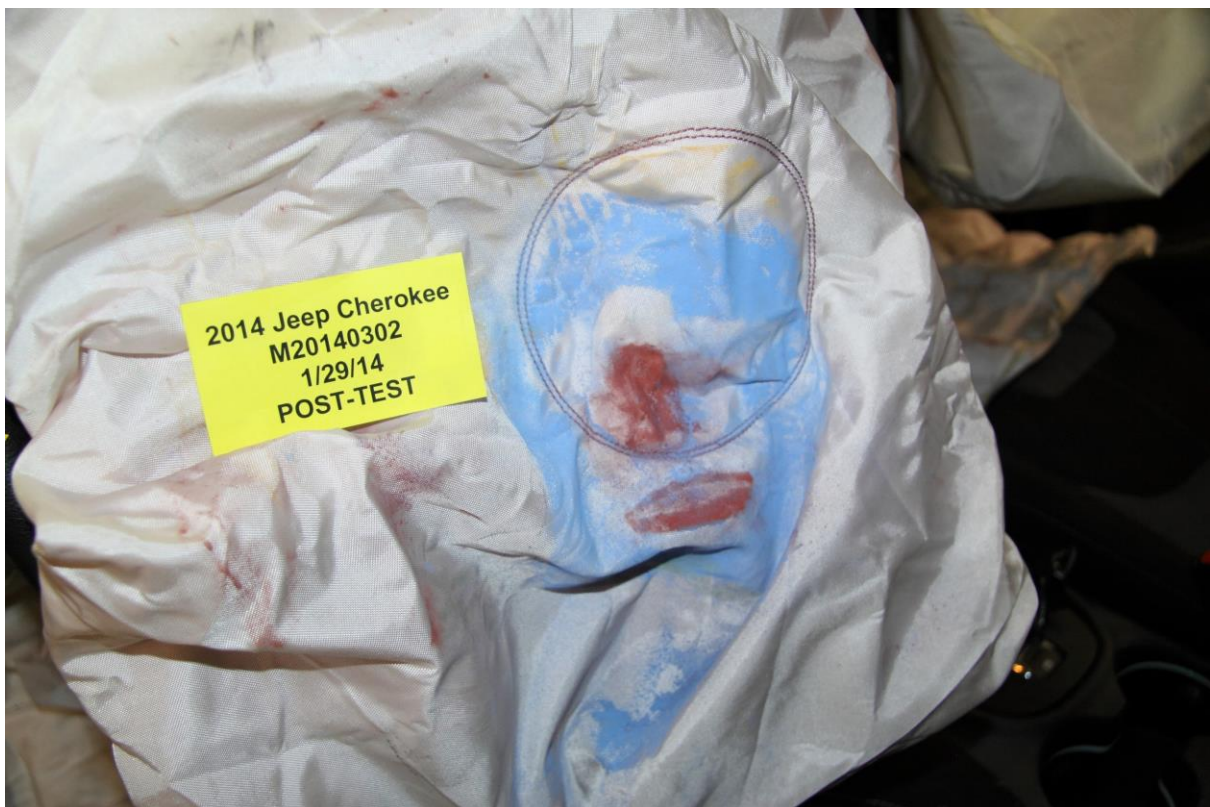
046 Post-Test Driver Dummy Contact With Airbag
