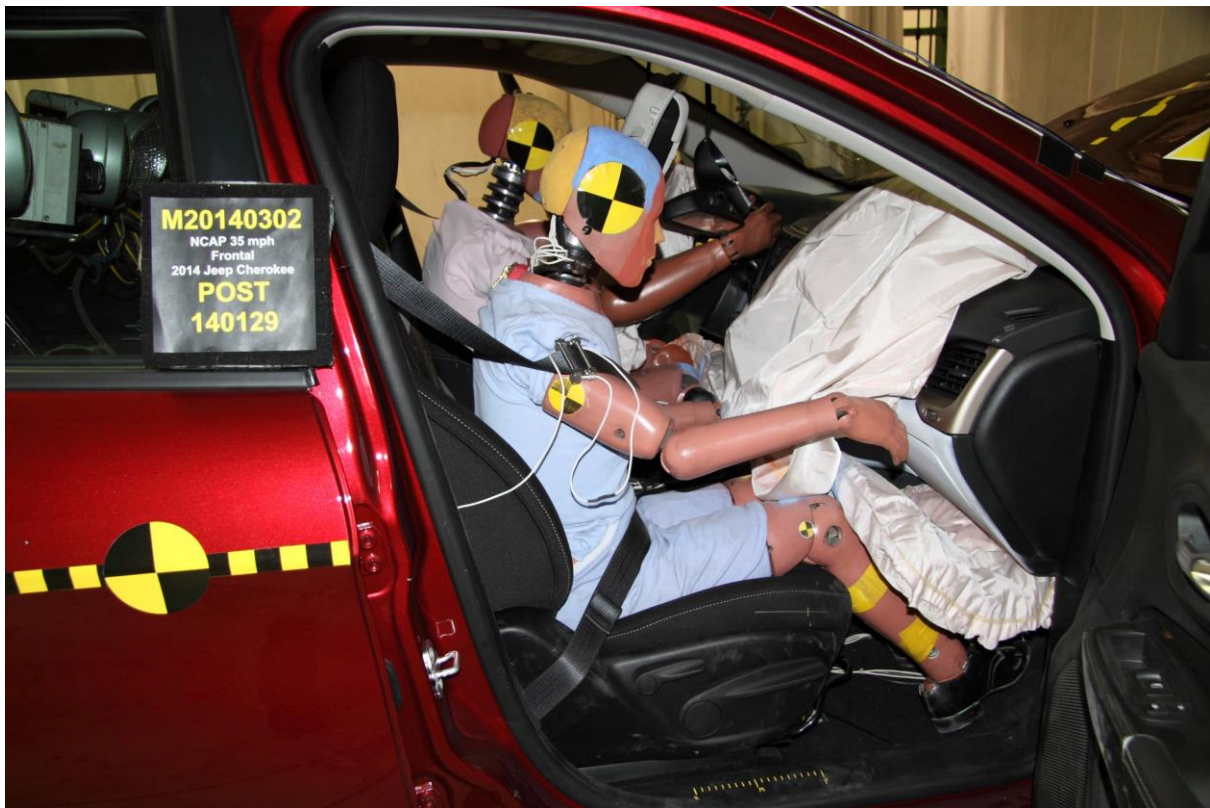
055 Post-Test Passenger Dummy and Vehicle Interior View
