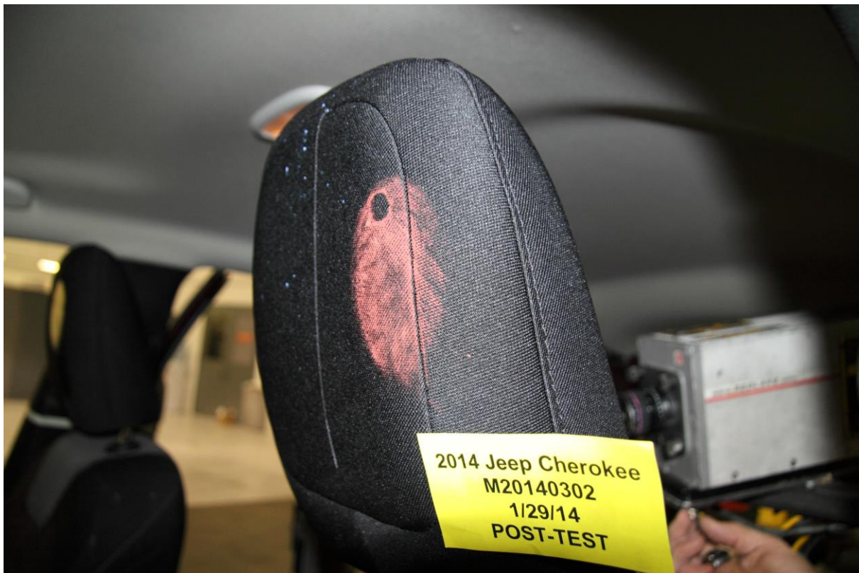
047 Post-Test Driver Dummy Contact With Headrest
