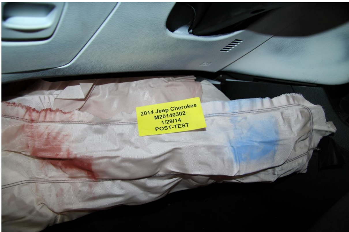
042 Post-Test Driver's Side Knee Bolster
