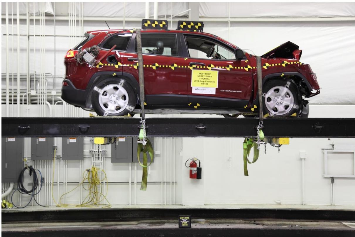
070 Vehicle at 0° on Static Rollover Device
