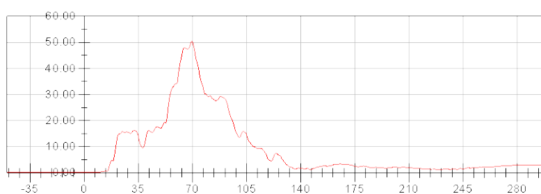
Passenger Chest Resultant Acceleration vs. Time Primary (g) vs. Time [ms]
