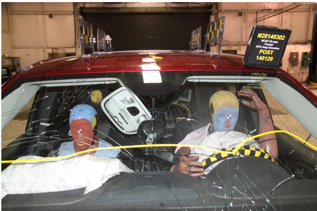
018 Post-Test Windshield View
