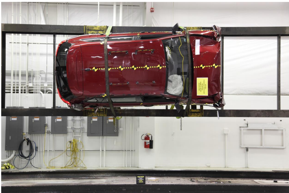
071 Vehicle at 90° on Static Rollover Device
