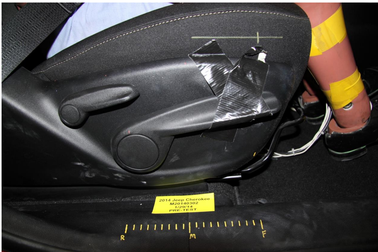
056 Pre-Test Passenger's Seat Fore-Aft Markings
