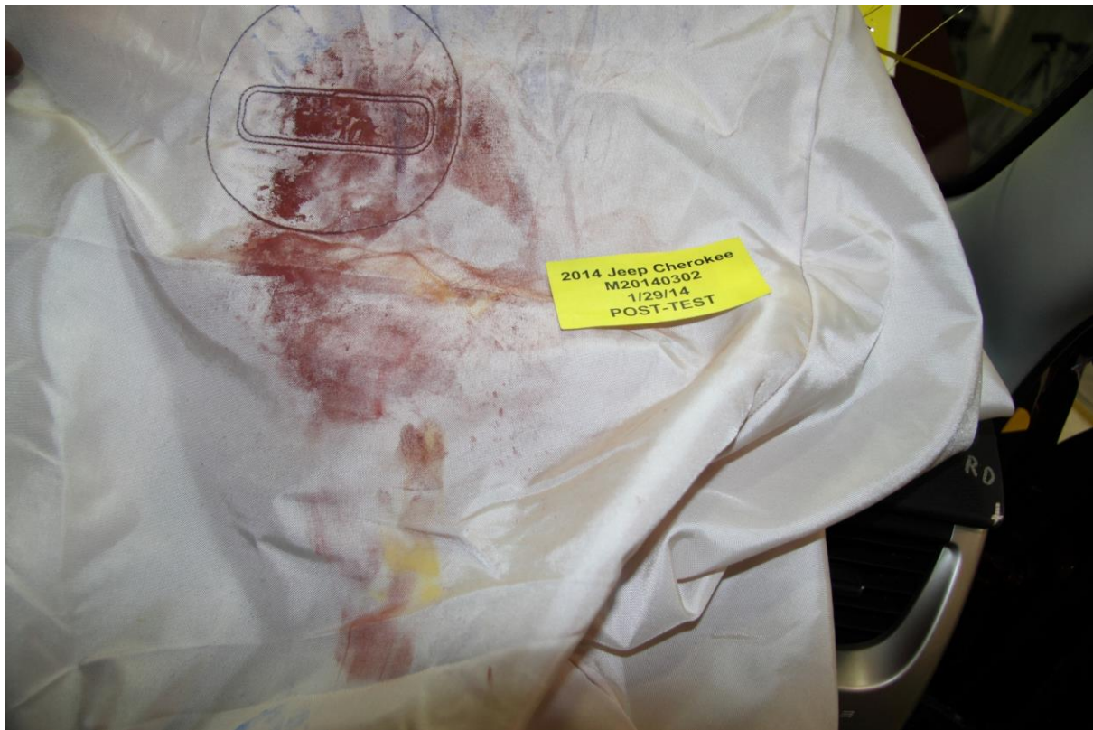
066a Post-Test Passenger Dummy Contact With Airbag
