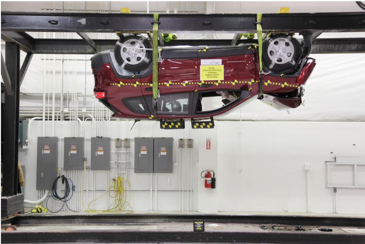
072 Vehicle at 180° on Static Rollover Device
