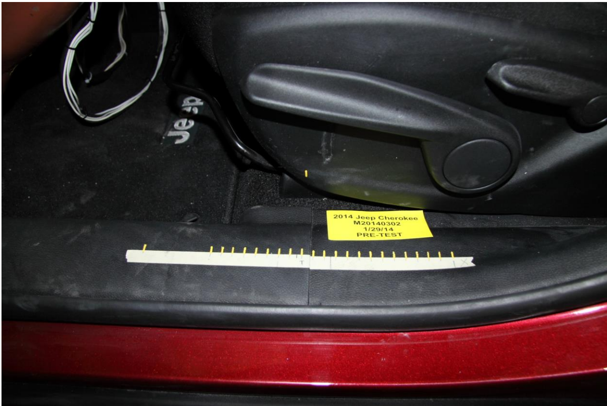
035 Pre-Test Driver's Seat Fore-Aft Markings
