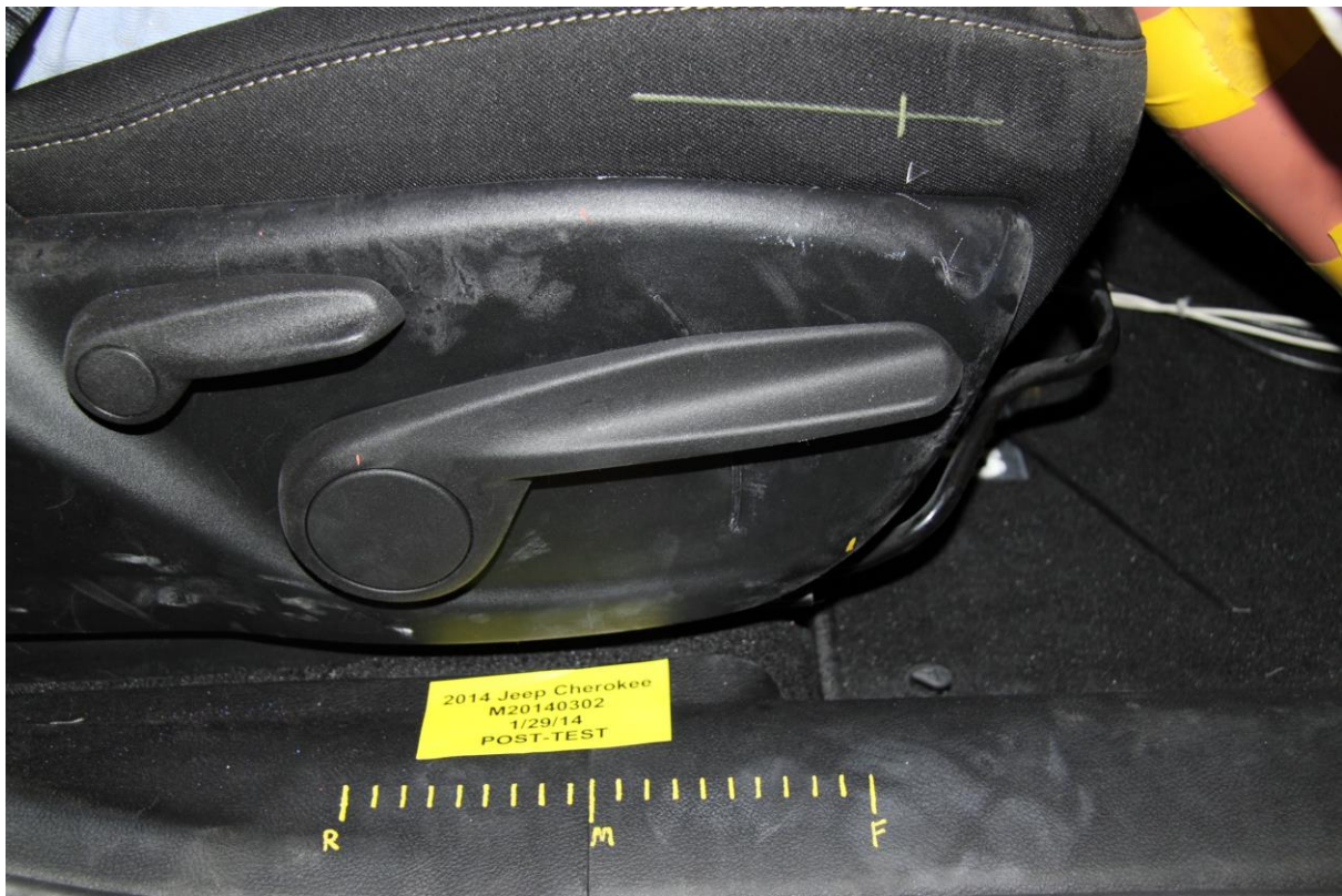
057 Post-Test Passenger's Seat Fore-Aft Markings
