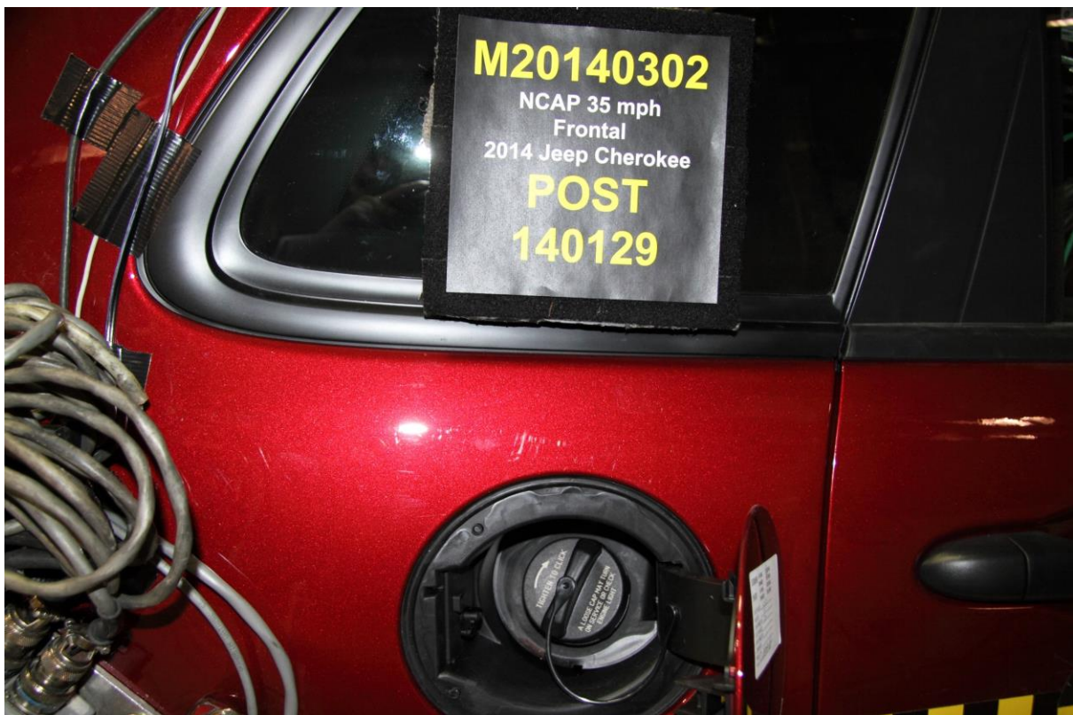
022 Post-Test Fuel Filler Cap View
