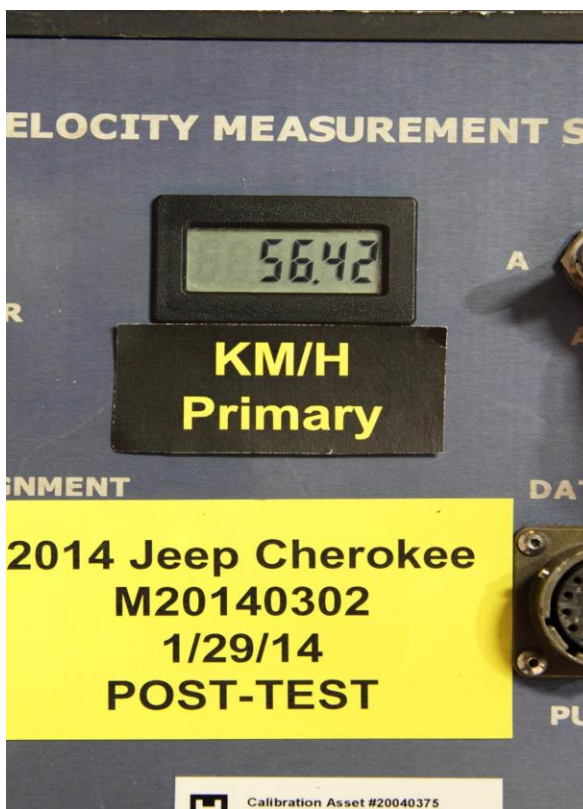
069 Post-Test Speed Trap Read-out
