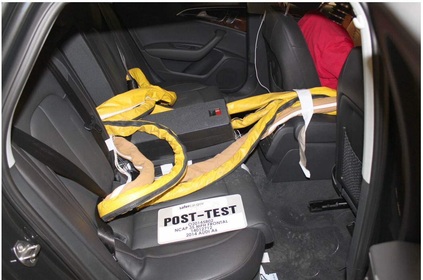
Post-Test Dummy Cable Routing
