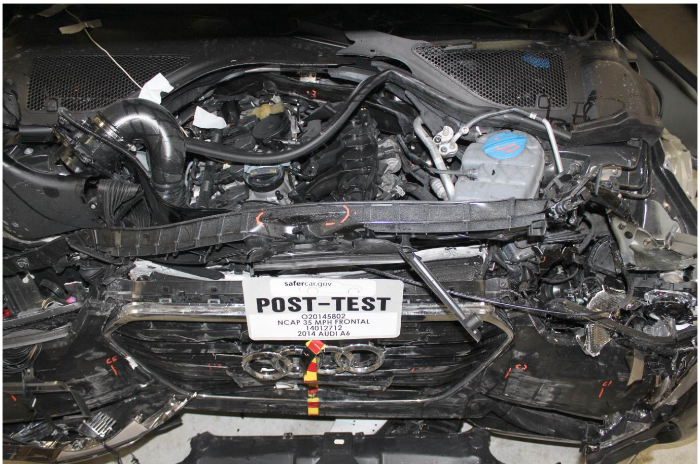
Post-Test Engine Compartment View
