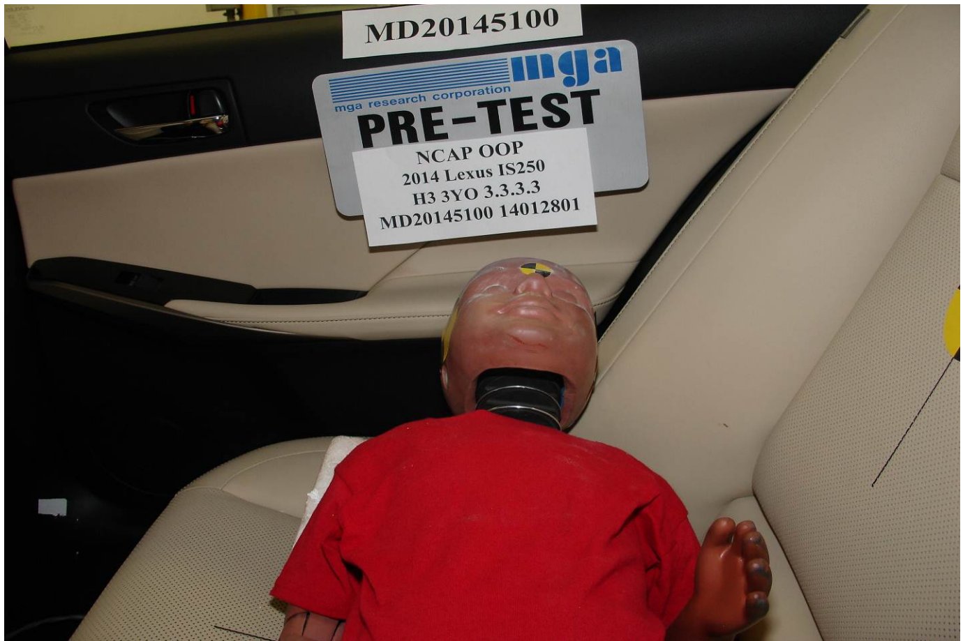
Pre-Test 3-Year-Old Child Dummy Left Side Closeup View
