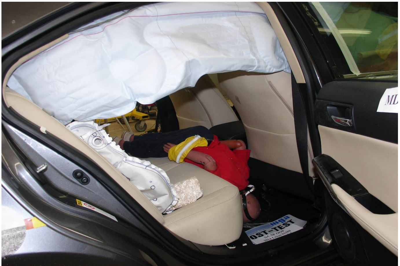
Post-Test 3-Year-Old Child Dummy Right Side View (Door Open)
