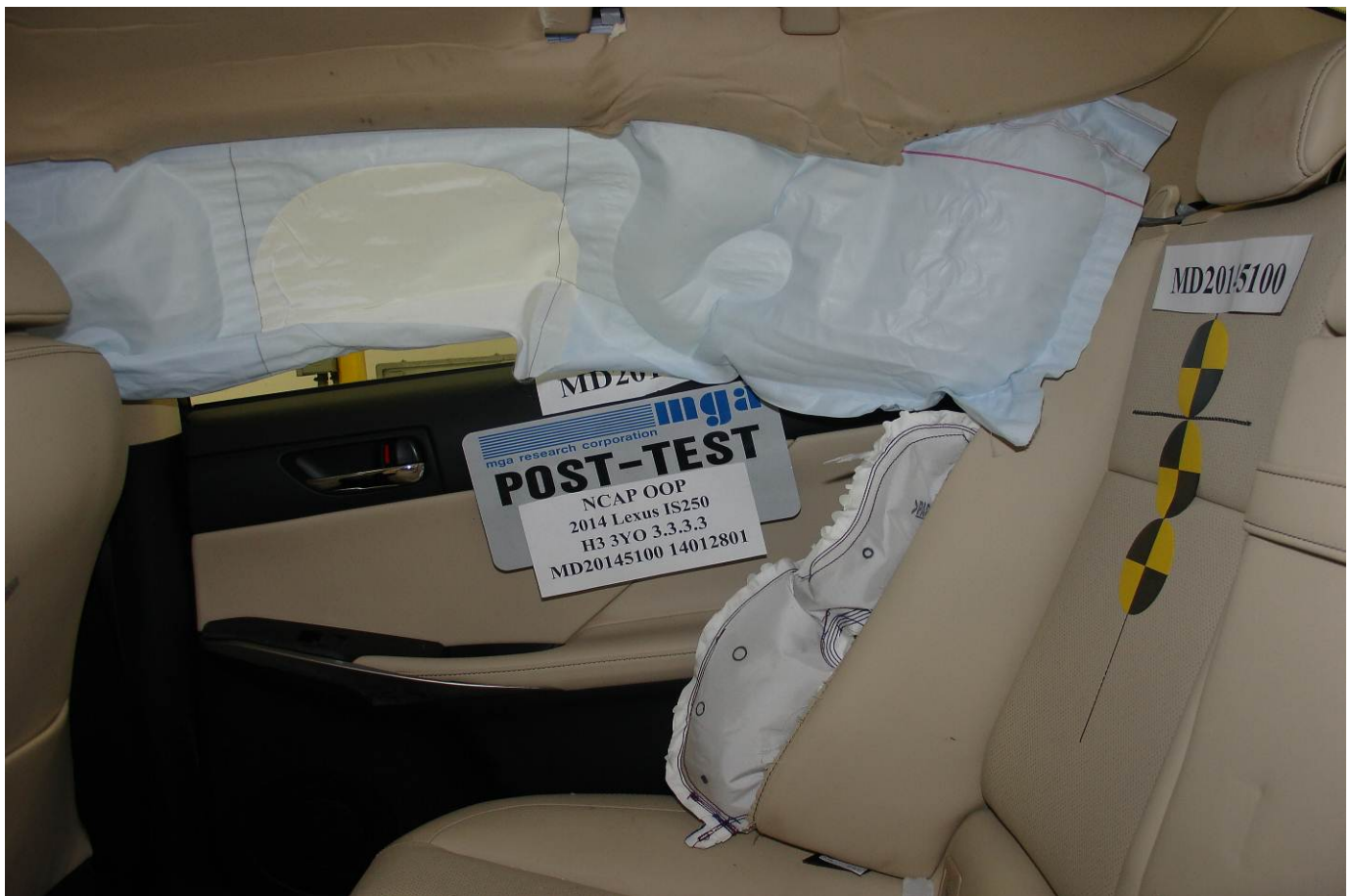
Post-Test Curtain Airbag Left Side View
