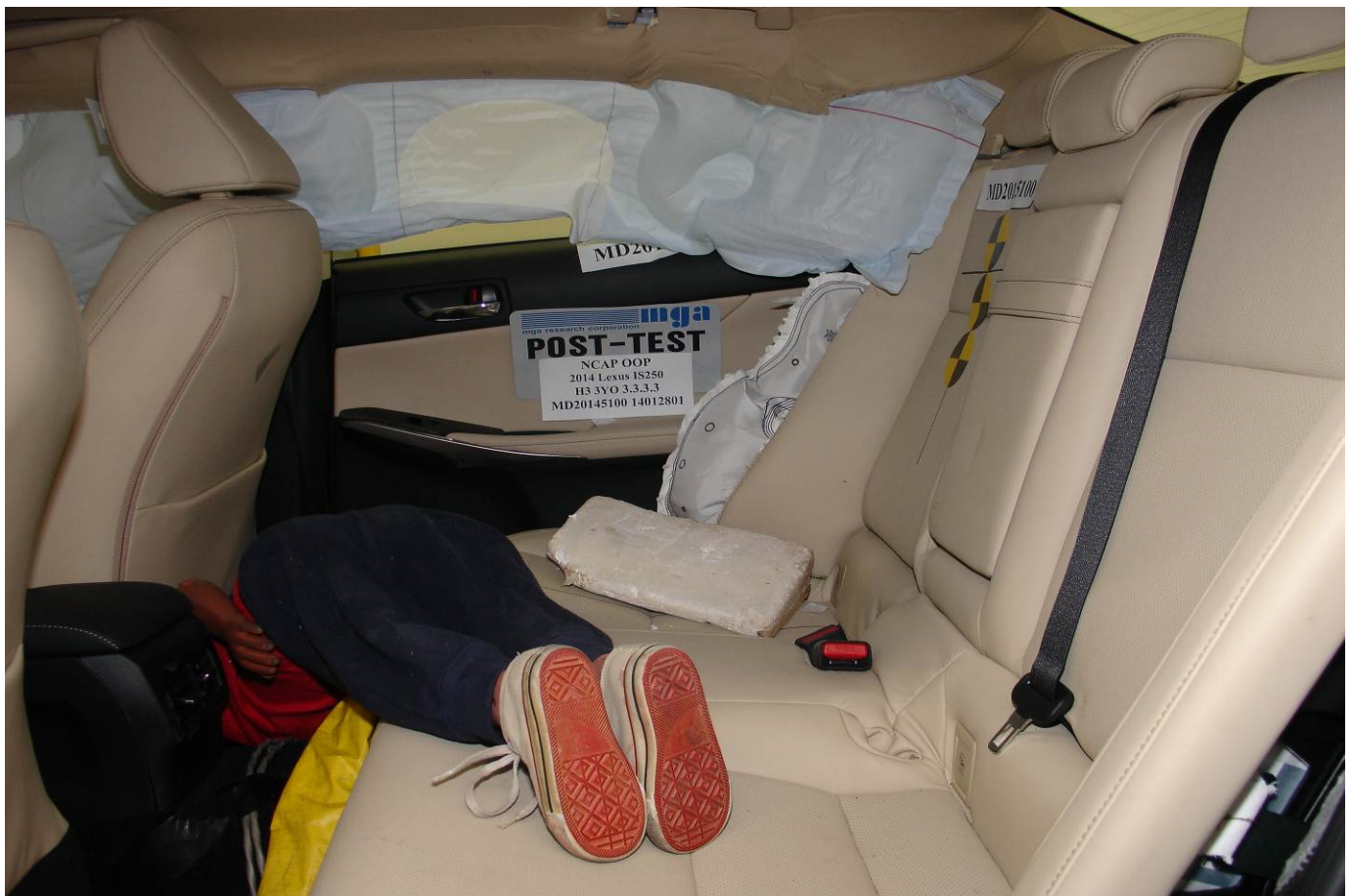
Post-Test 3-Year-Old Child Dummy Left Side View
