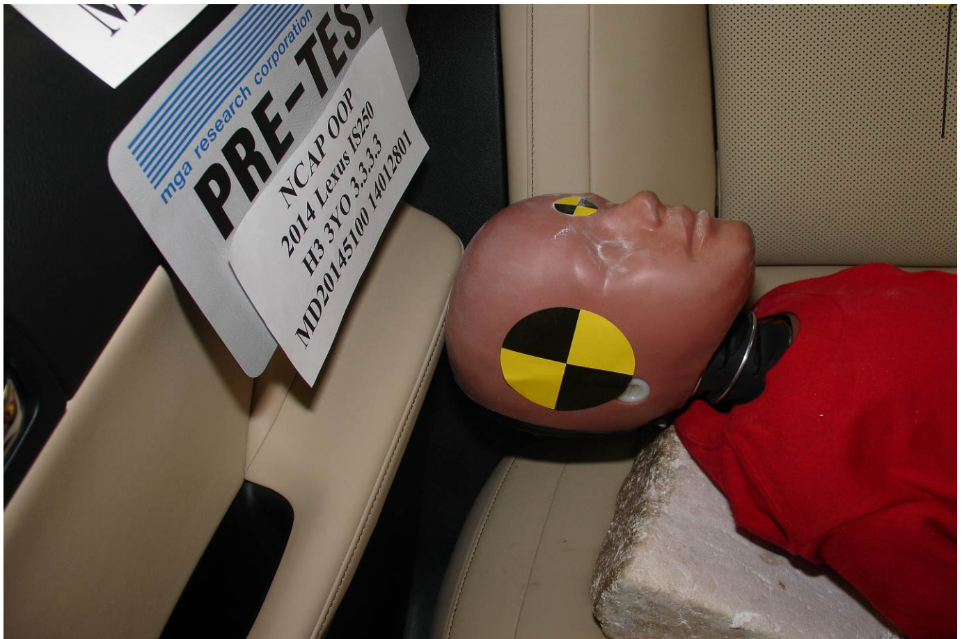
Pre-Test 3-Year-Old Child Dummy Front View
