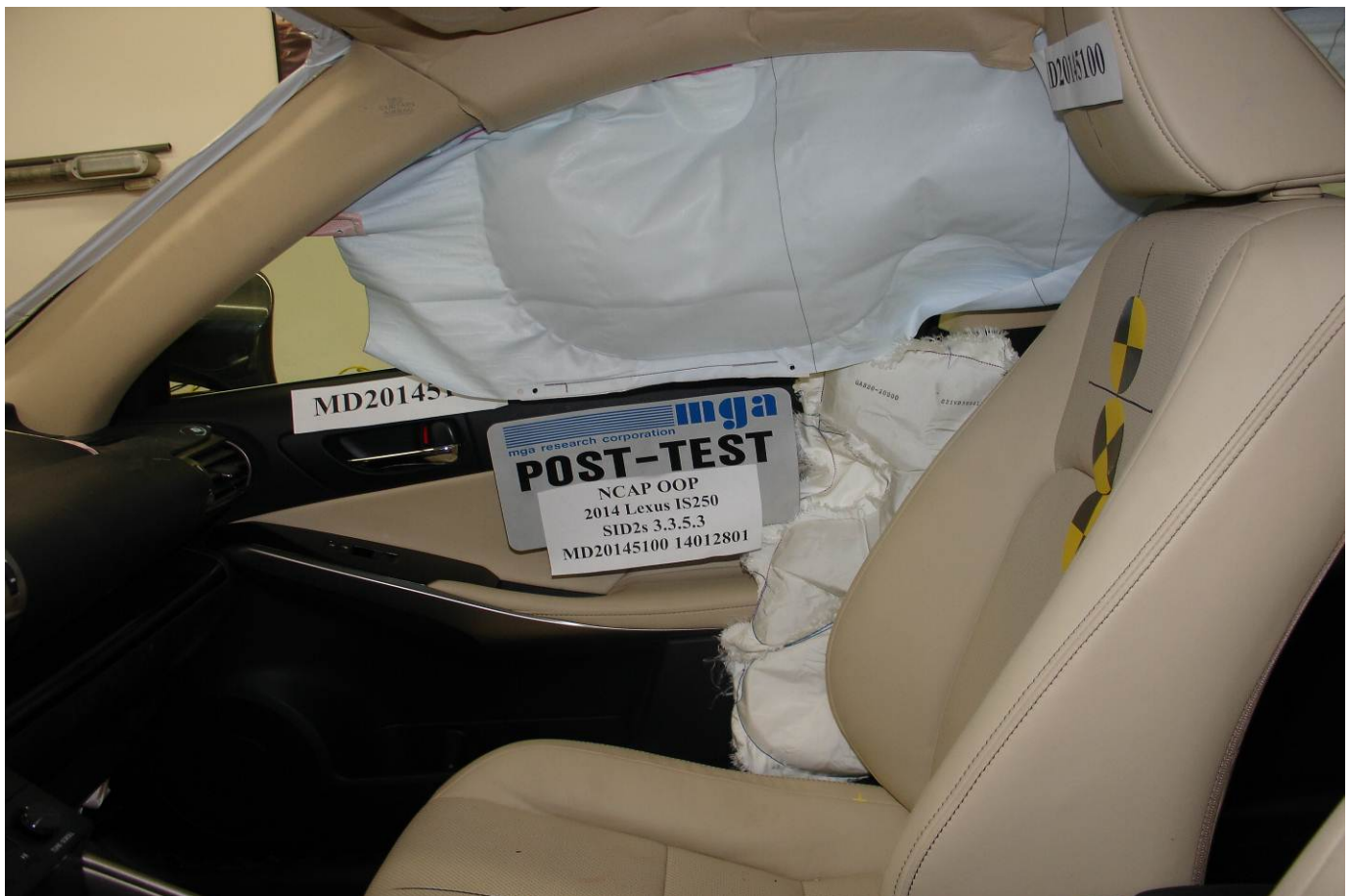
Post-Test Curtain Airbag Left Side View
