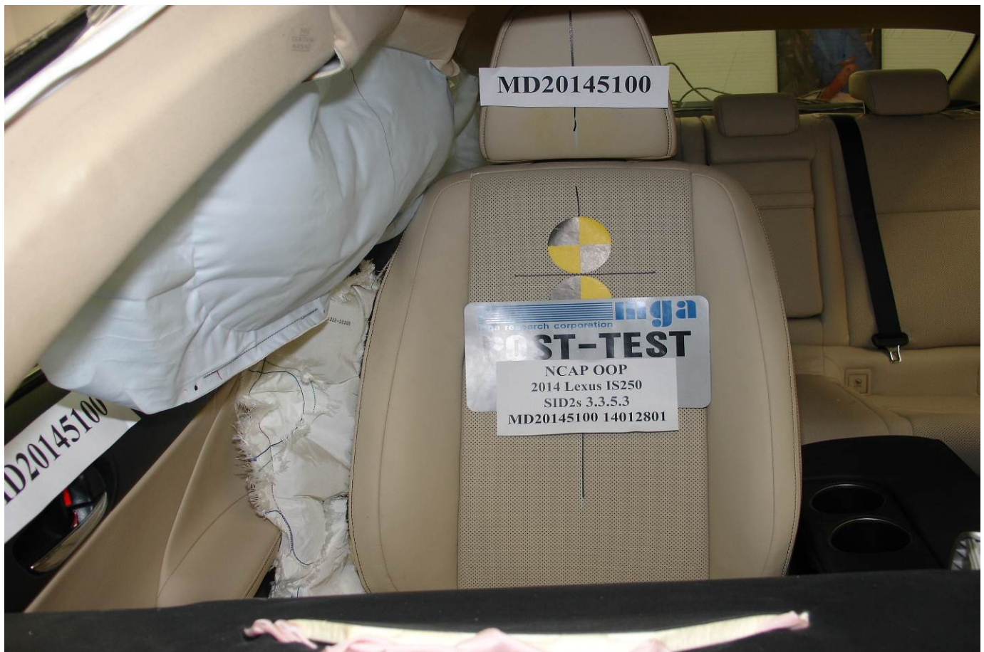
Post-Test Curtain Airbag Front View
