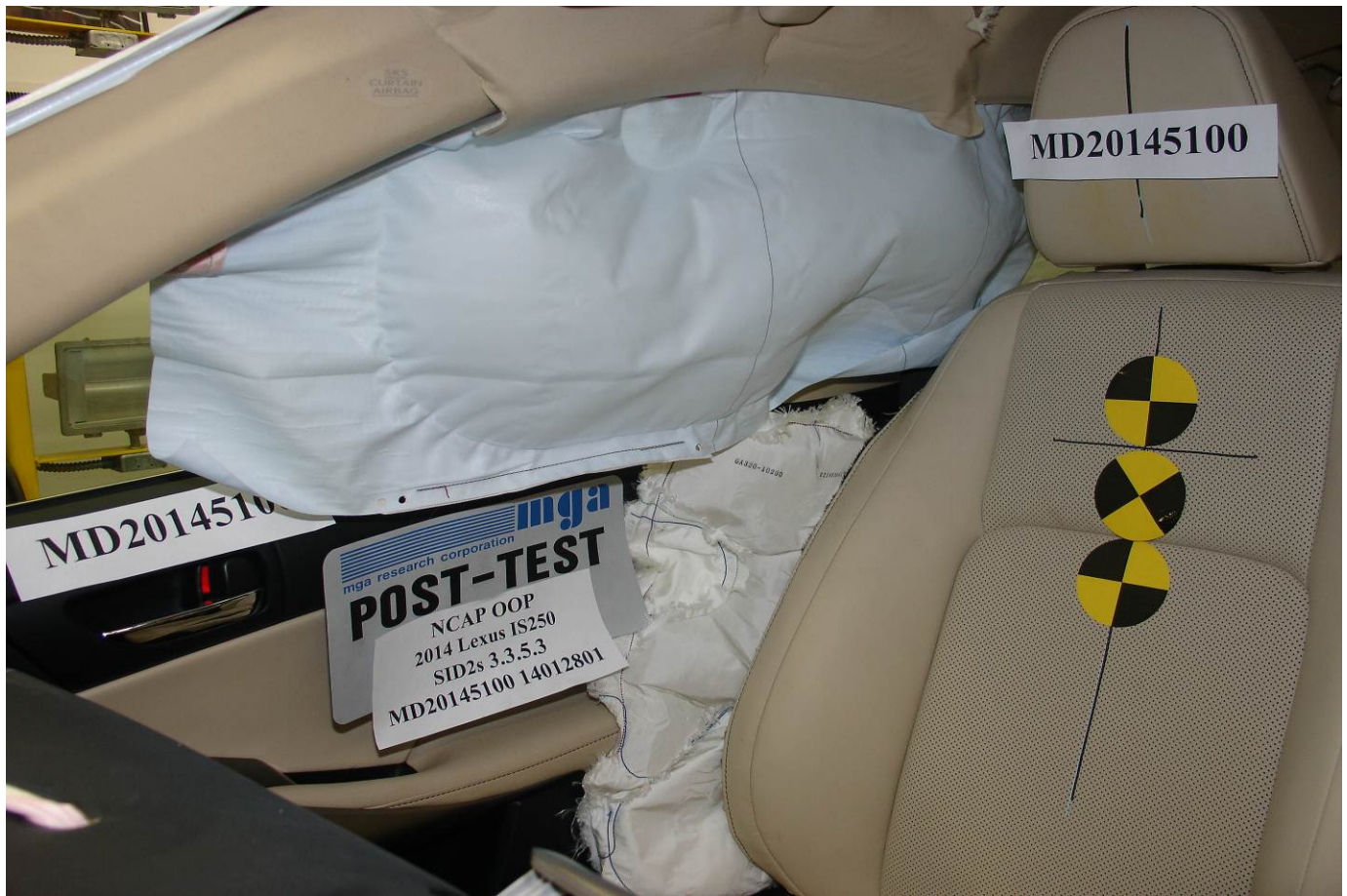
Post-Test Curtain Airbag Left 3/4 Front View
