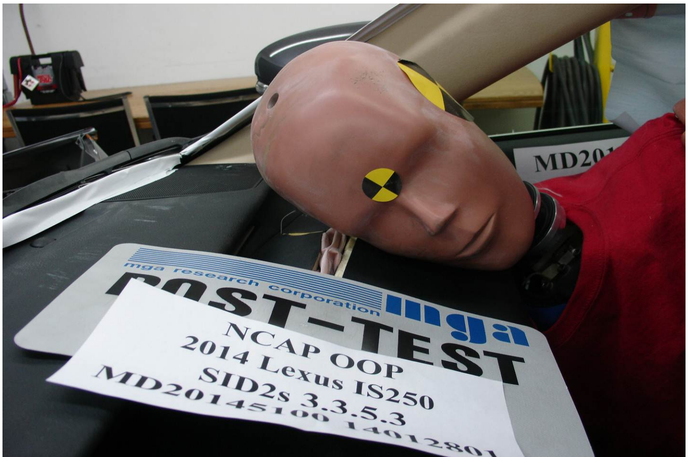
Post-Test SID-IIs Dummy Left Side Closeup View
