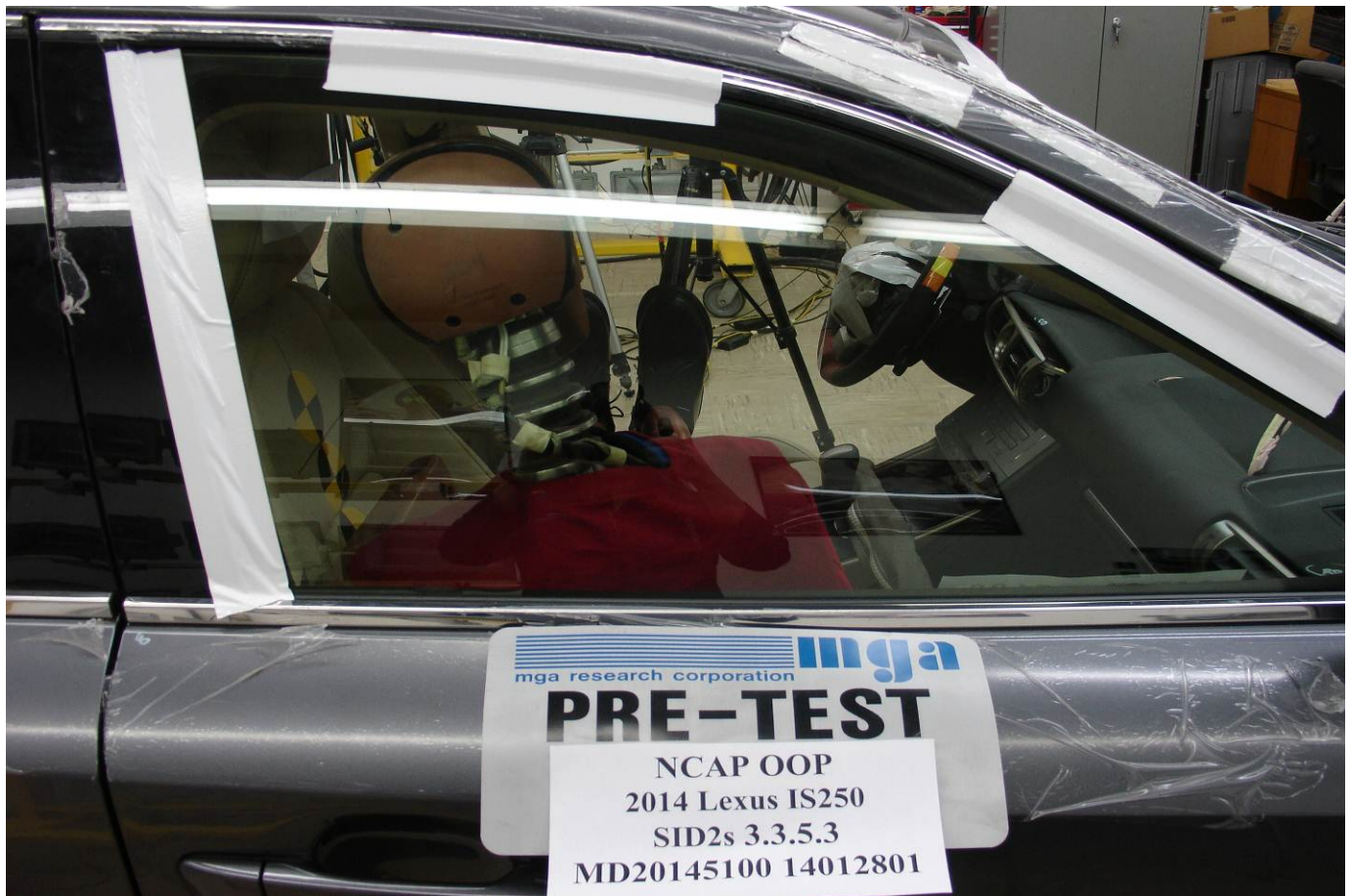
Pre-Test SID-IIs Dummy Right Side View
