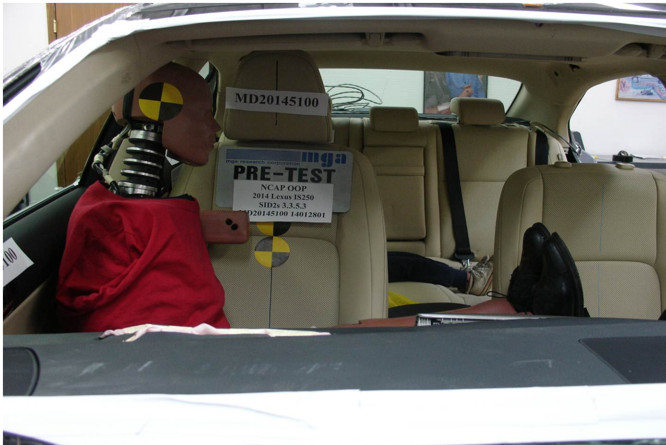
Pre-Test SID-IIs Dummy Front View
