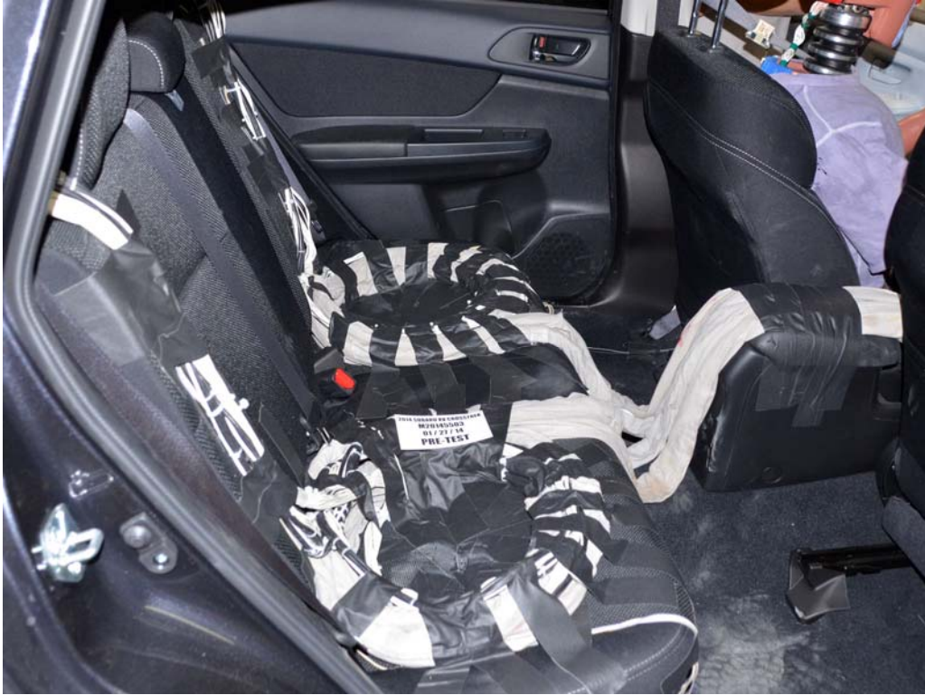
FIGURE 27. Pre-Test Dummy Cable Routing
