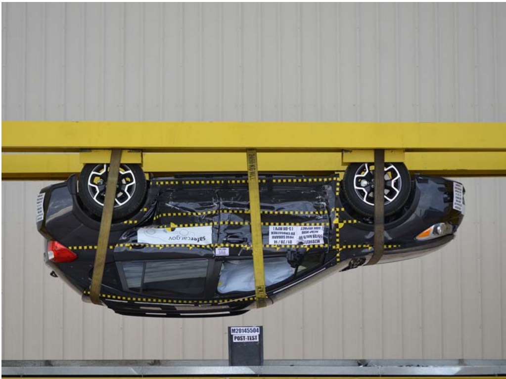
FIGURE 98. FMVSS No. 301 Static Rollover 180 Degrees
