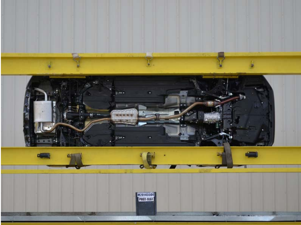
FIGURE 99. FMVSS No. 301 Static Rollover 270 Degrees
