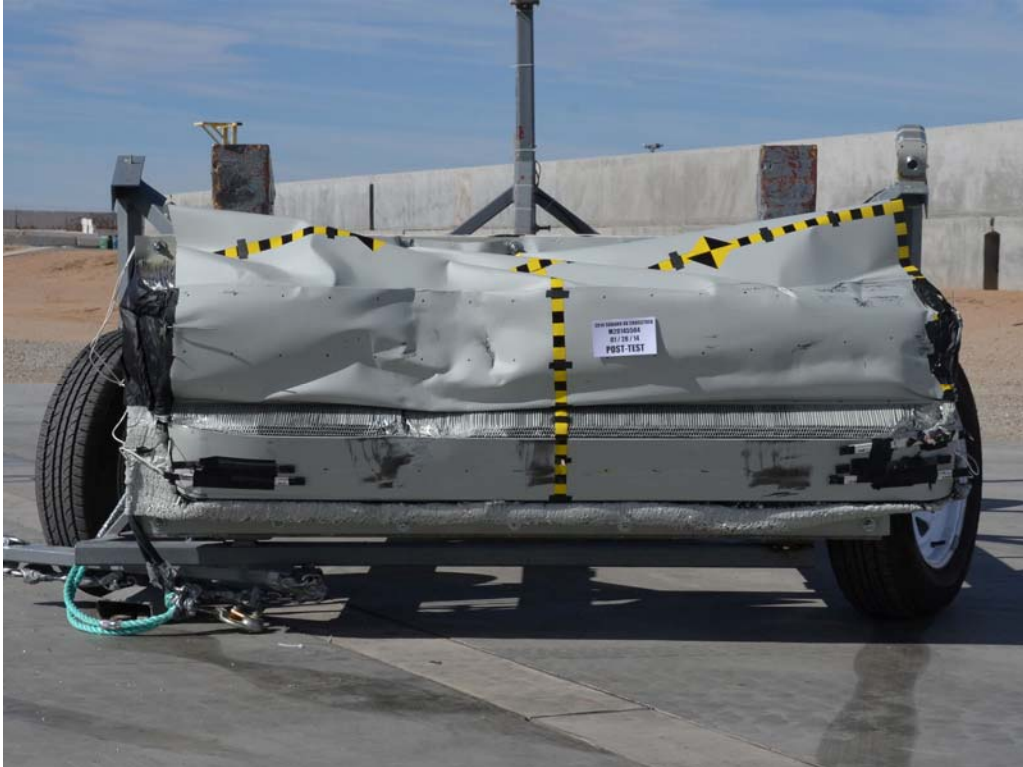
FIGURE 85. Post-Test Front View of MDB Impactor Face
