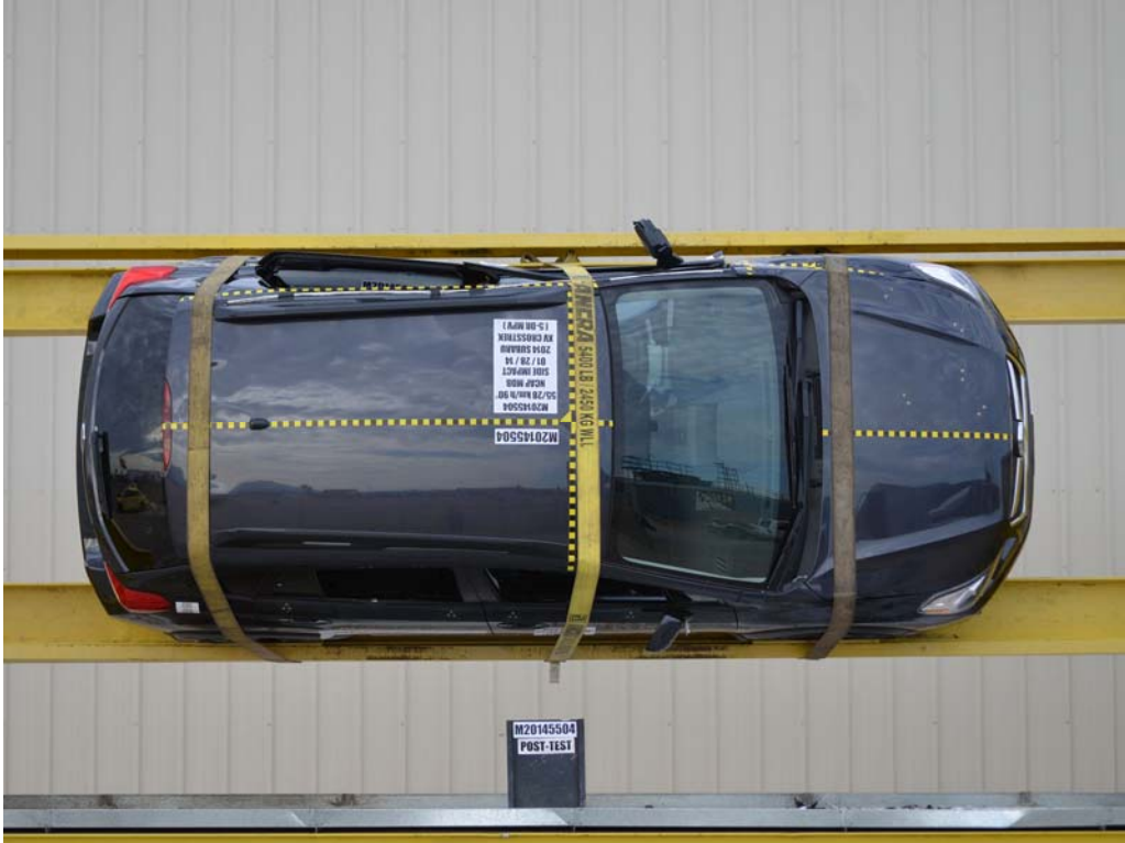
FIGURE 97. FMVSS No. 301 Static Rollover 90 Degrees
