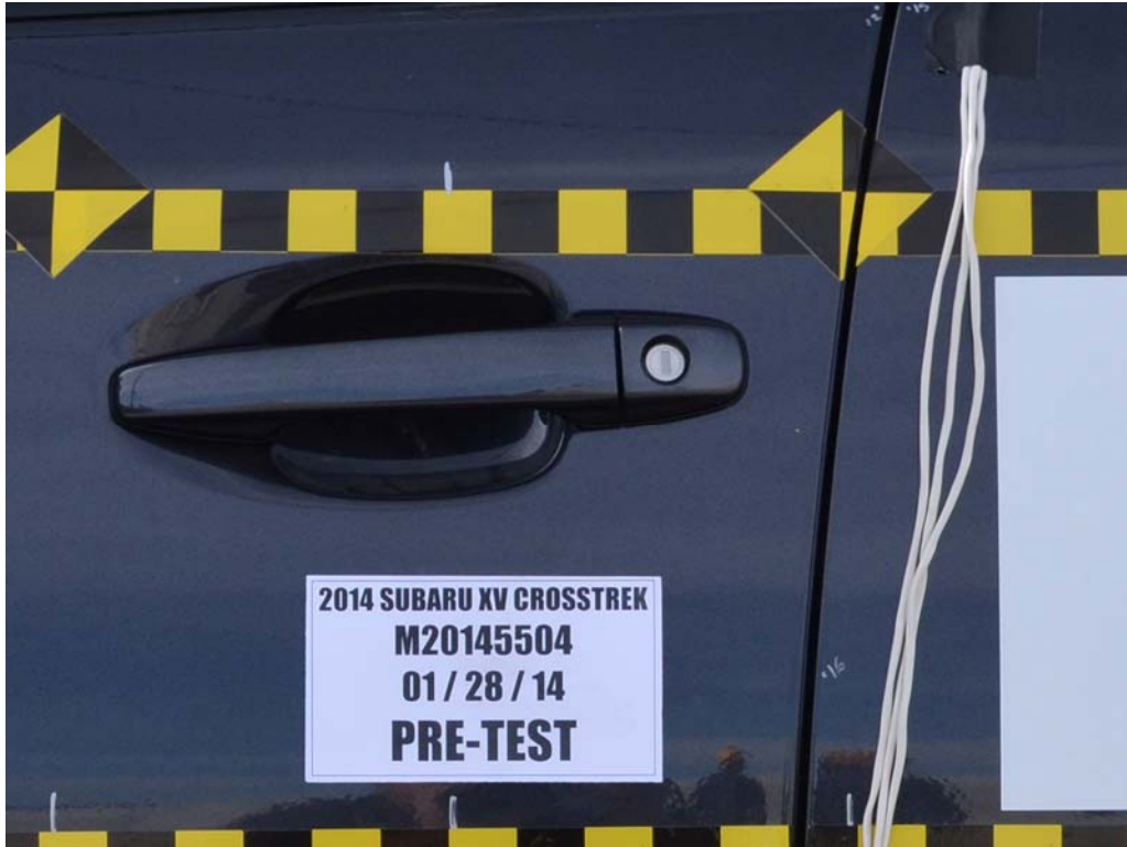
FIGURE 21. Pre-Test Left Front Door Latch Close-Up
