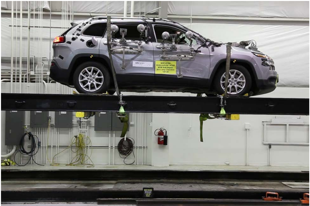
100 FMVSS No. 301 Static Rollover 360 Degrees
