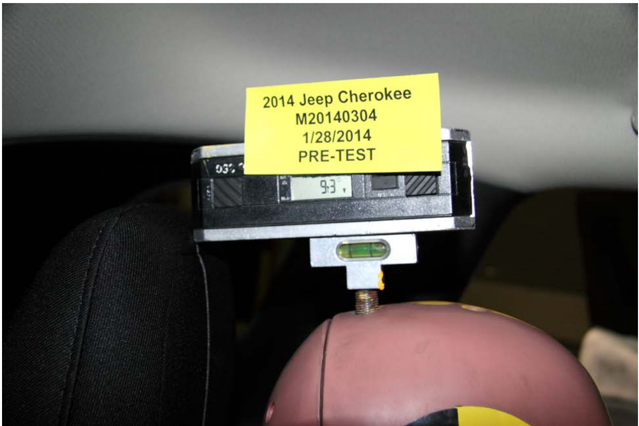
063 Pre-Test View of Rear Passenger Dummy's Head Showing Dummy's Head is Level
