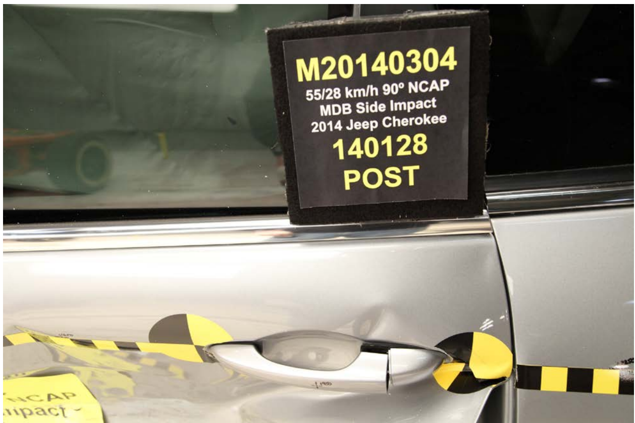
024 Post-Test Left Rear Door Latch Close-up
