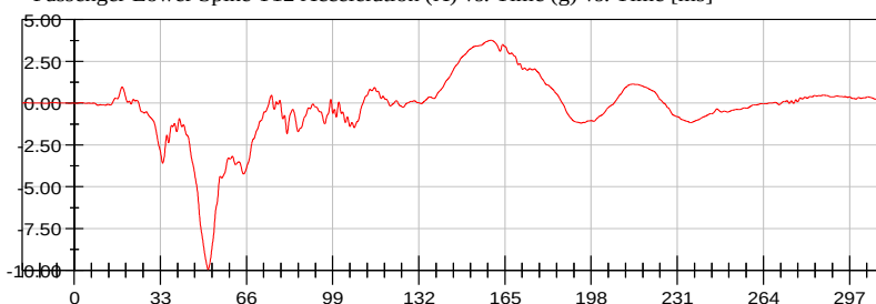
Passenger Lower Spine T12 Acceleration (Y) vs. Time (g) vs. Time [ms]
