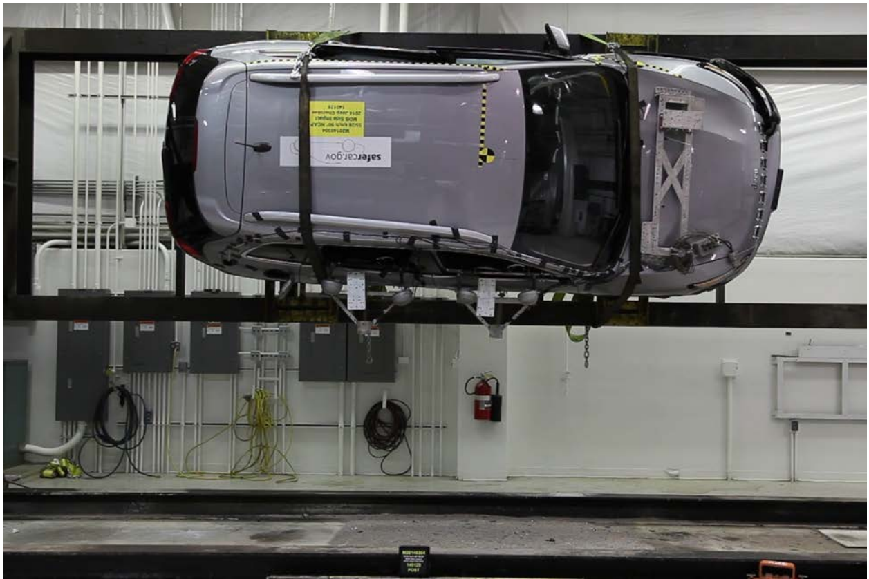
097 FMVSS No. 301 Static Rollover 90 Degrees
