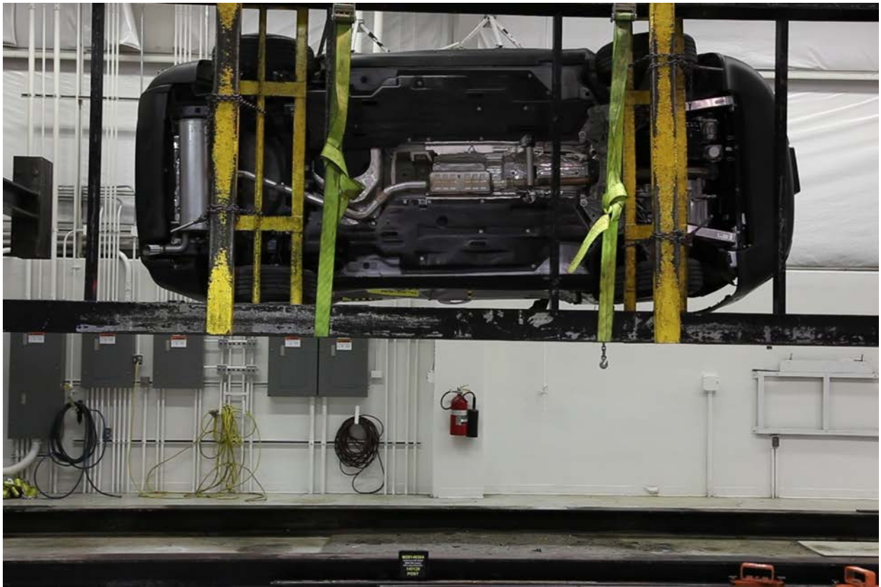
099 FMVSS No. 301 Static Rollover 270 Degrees
