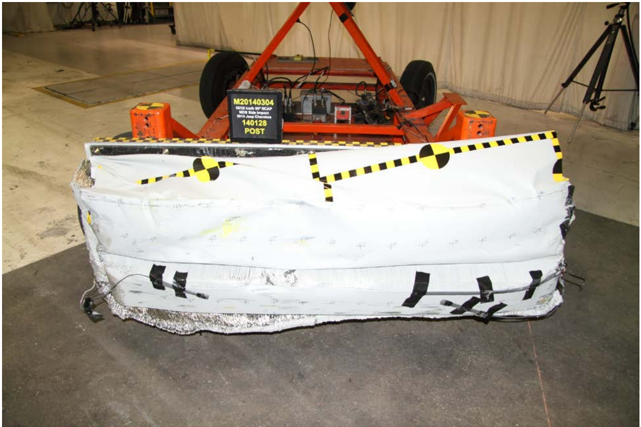
085 Post-Test Front View of MDB Impactor Face
