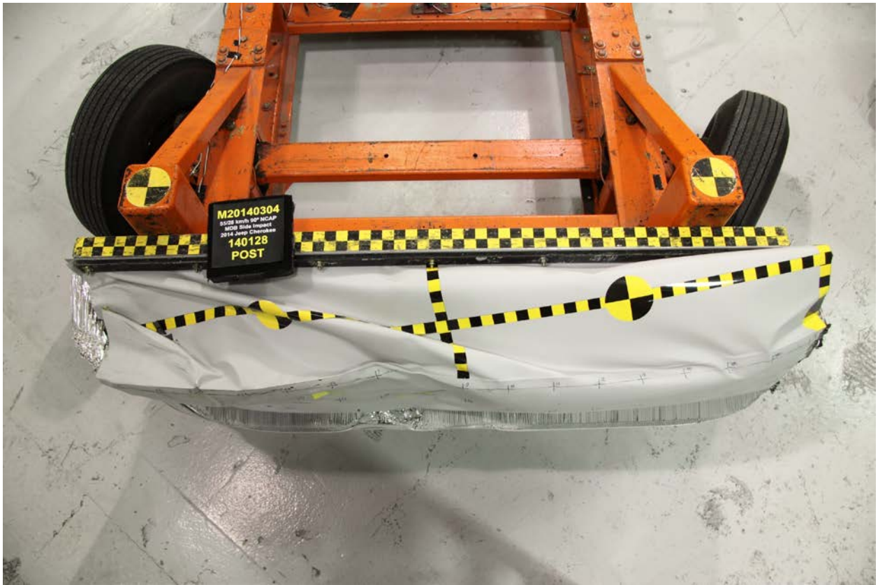
087 Post-Test Top View of MDB Impactor Face
