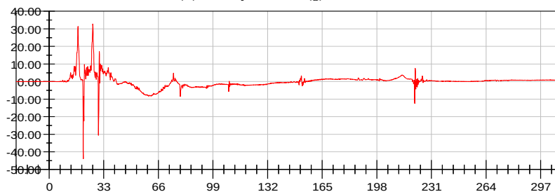
Driver Head Resultant Acceleration Primary vs. Time (g) vs. Time [ms]
