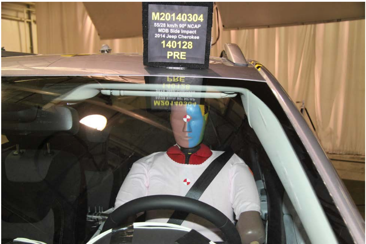
025 Pre-Test Front Close-up View of Driver Dummy
