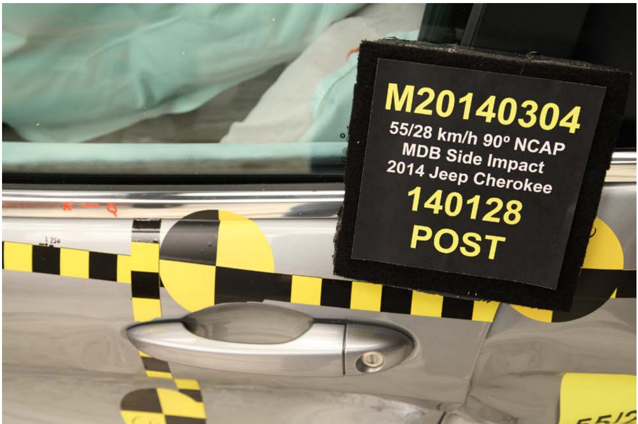
022 Post-Test Left Front Door Latch Close-up
