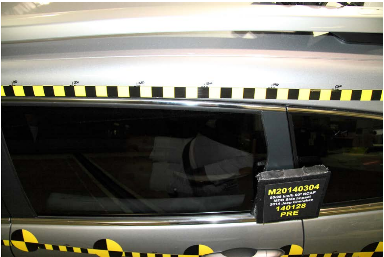
069 Pre-Test Passenger Dummy and Door Clearance View
