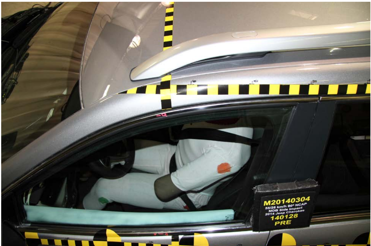
042 Pre-Test Driver Dummy and Door Clearance View
