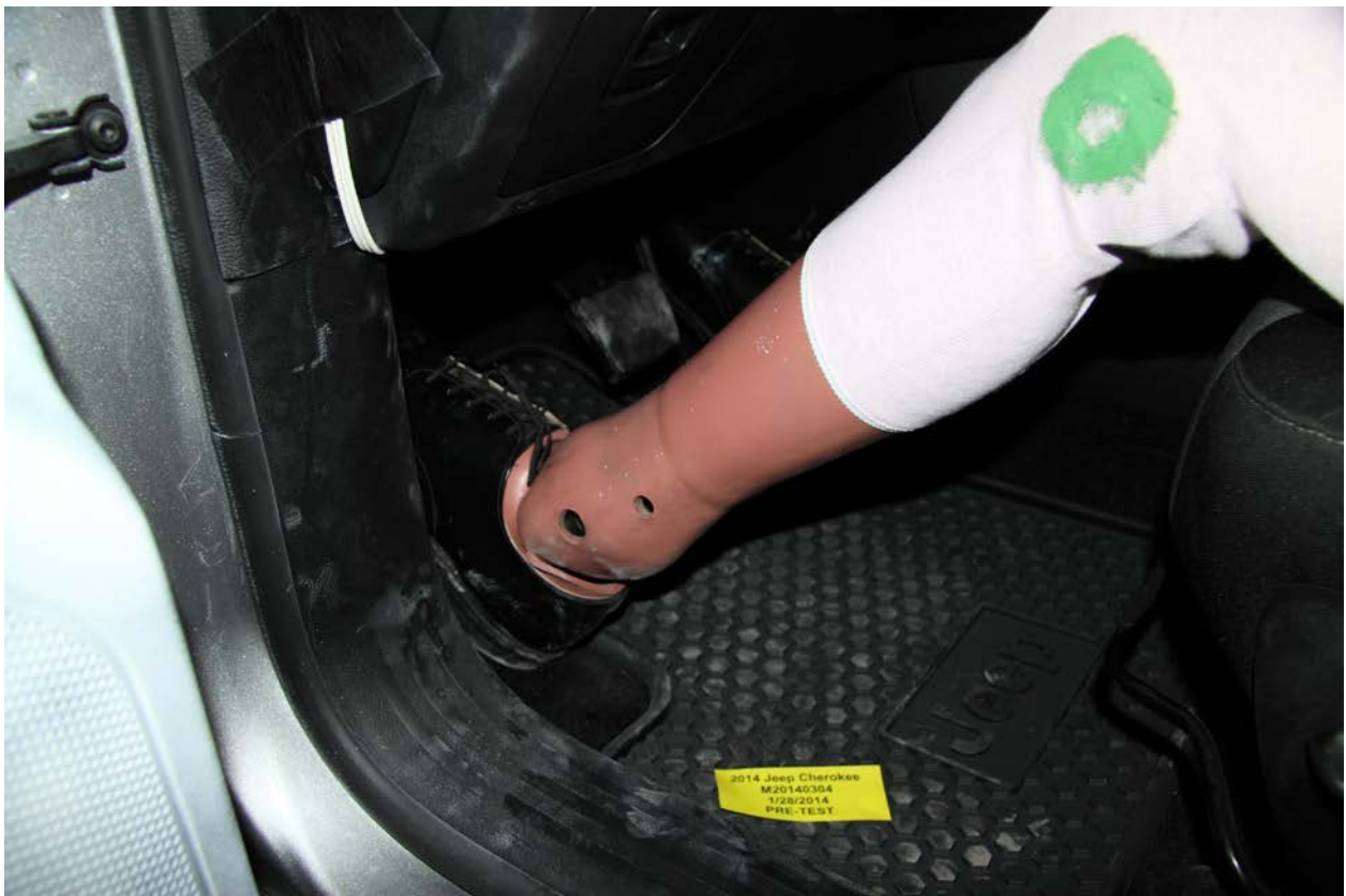
034 Pre-Test Placement of Driver Dummy Feet
