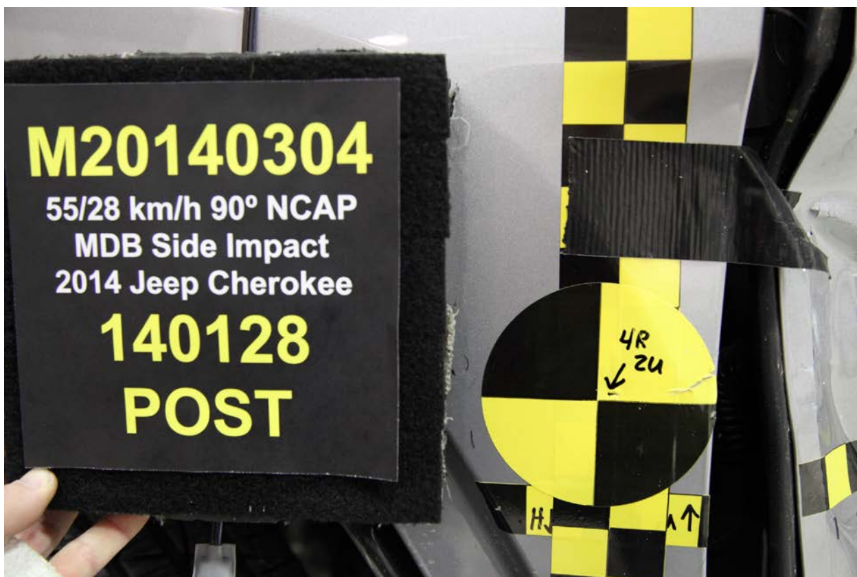
020 Post-Test Close-up View of Impact Point Target
