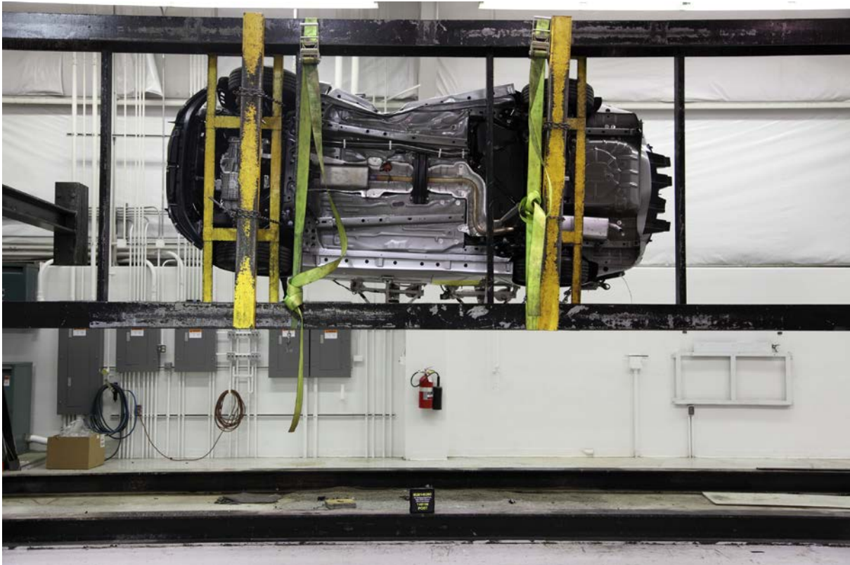
066 FMVSS No. 301 Static Rollover 270 Degrees
