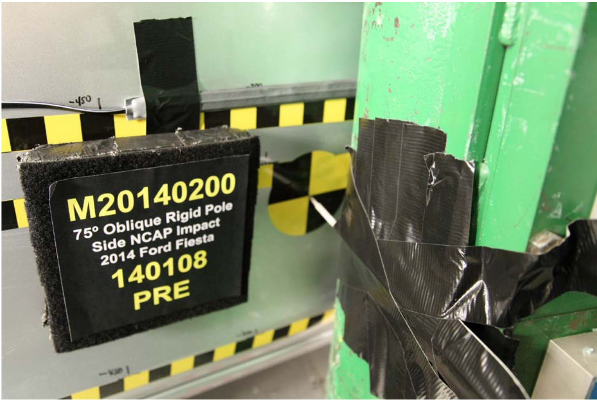
019 Pre-Test Close-Up View of Impact Point Target
