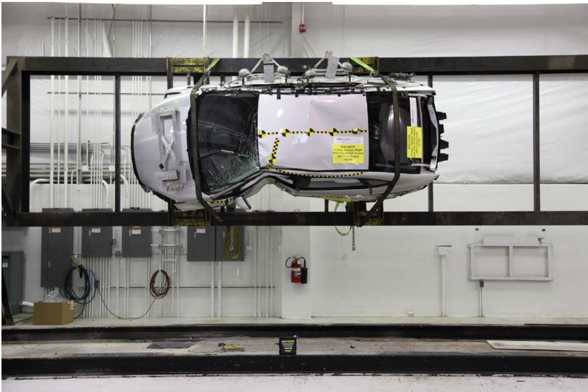
064 FMVSS No. 301 Static Rollover 90 Degrees
