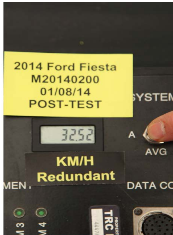
062 Post-Test Primary and Redundant Speed Trap Read-Out
