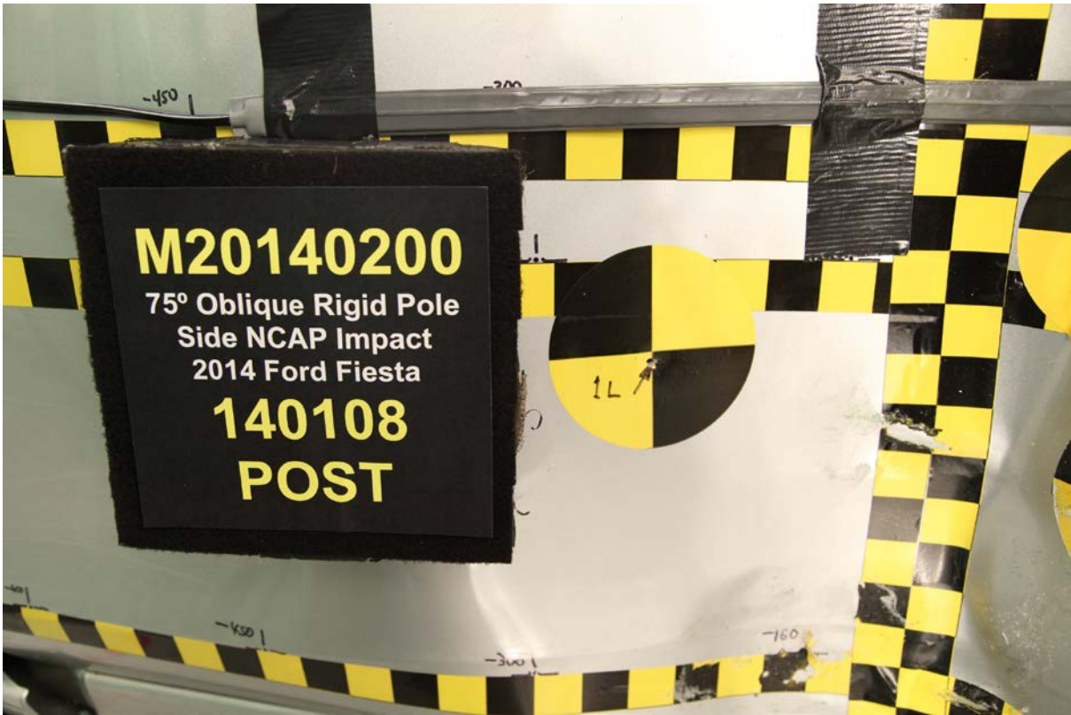
020 Post-Test Close-Up View of Impact Point Target Showing Impact Location
