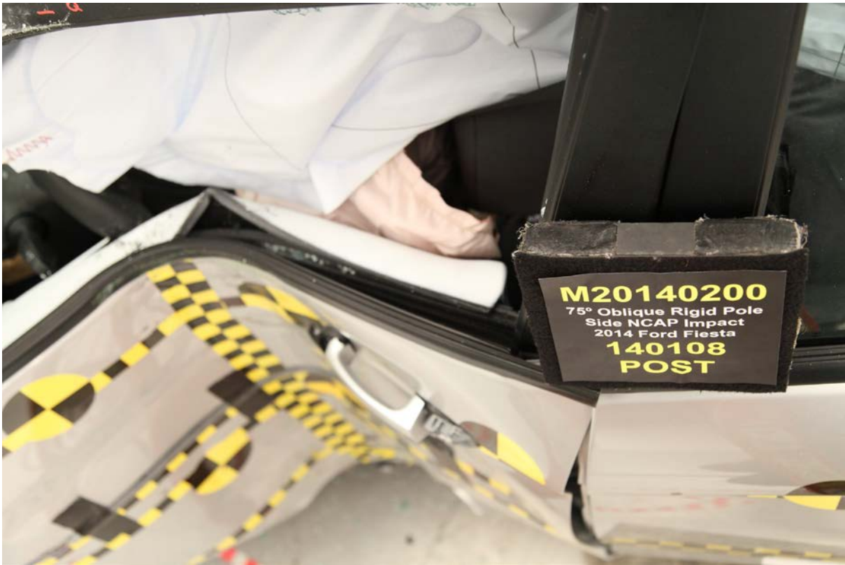
041 Post-Test Dummy and Door Clearance View
