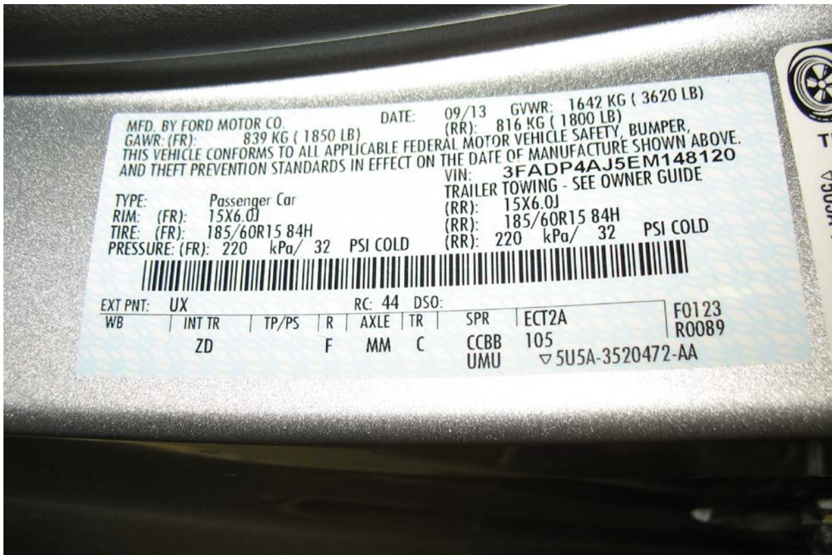
055 Close-Up View of Vehicle Certification Label
