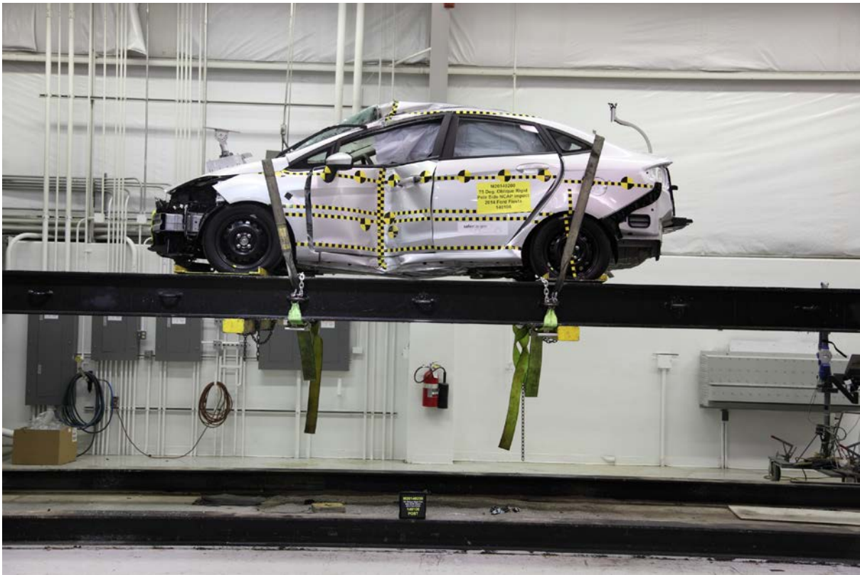
067 FMVSS No. 301 Static Rollover 360 Degrees
