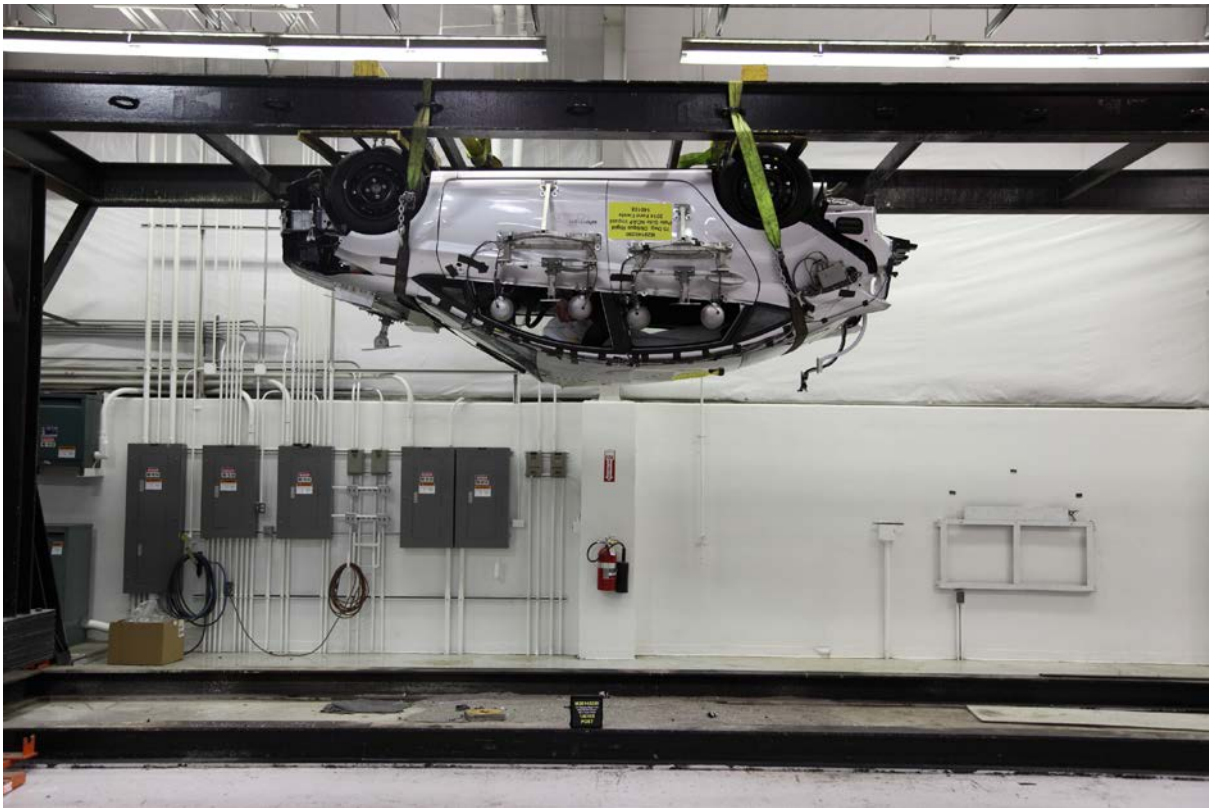
065 FMVSS No. 301 Static Rollover 180 Degrees
