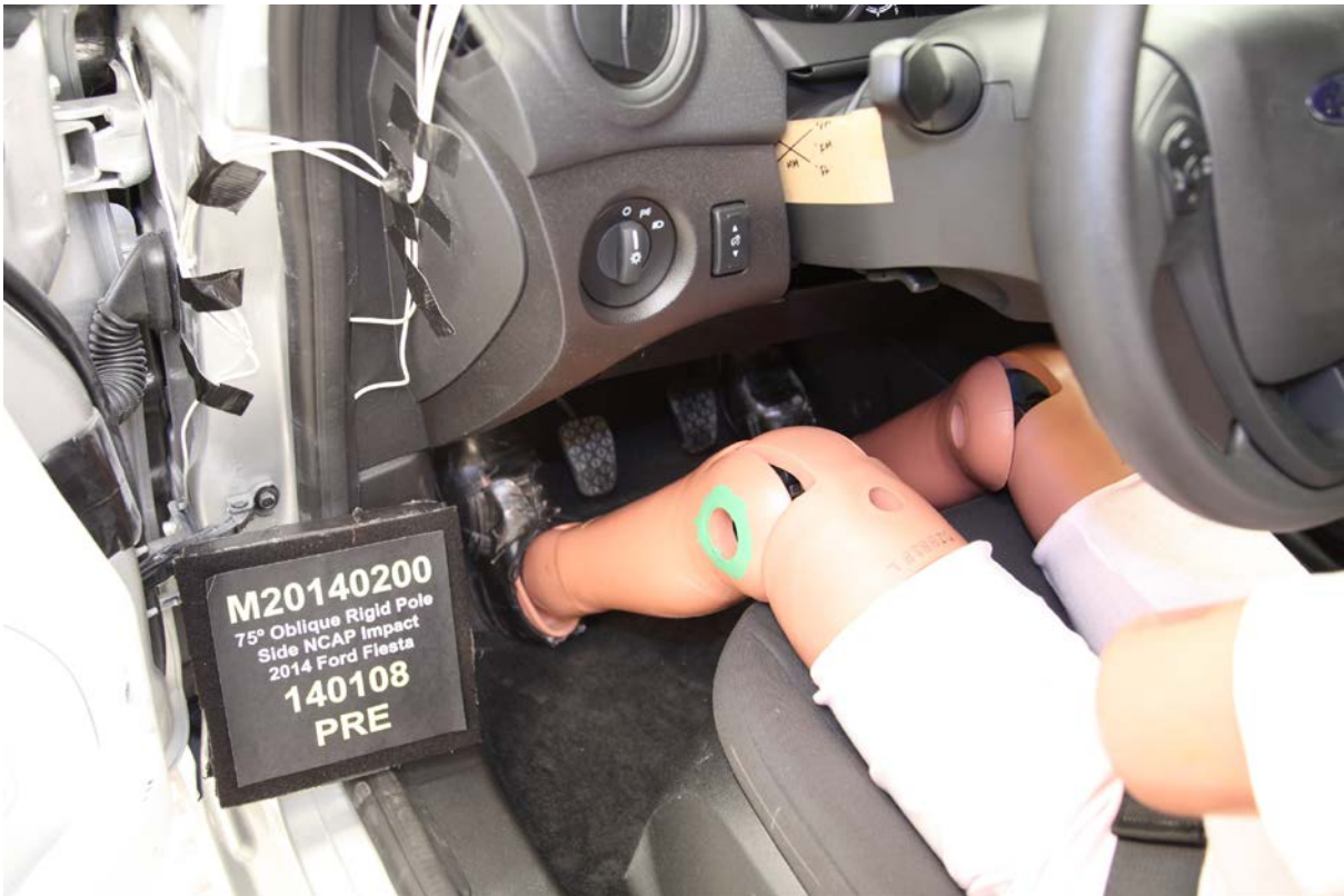
032 Pre-Test Placement of Dummy Feet
