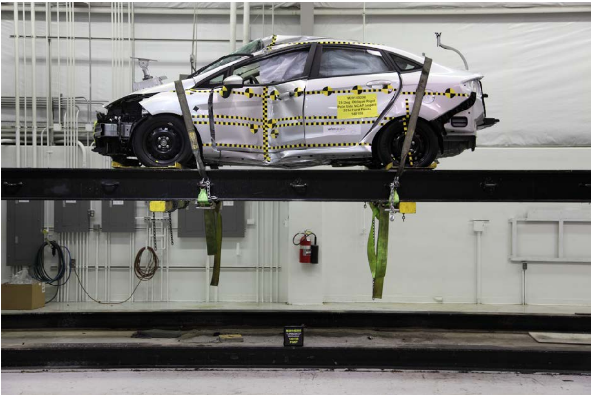
063 FMVSS No. 301 Static Rollover 0 Degrees
