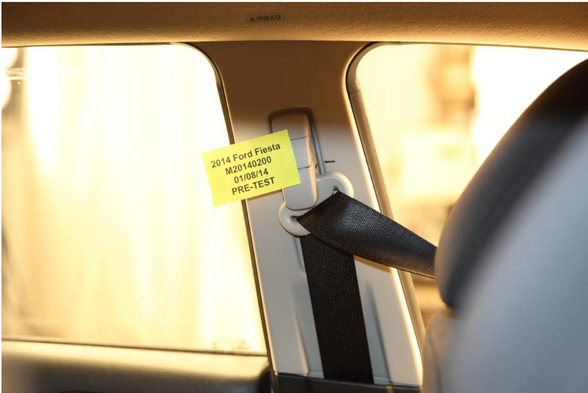
033 Pre-Test View of Belt Anchorage for Dummy
