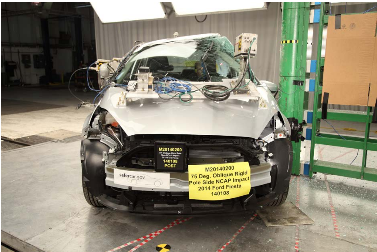
004 Post-Test Frontal View of Test Vehicle
