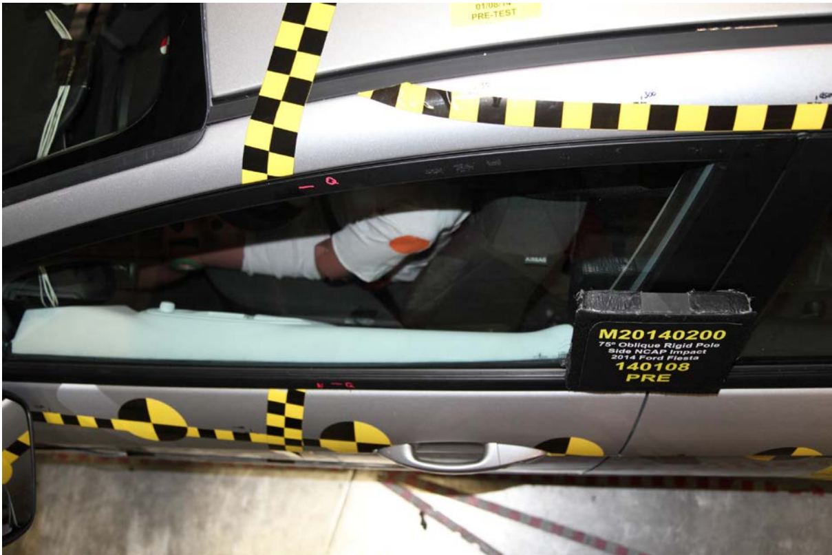
040 Pre-Test Dummy and Door Clearance View
