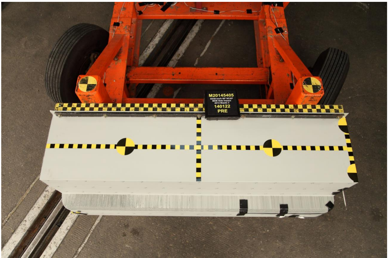
086 Pre-Test Top View of MDB Impactor Face
