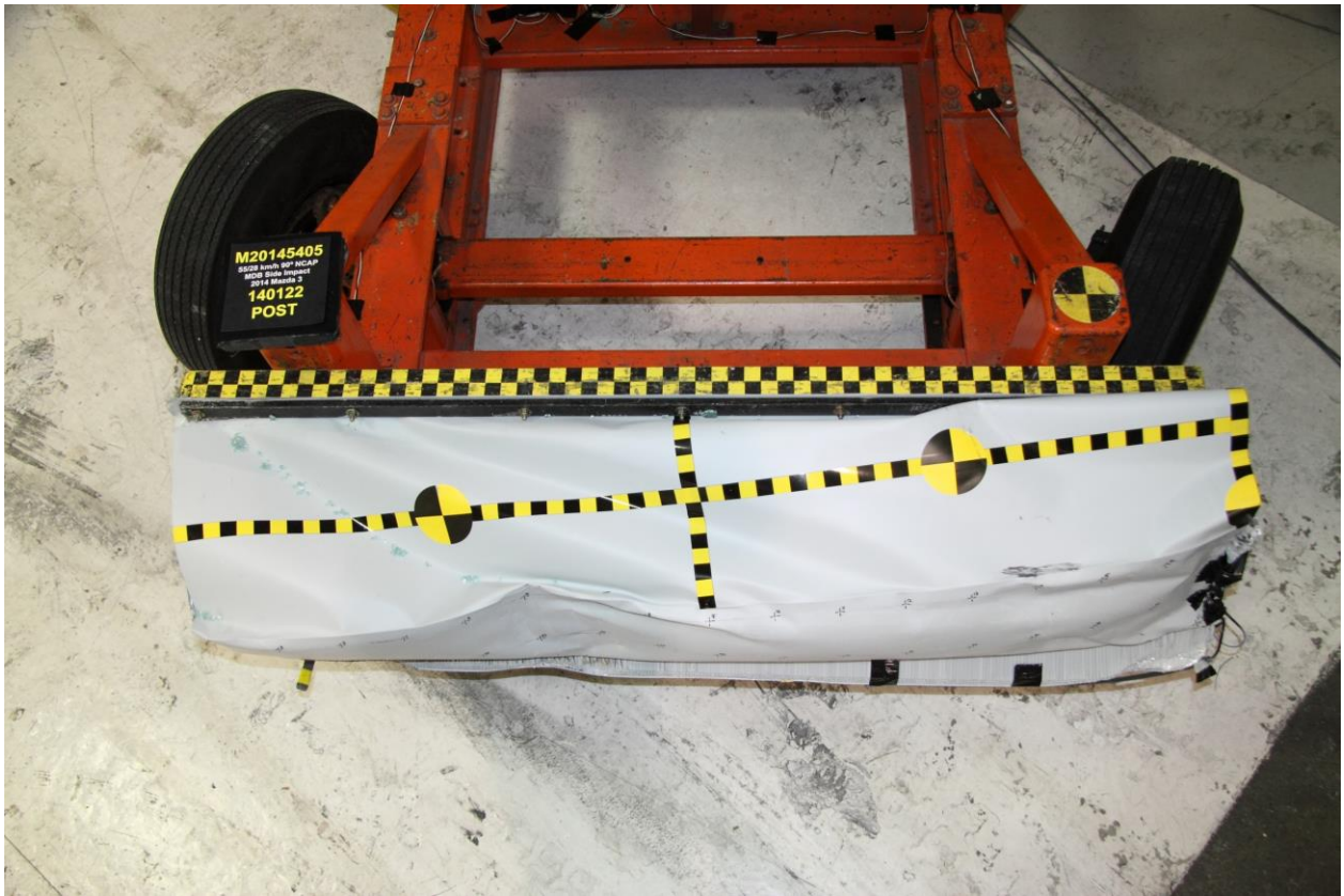
087 Post-Test Top View of MDB Impactor Face
