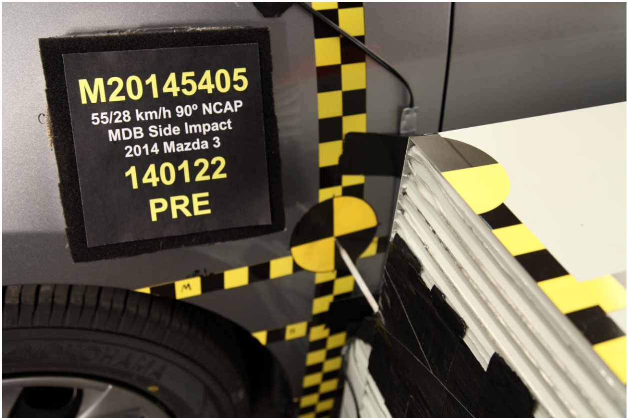
019 Pre-Test Close-up View of Impact Point Target
