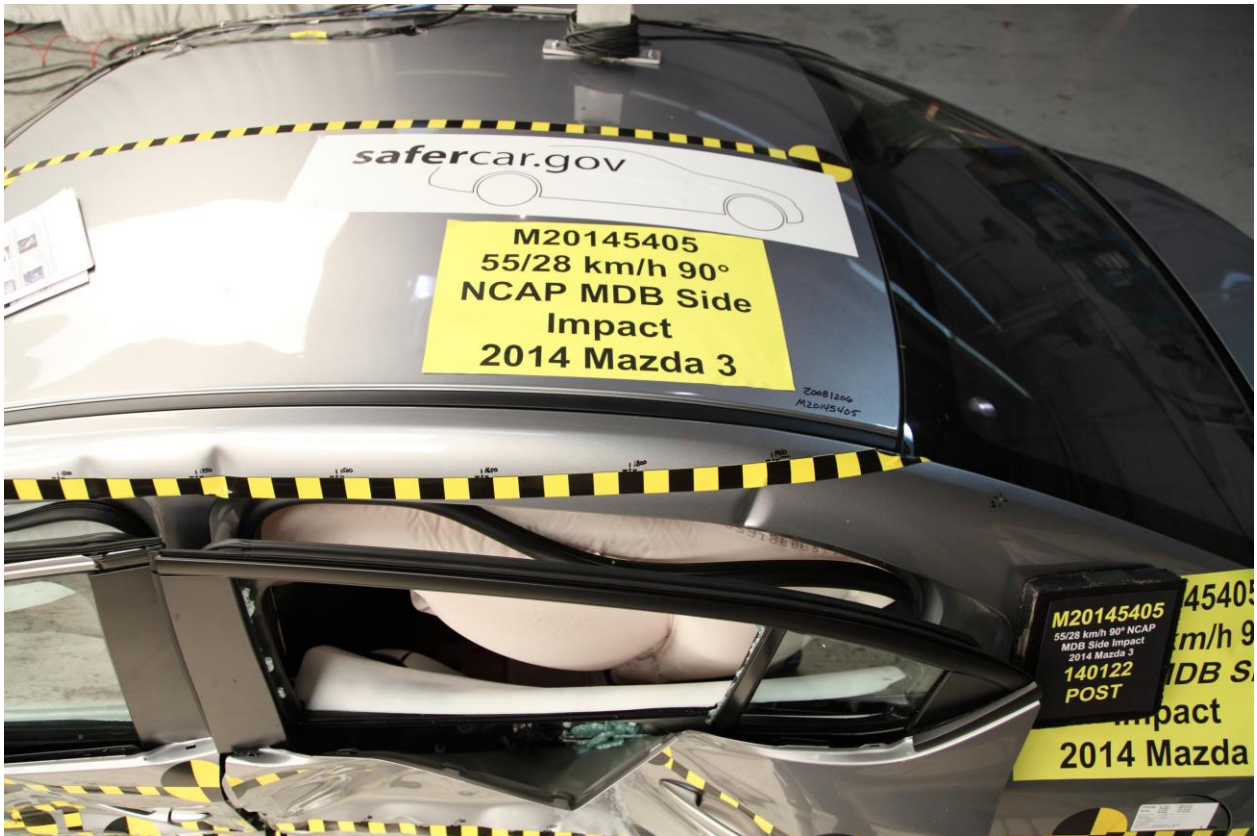
070 Post-Test Passenger Dummy and Door Clearance View
