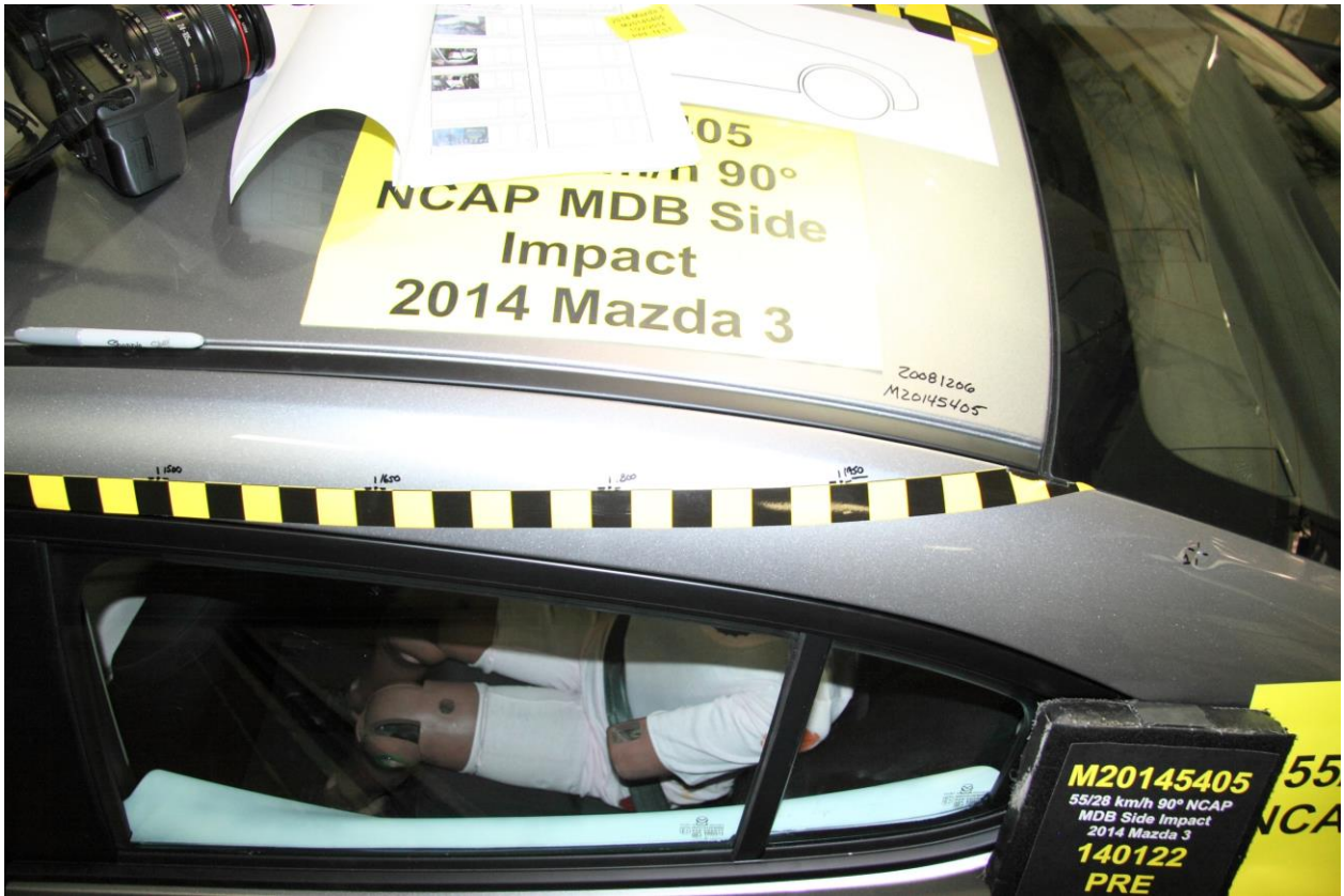
069 Pre-Test Passenger Dummy and Door Clearance View
