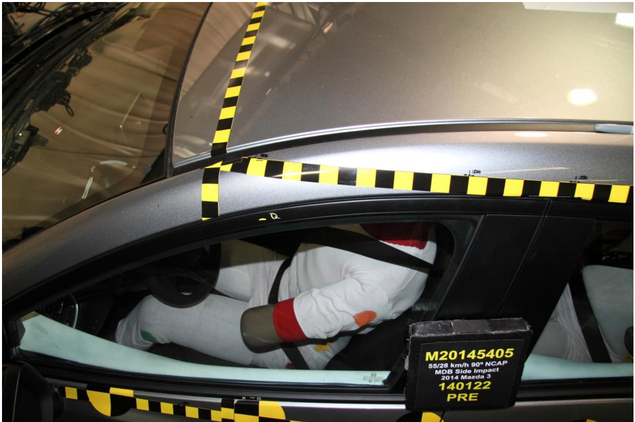
042 Pre-Test Driver Dummy and Door Clearance View
