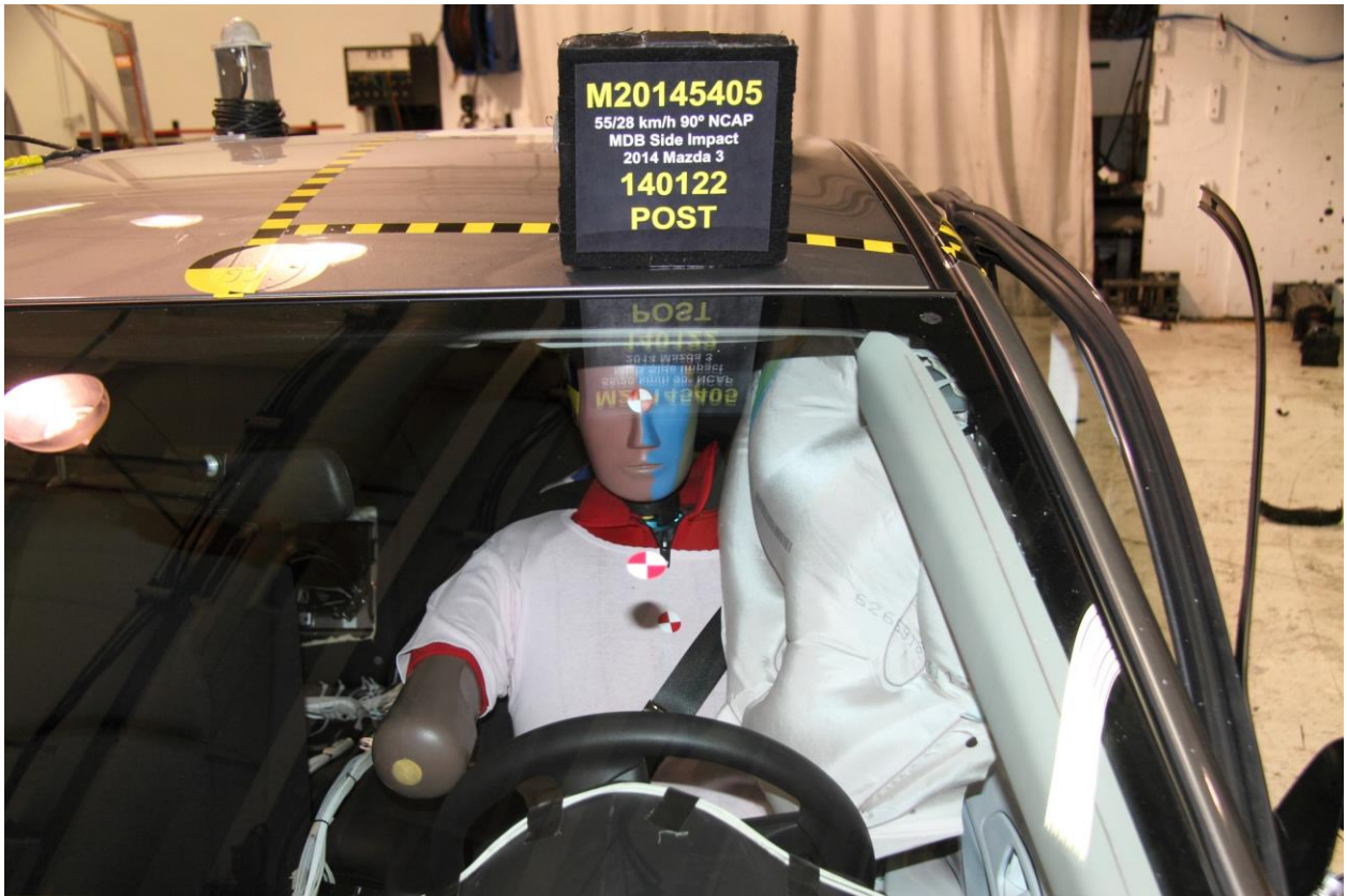
026 Post-Test Front Close-up View of Driver Dummy
