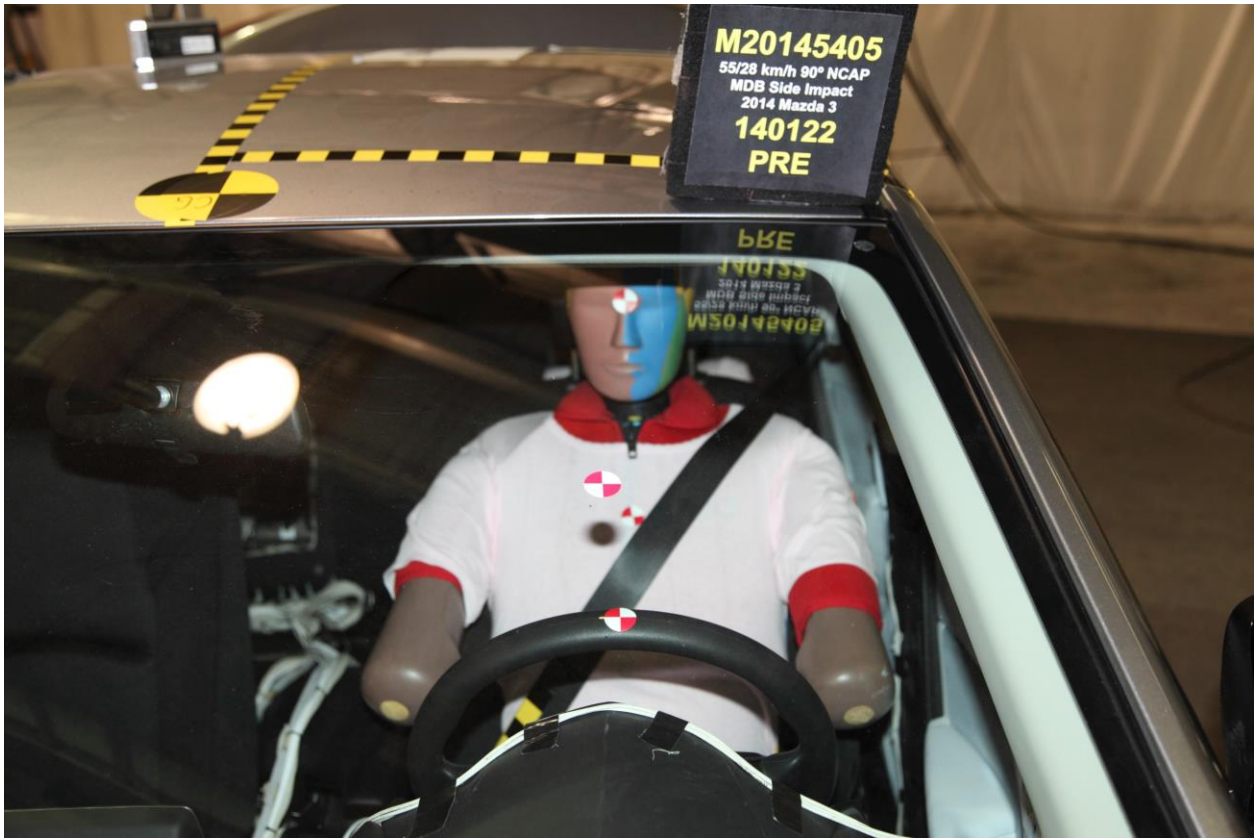
025 Pre-Test Front Close-up View of Driver Dummy
