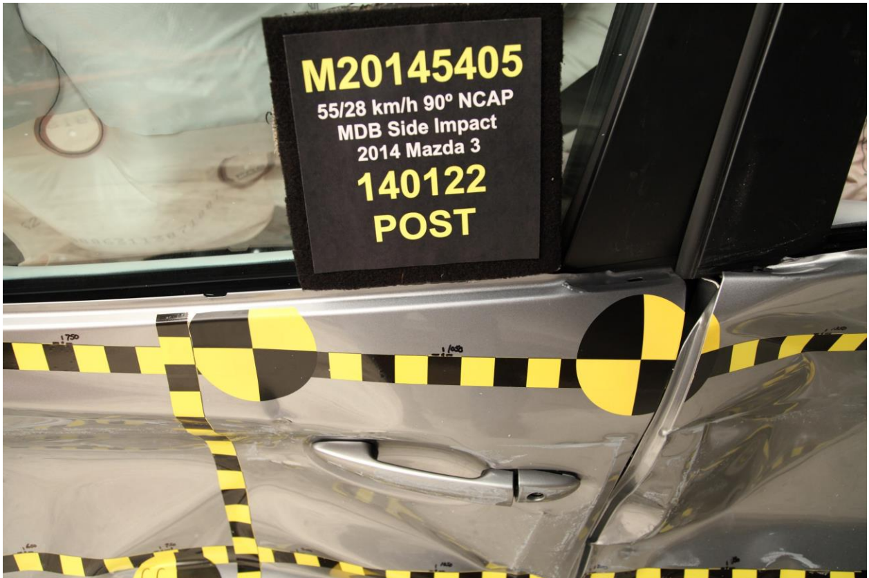
022 Post-Test Left Front Door Latch Close-up
