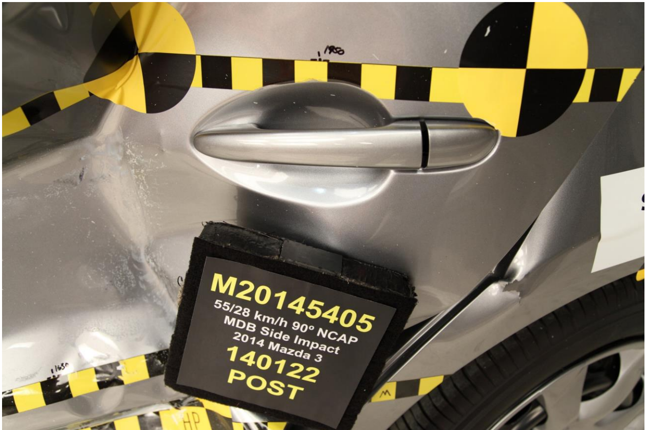
024 Post-Test Left Rear Door Latch Close-up
