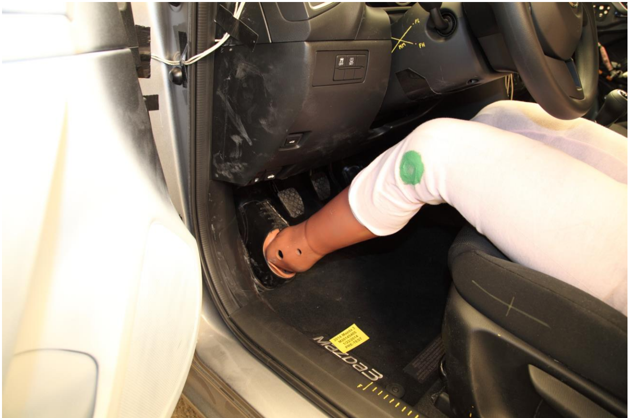
034 Pre-Test Placement of Driver Dummy Feet
