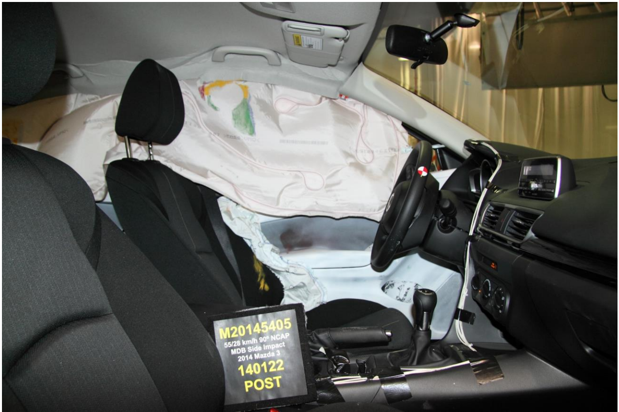
047 Post-Test Driver Inner Door Panel View
