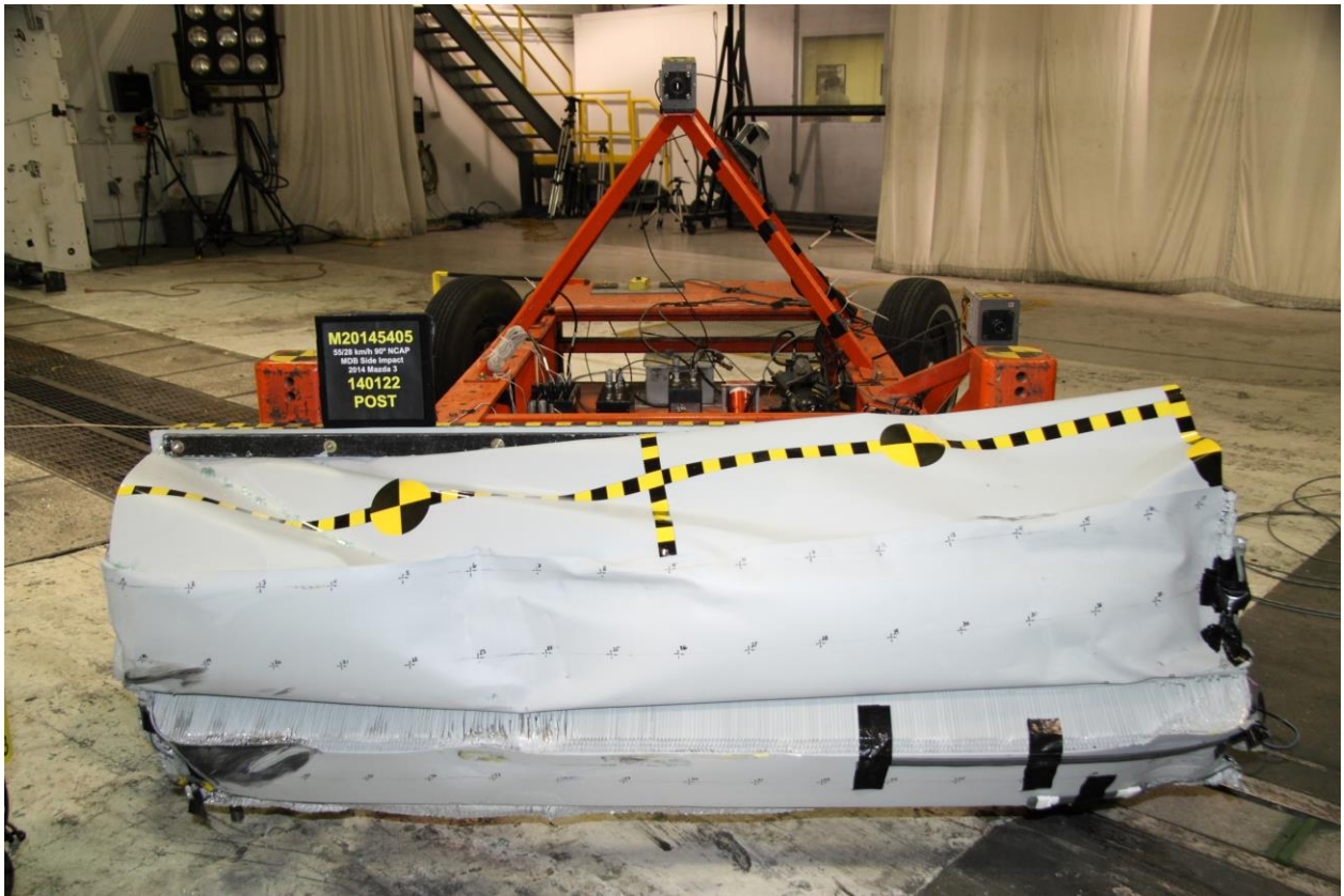
085 Post-Test Front View of MDB Impactor Face
