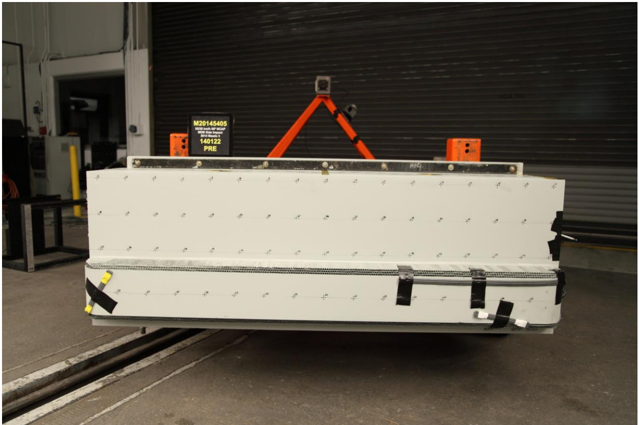
084 Pre-Test Front View of MDB Impactor Face
