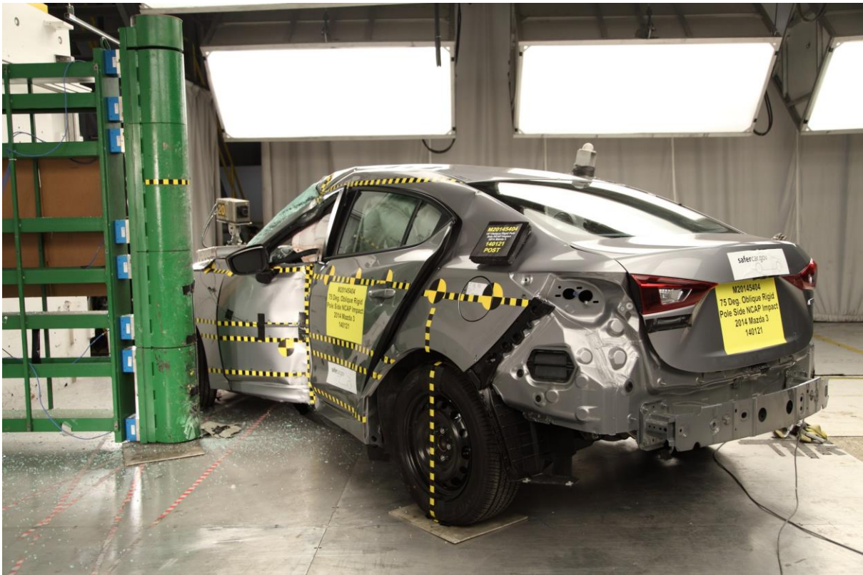
010 Post-Test Left Rear 3-4 View of Test Vehicle
