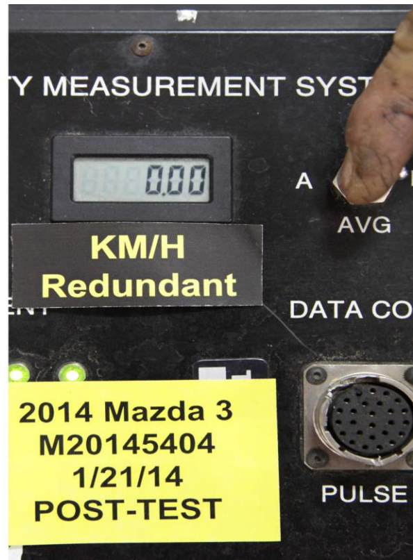
062 Post-Test Primary and Redundant Speed Trap Read-Out
