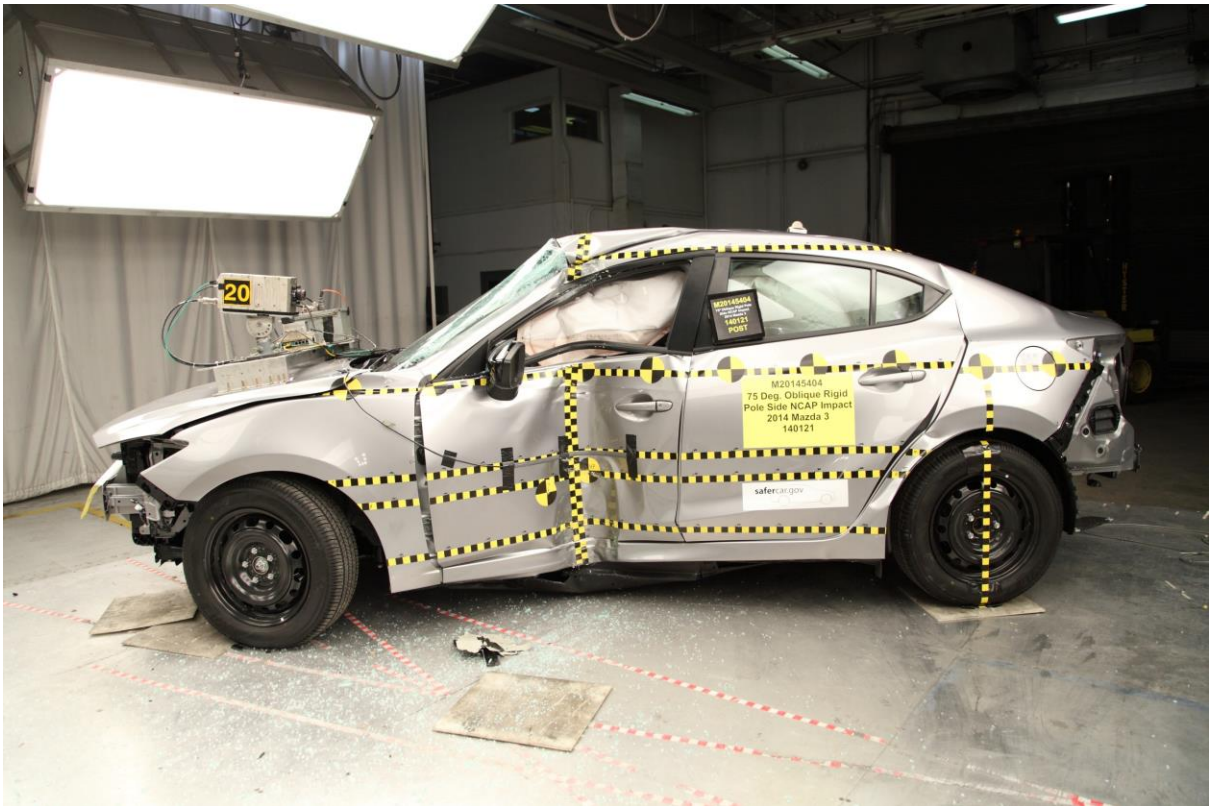
008 Post-Test Left Side View of Test Vehicle
