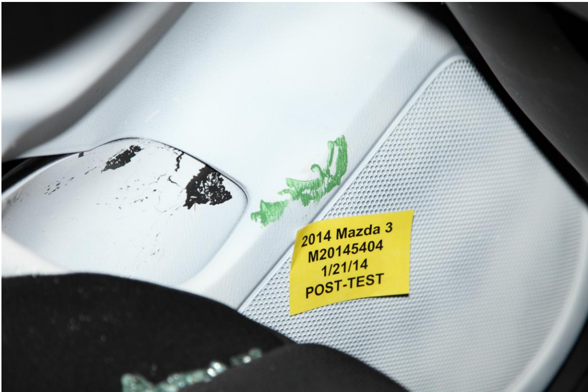
052 Post-Test Dummy Close-Up Knee Contact with Vehicle Interior View
