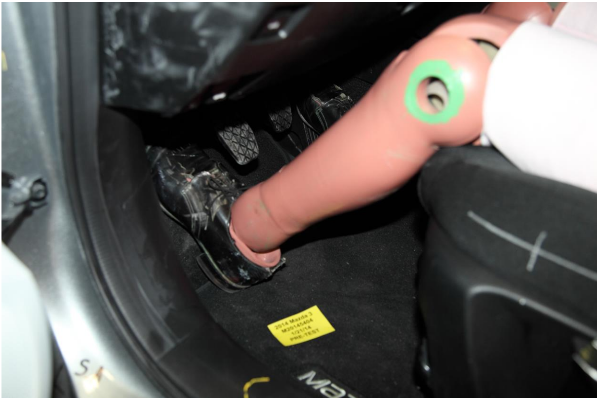
032 Pre-Test Placement of Dummy Feet
