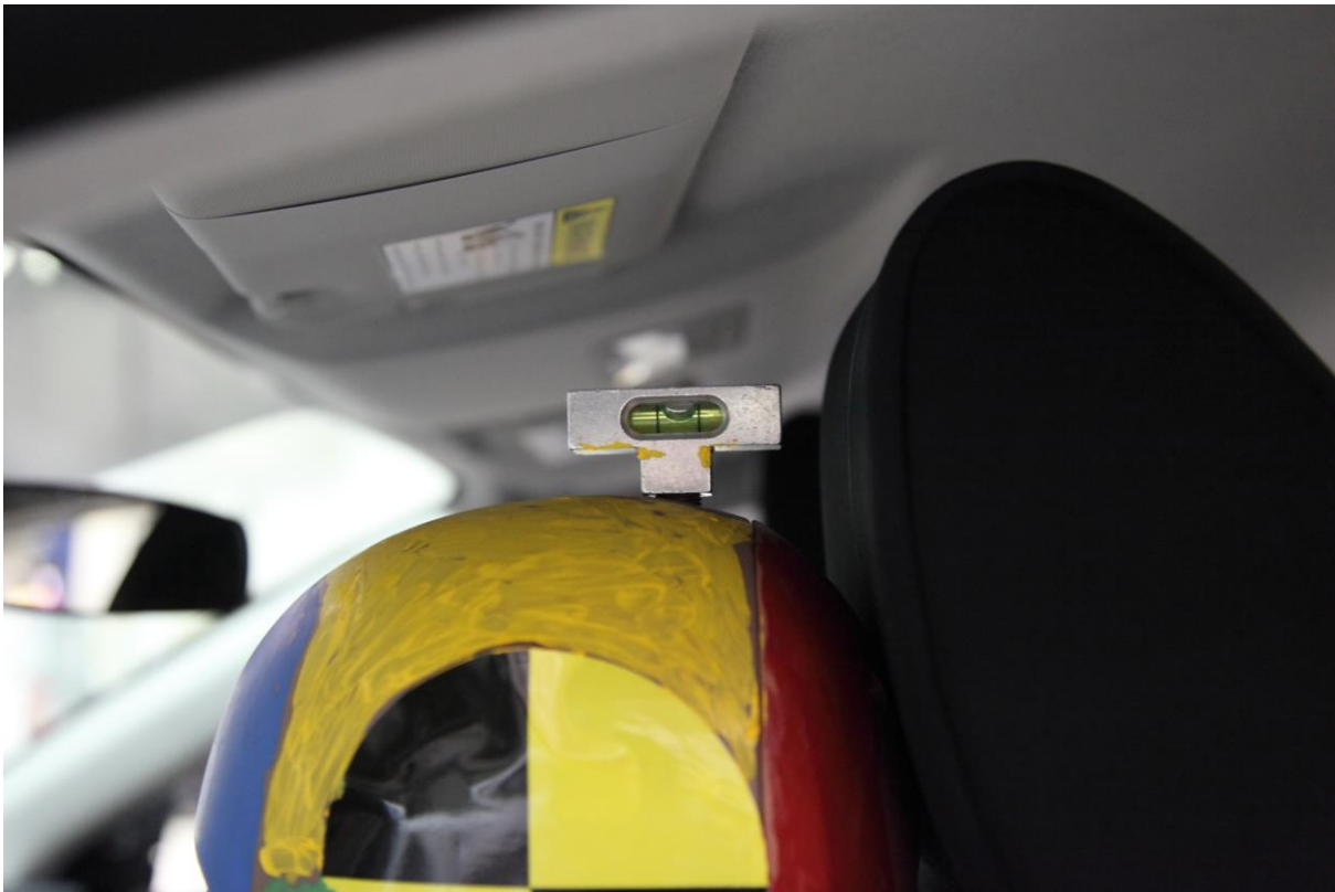
031 Pre-Test Left Side View of Dummy's Head Showing Dummy's Head is Level
