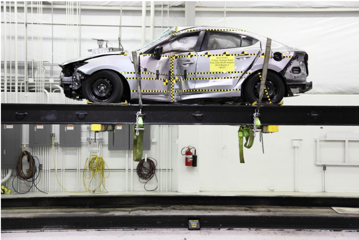
063 FMVSS No. 301 Static Rollover 0 Degrees
