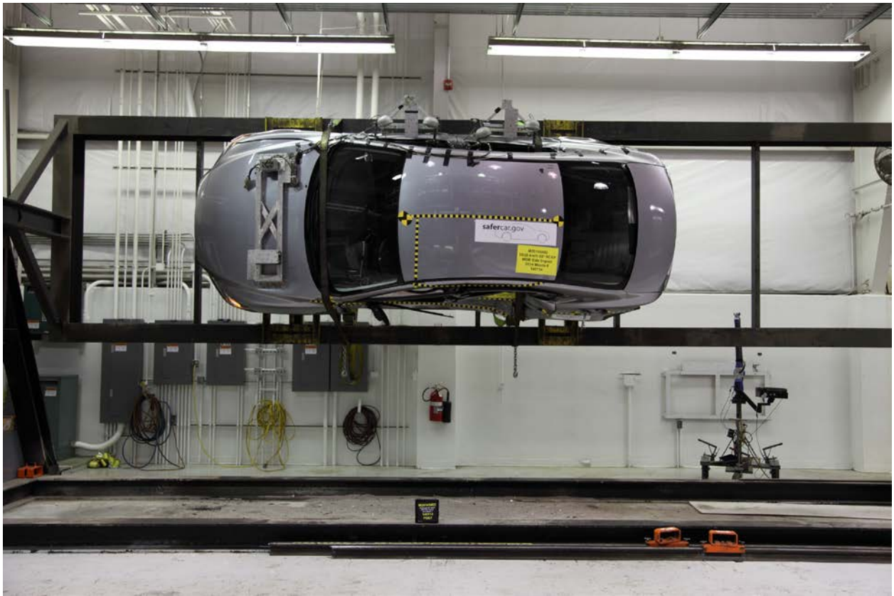
097 FMVSS No. 301 Static Rollover 90 Degrees
