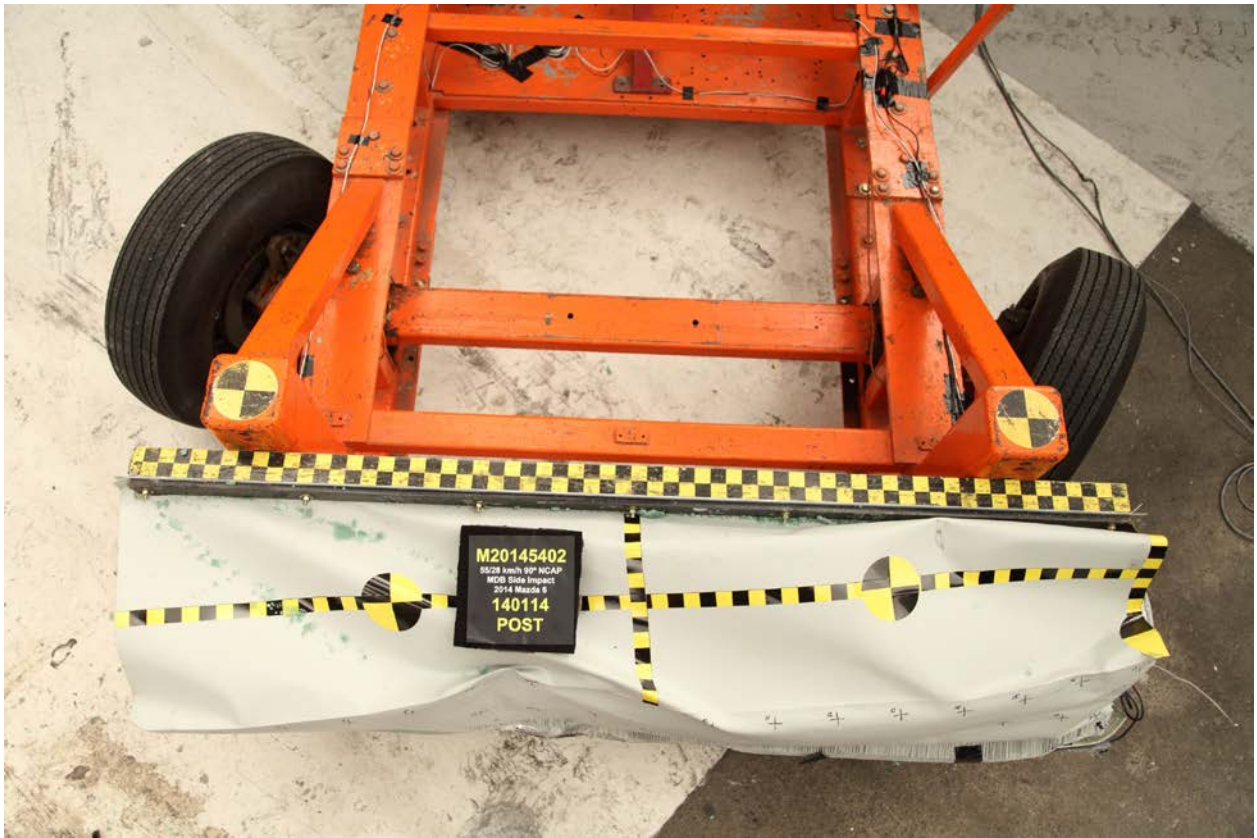
087 Post-Test Top View of MDB Impactor Face
