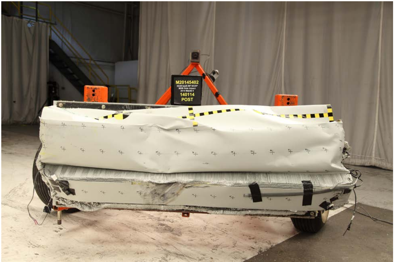
085 Post-Test Front View of MDB Impactor Face
