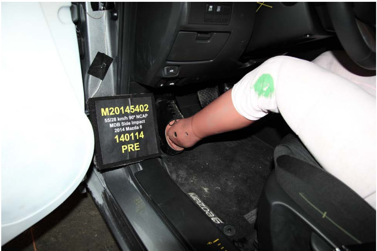
034 Pre-Test Placement of Driver Dummy Feet
