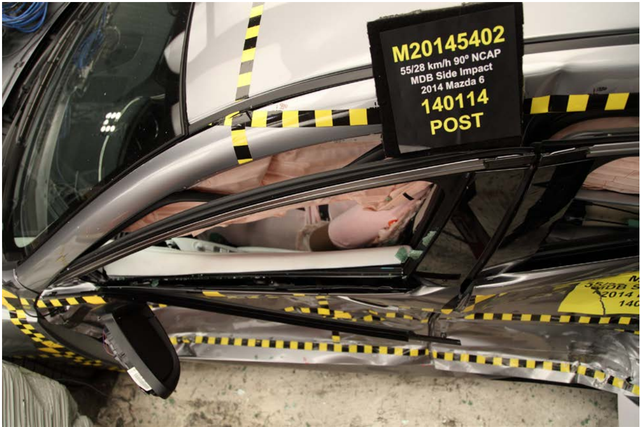
043 Post-Test Driver Dummy and Door Clearance View
