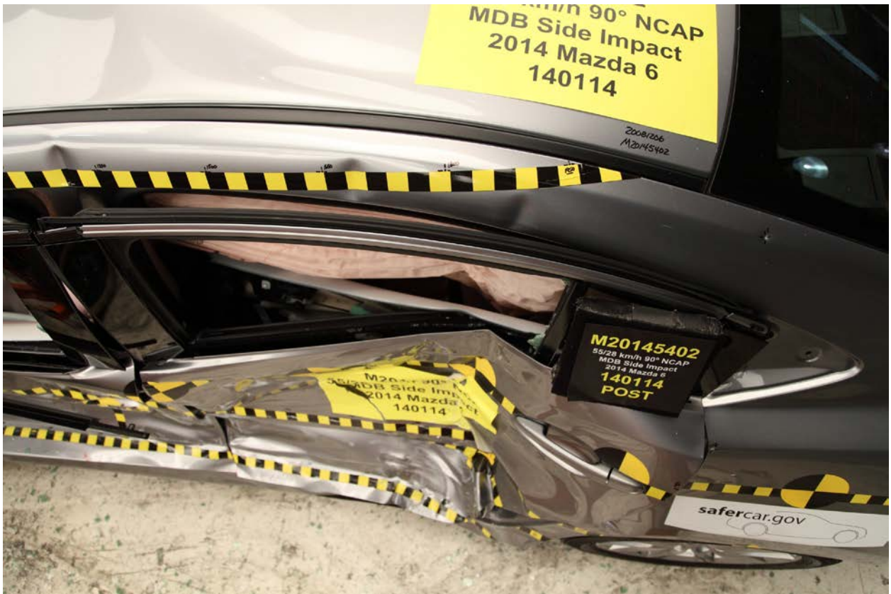
070 Post-Test Passenger Dummy and Door Clearance View
