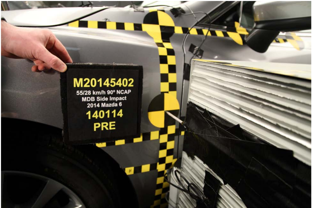
019 Pre-Test Close-up View of Impact Point Target
