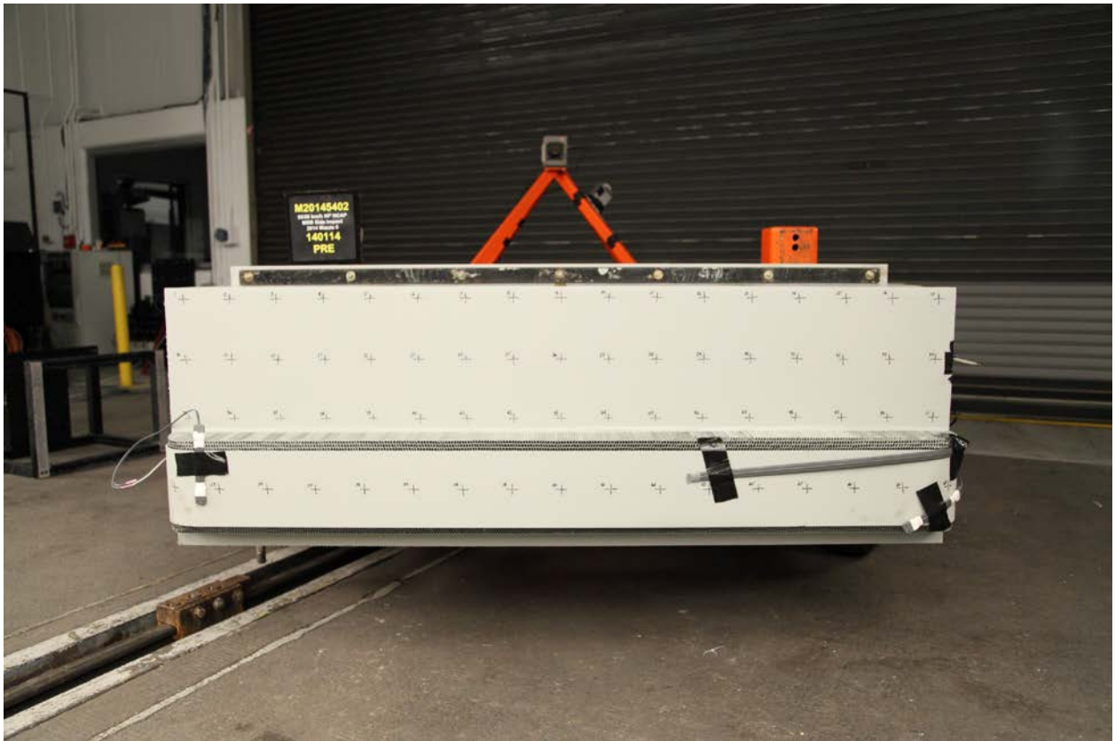
084 Pre-Test Front View of MDB Impactor Face
