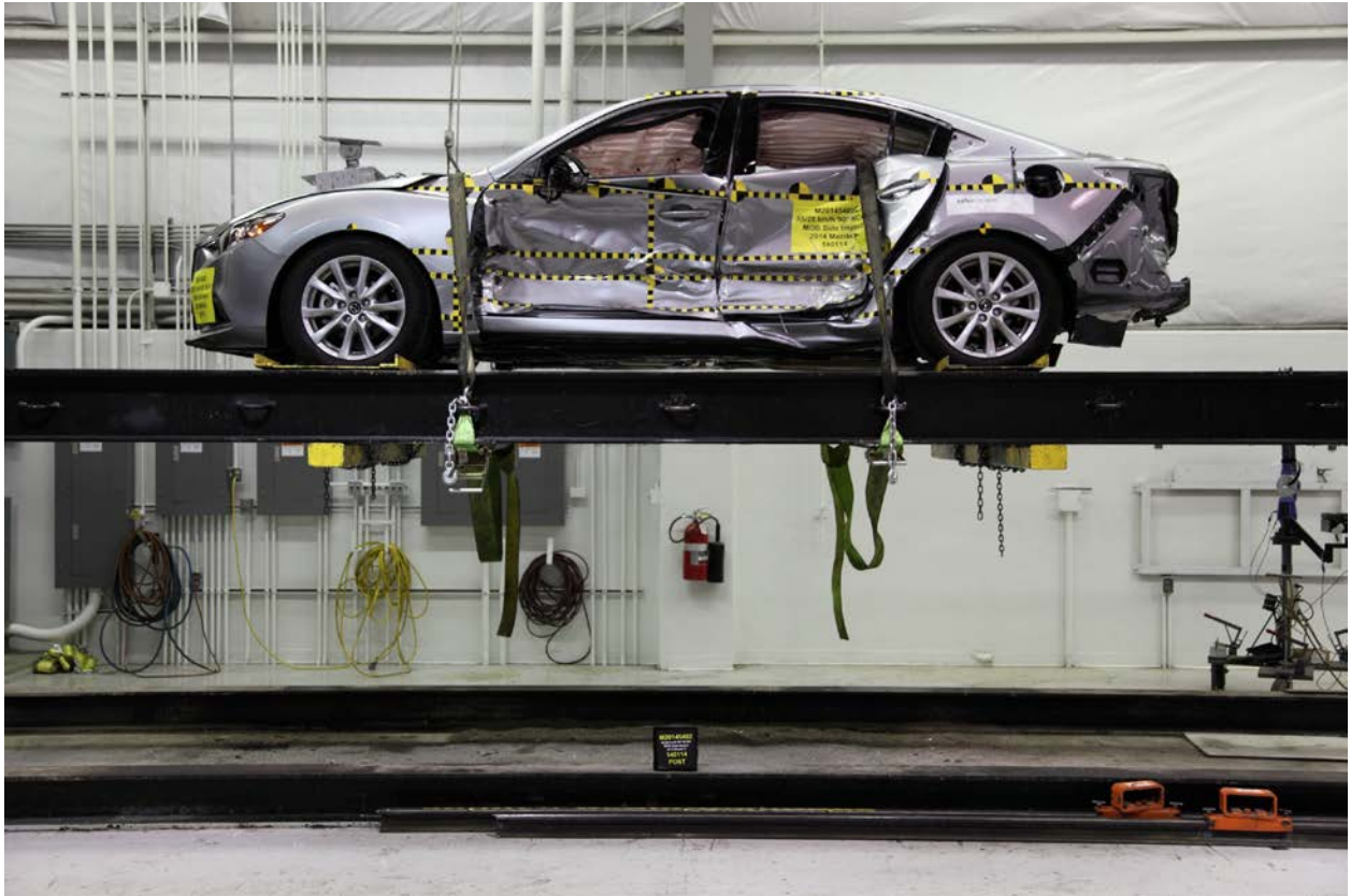
096 FMVSS No. 301 Static Rollover 0 Degrees
