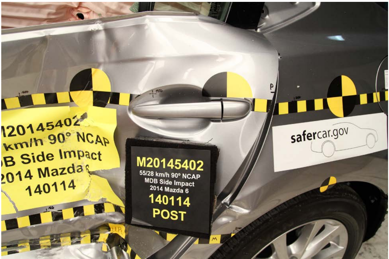
024 Post-Test Left Rear Door Latch Close-up
