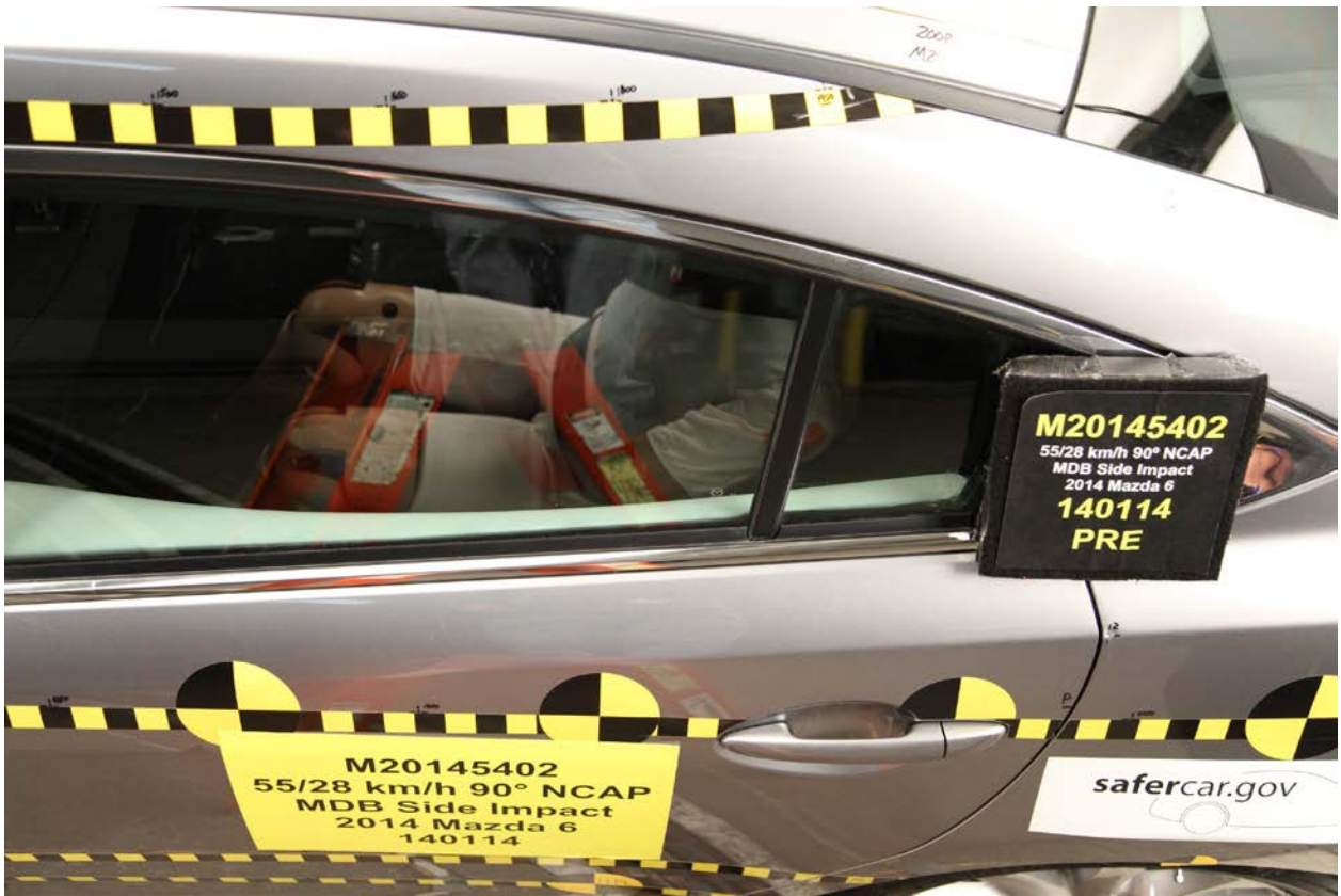
069 Pre-Test Passenger Dummy and Door Clearance View
