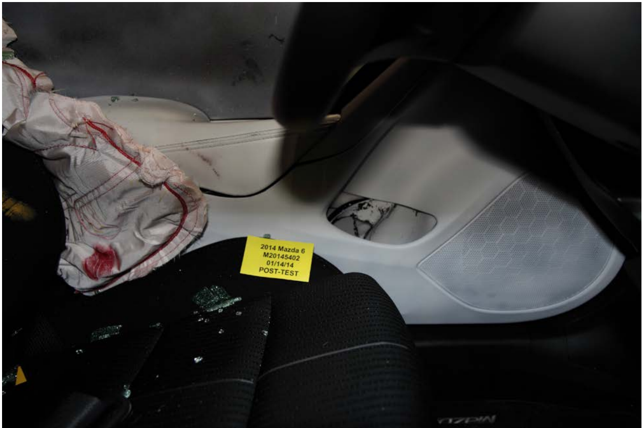
054 Post-Test Driver Dummy Close-Up Knee Contact View
