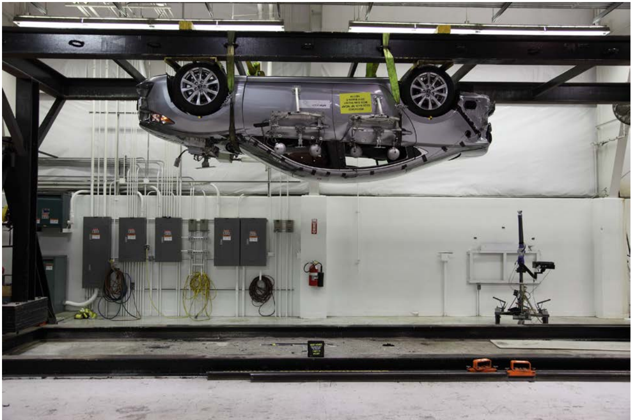
098 FMVSS No. 301 Static Rollover 180 Degrees
