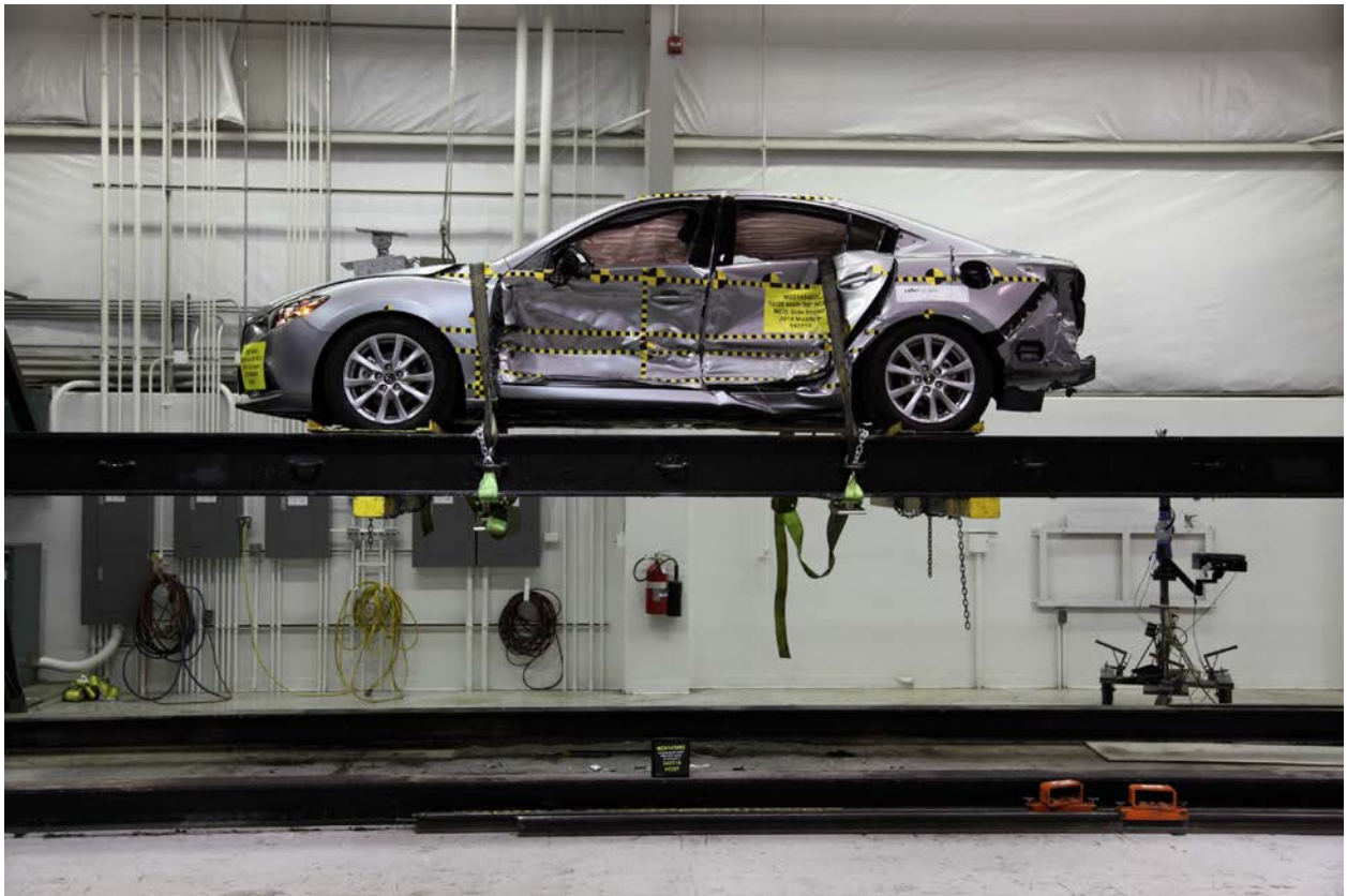
100 FMVSS No. 301 Static Rollover 360 Degrees
