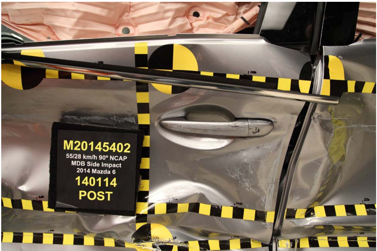
022 Post-Test Left Front Door Latch Close-up
