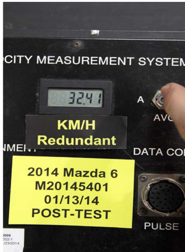
062 Post-Test Primary and Redundant Speed Trap Read-Out
