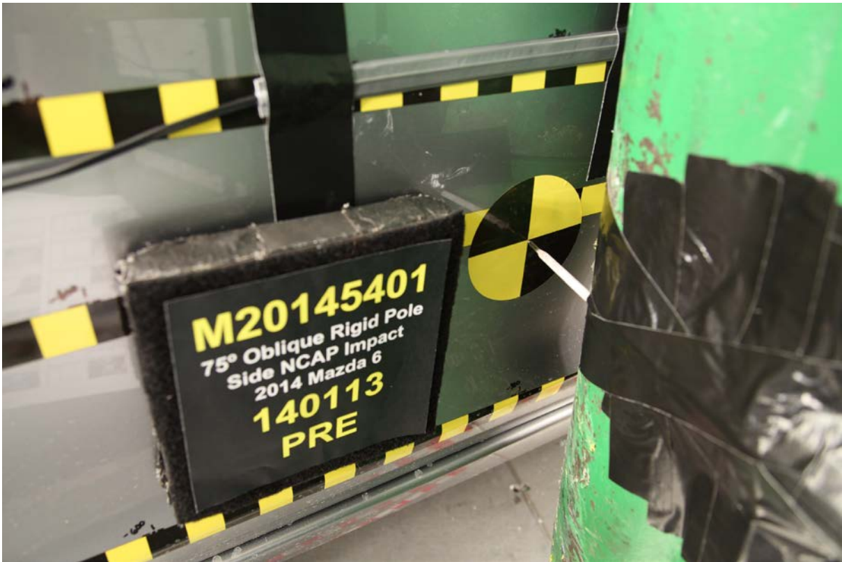
019 Pre-Test Close-Up View of Impact Point Target
