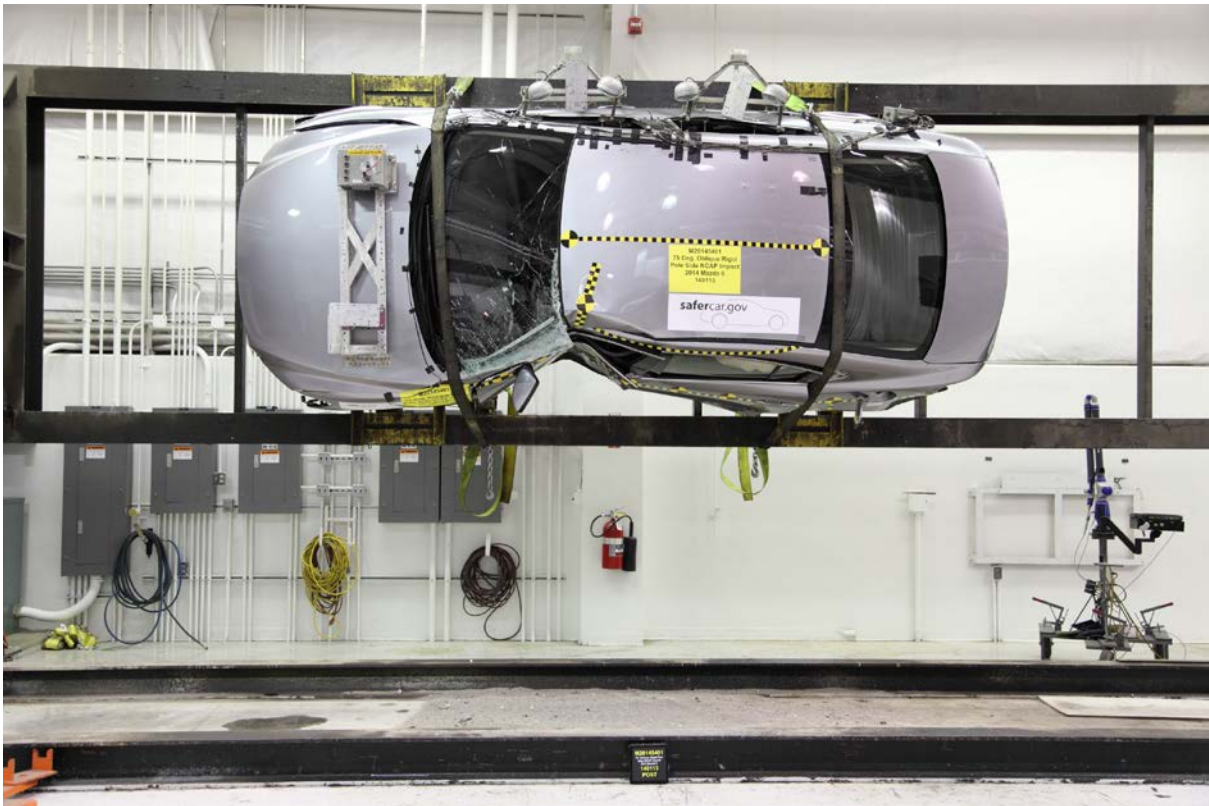
064 FMVSS No. 301 Static Rollover 90 Degrees
