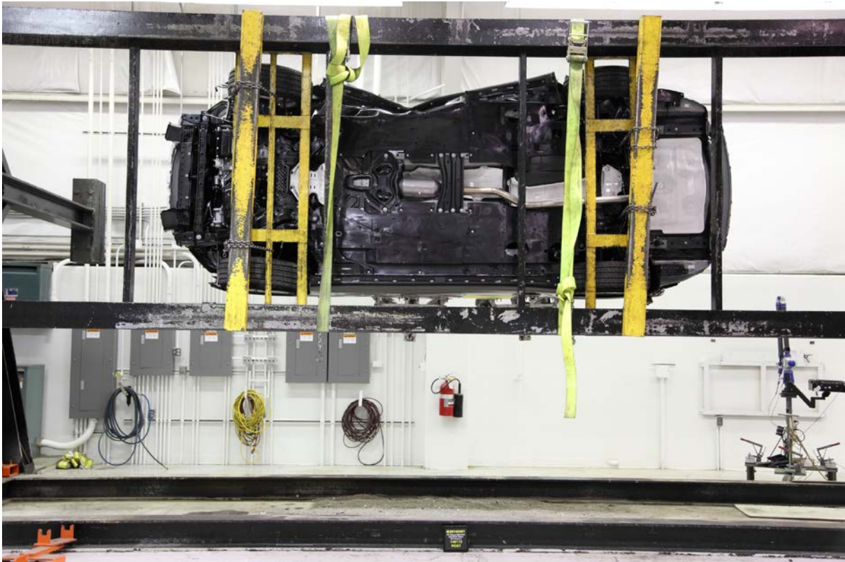
066 FMVSS No. 301 Static Rollover 270 Degrees
