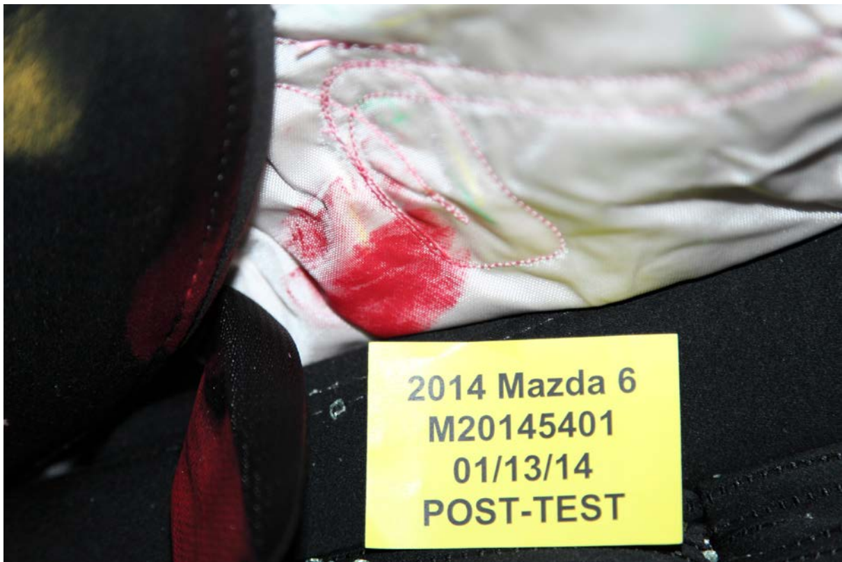
051 Post-Test Dummy Close-Up Pelvis Contact with Side Airbag View
