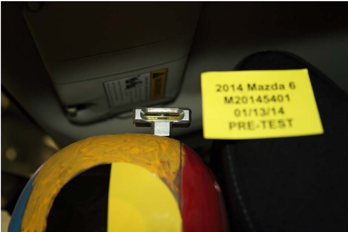
031 Pre-Test Left Side View of Dummy Head Showing Dummy Head is Level
