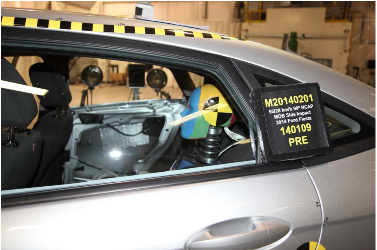
056 Pre-Test Left Side View of Passenger Dummy Shoulder and Door Top View
