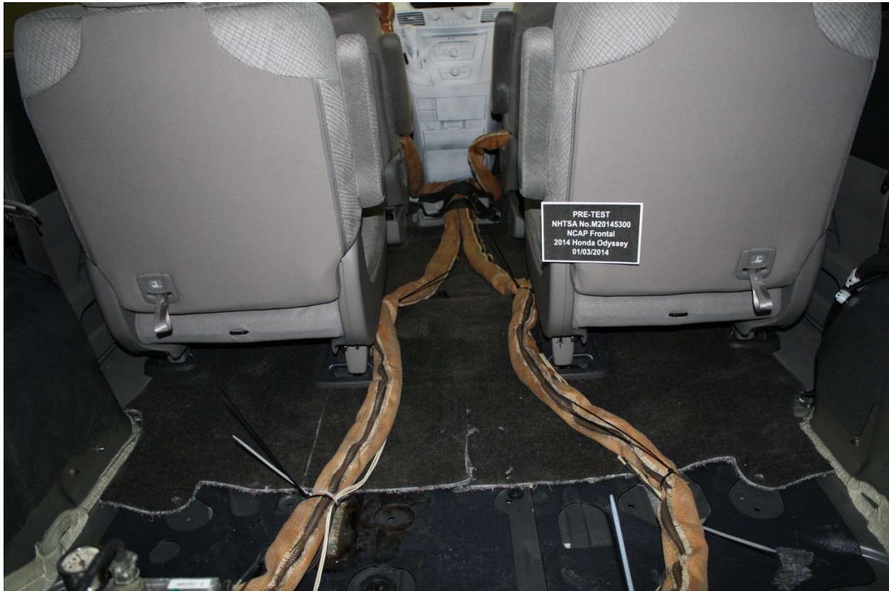
Figure A-27: Pre-Test Dummy Cable Routing
