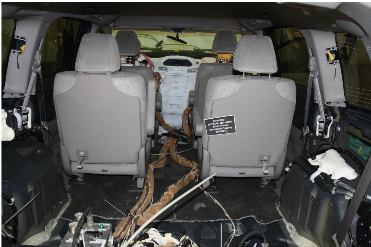
Figure A-28: Post-Test Dummy Cable Routing
