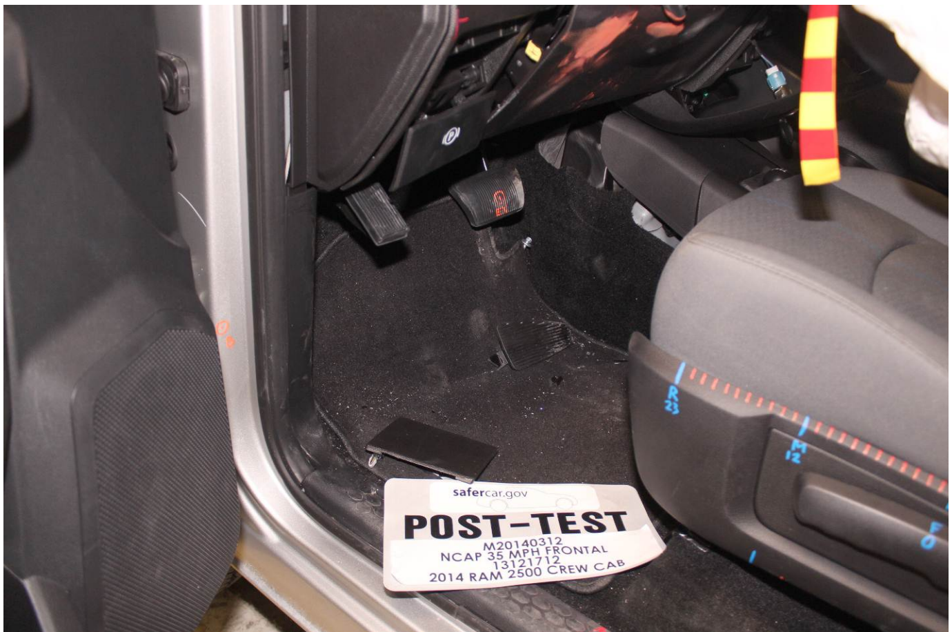
Post-Test Driver's Side Floorpan
