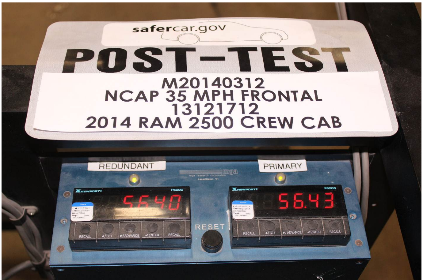
Post-Test Speed Trap Read-Out
