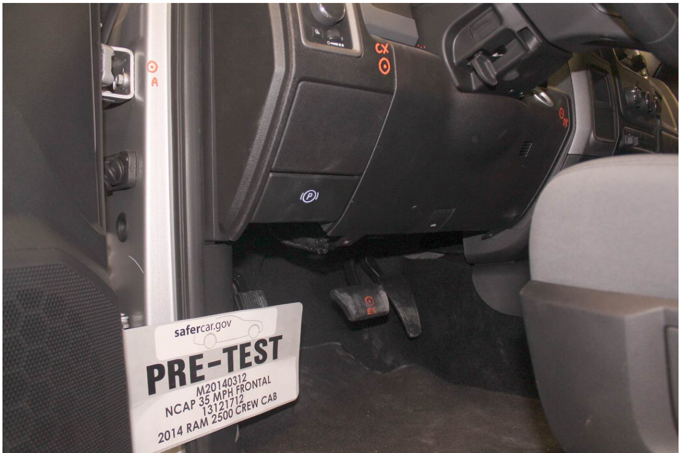
Pre-Test Driver's Side Knee Bolster (without dummy)
