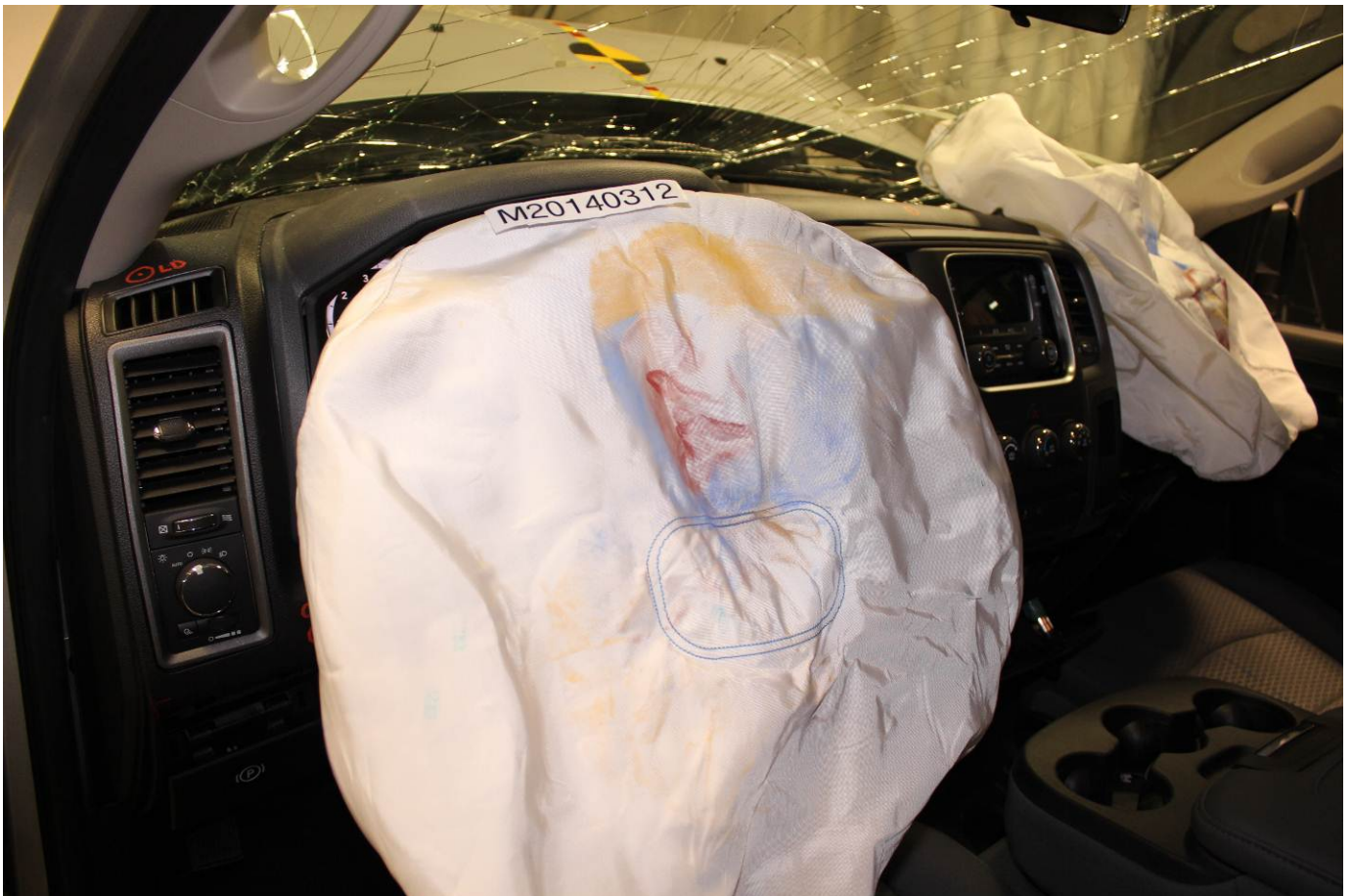
Post-Test Driver Dummy Contact with Airbag
