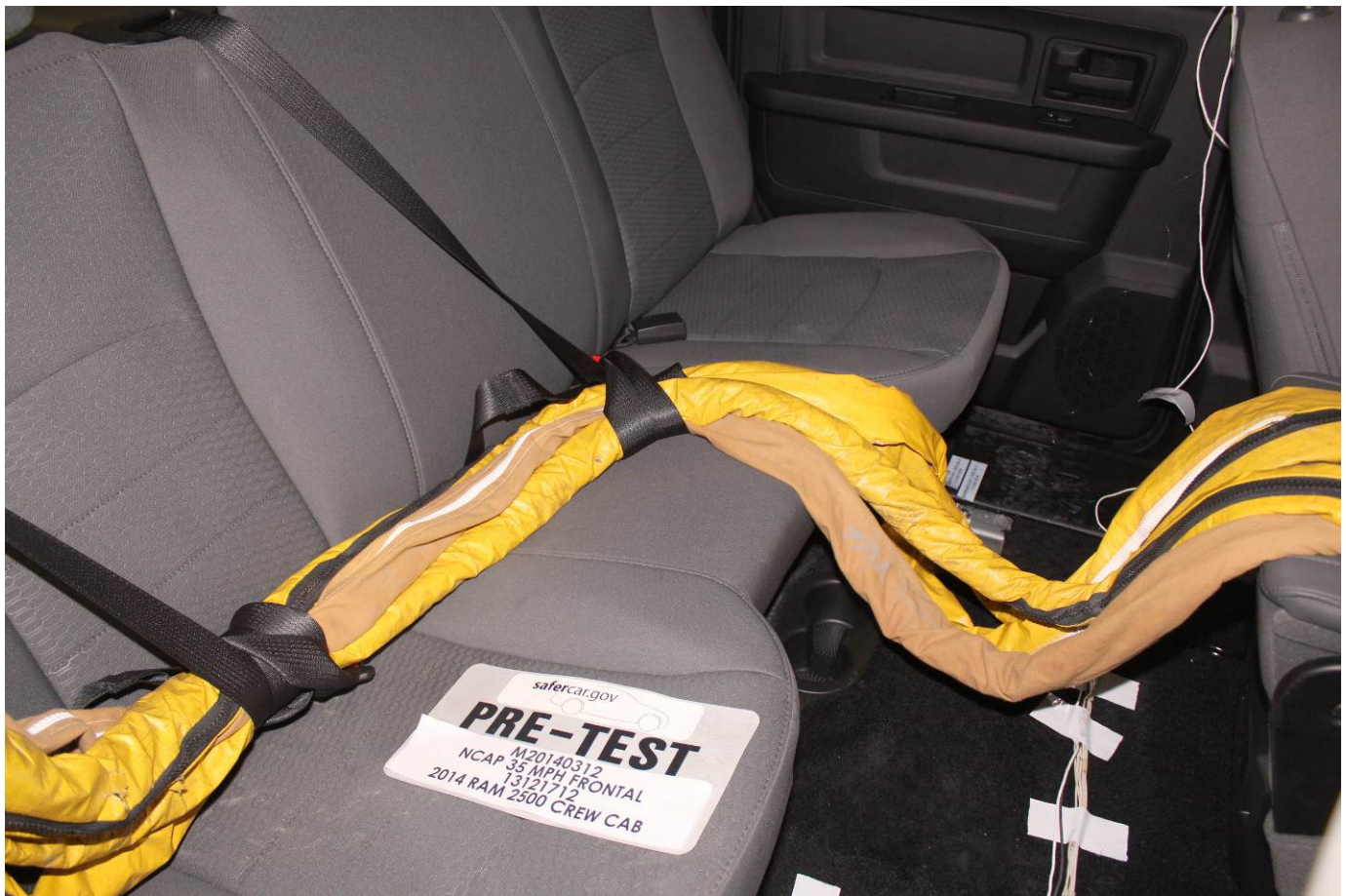
Pre-Test Dummy Cable Routing
