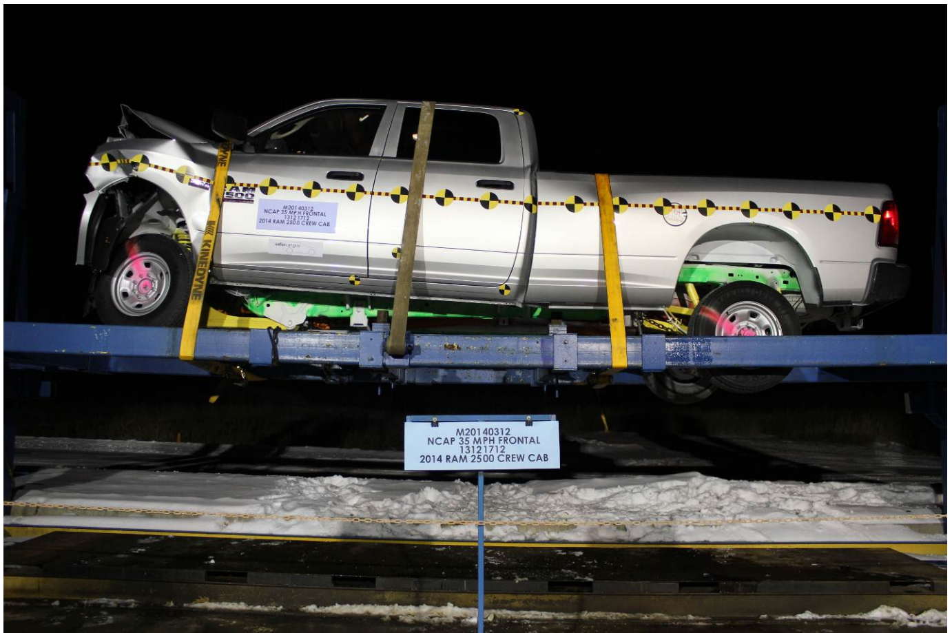
Vehicle at 0 Degree on Static Rollover Device
