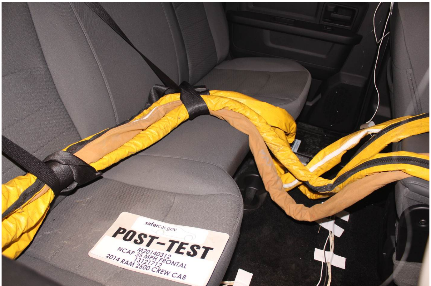
Post-Test Dummy Cable Routing
