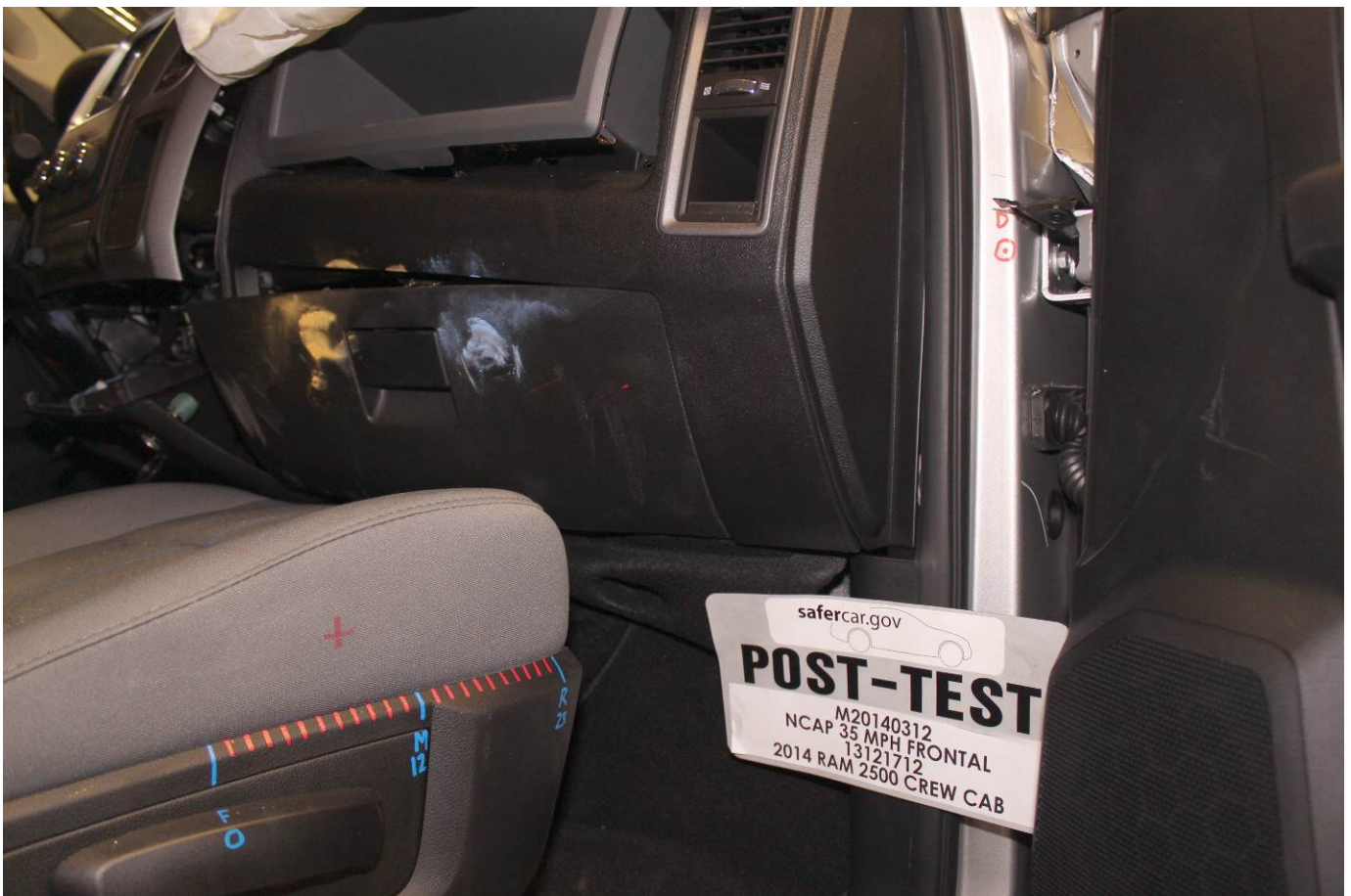
Post-Test Passenger's Side Knee Bolster (without dummy)
