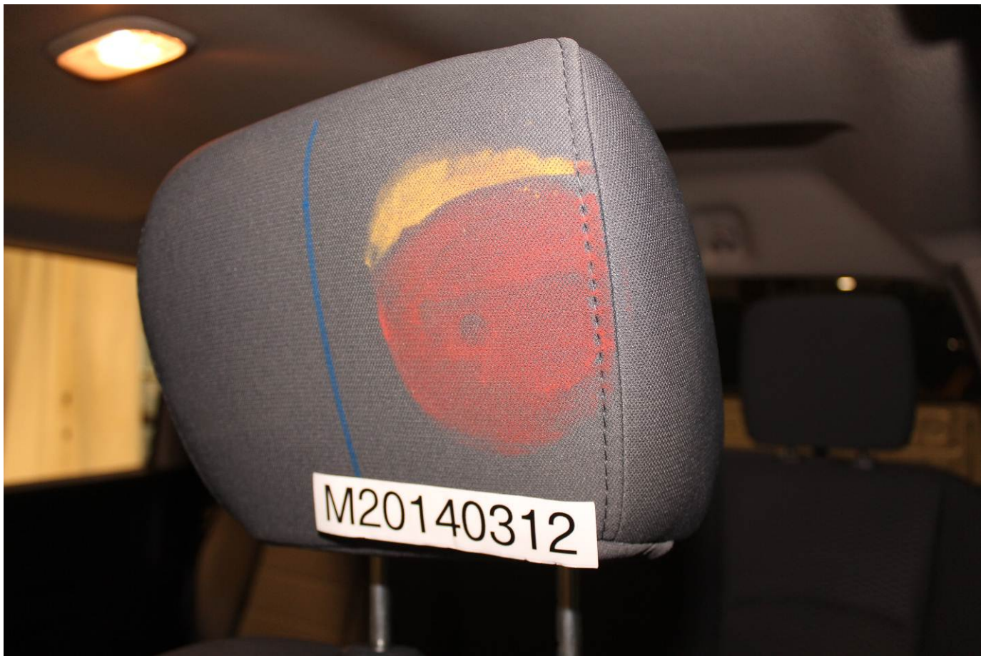
Post-Test Driver Dummy Contact with Headrest
