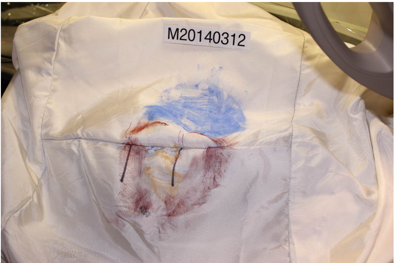
Post-Test Passenger Dummy Contact with Airbag
