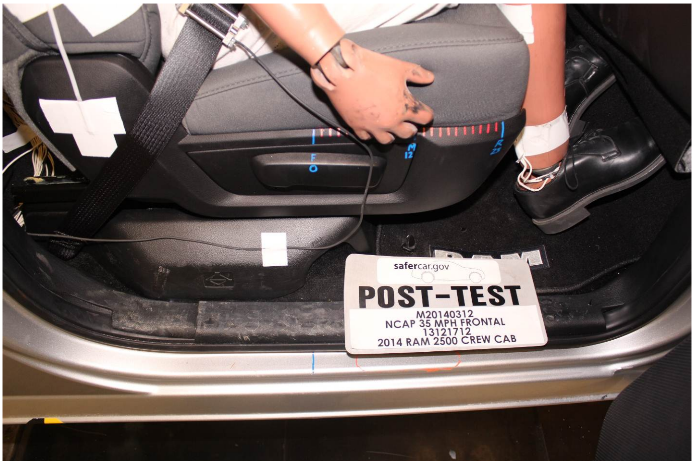
Post-Test Passenger's Seat Fore-Aft Markings
