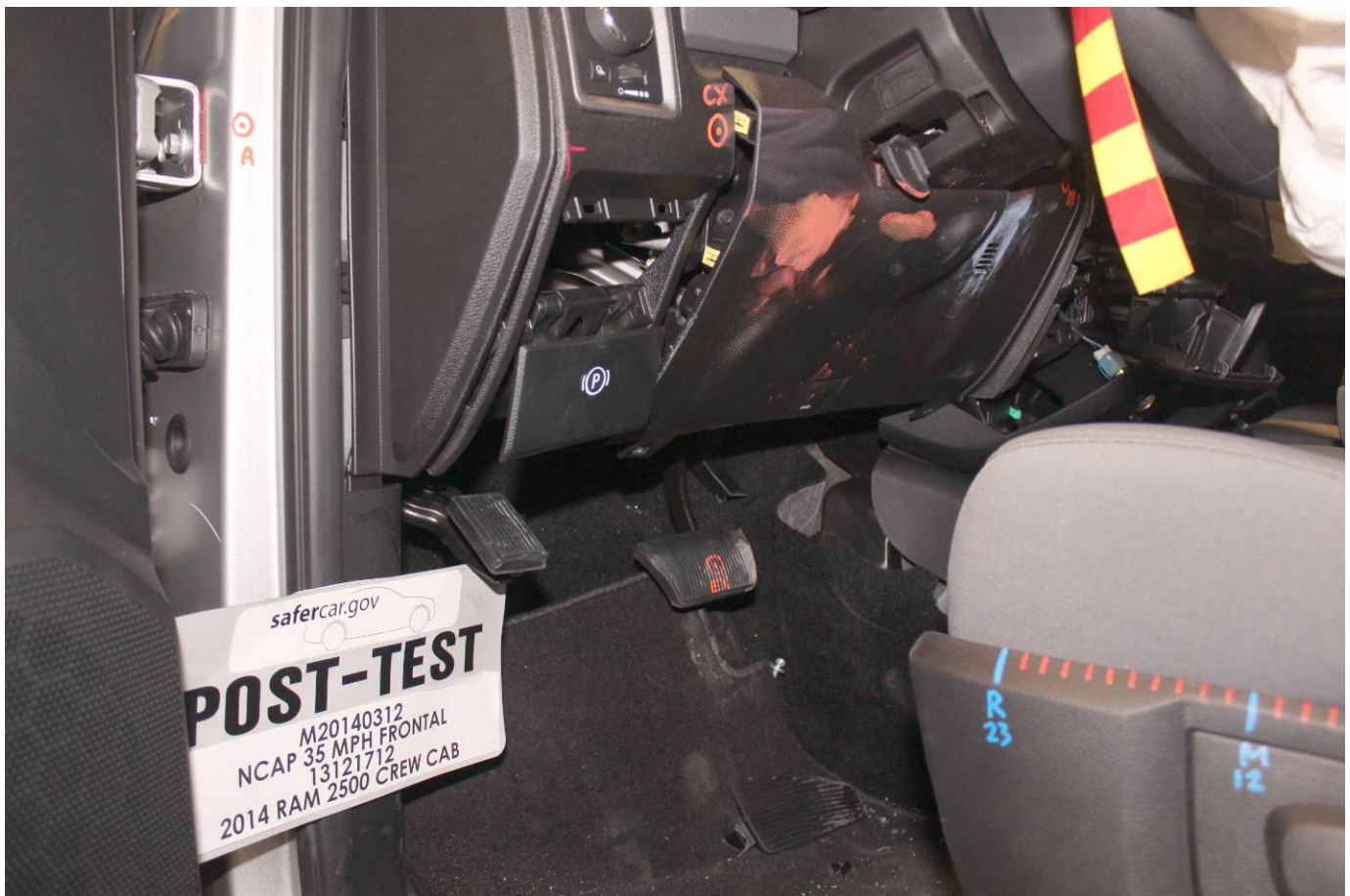
Post-Test Driver's Side Knee Bolster (without dummy)
