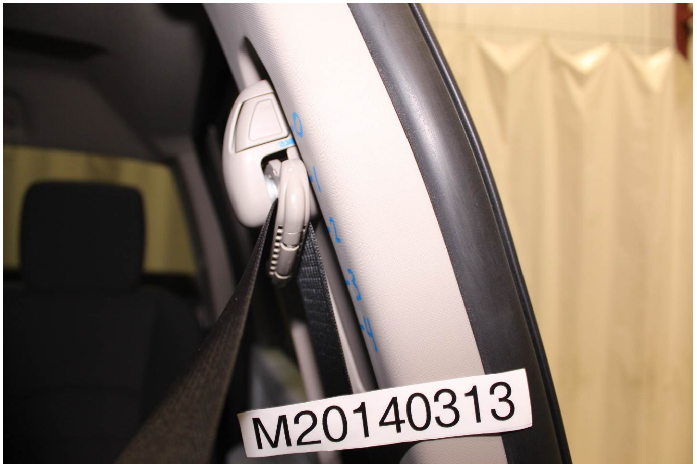
Pre-Test View of Belt Anchorage for Dummy
