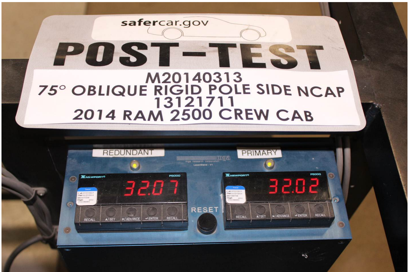
Post-Test Primary and Redundant Speed Trap Read-Out
