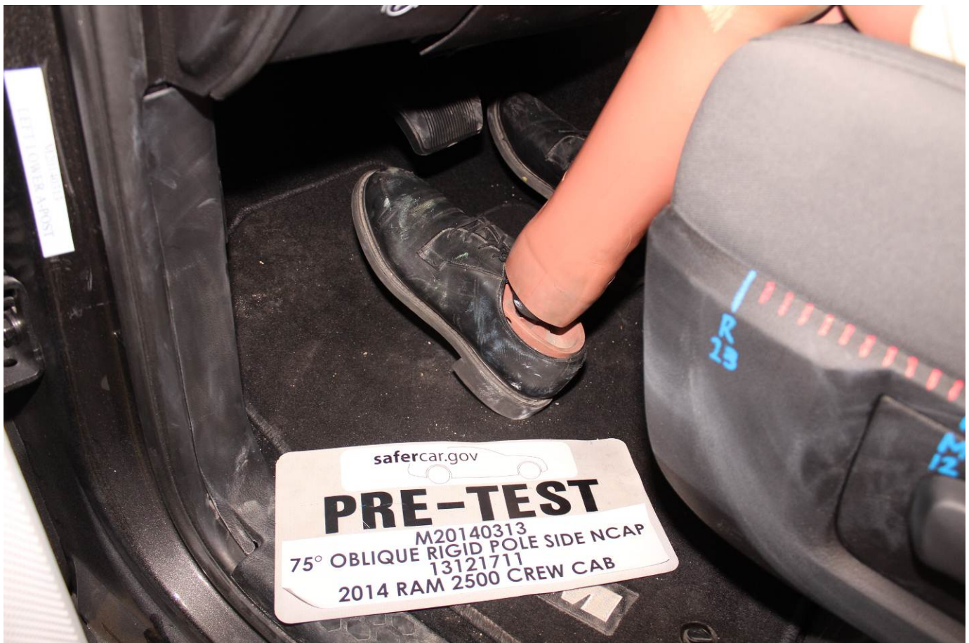
Pre-Test Placement of Dummy's Feet
