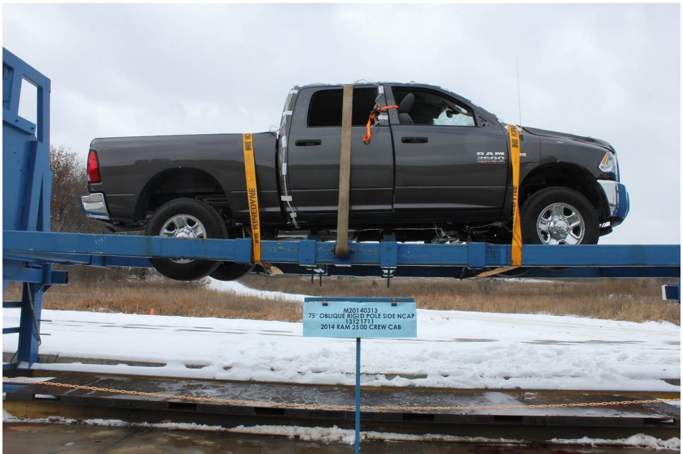
FMVSS No. 301 Static Rollover 360 Degrees
