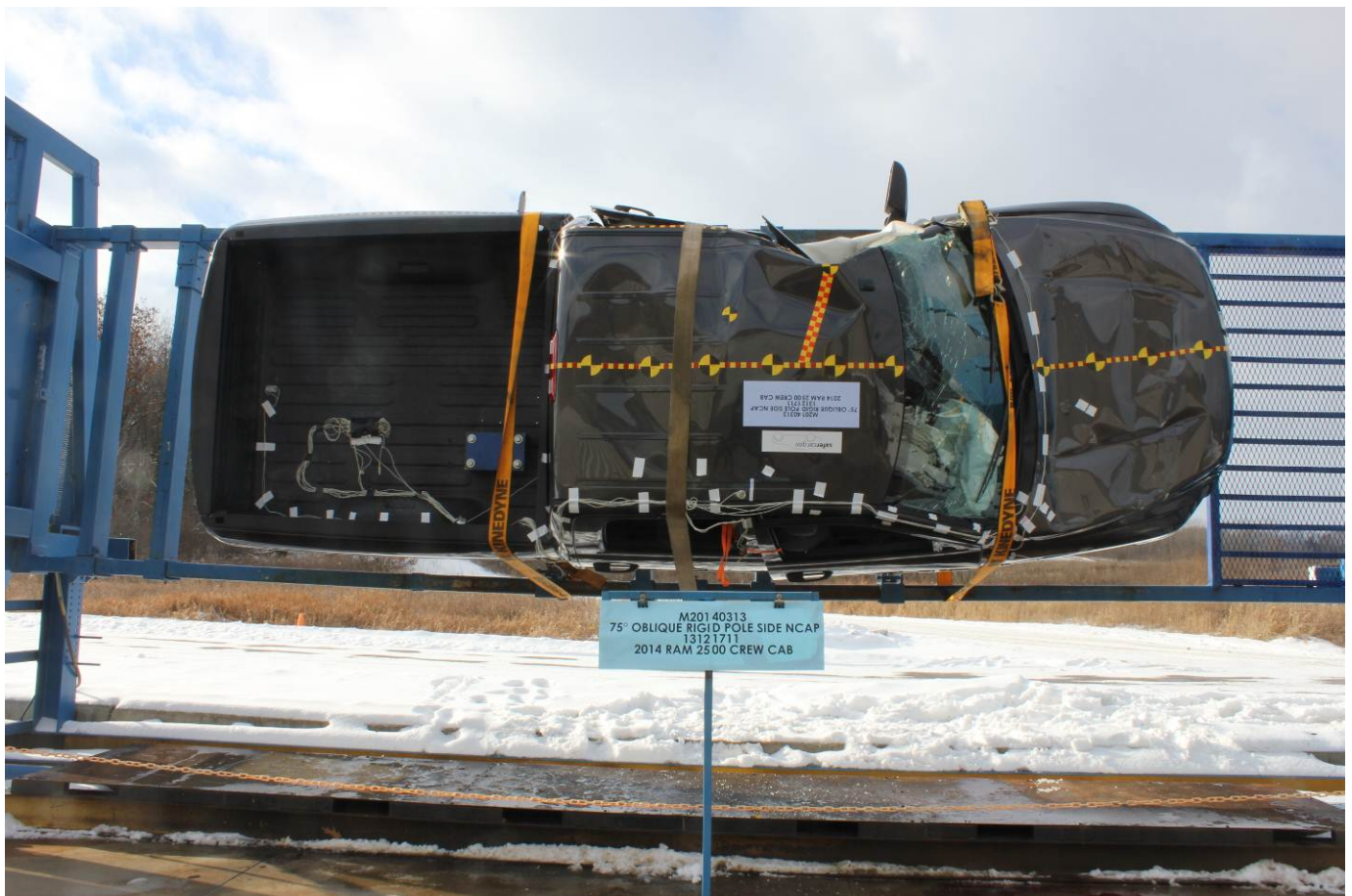
FMVSS No. 301 Static Rollover 270 Degrees
