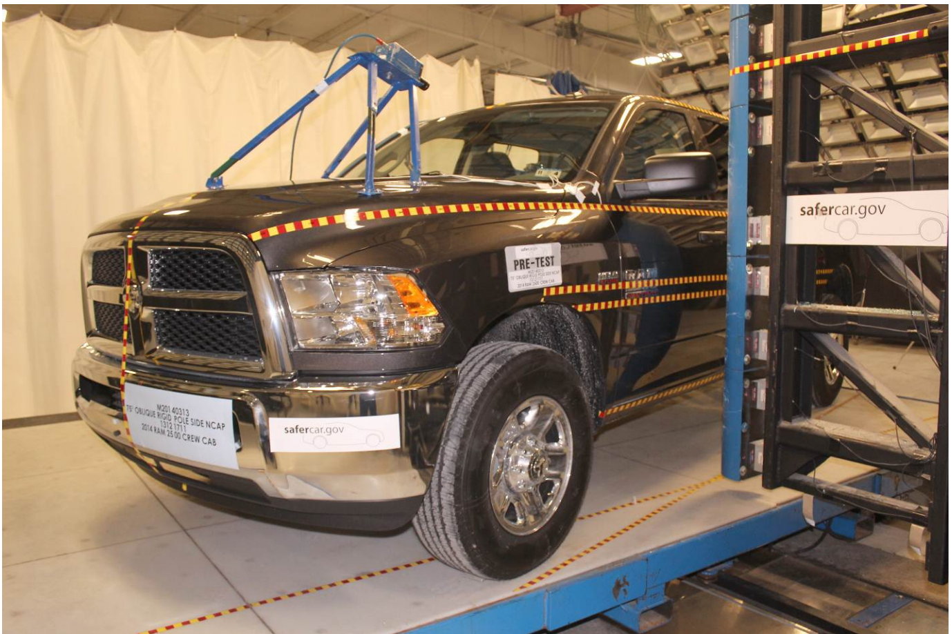
Pre-Test Left Side View of Pole Positioned Against Side of Vehicle
