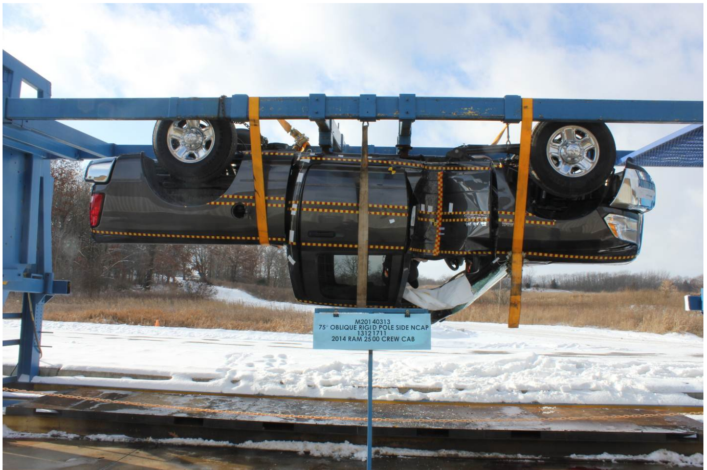
FMVSS No. 301 Static Rollover 180 Degrees
