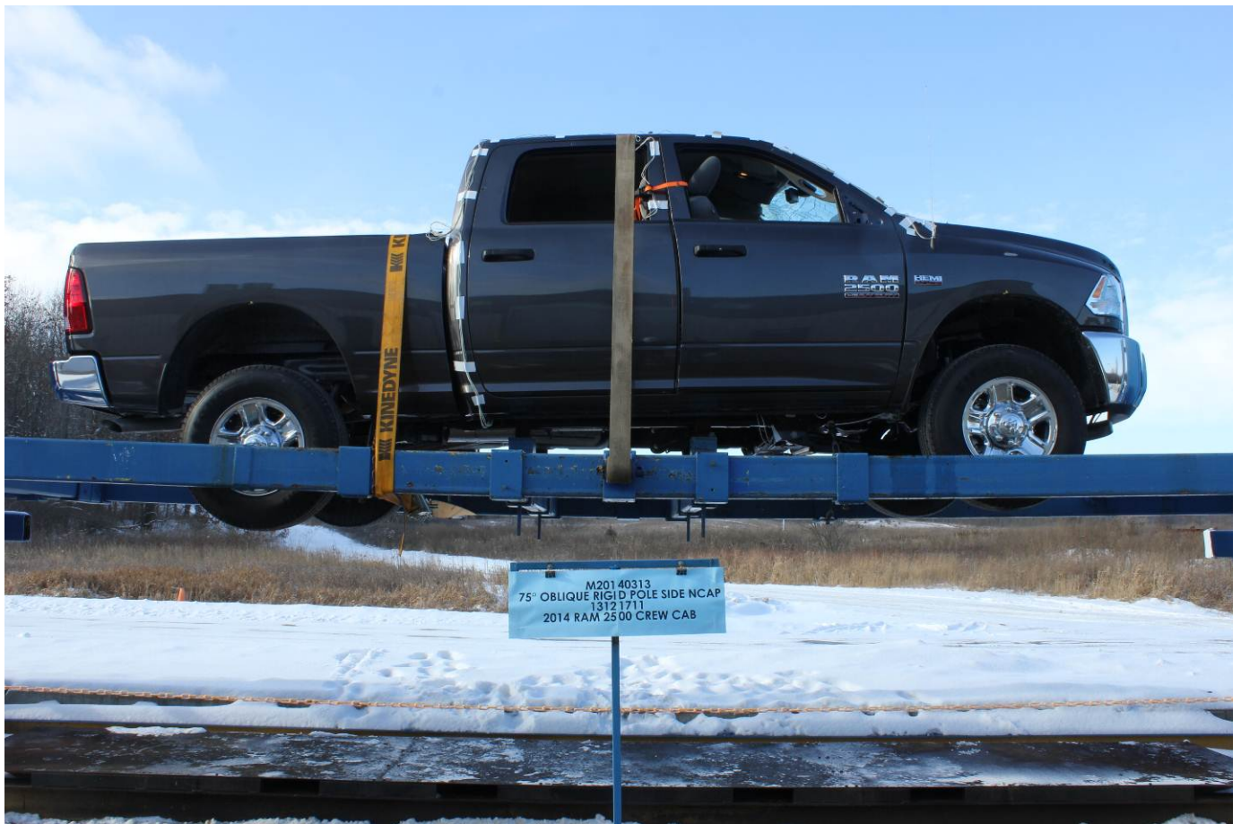
FMVSS No. 301 Static Rollover 0 Degrees
