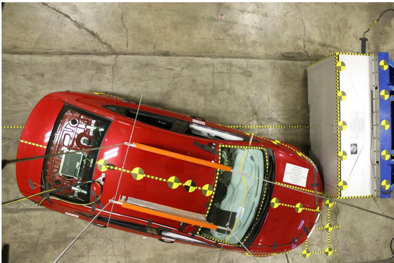
No. 022 Pre-Test Overhead View of RMDB against target vehicle at ideal Impact Point
