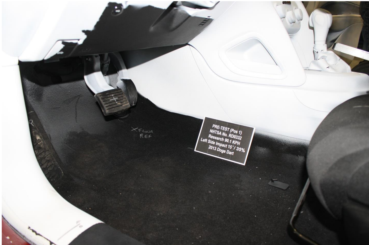
No. 044 Pre-Test View of Driver Floor pan at Left sill level, w/carpet
