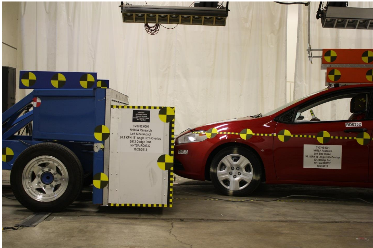
No. 024 Pre-Test Right Side View of RMDB against target vehicle at ideal Impact Point
