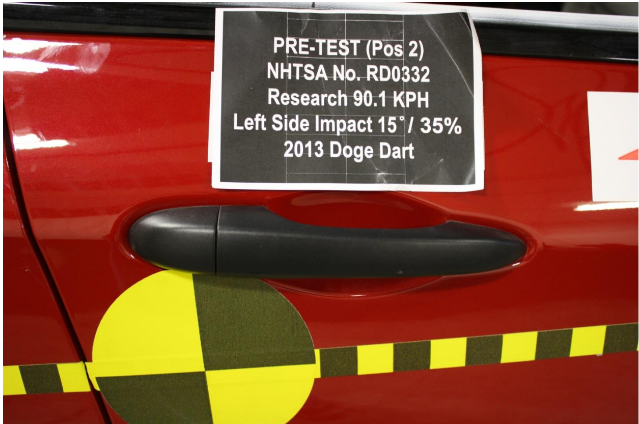
No. 030 Pre-Test Close-up View of Passenger Door Latch
