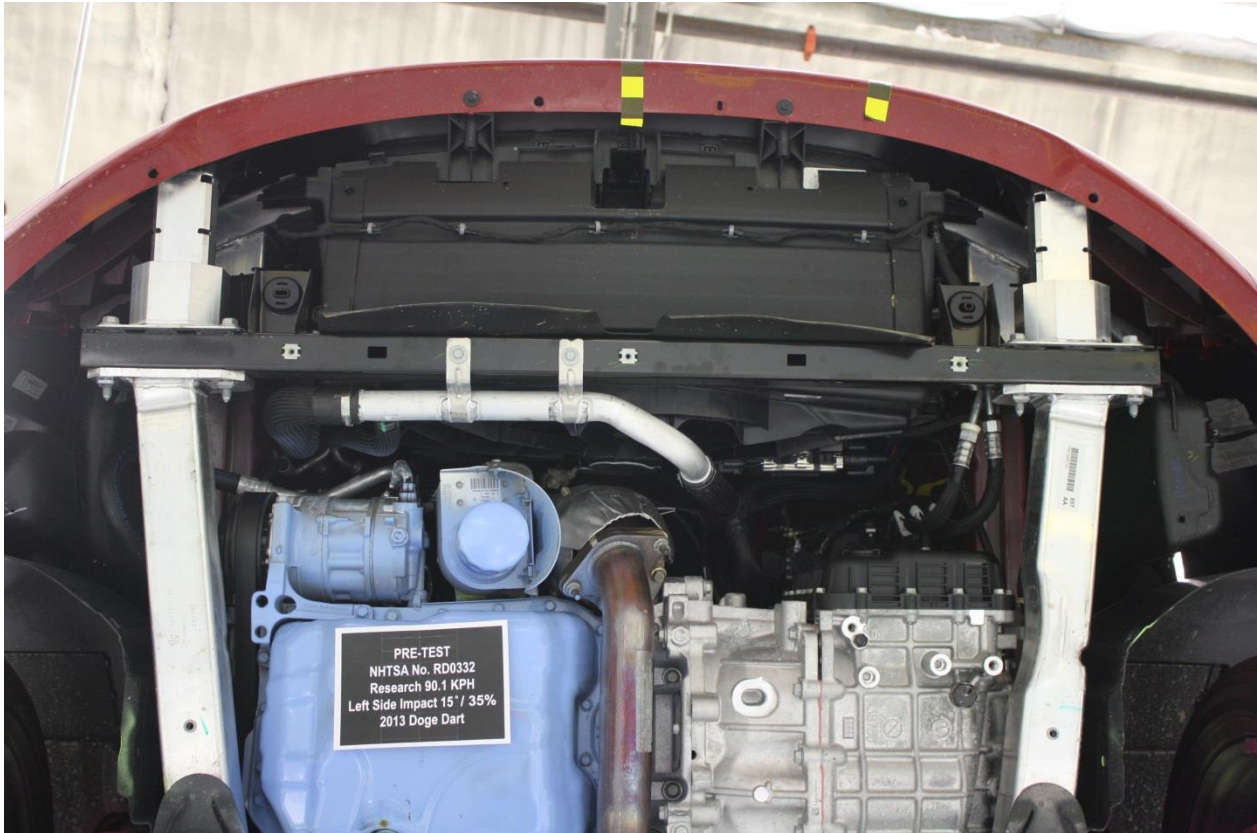
No. 137 Pre-Test Bumper to Rail Attachments and Crush Initiators
