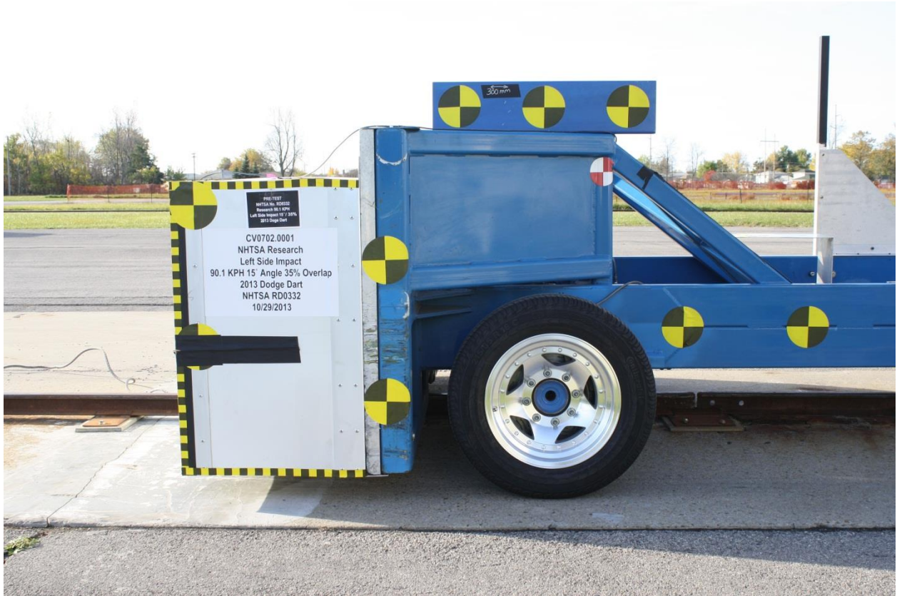
No. 162 Pre-Test Left Side View of RMDB
