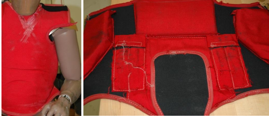
Jacket has tears around neck and at most seam ends as seen here on the front left shoulder.
