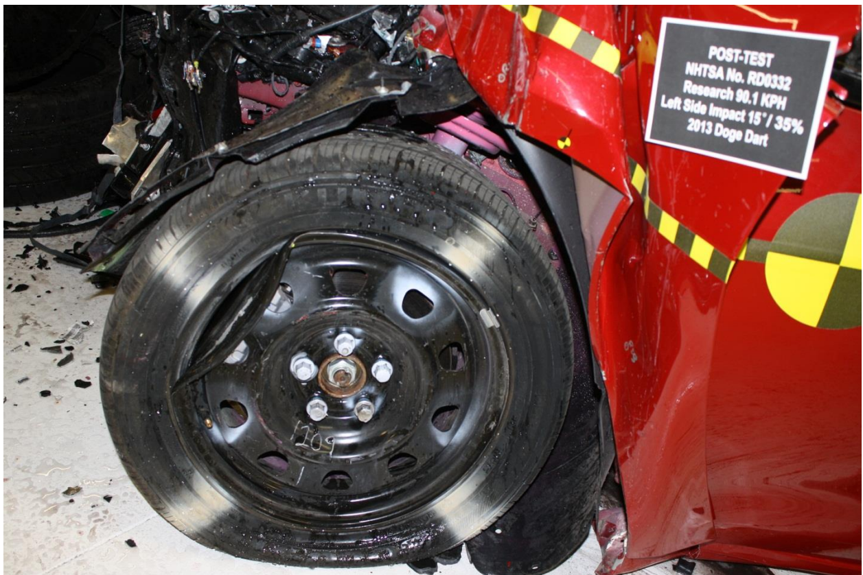
No. 159 Post-Test View of Wheel and/or Tire Deformation-Struck Side
