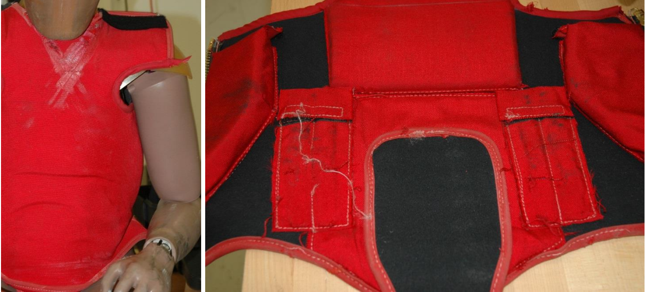
Jacket has tears around neck and at most seam ends as seen here on the front left shoulder.
