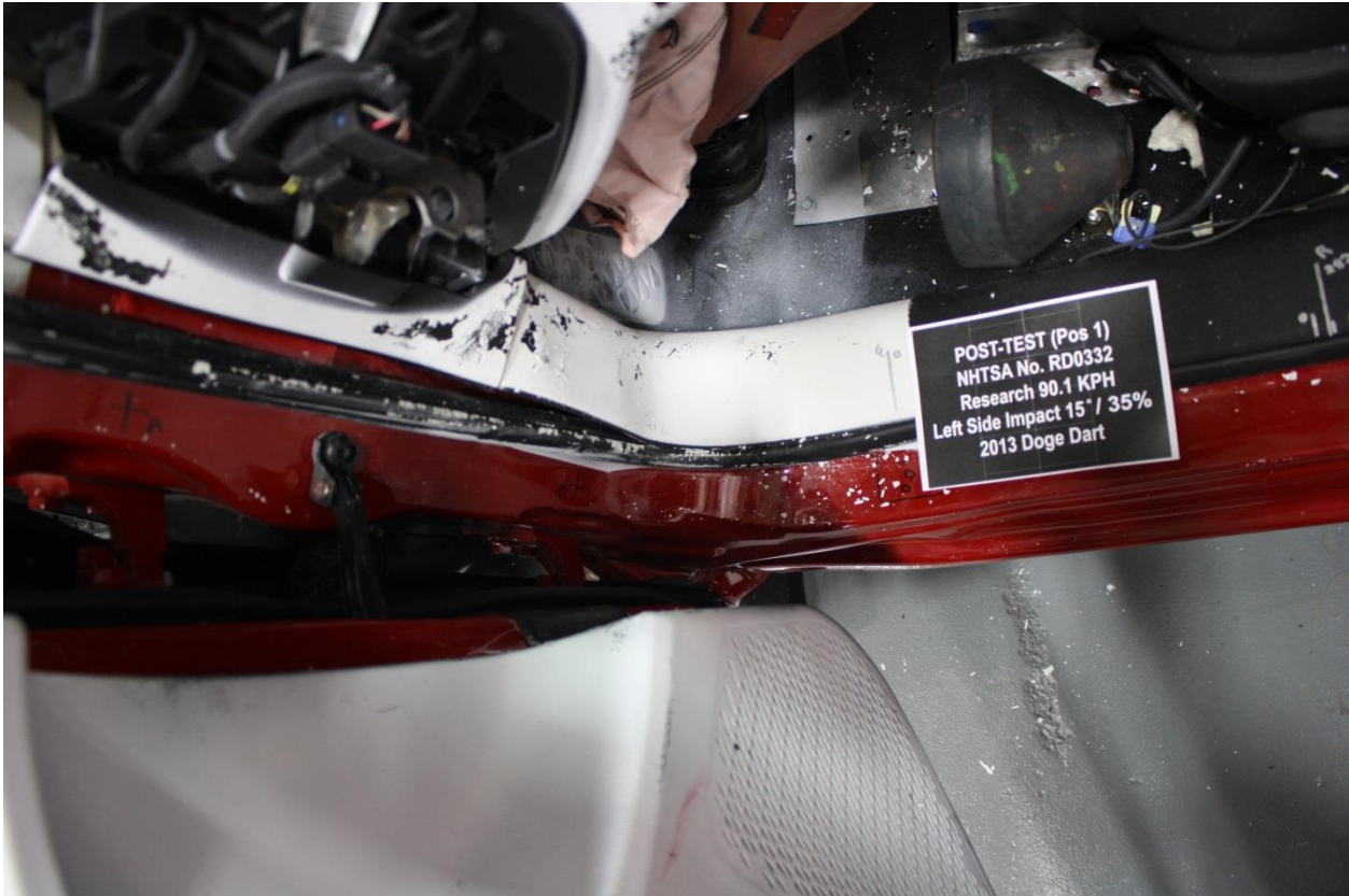
No. 160 Post-Test View of Deformation of Rocker or Post-Struck Side
