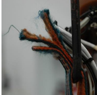
Lifting strap torn
