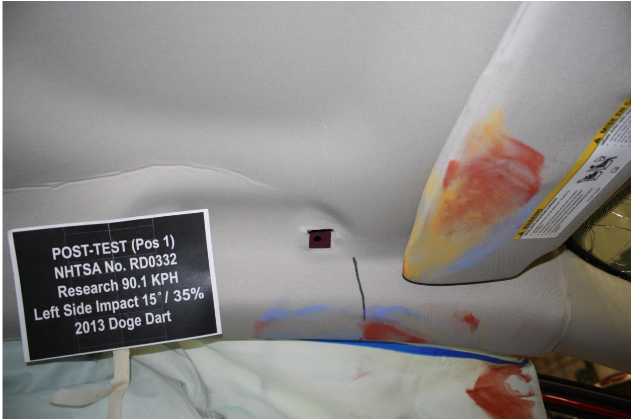
No. 081 Post-Test View of Driver Head Contact with Vehicle Interior – A
