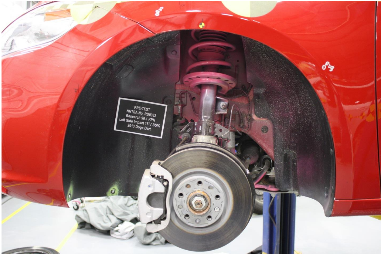
No. 142 Pre-Test View of Front Driver Wheel Well w/ Tire Removed
