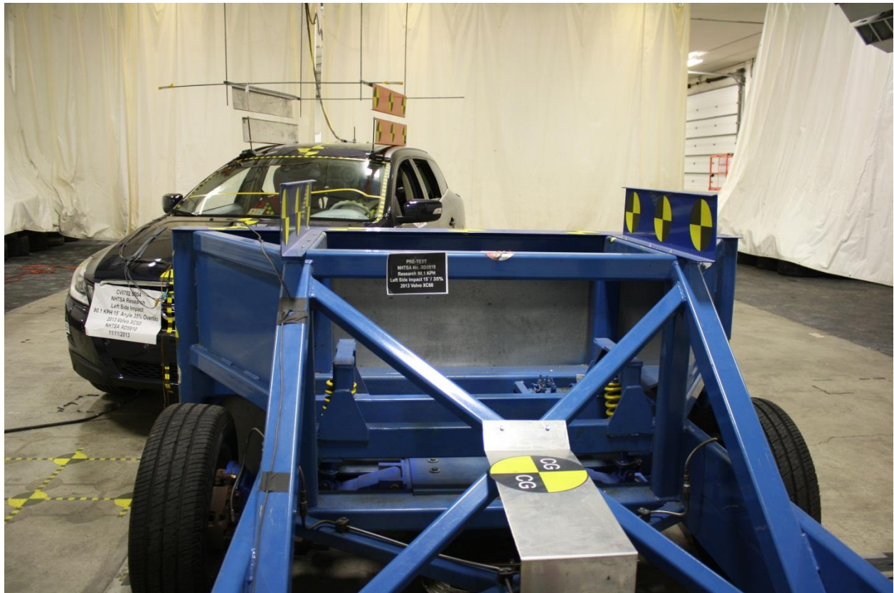
No. 176 Pre-Test RMDB & Vehicle, Rear View
