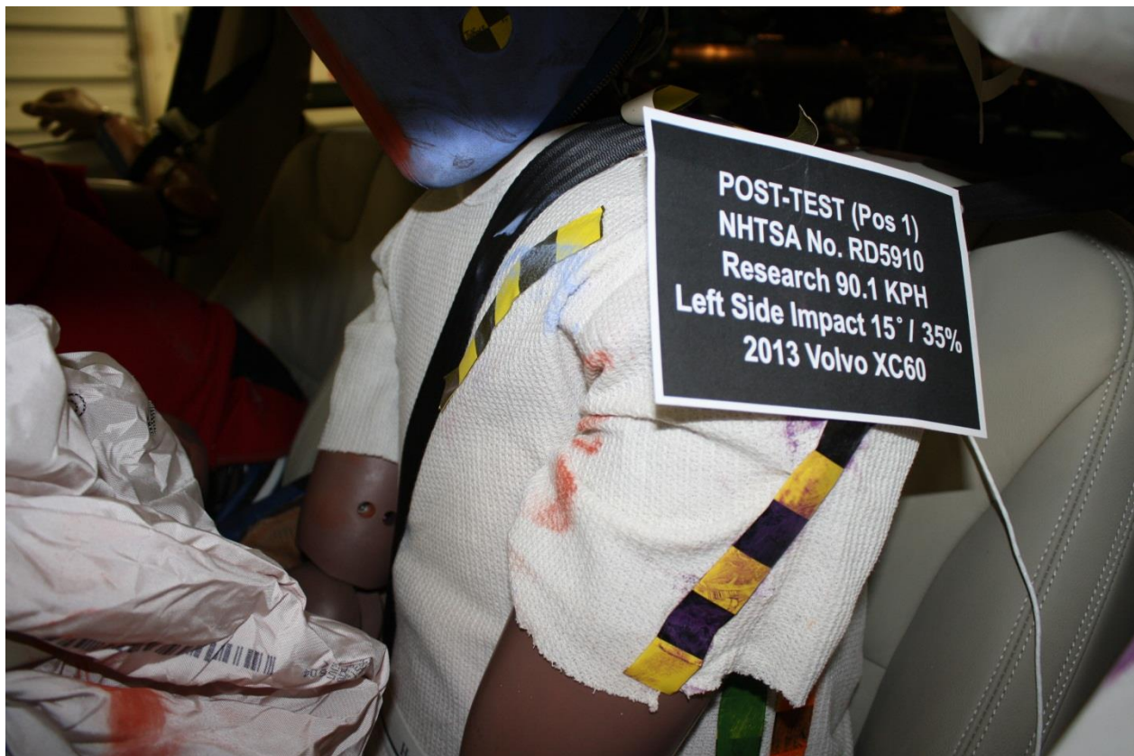
No. 076 Post-Test View of Driver Abdomen
