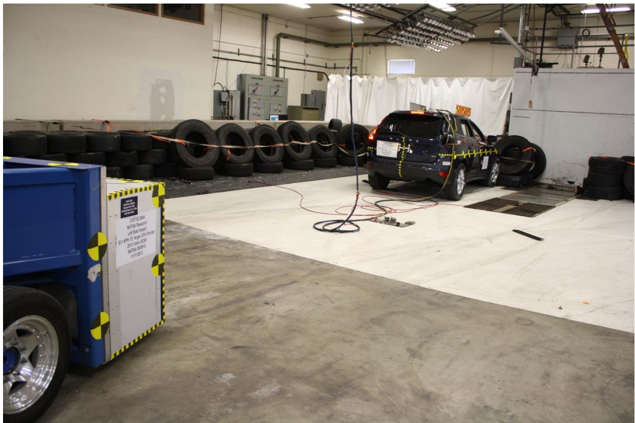
No. 171 Post-Test RMDB & Vehicle, Right Side
