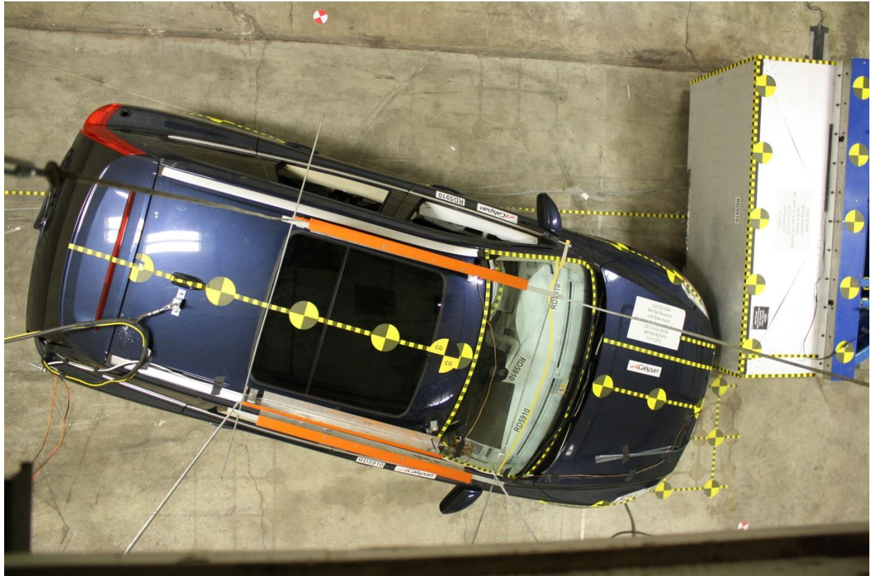
No. 174 Pre-Test RMDB & Vehicle, Top View
