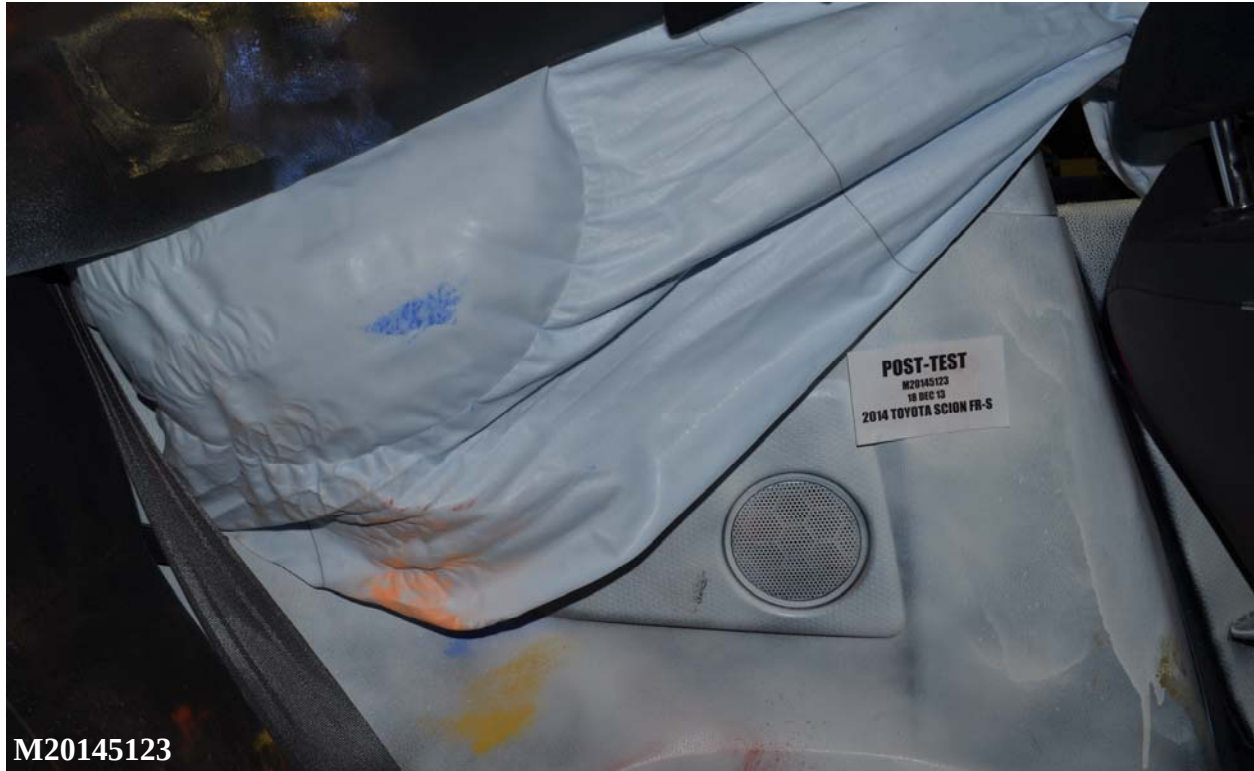
Figure A-77: Post-Test Rear Passenger Dummy Close-Up Torso Contact with Vehicle Interior View
