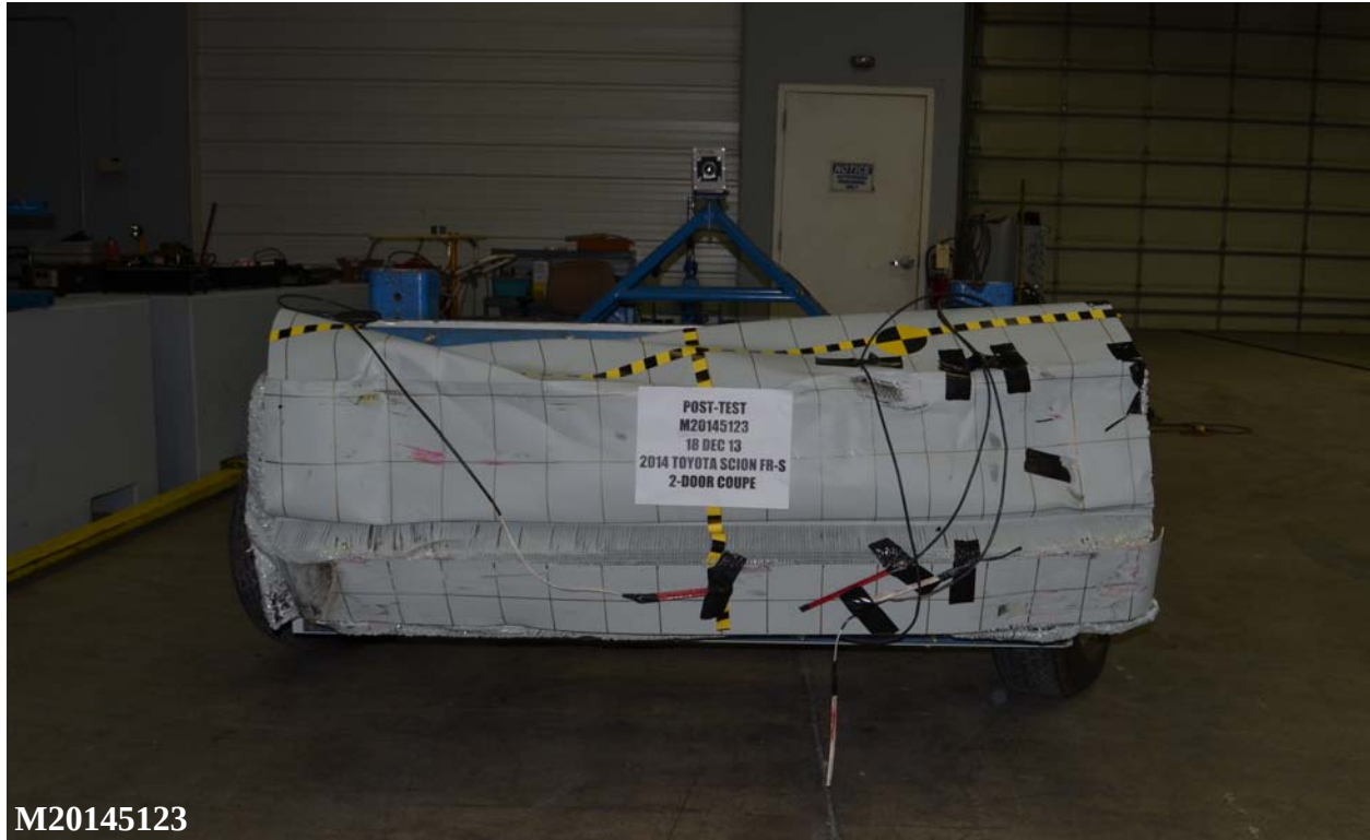
Figure A-85: Post-Test Front View of MDB Impactor Face
