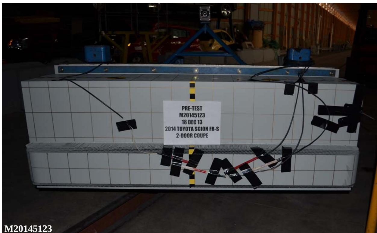
Figure A-84: Pre-Test Front View of MDB Impactor Face
