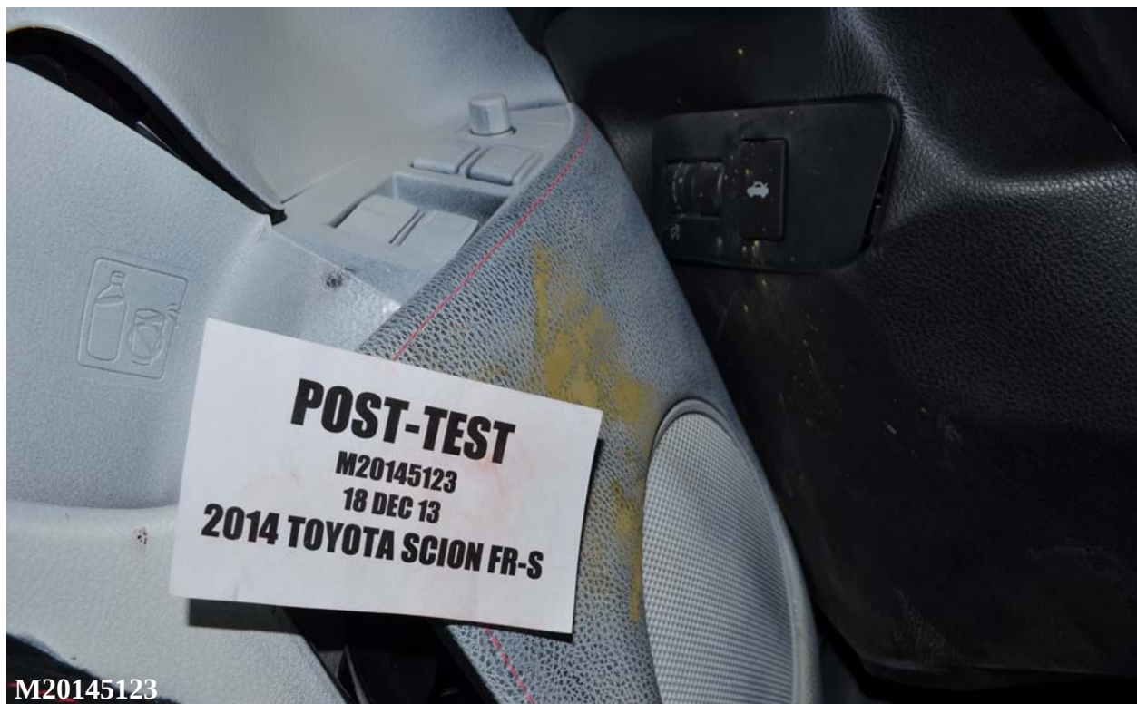
Figure A-54: Post-Test Driver Dummy Close-Up Knee Contact View
