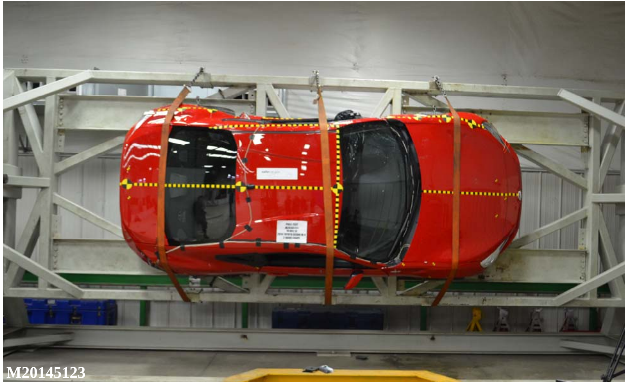
Figure A-97: FMVSS No. 301 Static Rollover 90 Degrees
