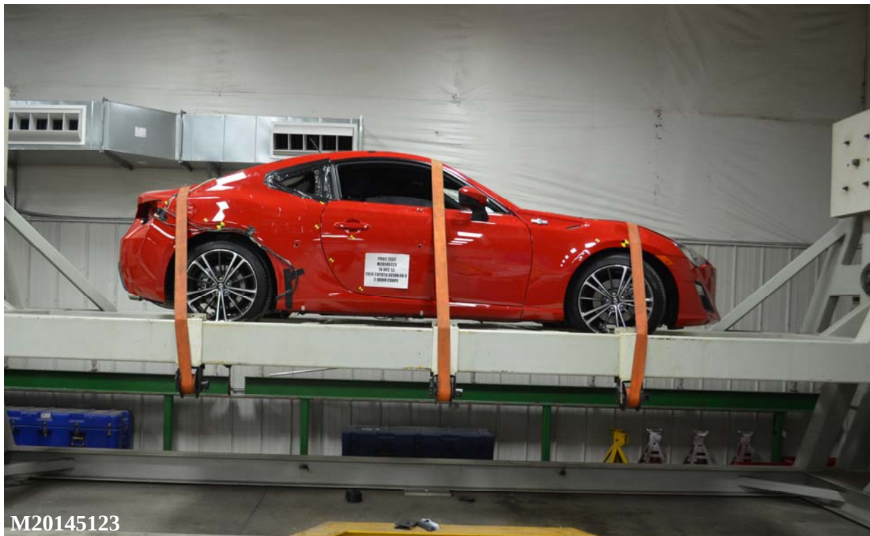
Figure A-100: FMVSS No. 301 Static Rollover 360 Degrees
