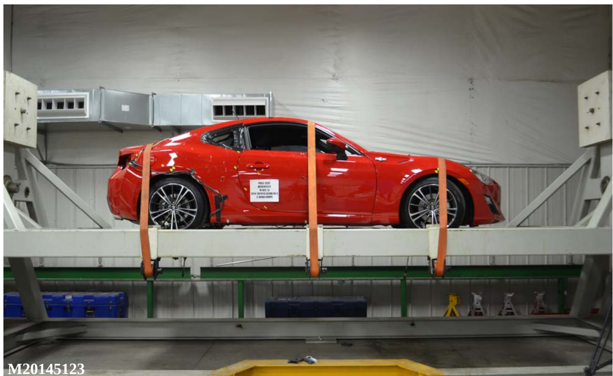
Figure A-96: FMVSS No. 301 Static Rollover 0 Degrees
