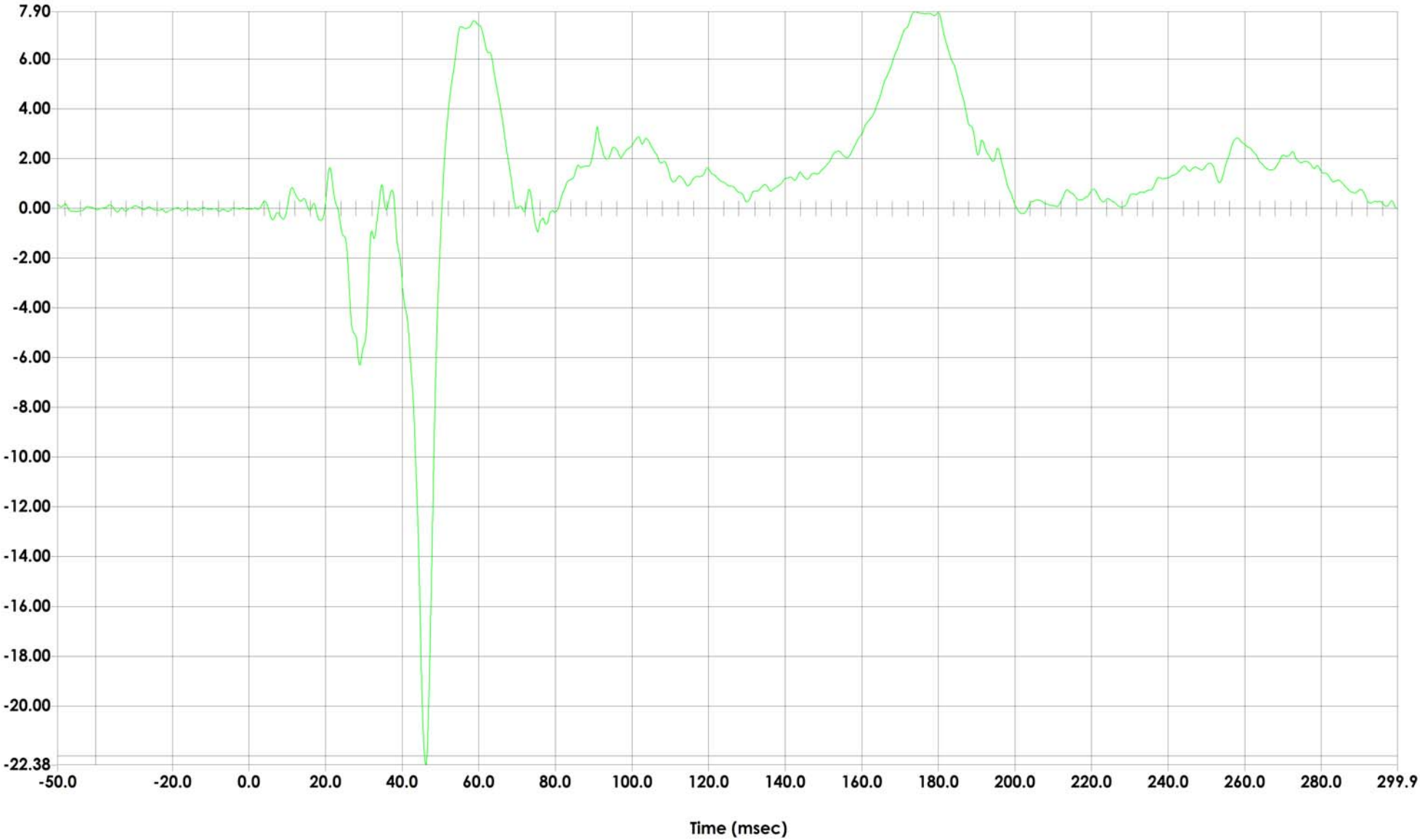
Passenger Lower Spine T12 Acceleration (X) vs. Time
