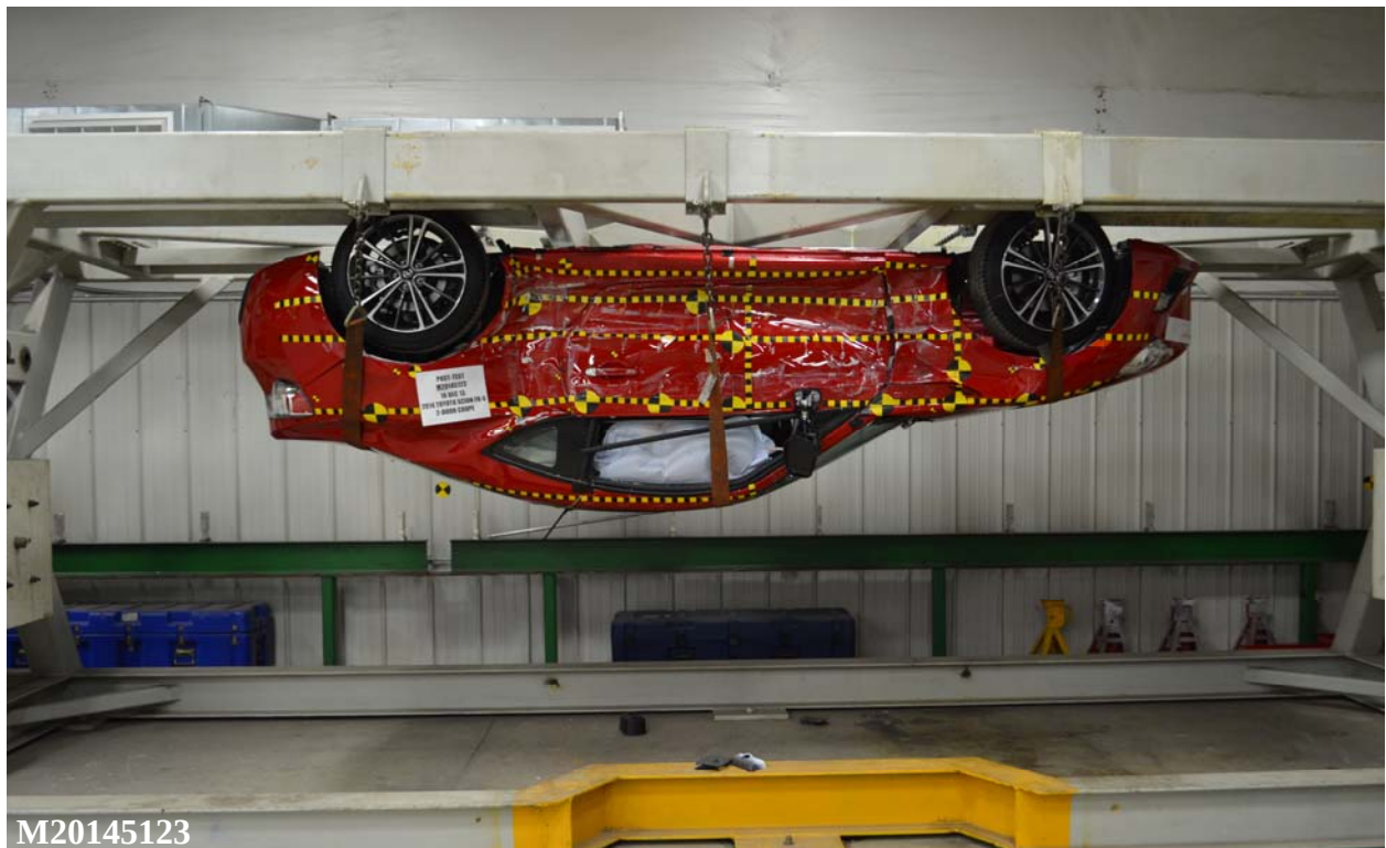
Figure A-98: FMVSS No. 301 Static Rollover 180 Degrees
