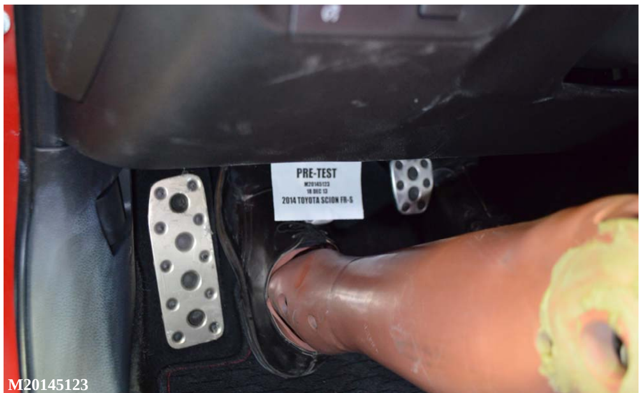
Figure A-34: Pre-Test Placement of Driver Dummy's Feet
