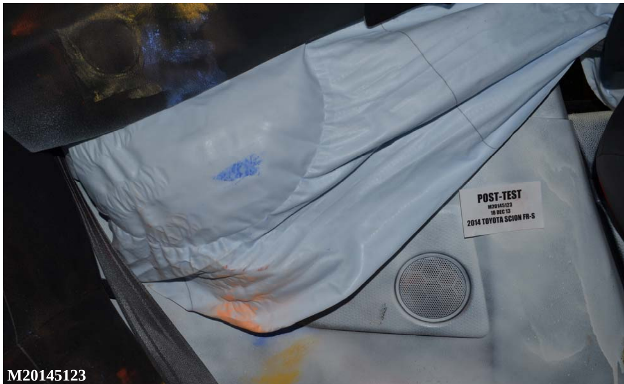
Figure A-78: Post-Test Rear Passenger Dummy Close-Up Torso Contact with Side Airbag View
