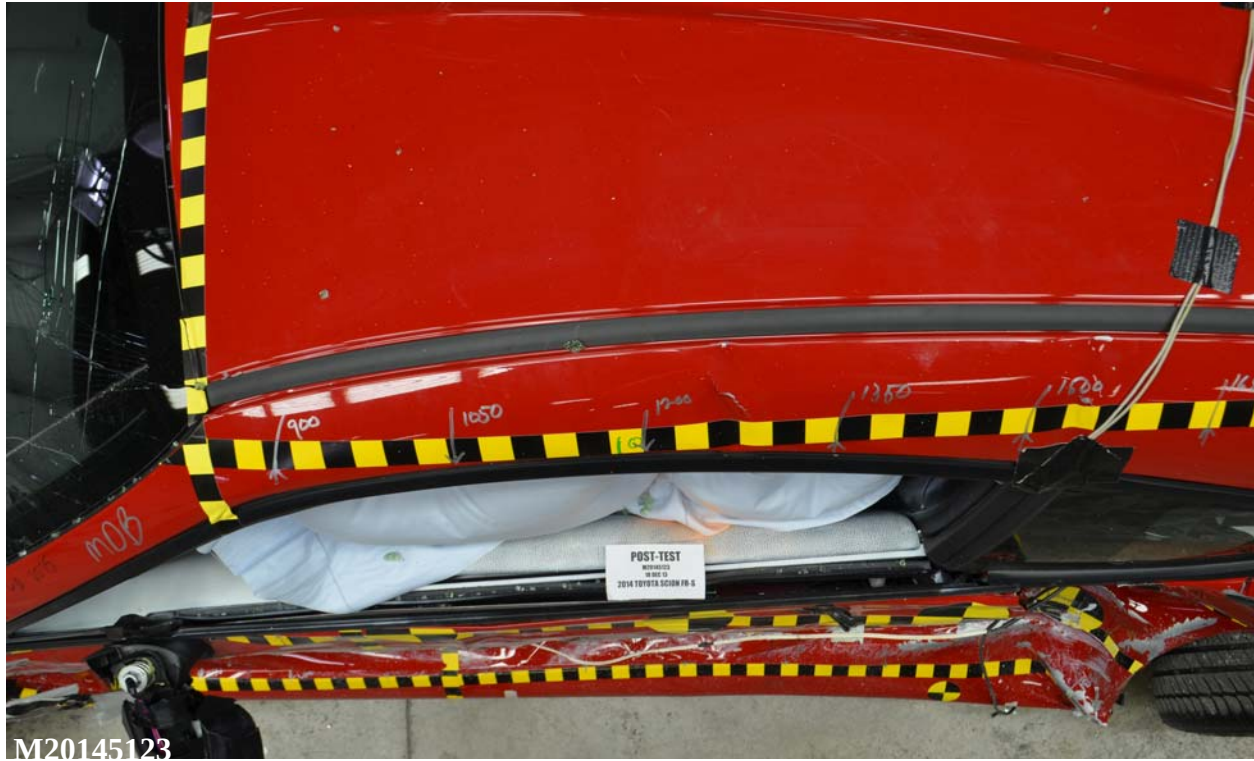
Figure A-43: Post-Test Driver Dummy and Door Clearance View
