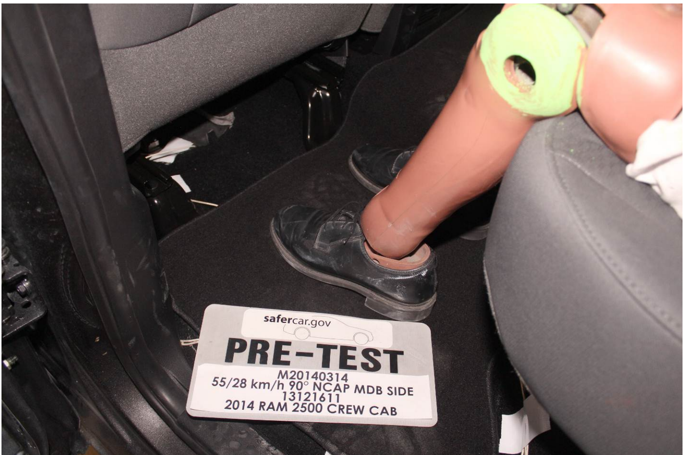
Pre-Test Placement of Rear Passenger Dummy's Feet
