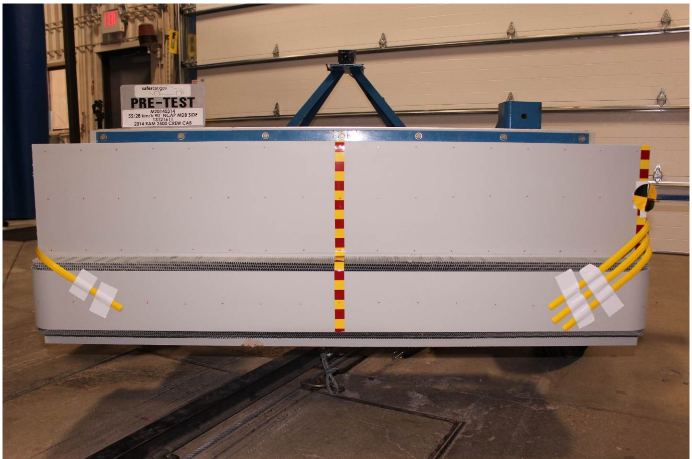
Pre-Test Front View of MDB Impactor Face
