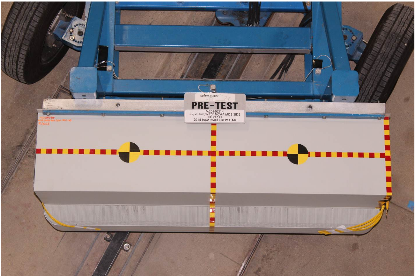
Pre-Test Top View of MDB Impactor Face
