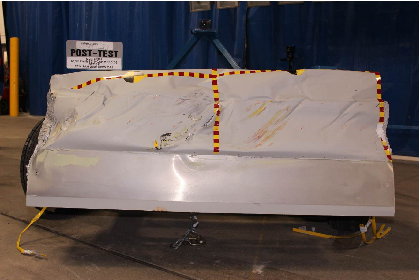
Post-Test Front View of MDB Impactor Face
