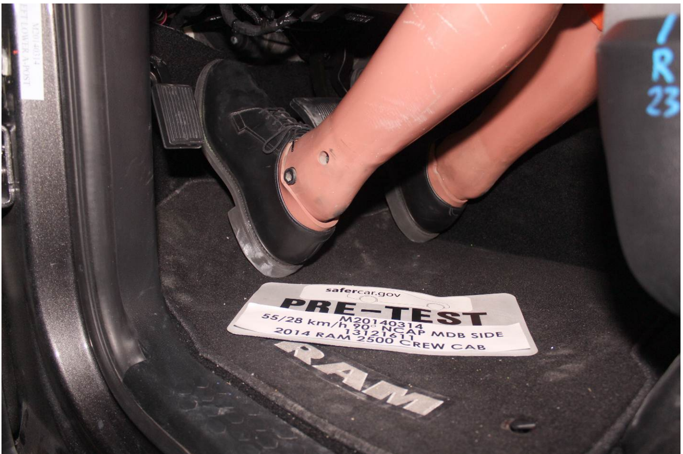
Pre-Test Placement of Driver Dummy's Feet
