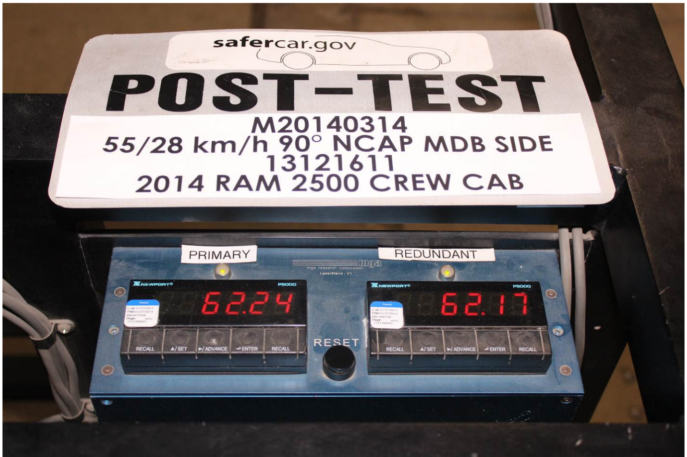
Post-Test Primary and Redundant Speed Trap Read-Out
