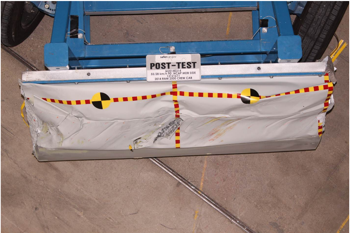
Post-Test Top View of MDB Impactor Face
