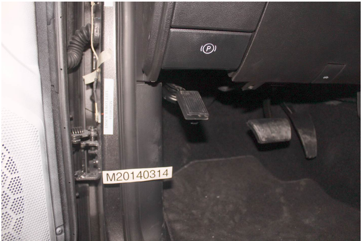
Pre-Test View of Disengaged Parking Brake
