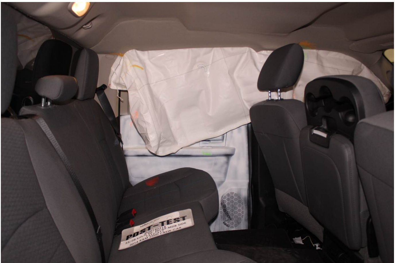
Post-Test Rear Passenger Inner Door Panel View
