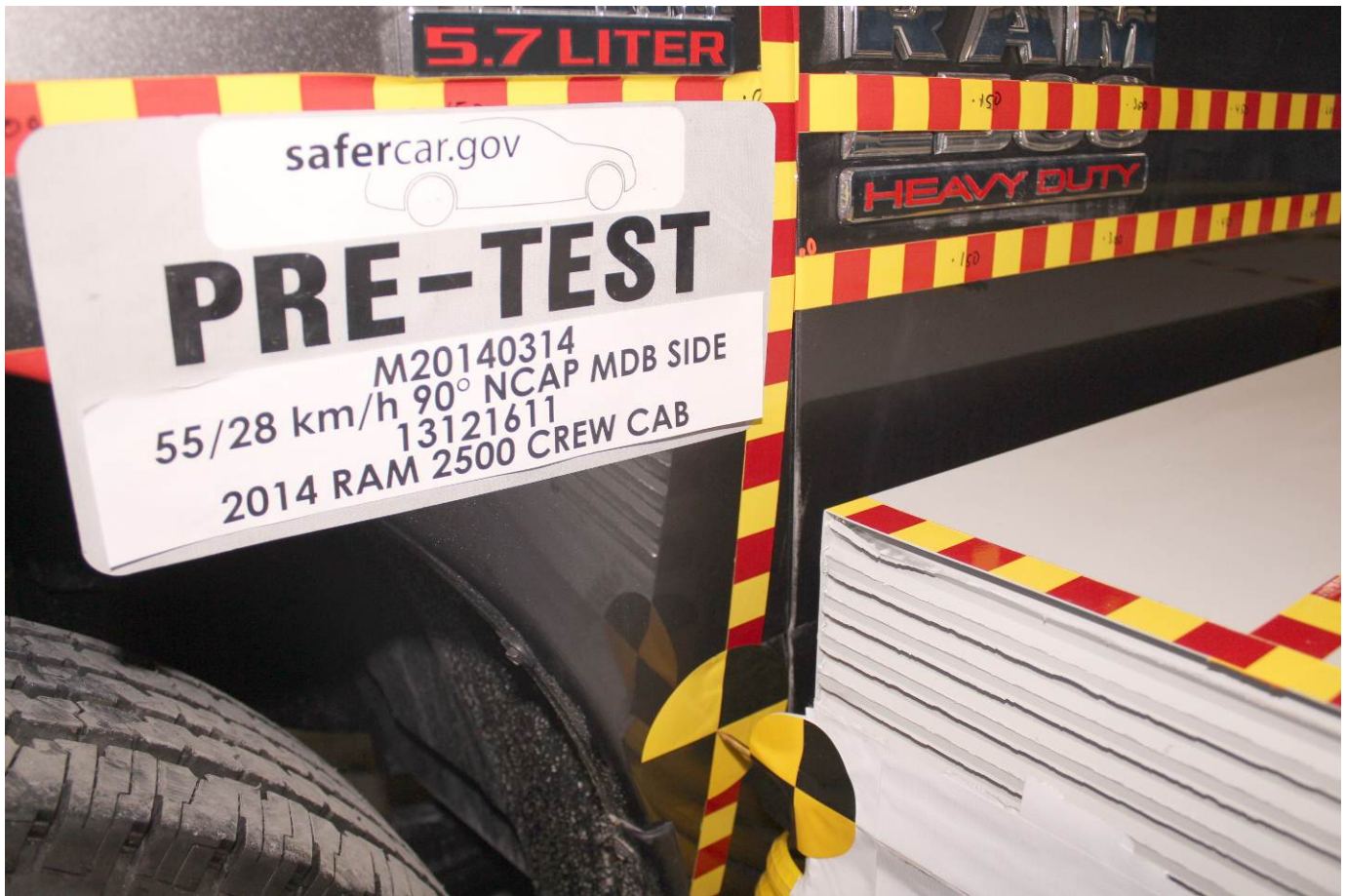
Pre-Test Close-Up View of Impact Point Target
