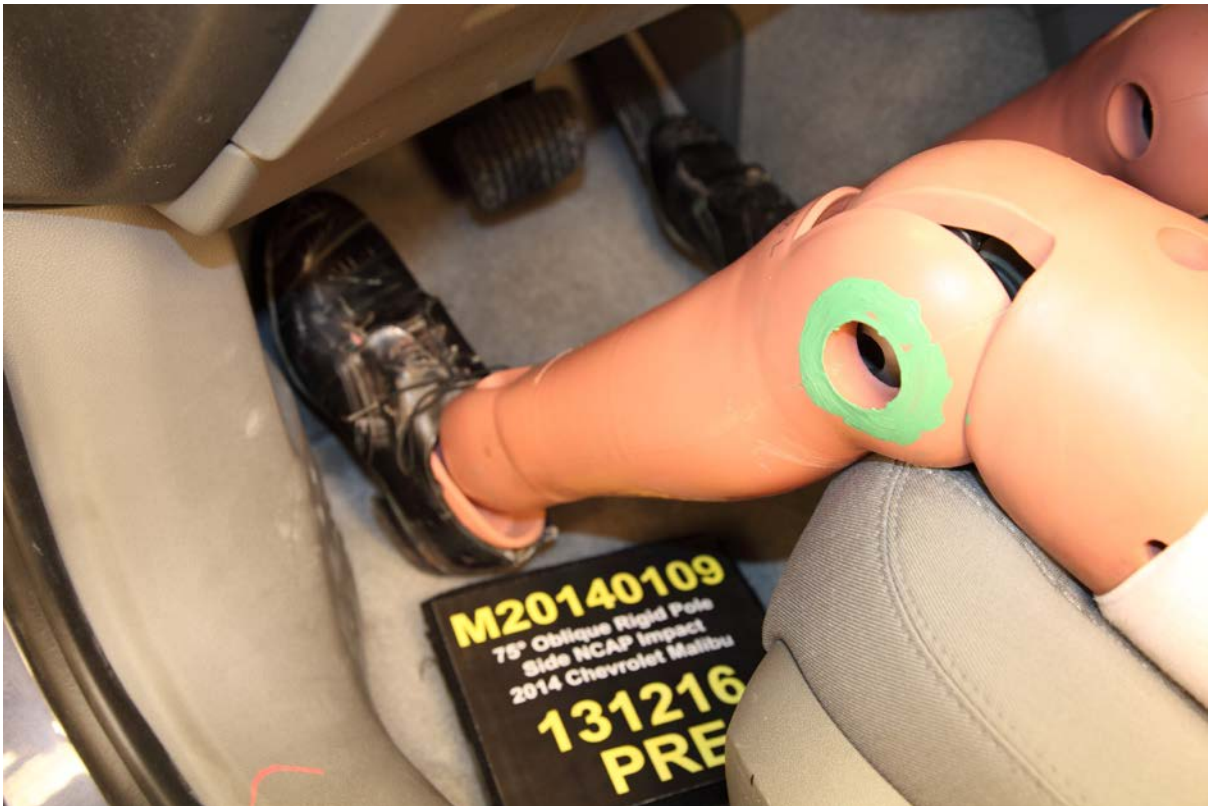
032 Pre-Test Placement of Dummy Feet
