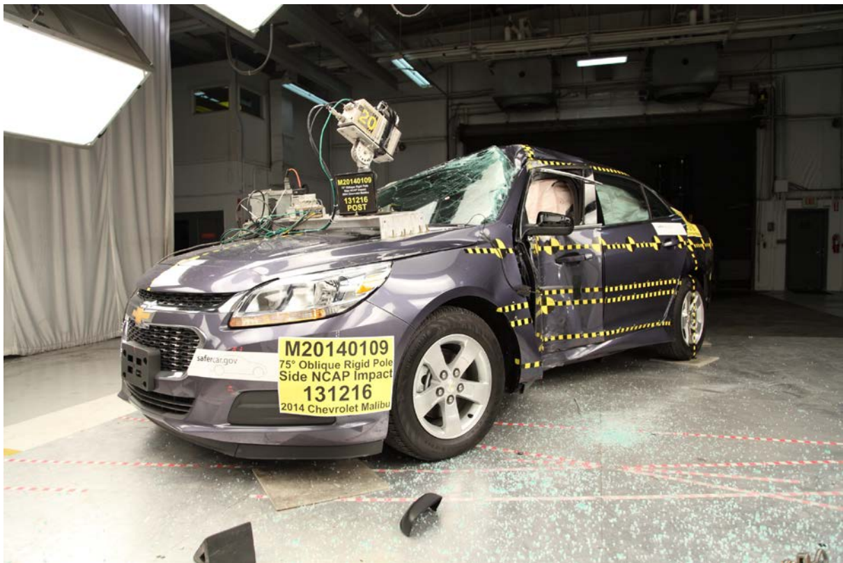
006 Post-Test Left Front 3-4 View of Test Vehicle
