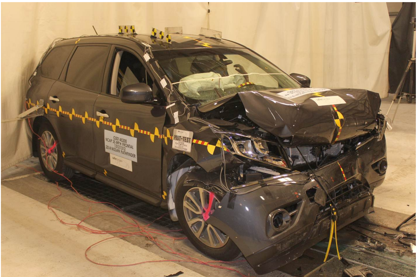
Post-Test Right Front 3-4 View
