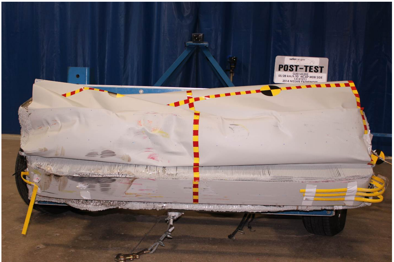
Post-Test Front View of MDB Impactor Face
