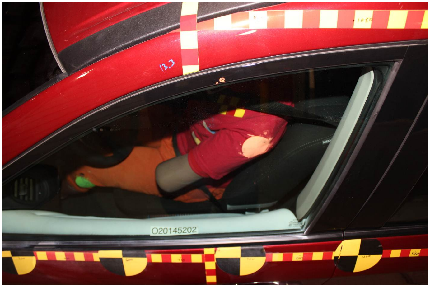
Pre-Test Driver Dummy and Door Clearance View
