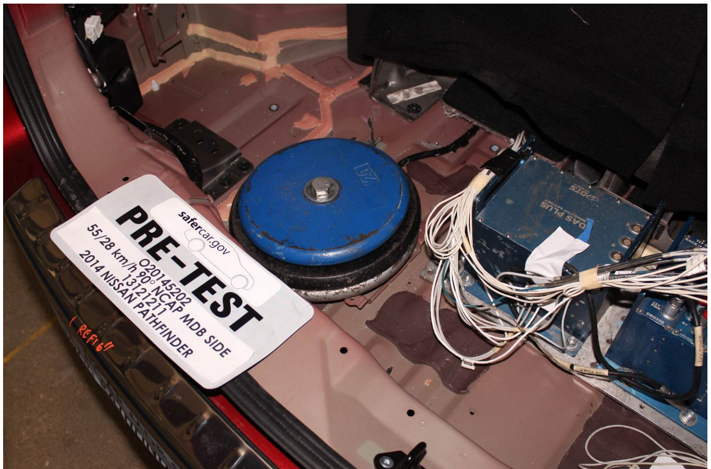
Pre-Test Ballast View
