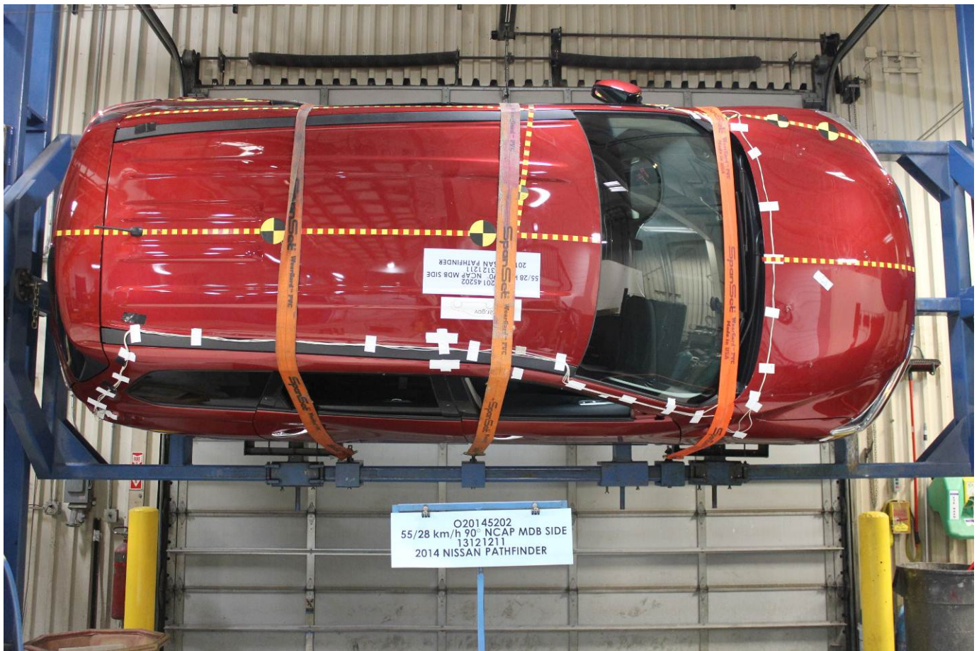
FMVSS No. 301 Static Rollover 270 Degrees
