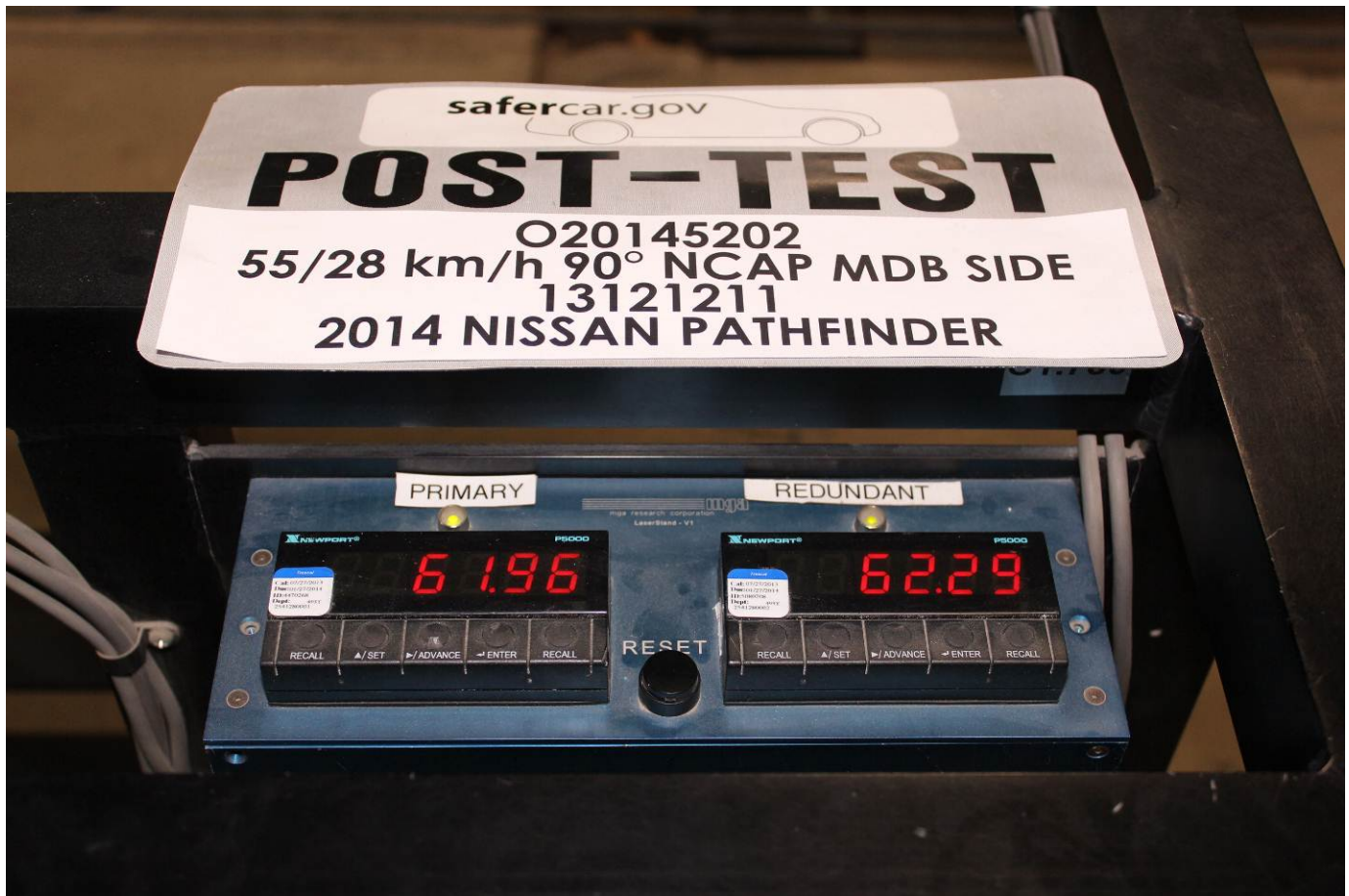
Post-Test Primary and Redundant Speed Trap Read-Out
