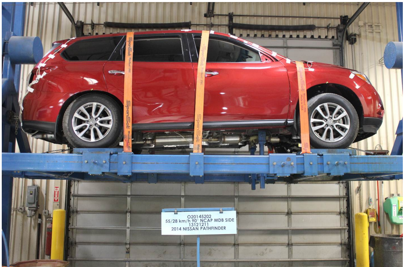
FMVSS No. 301 Static Rollover 0 Degrees
