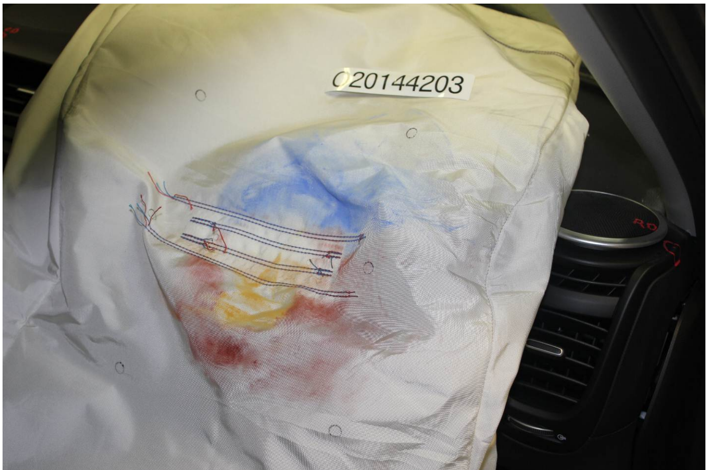
Post-Test Passenger Dummy Contact with Airbag
