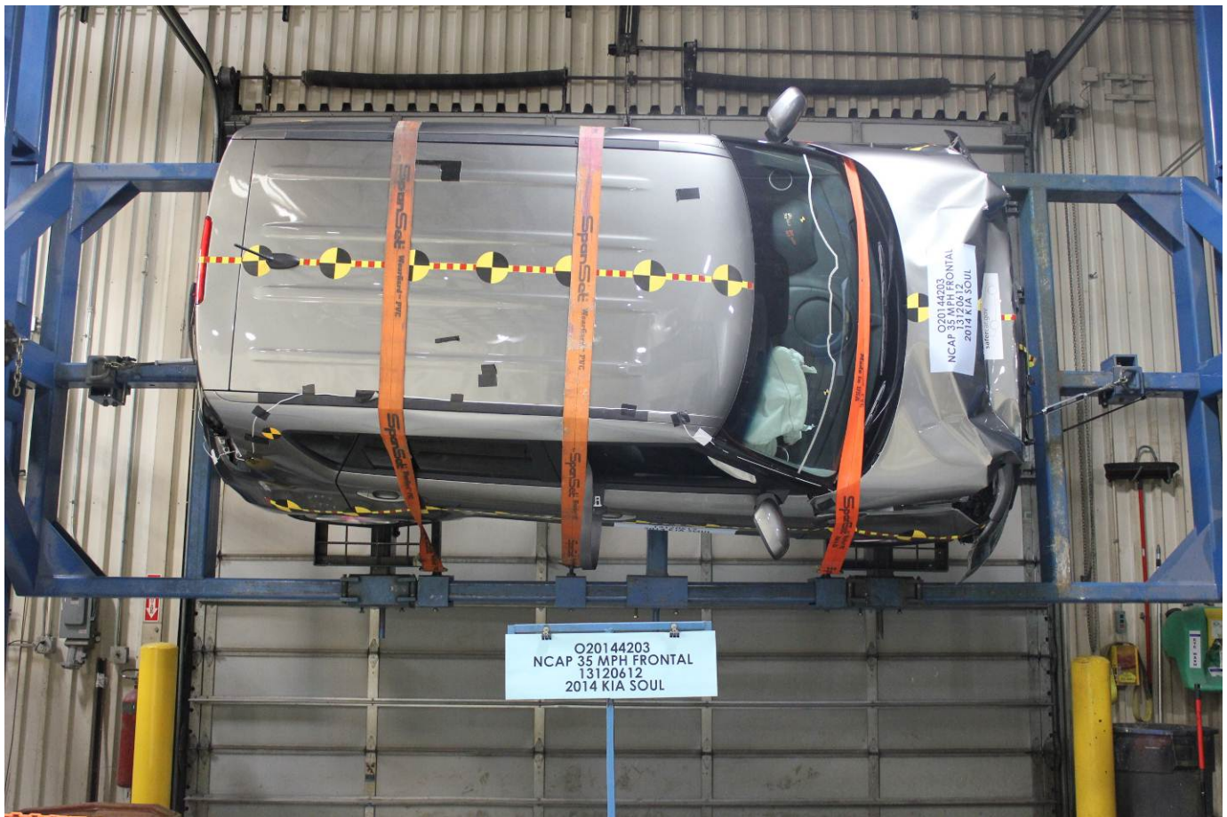
Vehicle at 270 Degrees on Static Rollover Device
