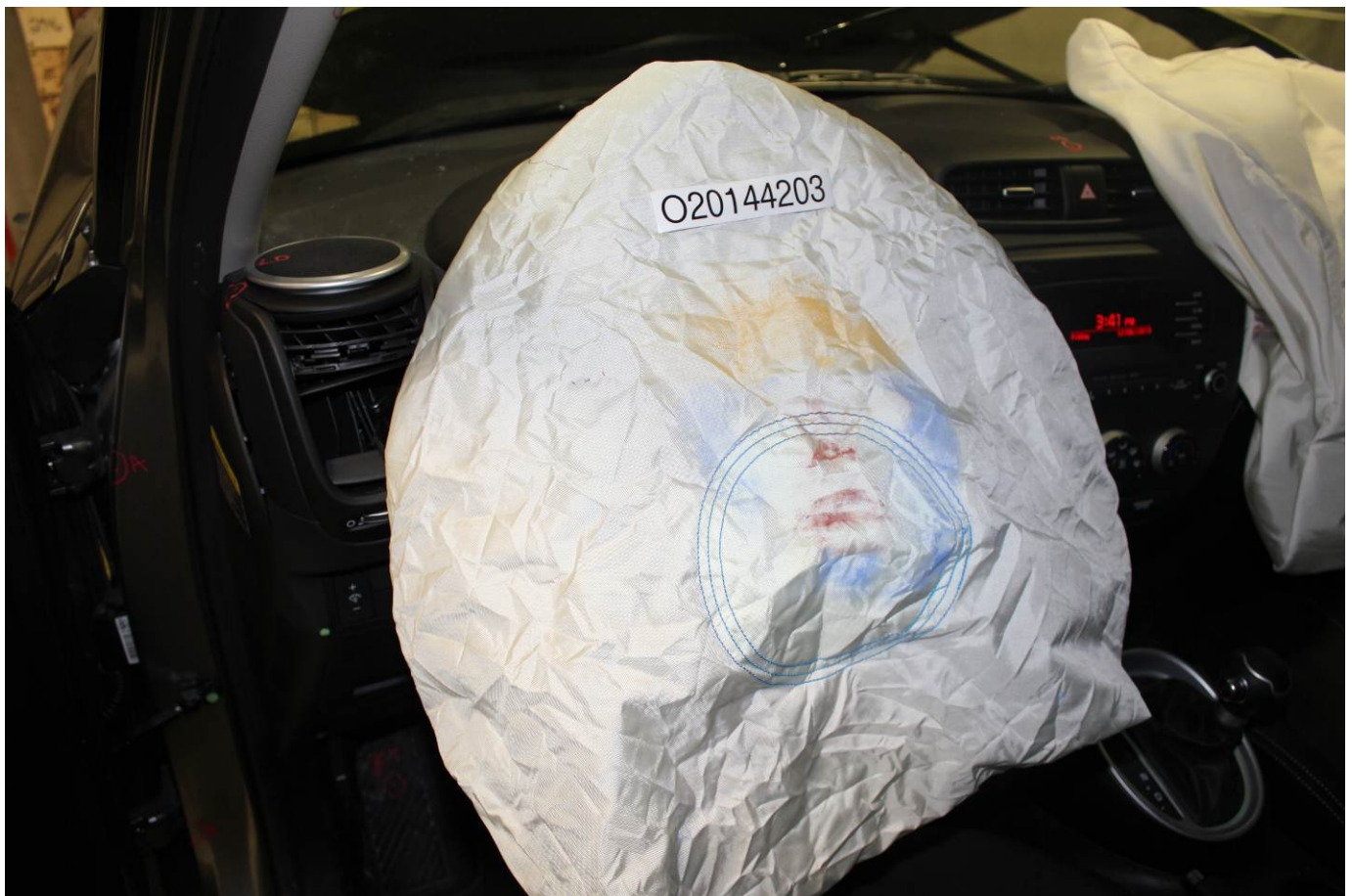
Post-Test Driver Dummy Contact with Airbag
