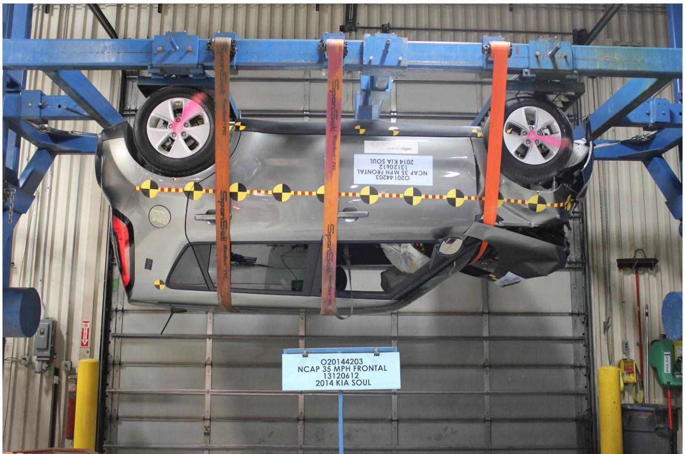
Vehicle at 180 Degrees on Static Rollover Device
