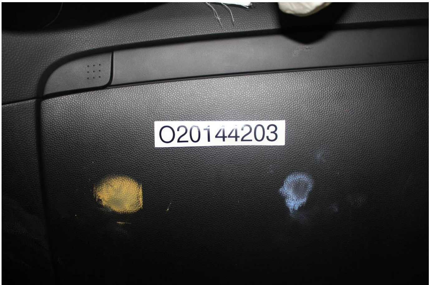
Post-Test Passenger Dummy Contact with Glovebox
