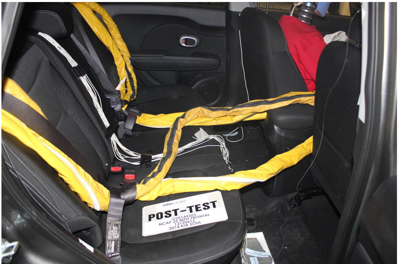
Post-Test Dummy Cable Routing
