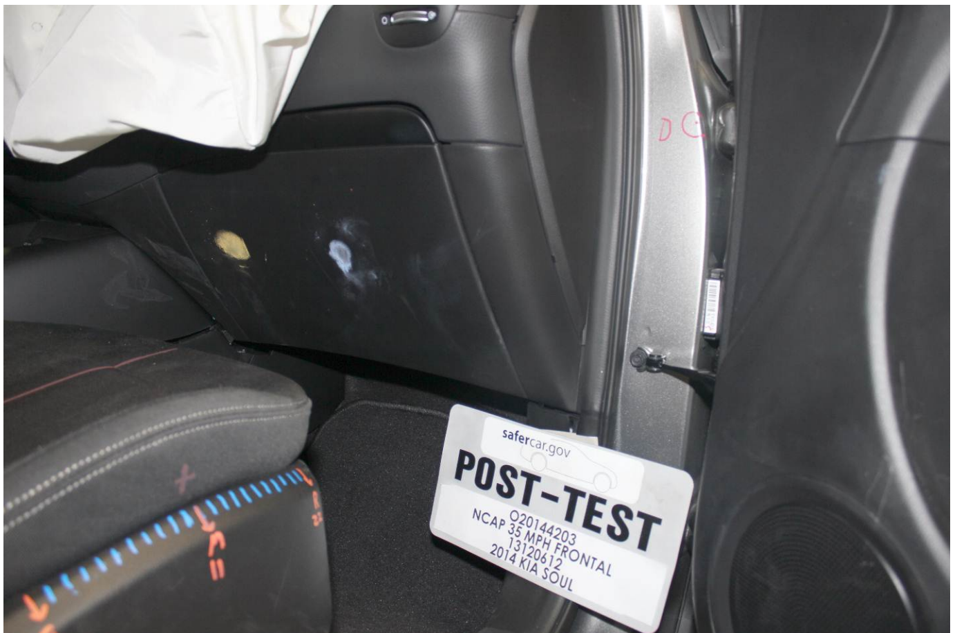
Post-Test Passenger's Side Knee Bolster (without dummy)
