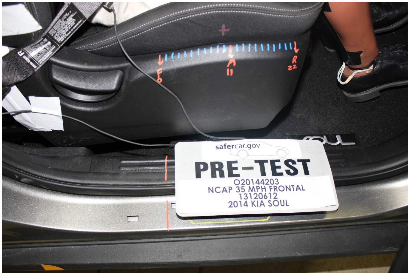
Pre-Test Passenger's Seat Fore-Aft Markings
