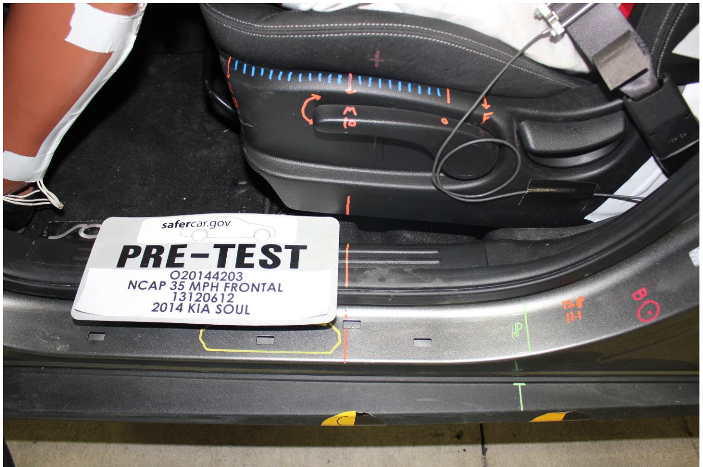
Pre-Test Driver's Seat Fore-Aft Markings
