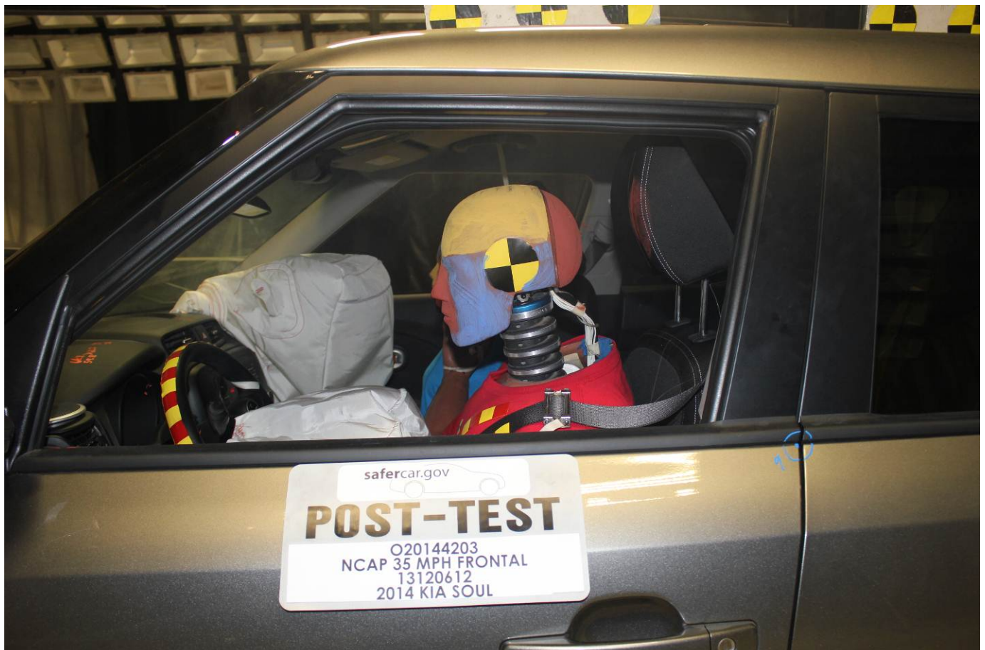
Post-Test Driver Dummy Window View
