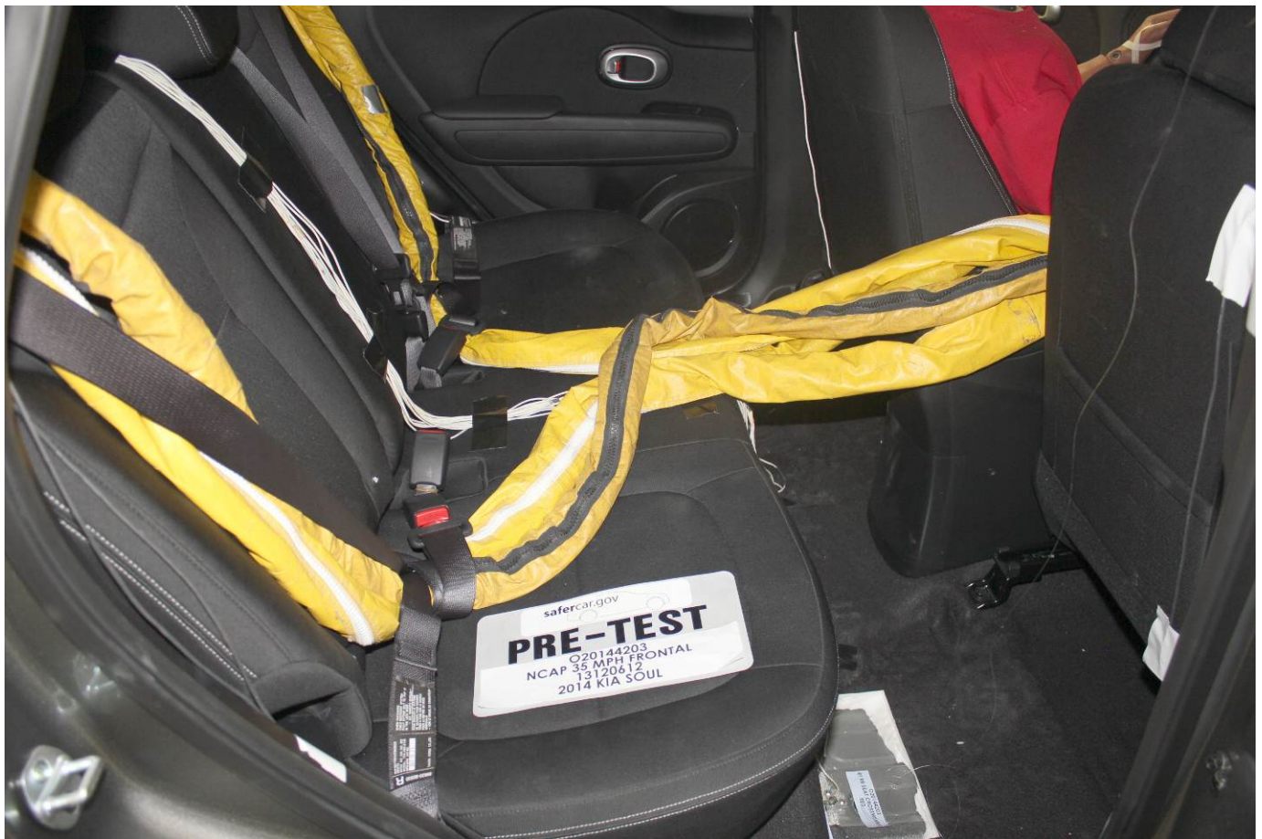
Pre-Test Dummy Cable Routing
