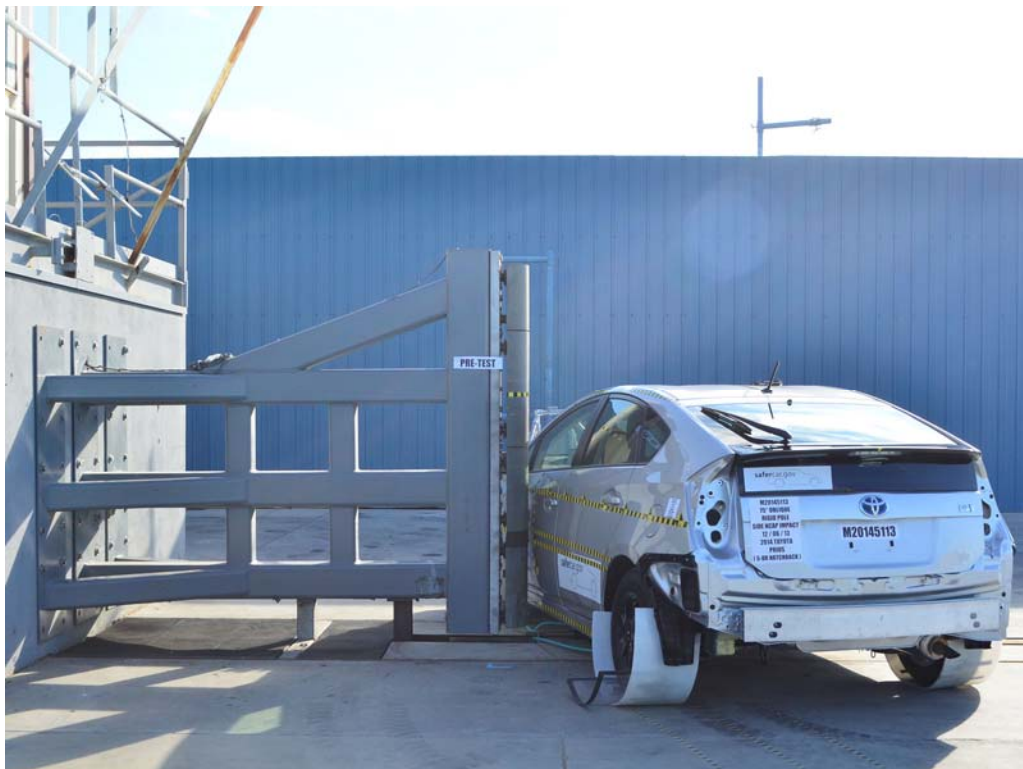
FIGURE 18. Pre-Test Right Side View of Pole Positioned Against Side of Vehicle
