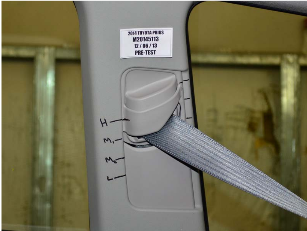
FIGURE 33. Pre-Test View of Belt Anchorage for Dummy
