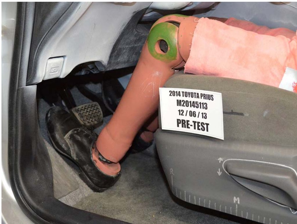
FIGURE 32. Pre-Test Placement of Dummy's Feet
