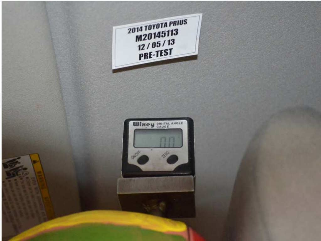
FIGURE 31. Pre-Test Left Side View of Dummy's Head Showing Dummy's Head is Level
