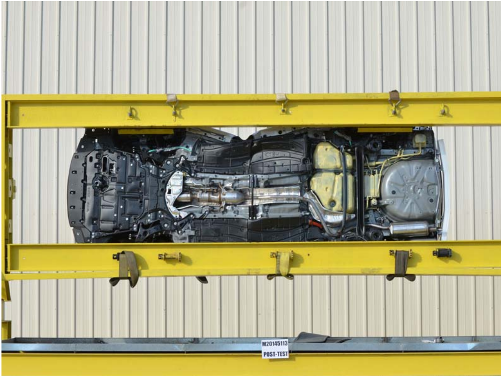
FIGURE 66. FMVSS No. 301 Static Rollover 270 Degrees
