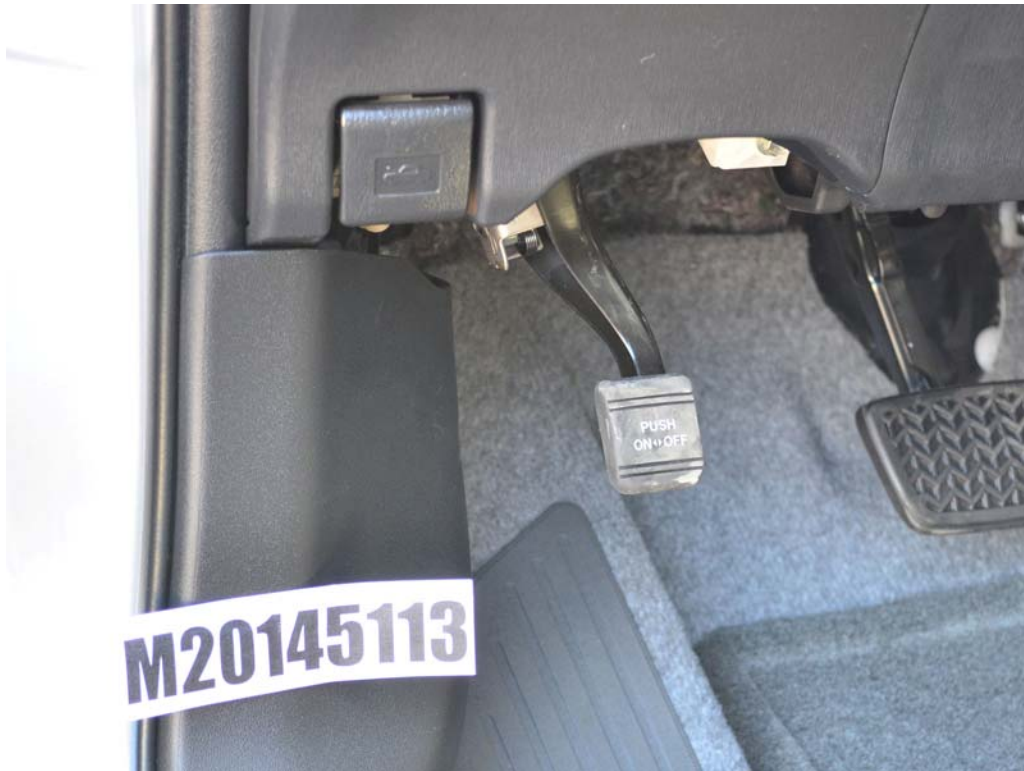
FIGURE 35. View of Disengaged Parking Brake
