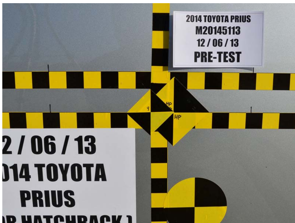
FIGURE 19. Pre-Test Close-Up View of Impact Point Target
