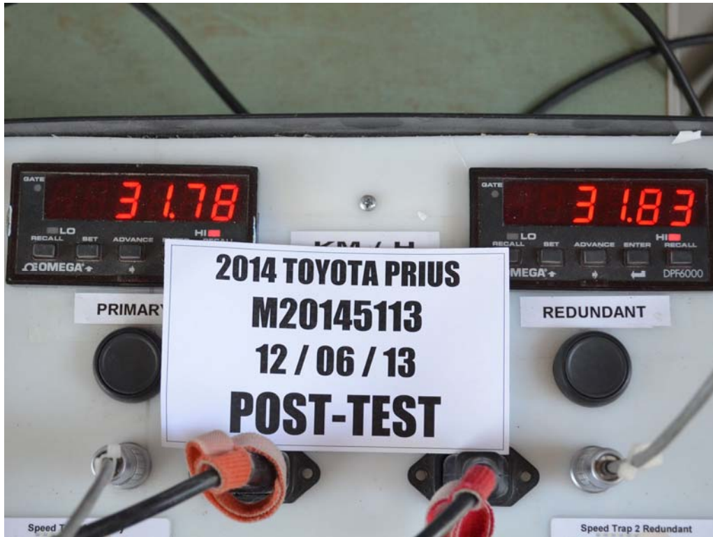
FIGURE 62. Post-Test Primary and Redundant Speed Trap Read-Out
