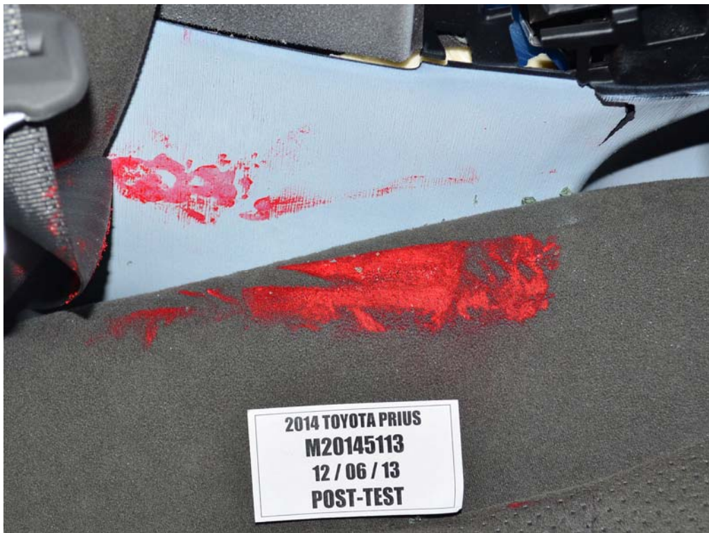
FIGURE 50. Post-Test Dummy Close-Up Pelvis Contact With Vehicle Interior View
