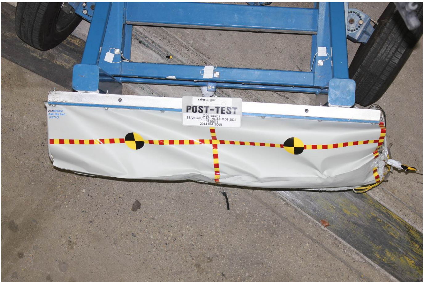
Post-Test Top View of MDB Impactor Face
