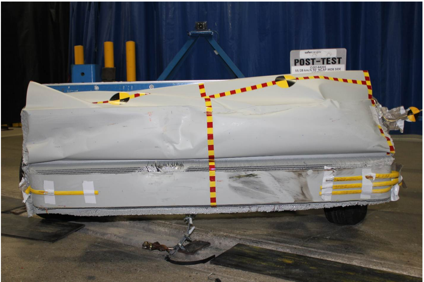
Post-Test Front View of MDB Impactor Face
