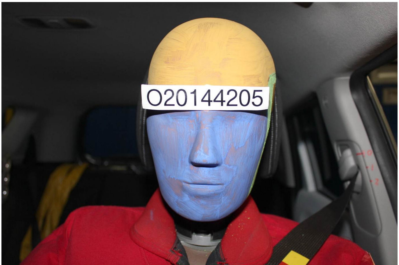
Pre-Test Frontal View of Driver Dummy Head and Shoulders in Relation to Head Restraint
