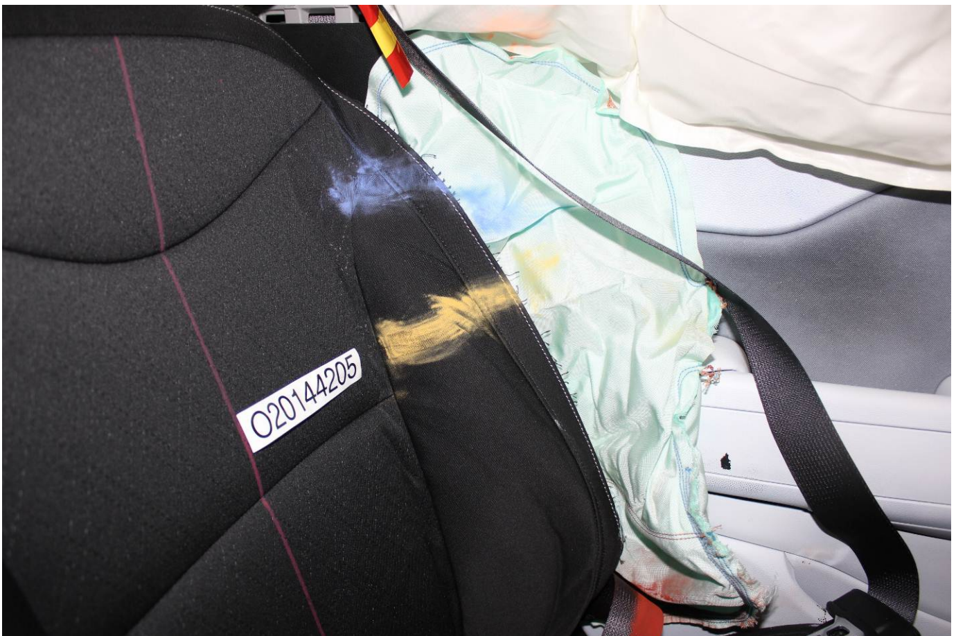
Post-Test Driver Dummy Close-up Torso Contact with Vehicle Interior View
