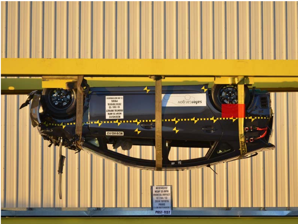
FIGURE 30. FMVSS No. 305 Static Rollover at 180°
