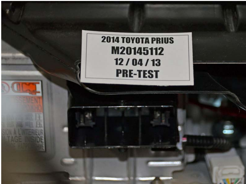
FIGURE 8. Manual High Voltage Service Disconnect Removed
