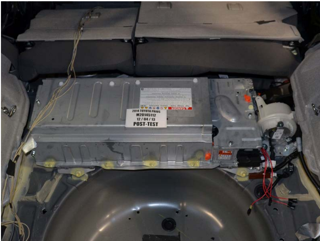
FIGURE 11. Post-Impact Rear View of Propulsion Battery
