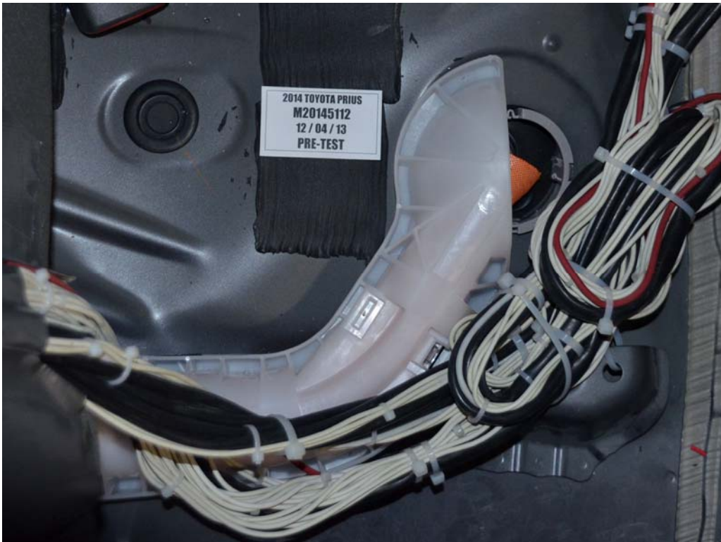
FIGURE 18c. Pre-Impact View of High Voltage Interconnects
