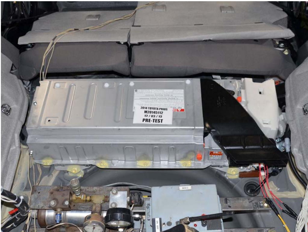
FIGURE 9a. Pre-Impact View of Propulsion Battery
