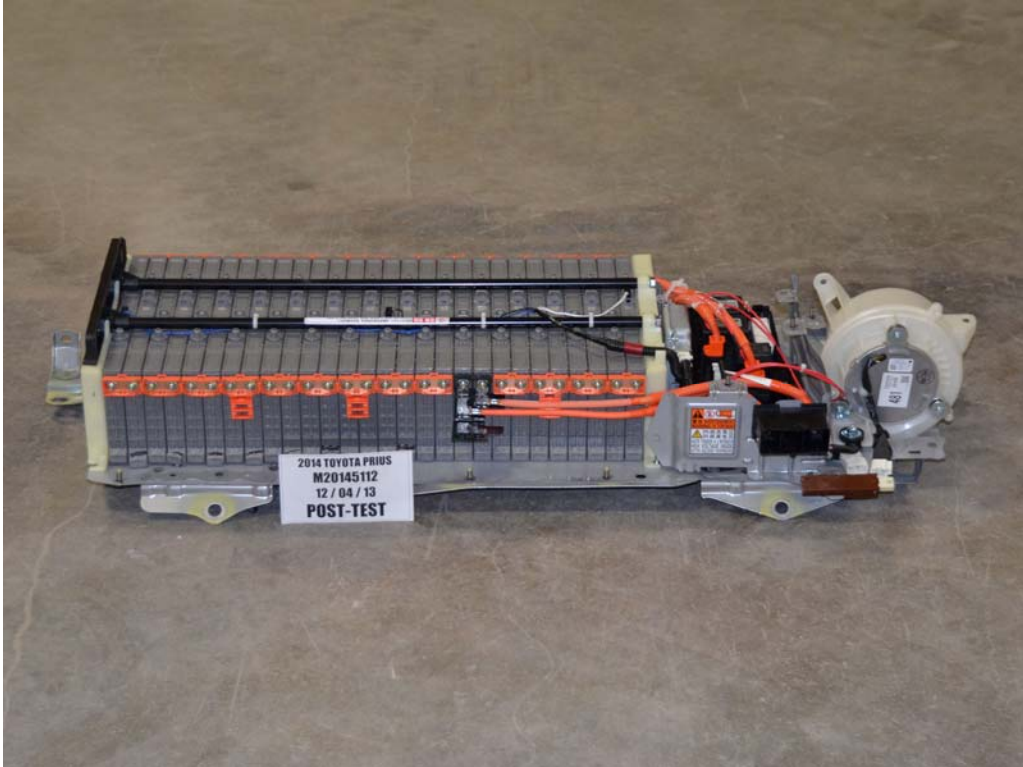
FIGURE 15c. Post-Impact View of Propulsion Battery Modules
