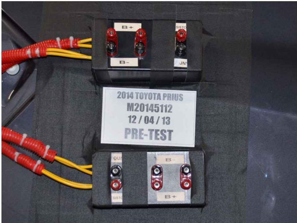
FIGURE 24. Pre-Impact View of Installed Test Interface Port
