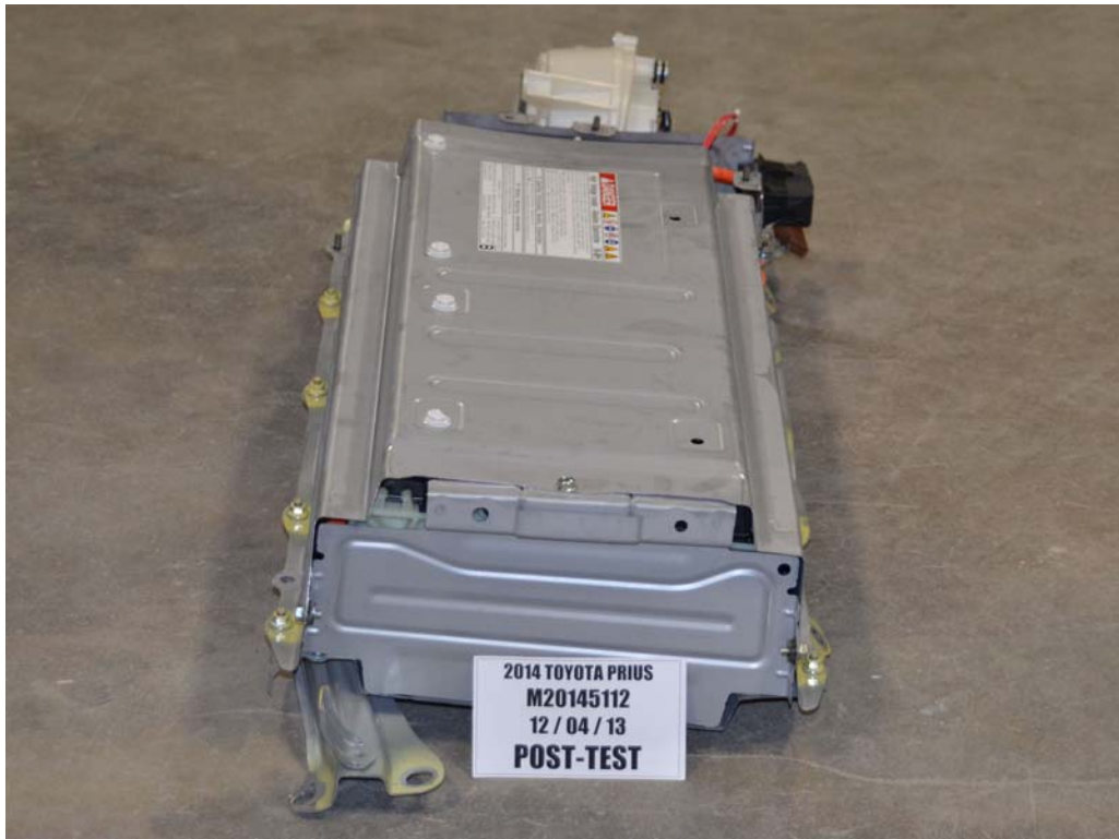
FIGURE 13d. Post-Impact View of Battery Box or Container which Holds Individual Battery Modules
