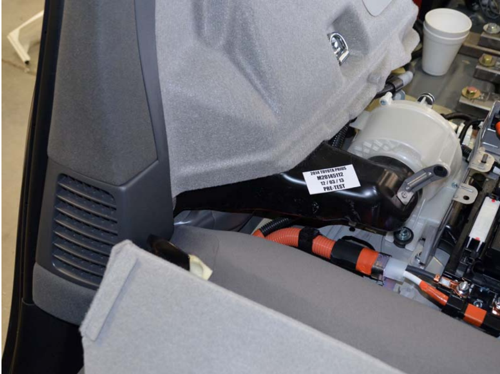
FIGURE 19. Pre-Impact View of Propulsion Battery Venting System
