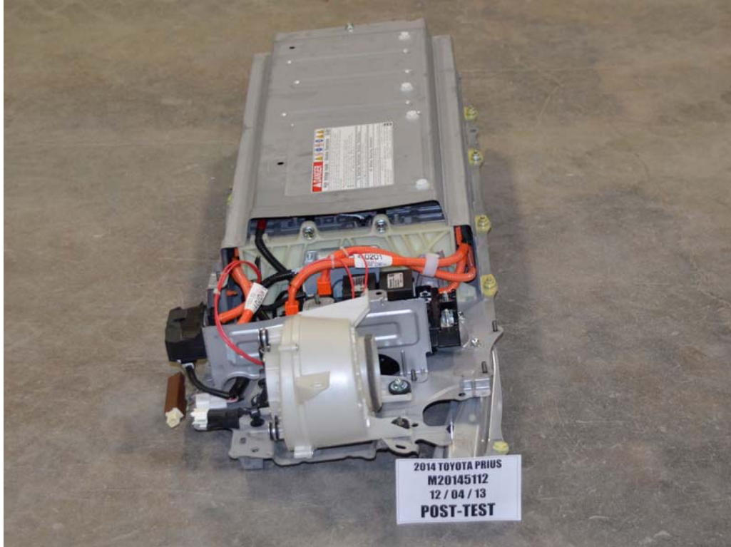
FIGURE 13c. Post-Impact View of Battery Box or Container which Holds Individual Battery Modules
