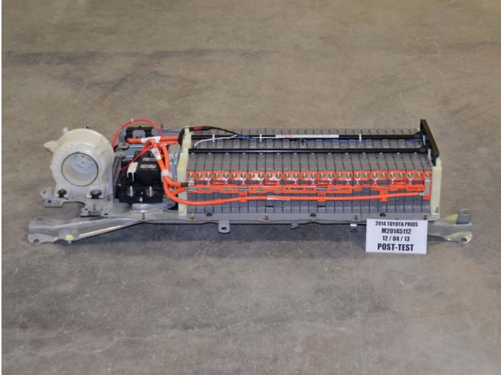
FIGURE 15a. Post-Impact View of Propulsion Battery Modules
