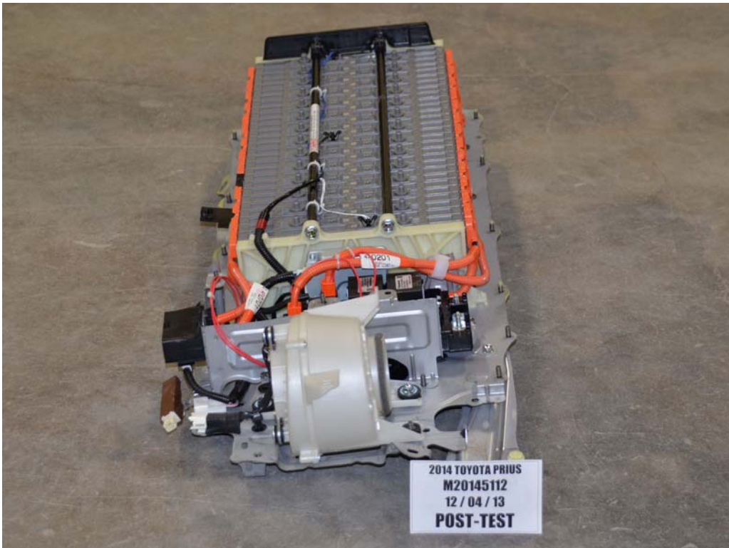
FIGURE 15b. Post-Impact View of Propulsion Battery Modules
