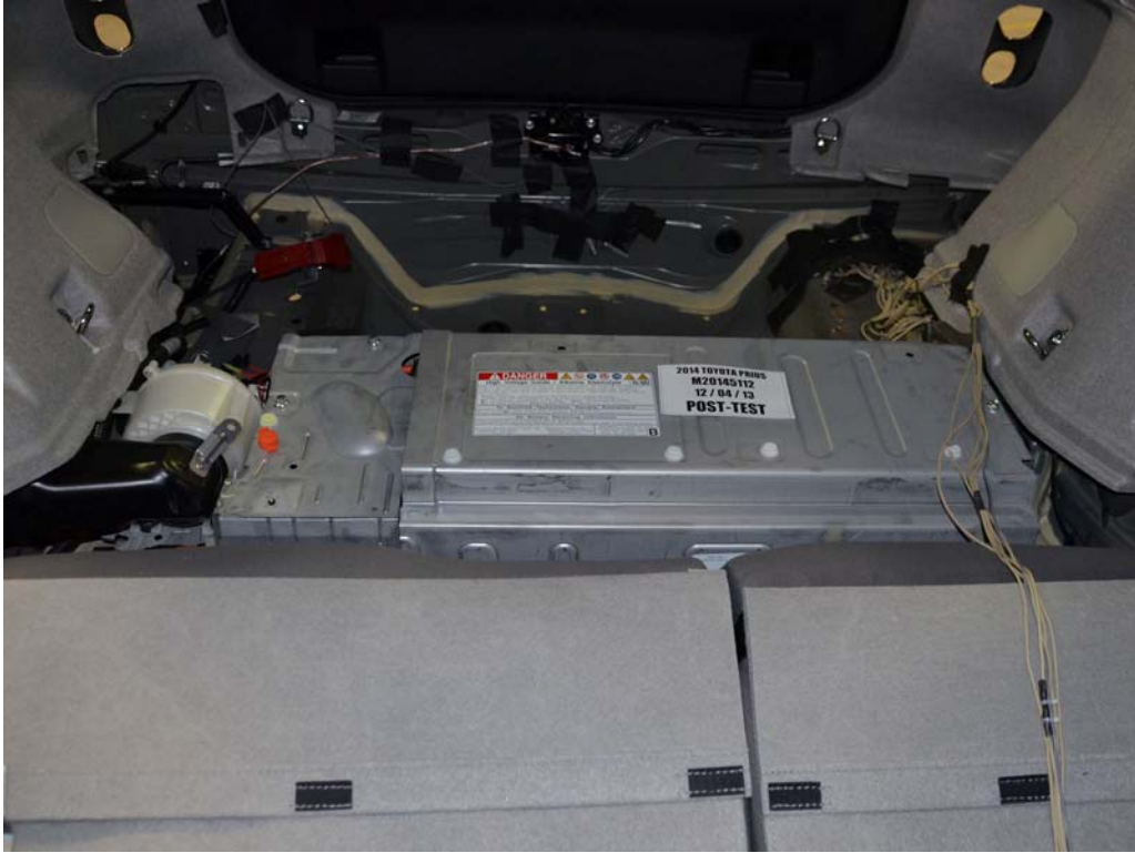
FIGURE 10. Post-Impact Front View of Propulsion Battery
