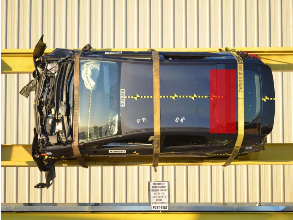
FIGURE 29. FMVSS No. 305 Static Rollover at 90°
