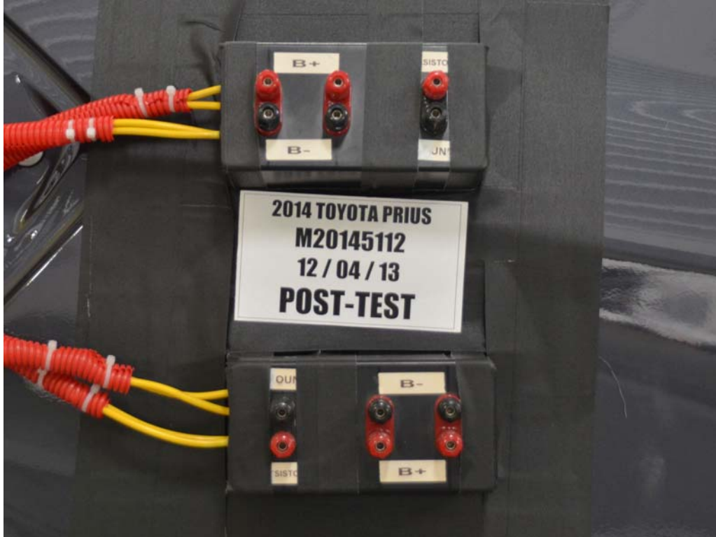
FIGURE 25. Post-Impact View of Installed Test Interface Port
