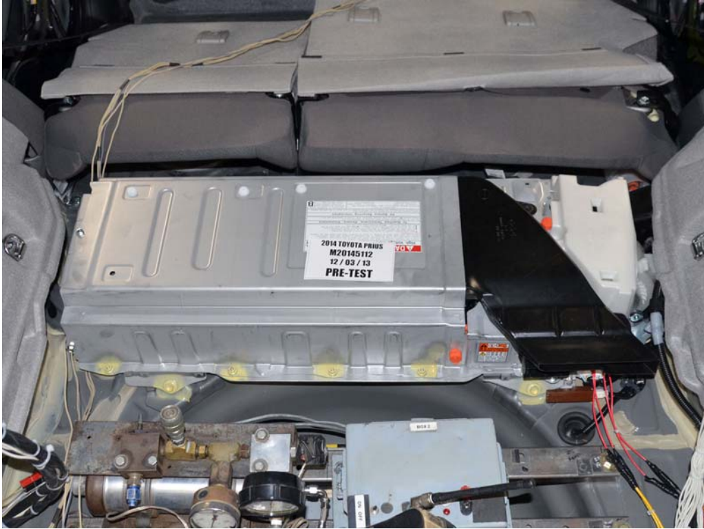
FIGURE 12. Pre-Impact View of Battery Box or Container which Holds Individual Battery Modules
