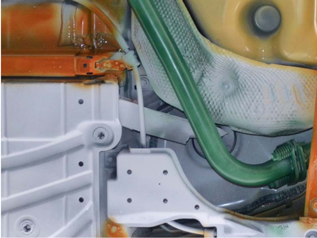
FIGURE 18b. Pre-Impact View of High Voltage Interconnects
