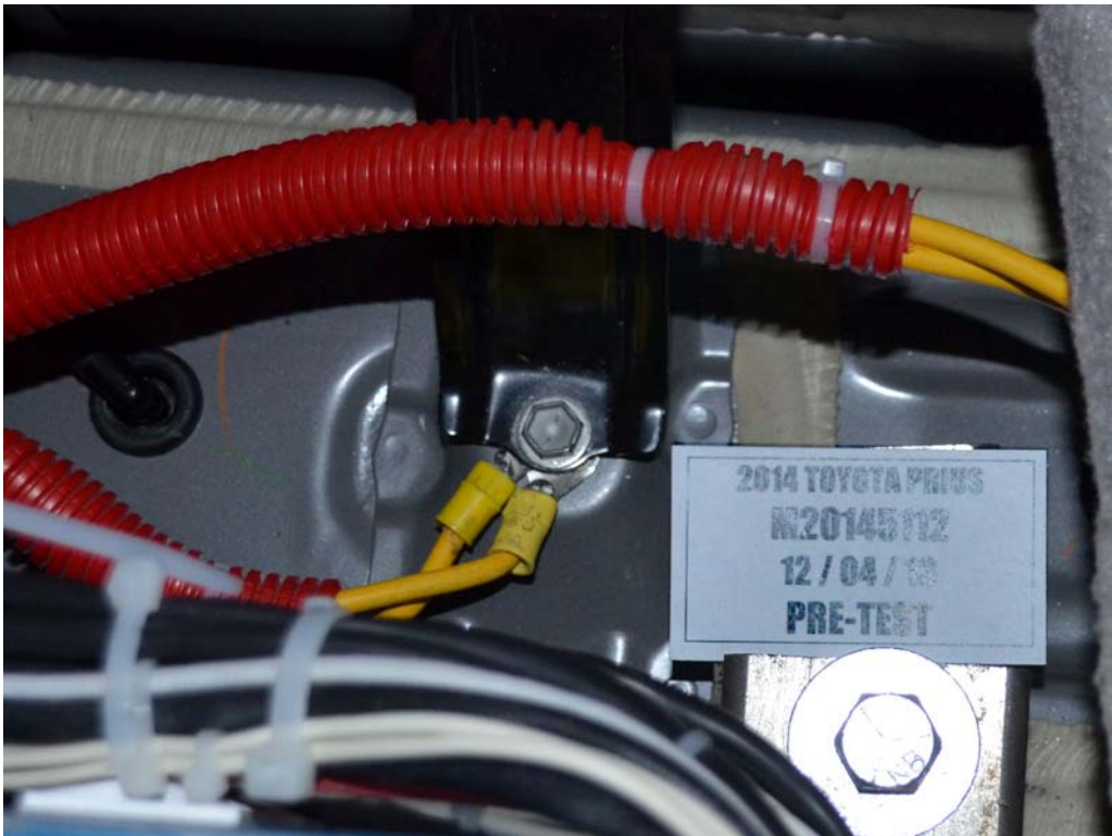
FIGURE 21. Pre-Impact View of Ground Lead Attached
