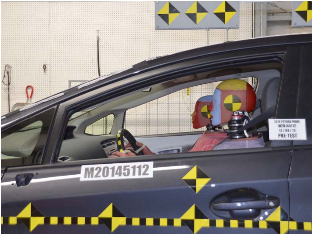
FIGURE 31. Pre-Test Driver Dummy Window View
