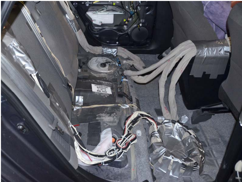
FIGURE 27. Pre-Test Dummy Cable Routing
