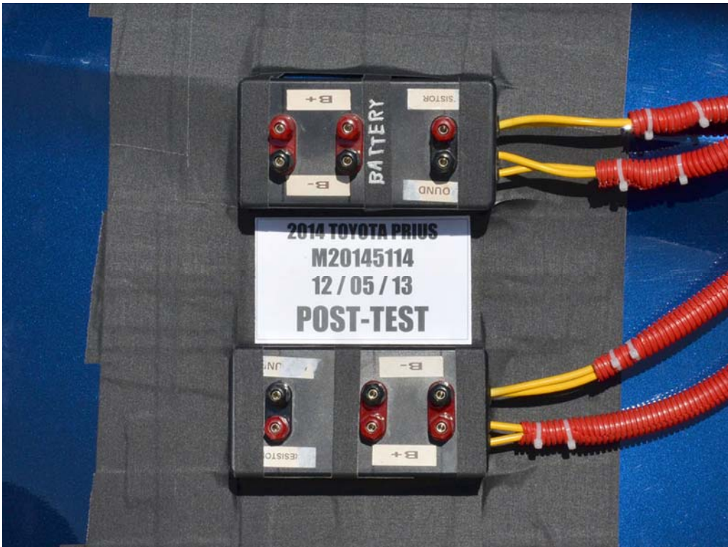
FIGURE 25. Post-Impact View of Installed Test Interface Port
