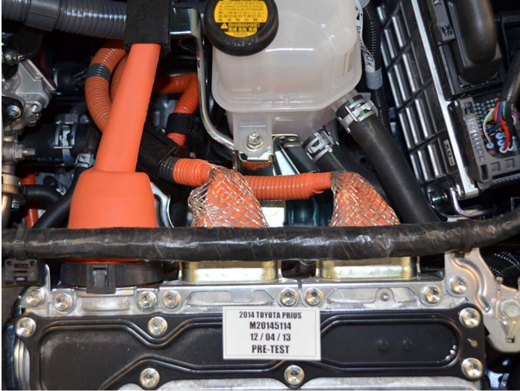
FIGURE 18. Pre-Impact View of High Voltage Interconnects
