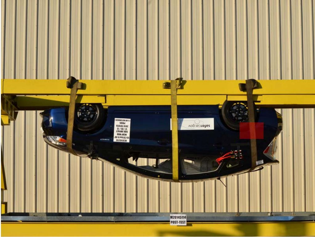
FIGURE 30. FMVSS No. 305 Static Rollover at 180°
