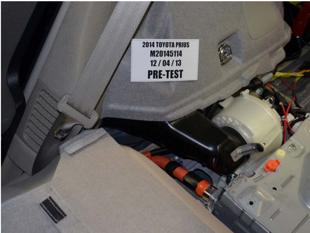
FIGURE 19. Pre-Impact View of Propulsion Battery Venting System
