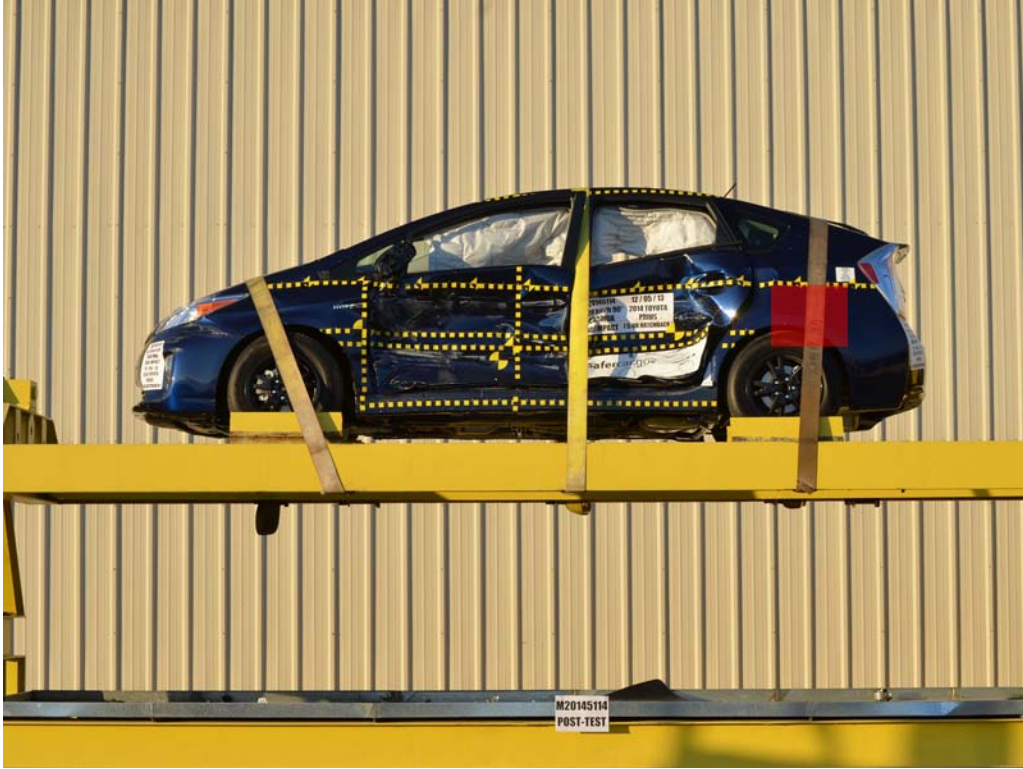
FIGURE 32. FMVSS No. 305 Static Rollover at 360°
