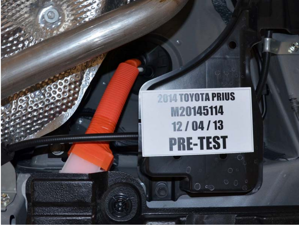
FIGURE 18b. Pre-Impact View of High Voltage Interconnects
