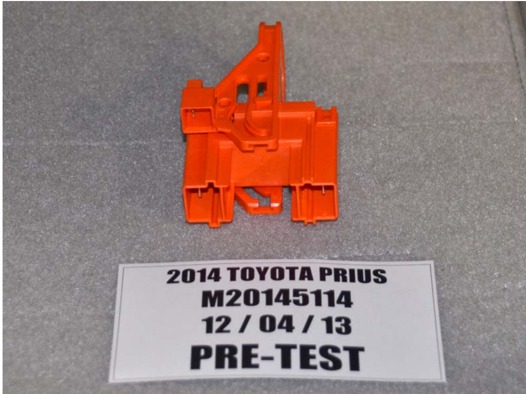
FIGURE 7. Manual High Voltage Service Disconnect Removed
