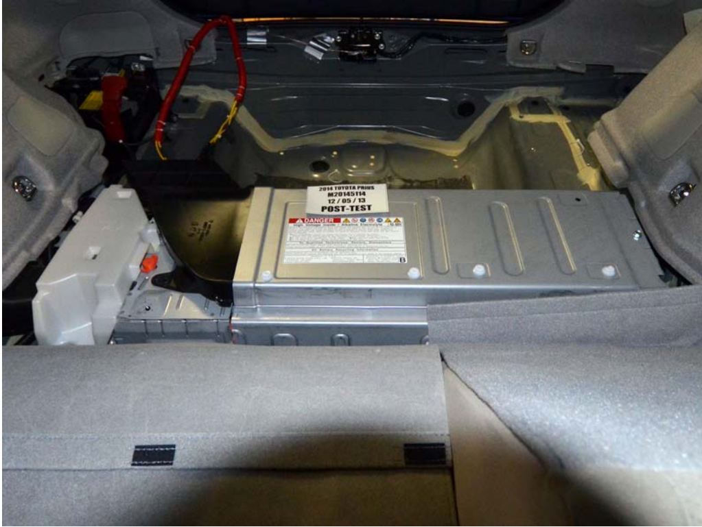
FIGURE 10. Post-Impact Front View of Propulsion Battery
