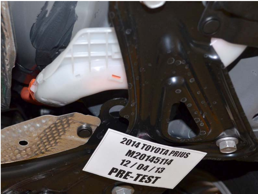
FIGURE 18a. Pre-Impact View of High Voltage Interconnects
