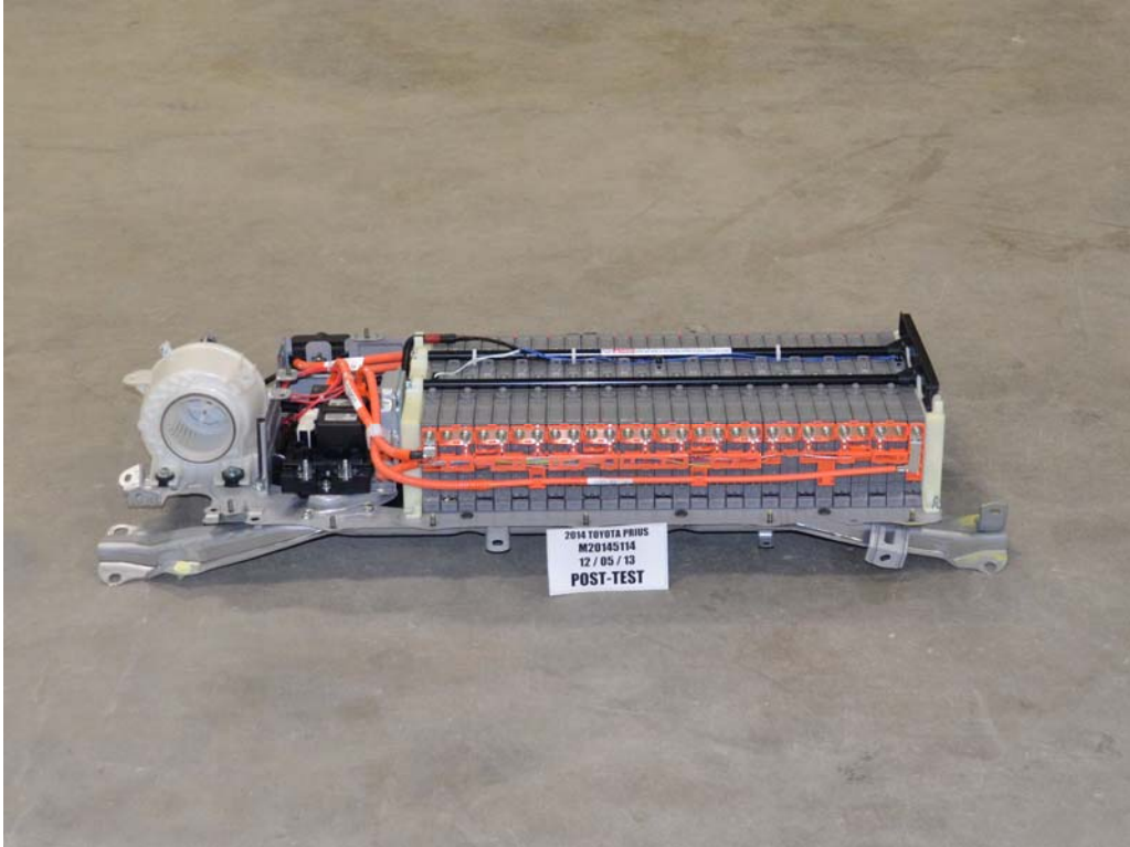
FIGURE 15a. Post-Impact View of Propulsion Battery Modules
