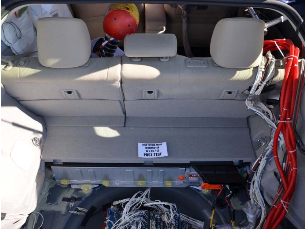
FIGURE 34a. Post-Impact View of the Vehicle Passenger Compartment Adjacent to Propulsion Battery
