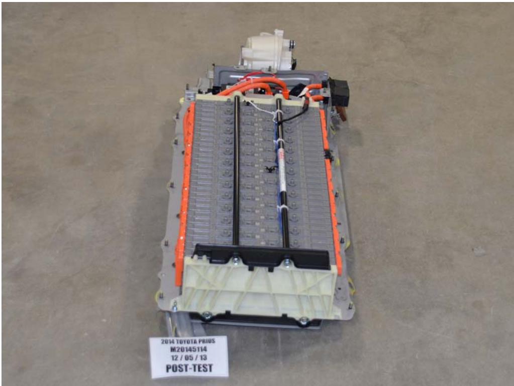
FIGURE 15d. Post-Impact View of Propulsion Battery Modules
