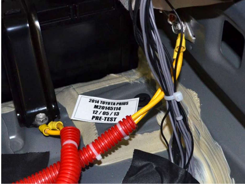
FIGURE 21. Pre-Impact View of Ground Lead Attached
