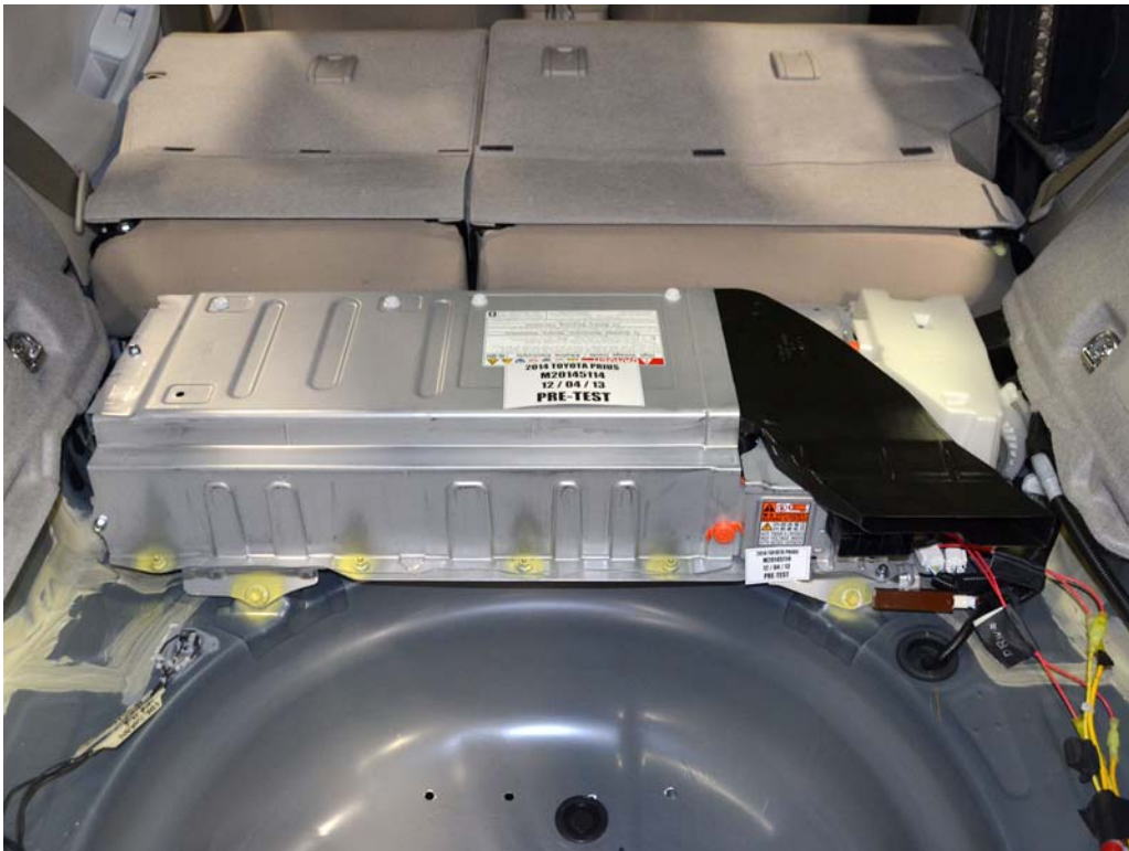
FIGURE 9a. Pre-Impact View of Propulsion Battery
