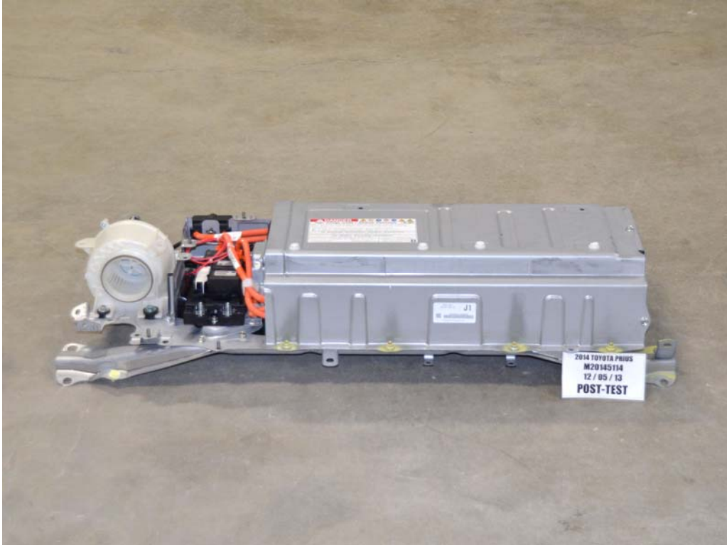
FIGURE 13a. Post-Impact View of Battery Box or Container which Holds Individual Battery Modules
