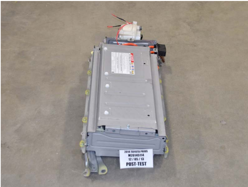
FIGURE 13b. Post-Impact View of Battery Box or Container which Holds Individual Battery Modules
