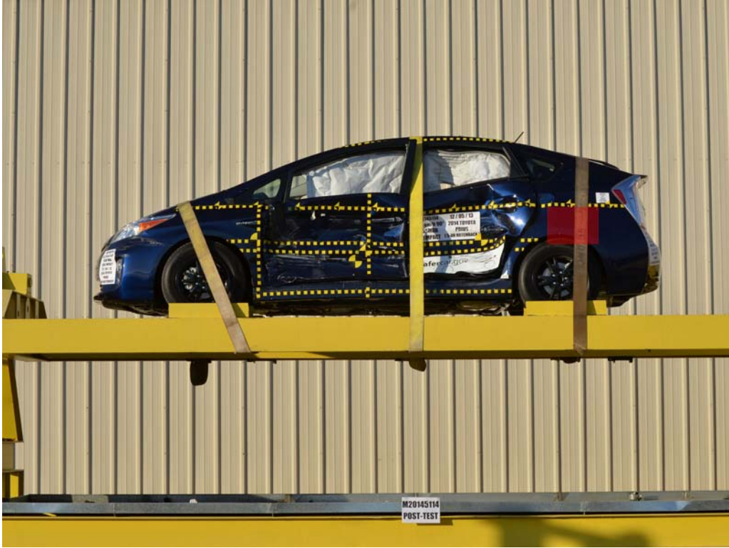
FIGURE 28. FMVSS No. 305 Static Rollover at 0°
