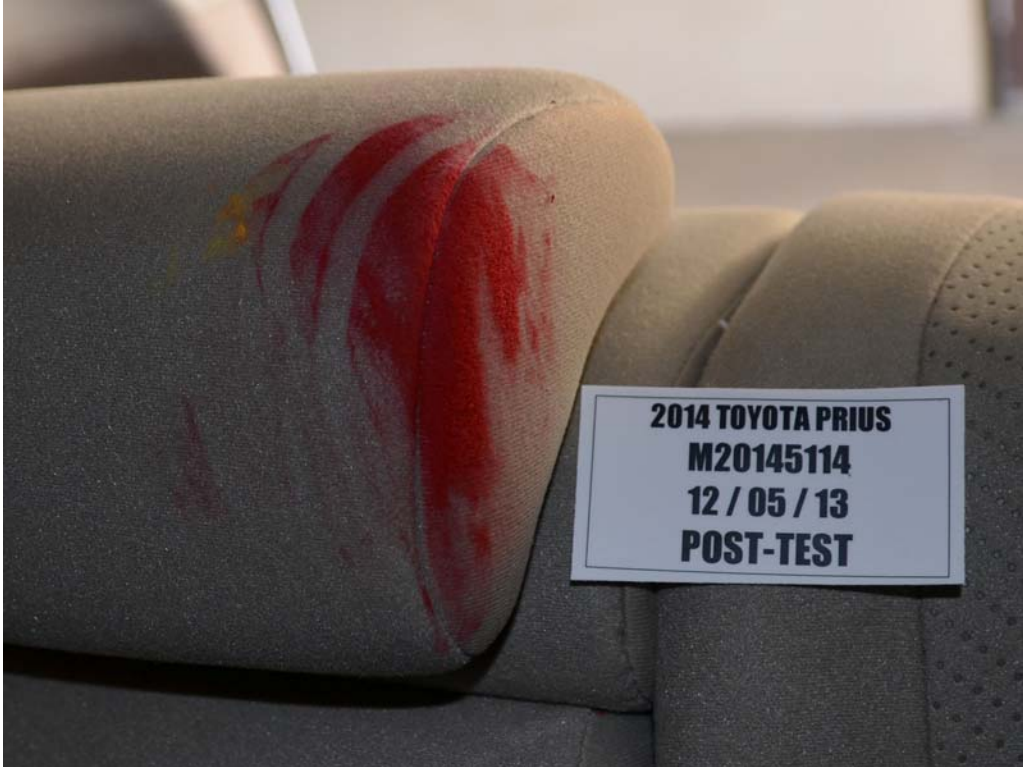
FIGURE 75. Post-Test Rear Passenger Dummy Close-Up Head Contact with Vehicle View
