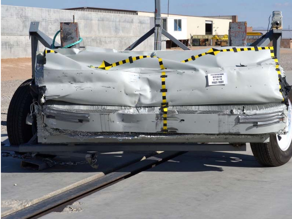
FIGURE 85. Post-Test Front View of MDB Impactor Face
