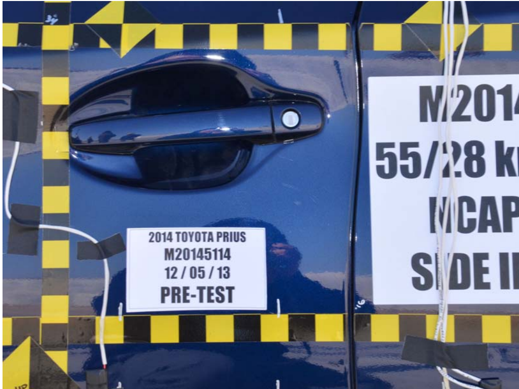
FIGURE 21. Pre-Test Left Front Door Latch Close-Up
