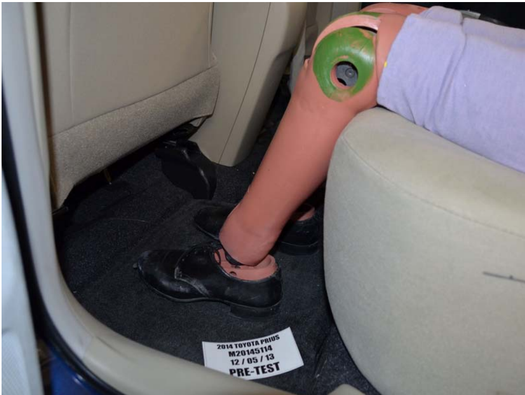
FIGURE 64. Pre-Test Placement of Rear Passenger Dummy's Feet
