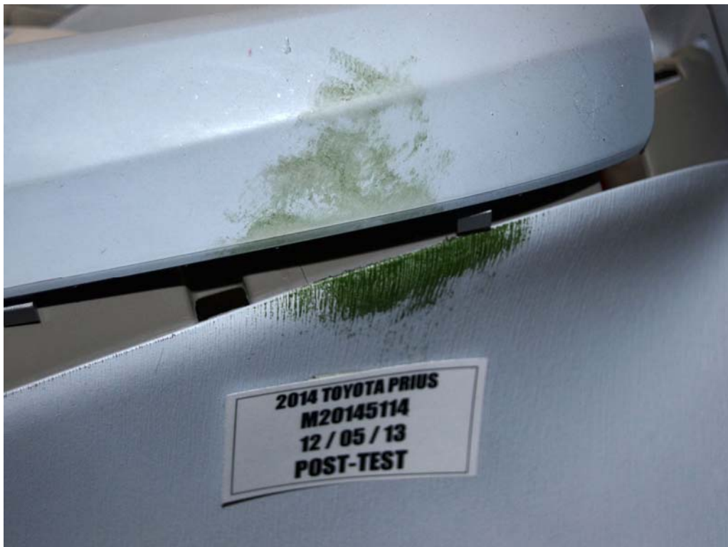
FIGURE 54. Post-Test Driver Dummy Close-Up Knee Contact View
