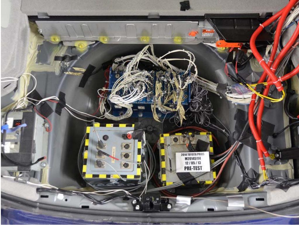
FIGURE 94. Pre-Test Ballast View
