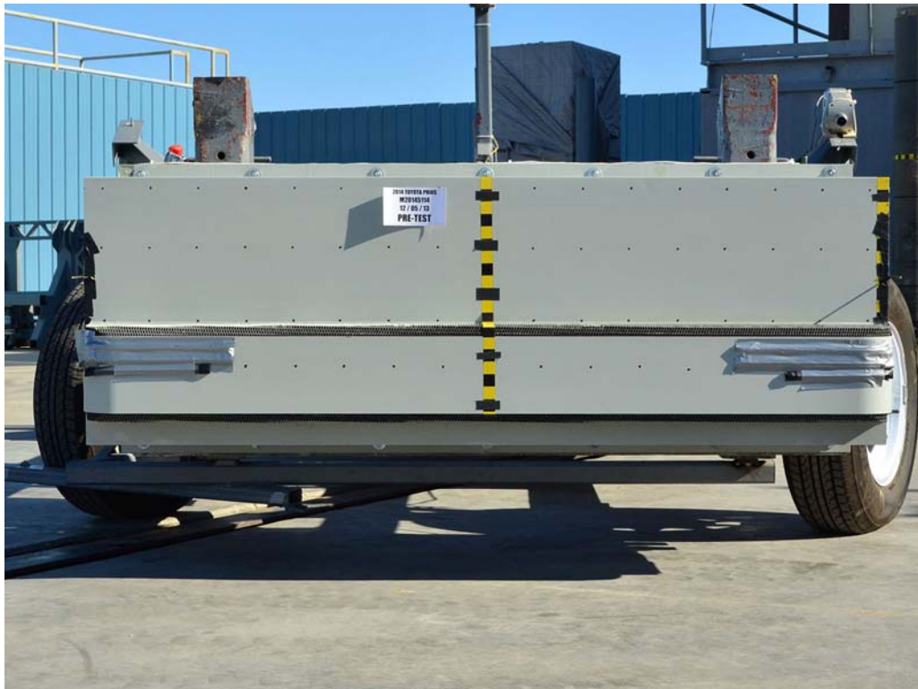
FIGURE 84. Pre-Test Front View of MDB Impactor Face
