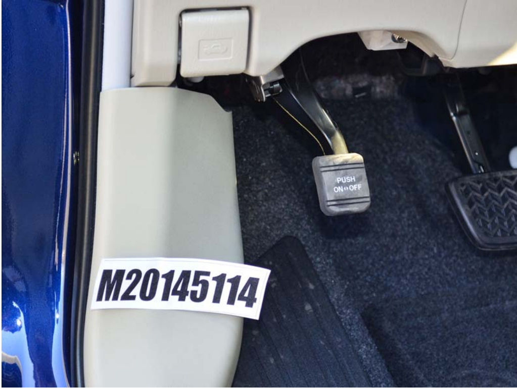
FIGURE 37. View of Disengaged Parking Brake
