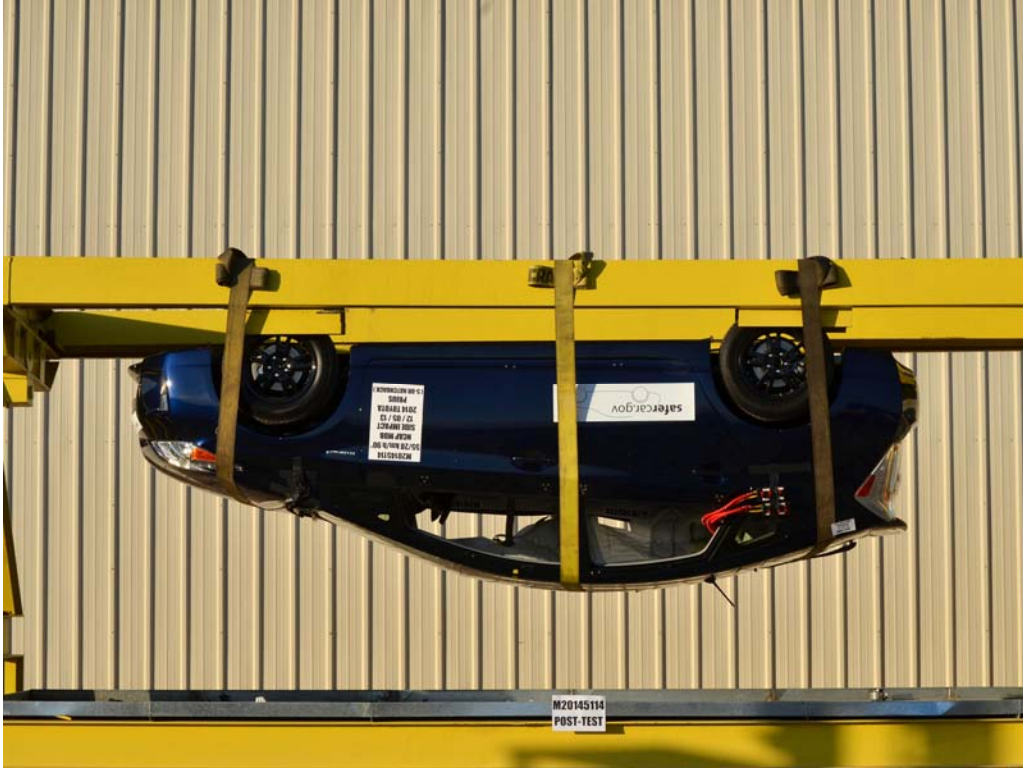
FIGURE 98. FMVSS No. 301 Static Rollover 180 Degrees
