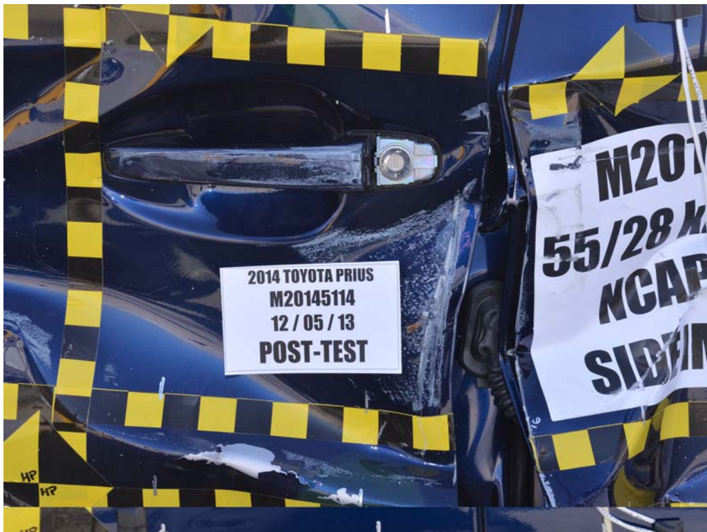
FIGURE 22. Post-Test Left Front Door Latch Close-Up
