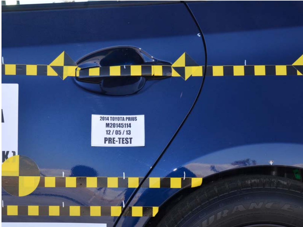
FIGURE 23. Pre-Test Left Rear Door Latch Close-Up
