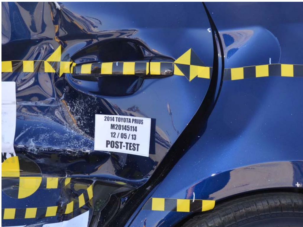
FIGURE 24. Post-Test Left Rear Door Latch Close-Up
