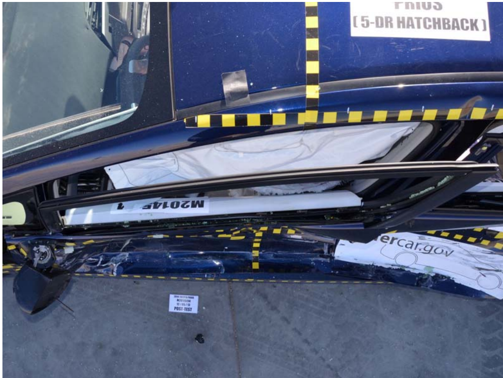
FIGURE 43. Post-Test Driver Dummy and Door Clearance View
