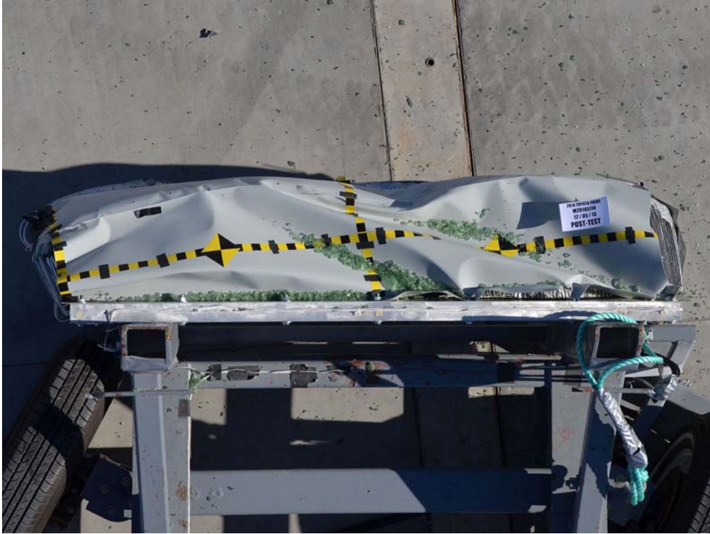
FIGURE 87. Post-Test Top View of MDB Impactor Face
