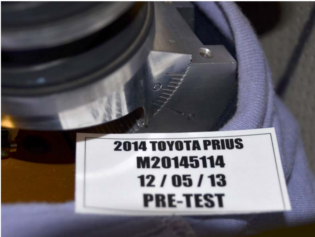
FIGURE 62. Pre-Test View of Rear Passenger Dummy's Neck Showing Position of Adjustable Neck Bracket
