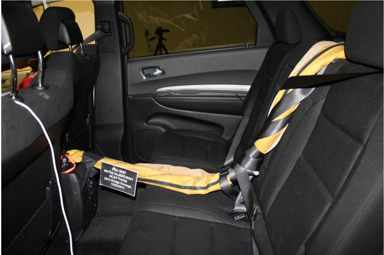
Figure A-27: Pre-Test Dummy Cable Routing
