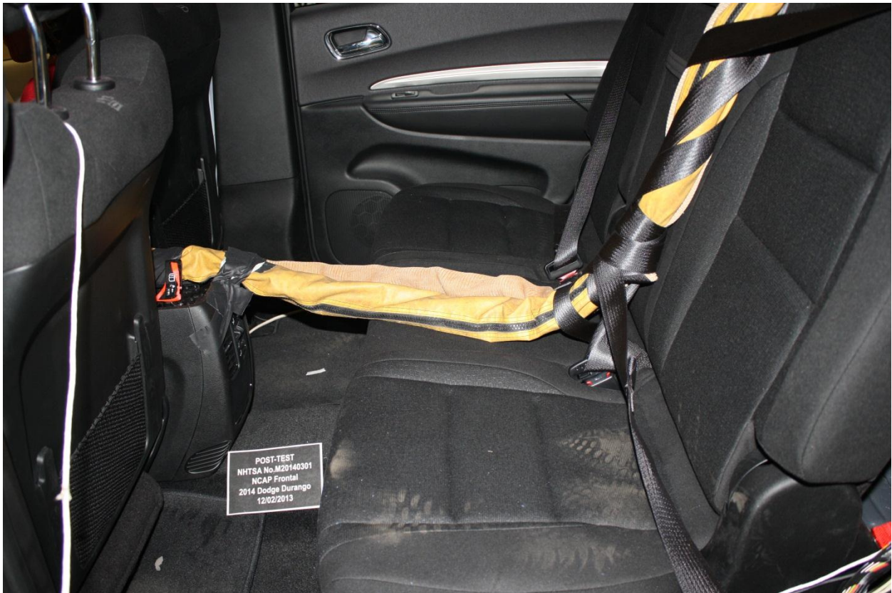
Figure A-28: Post-Test Dummy Cable Routing
