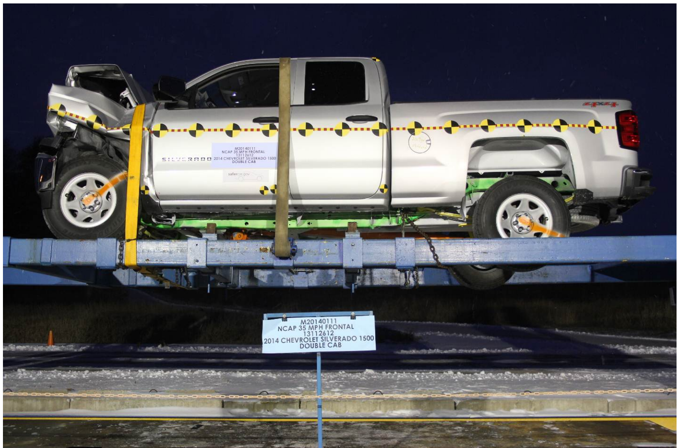
Vehicle at 0 Degree on Static Rollover Device
