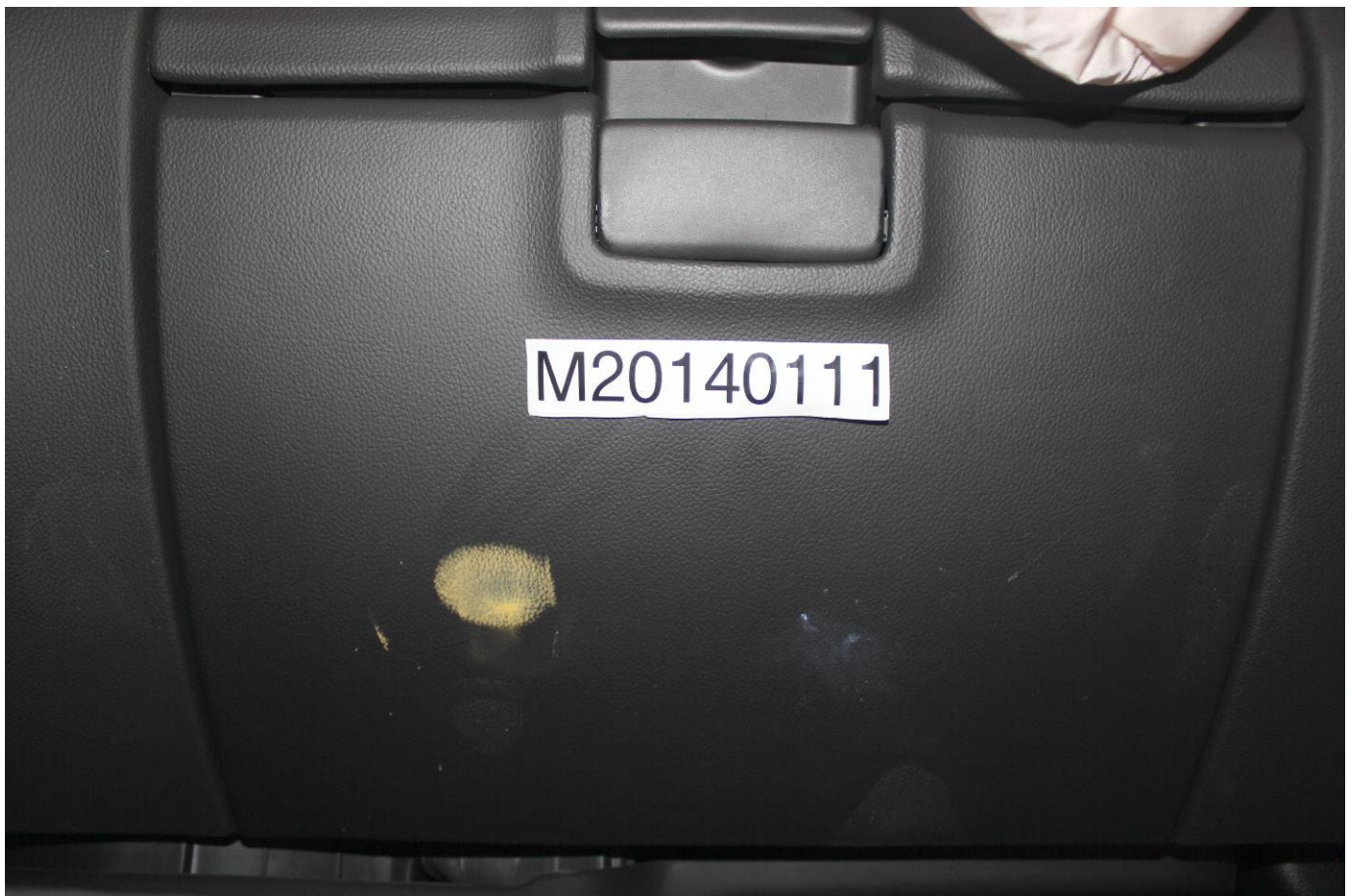
Post-Test Passenger Dummy Contact with Glovebox
