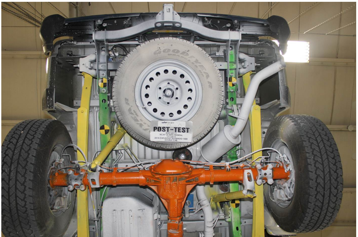
Post-Test Rear Underbody View
