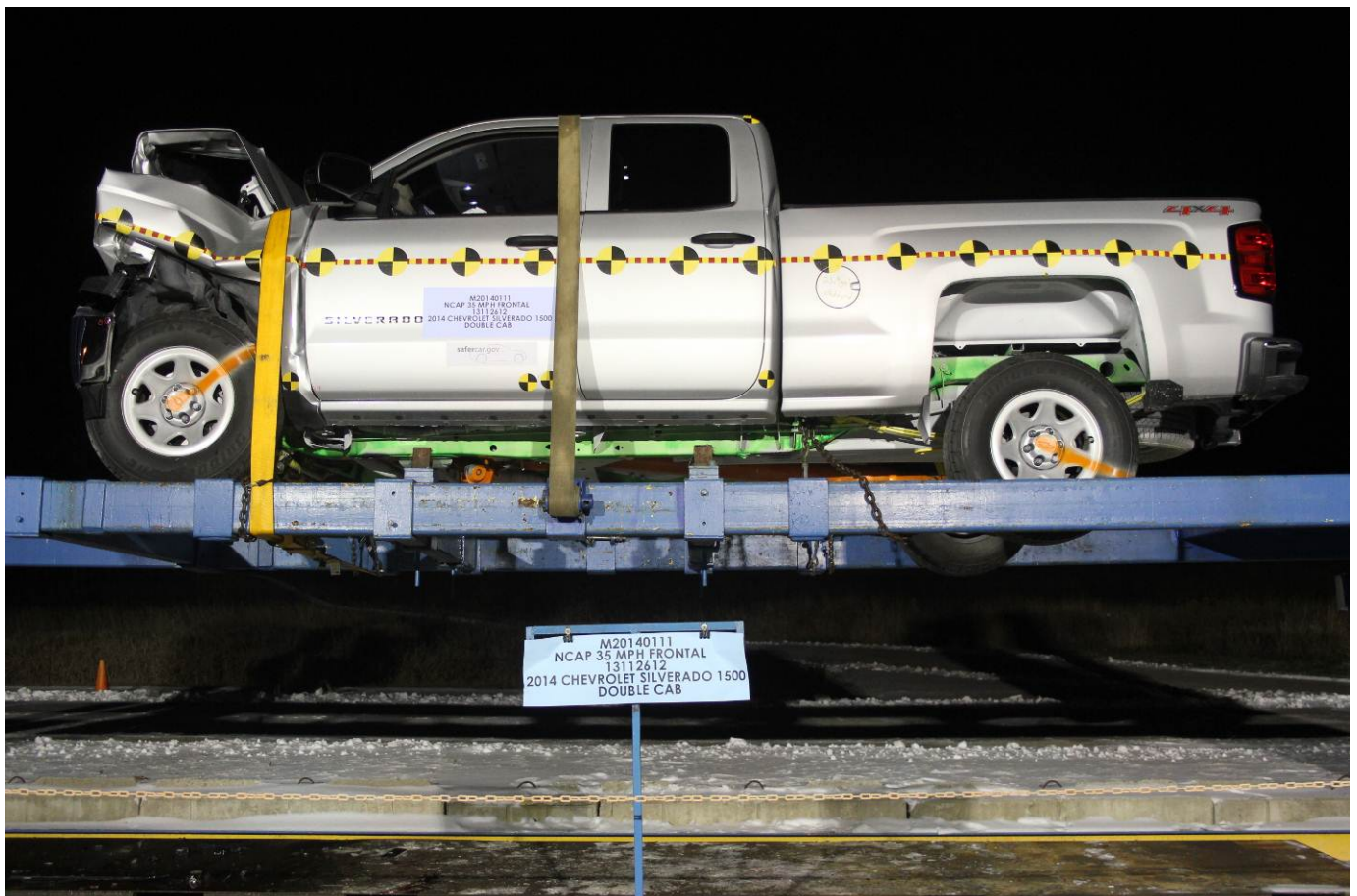
Vehicle at 360 Degrees on Static Rollover Device
