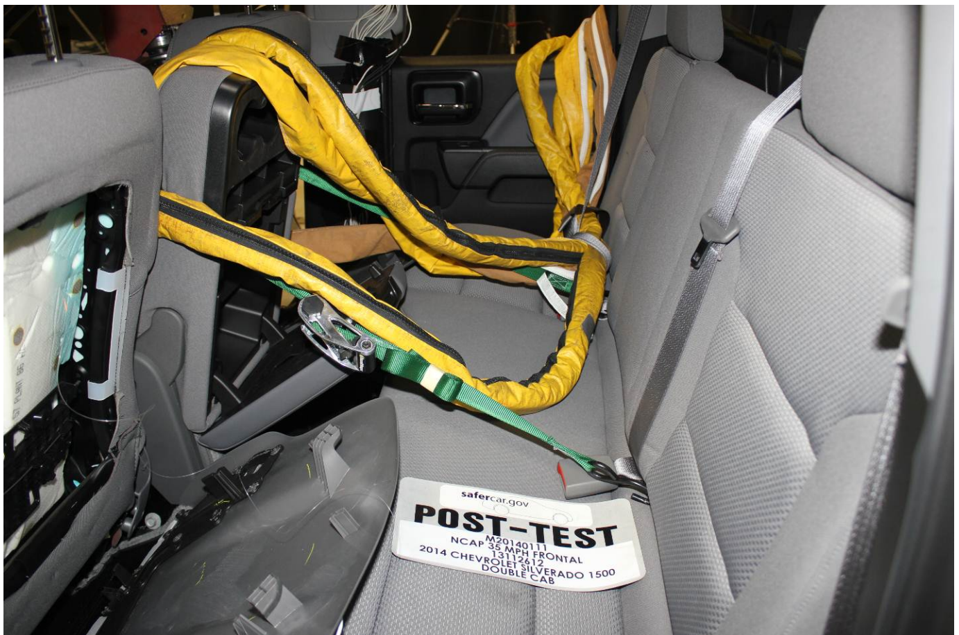
Post-Test Dummy Cable Routing
