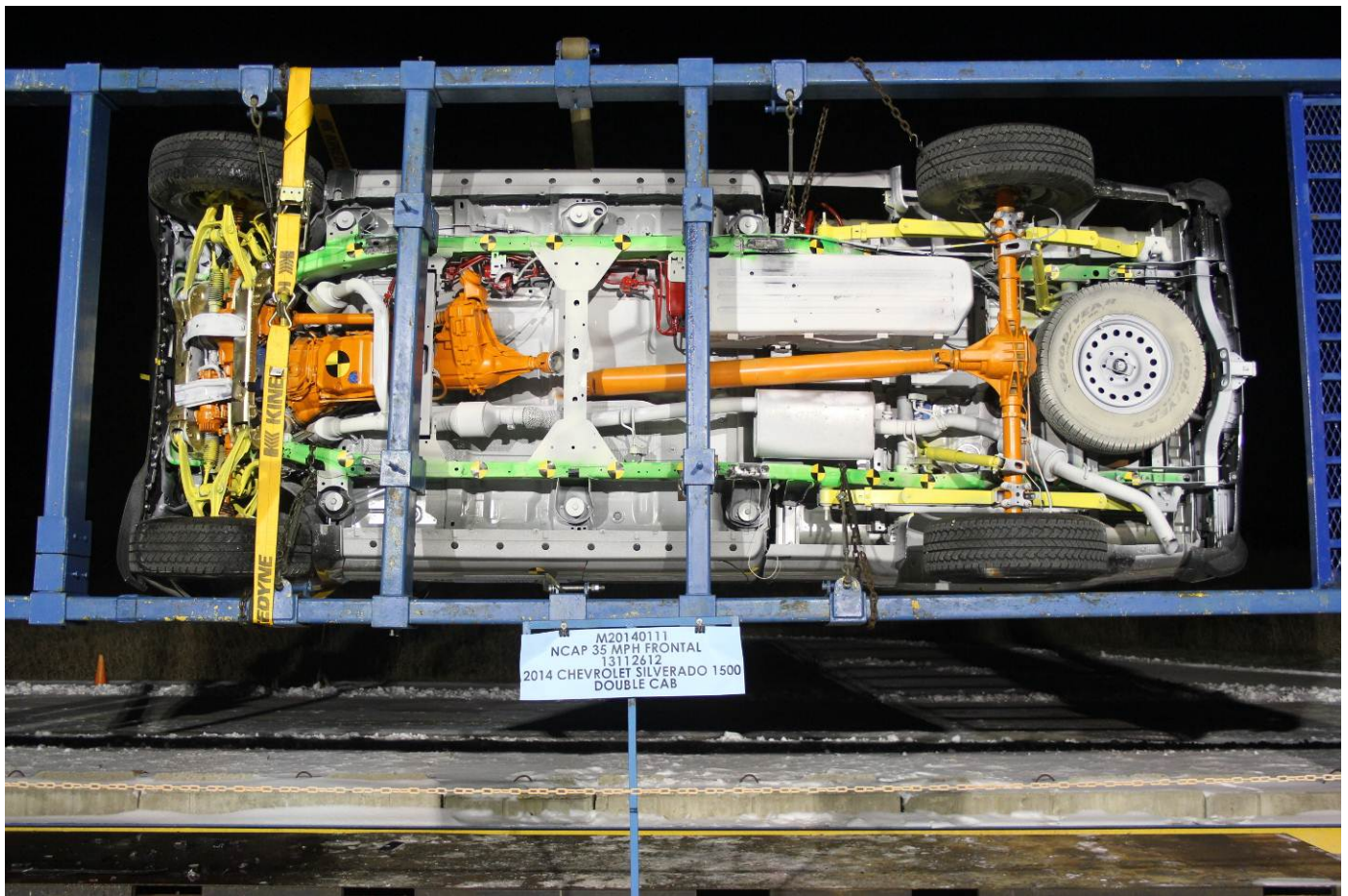
Vehicle at 270 Degrees on Static Rollover Device
