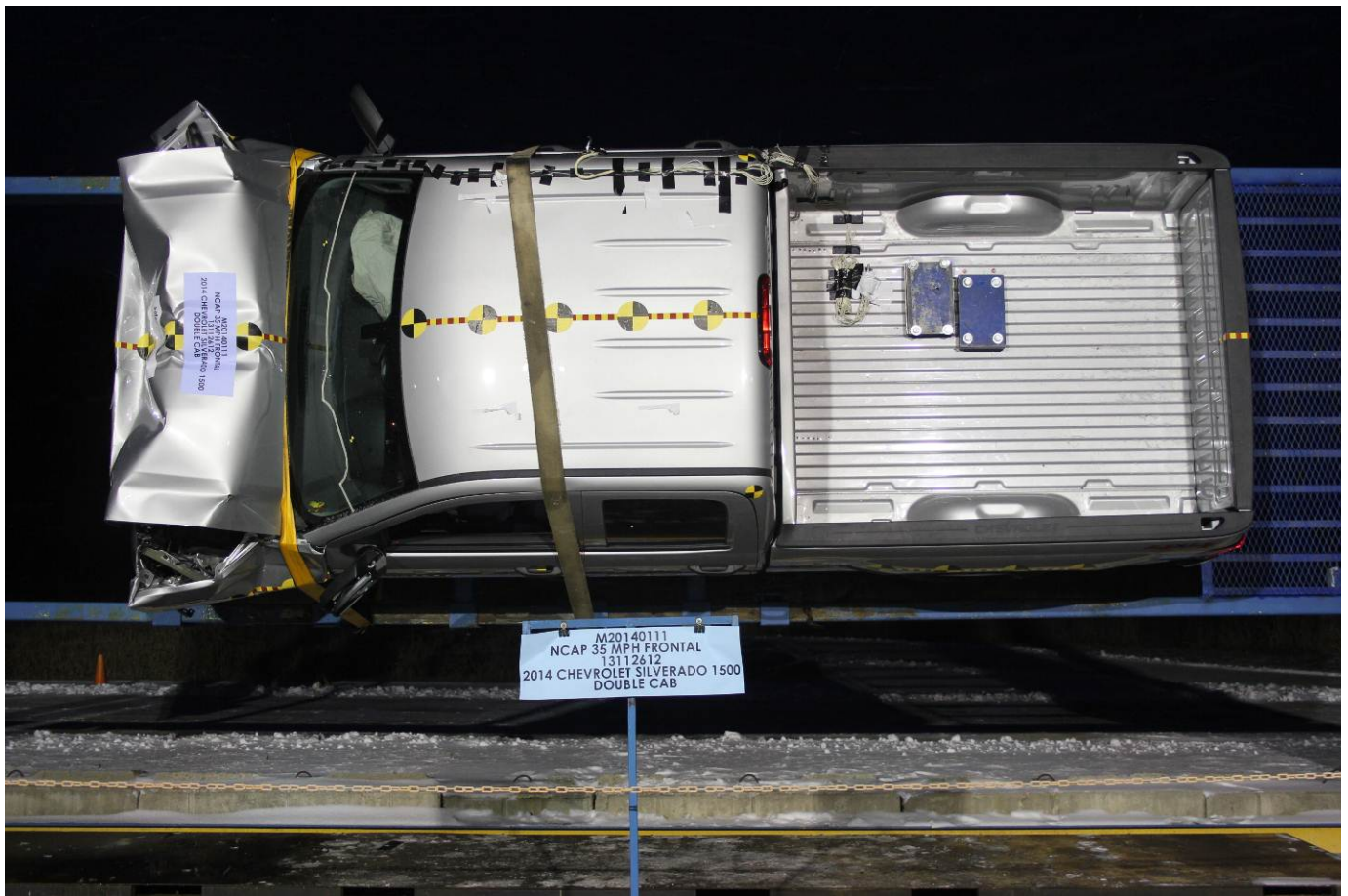
Vehicle at 90 Degrees on Static Rollover Device
