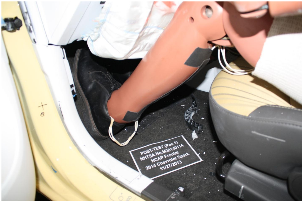
Figure A-40: Post-Test Driver Dummy Feet
