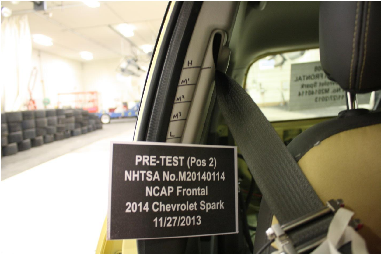
Figure A-59: Post-Test View of Belt Anchorage for Passenger Dummy– Wrong Placard was used
