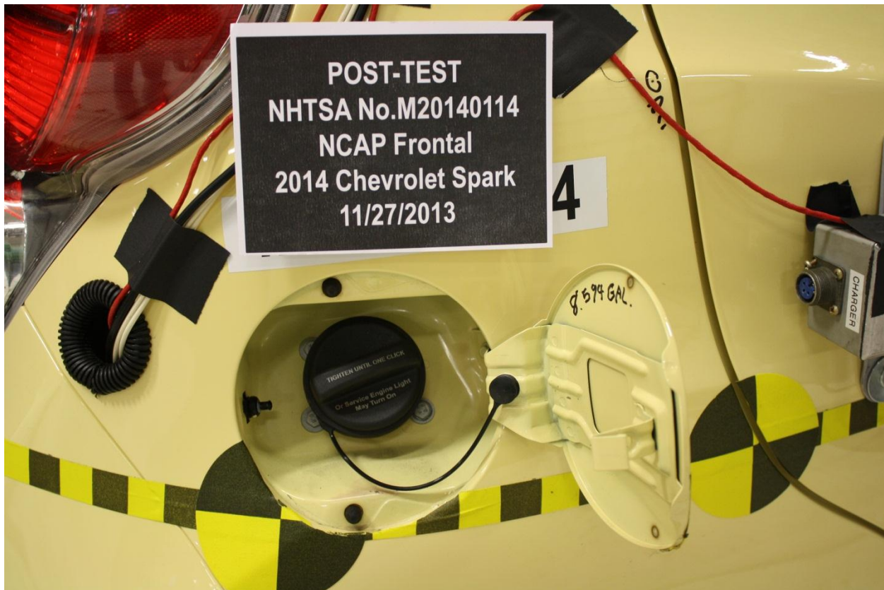
Figure A-22: Post-Test Fuel Filler Cap View
