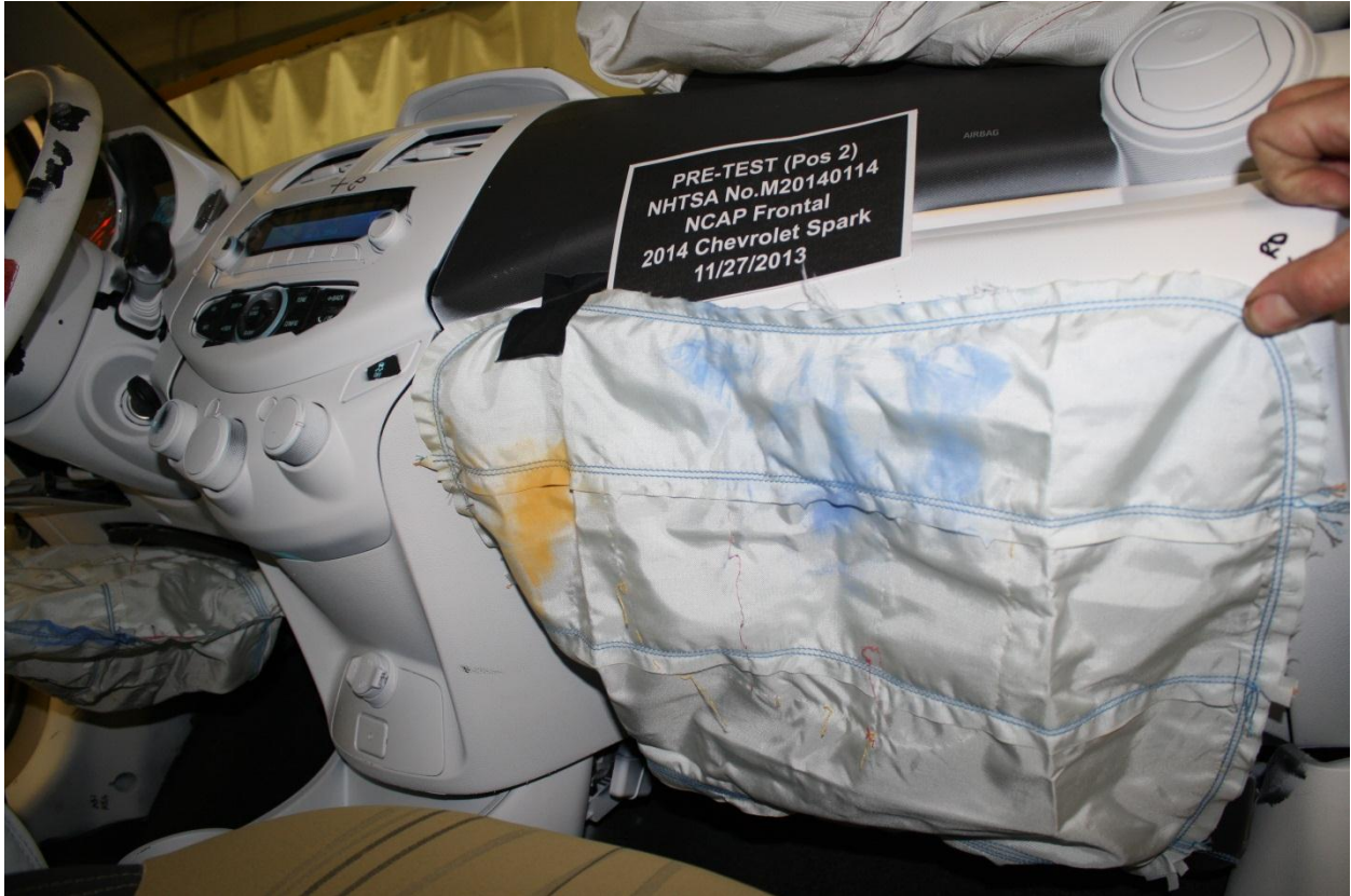
Figure A-63: Post-Test Passenger's Side Knee Bolster– Wrong Placard was used
