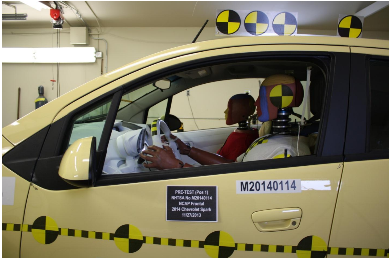
Figure A-31: Pre-Test Driver Dummy Window View
