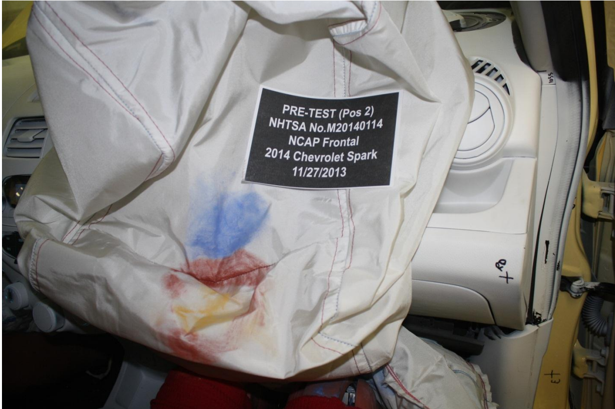
Figure A-67: Post-Test Passenger Dummy Contact With Airbag– Wrong Placard was used
