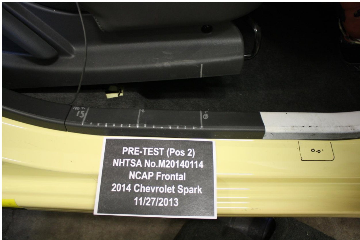
Figure A-56: Pre-Test Passenger's Seat Fore-Aft Markings
