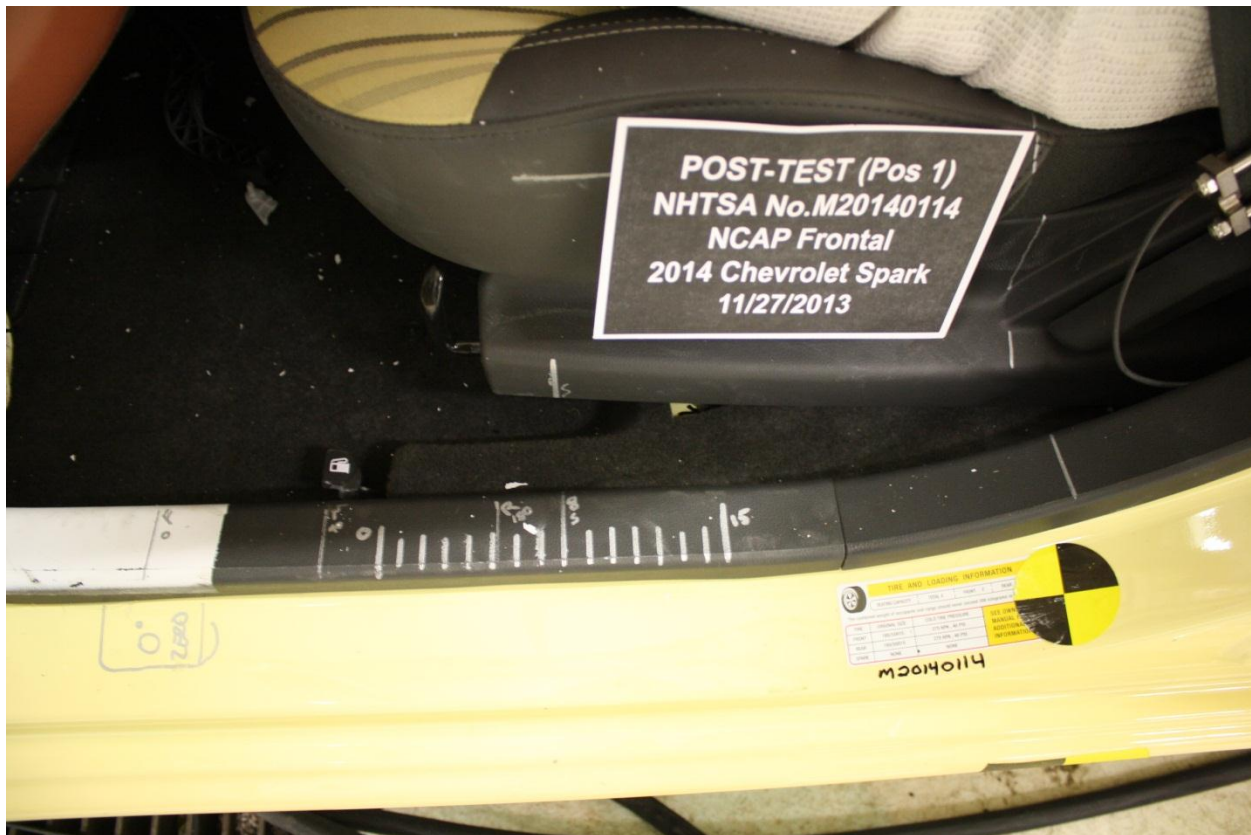
Figure A-36: Post-Test Driver's Seat Fore-Aft Markings
