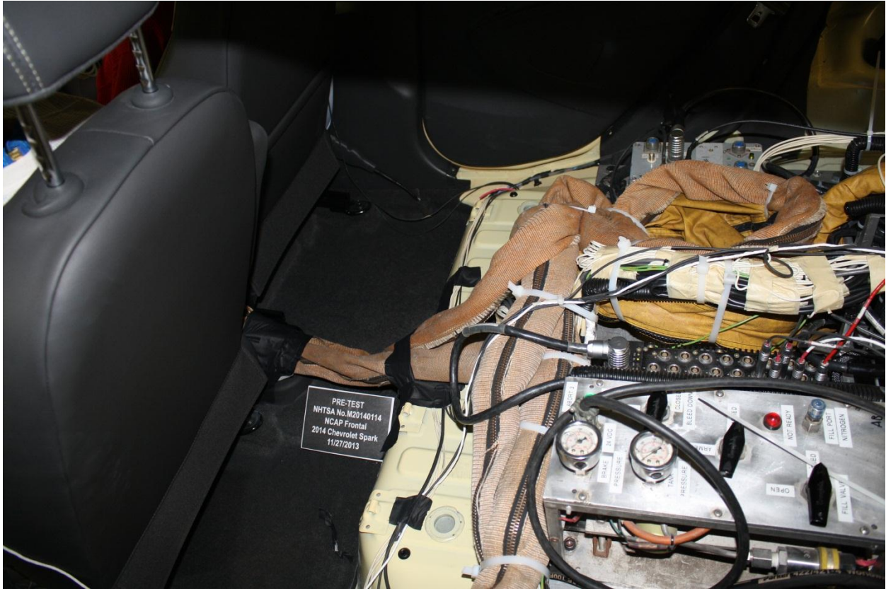
Figure A-27: Pre-Test Dummy Cable Routing
