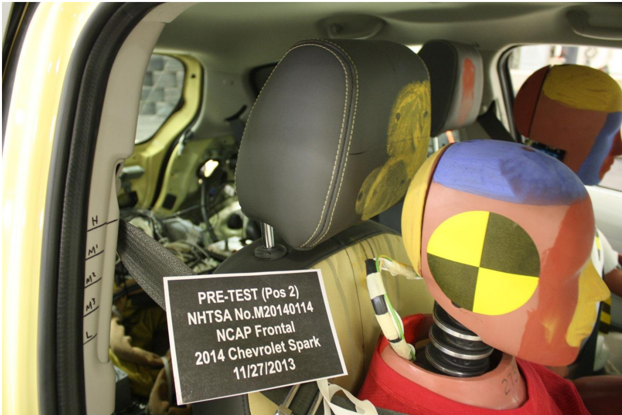
Figure A-68: Post-Test Passenger Dummy Contact With Headrest– Wrong Placard was used
