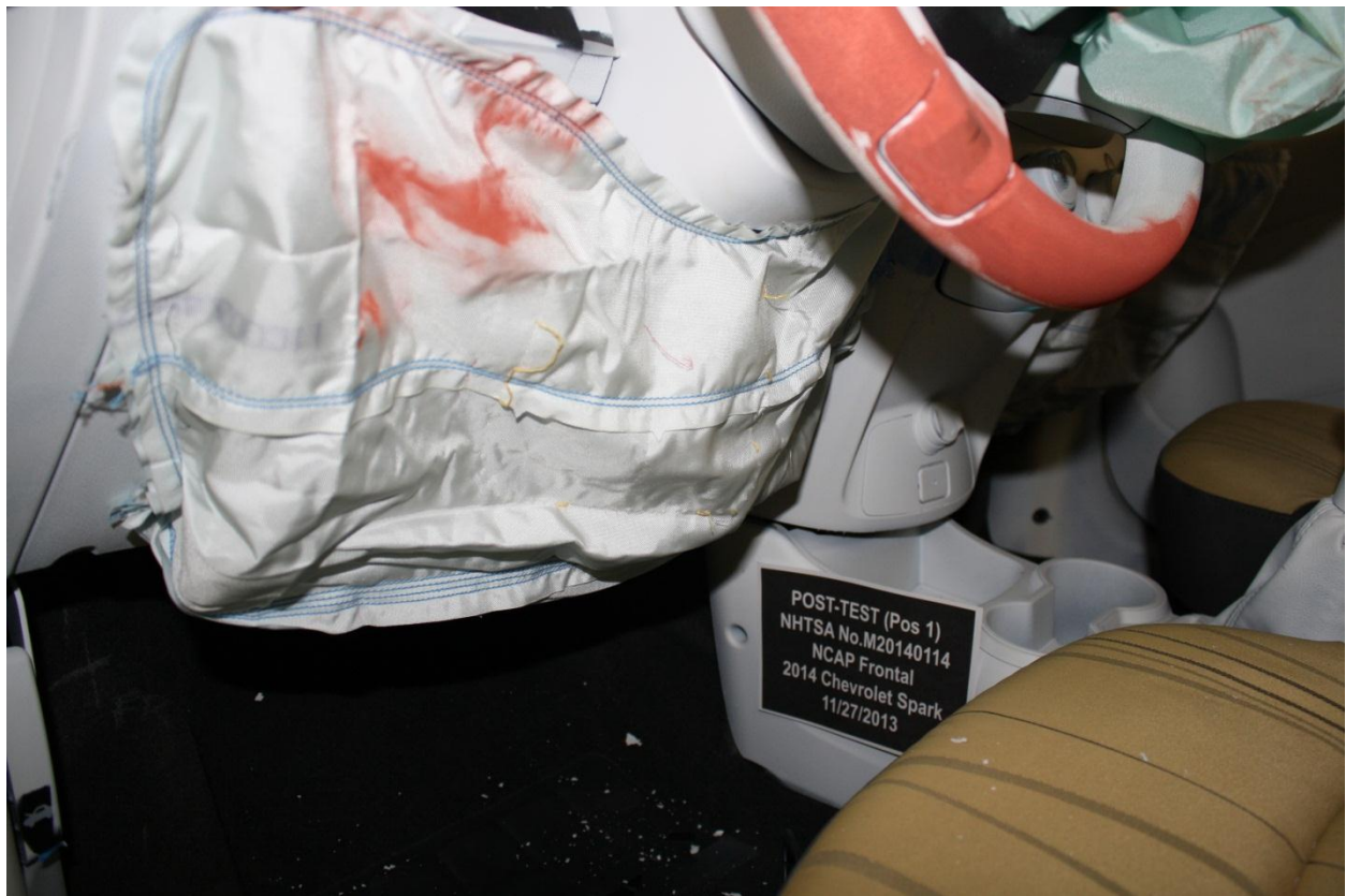
Figure A-42: Post-Test Driver's Side Knee Bolster
