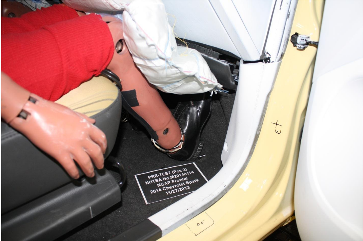
Figure A-61: Post-Test Passenger Dummy Feet– Wrong Placard was used
