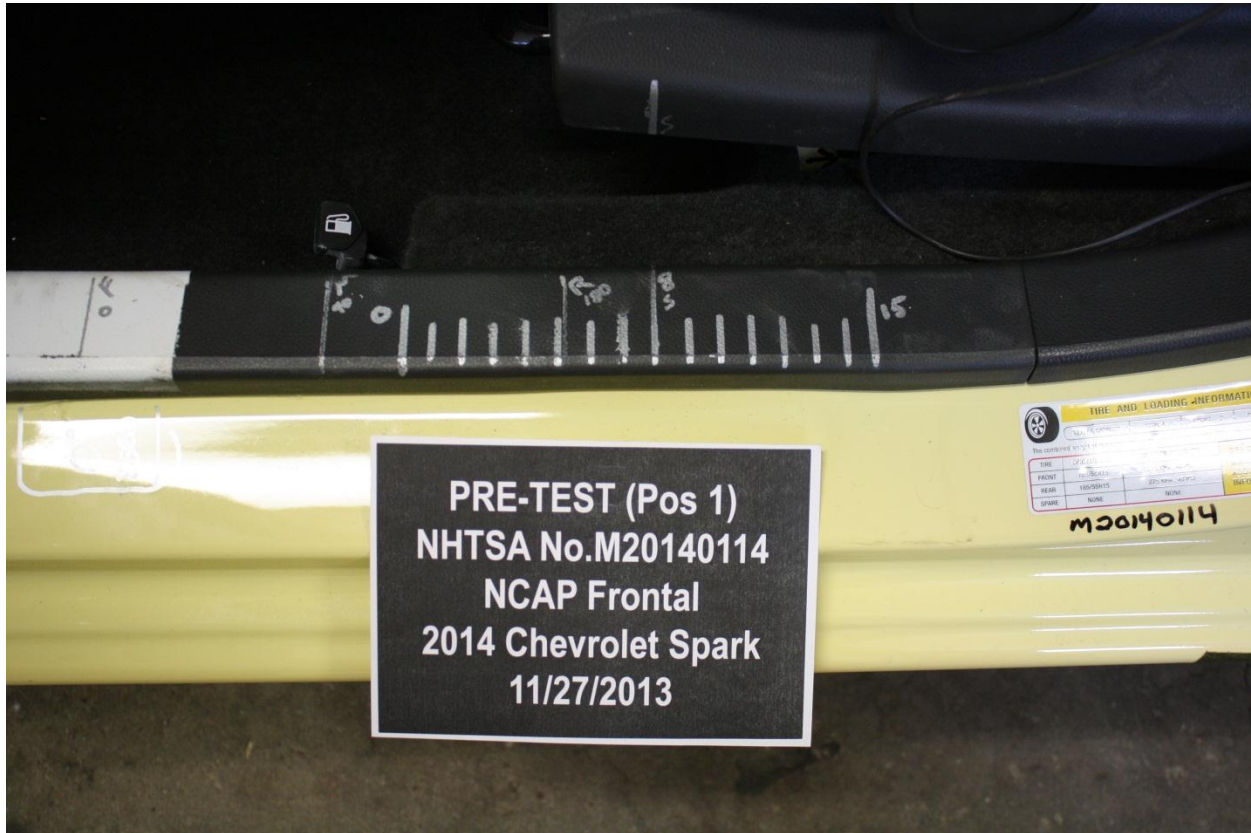
Figure A-35: Pre-Test Driver's Seat Fore-Aft Markings
