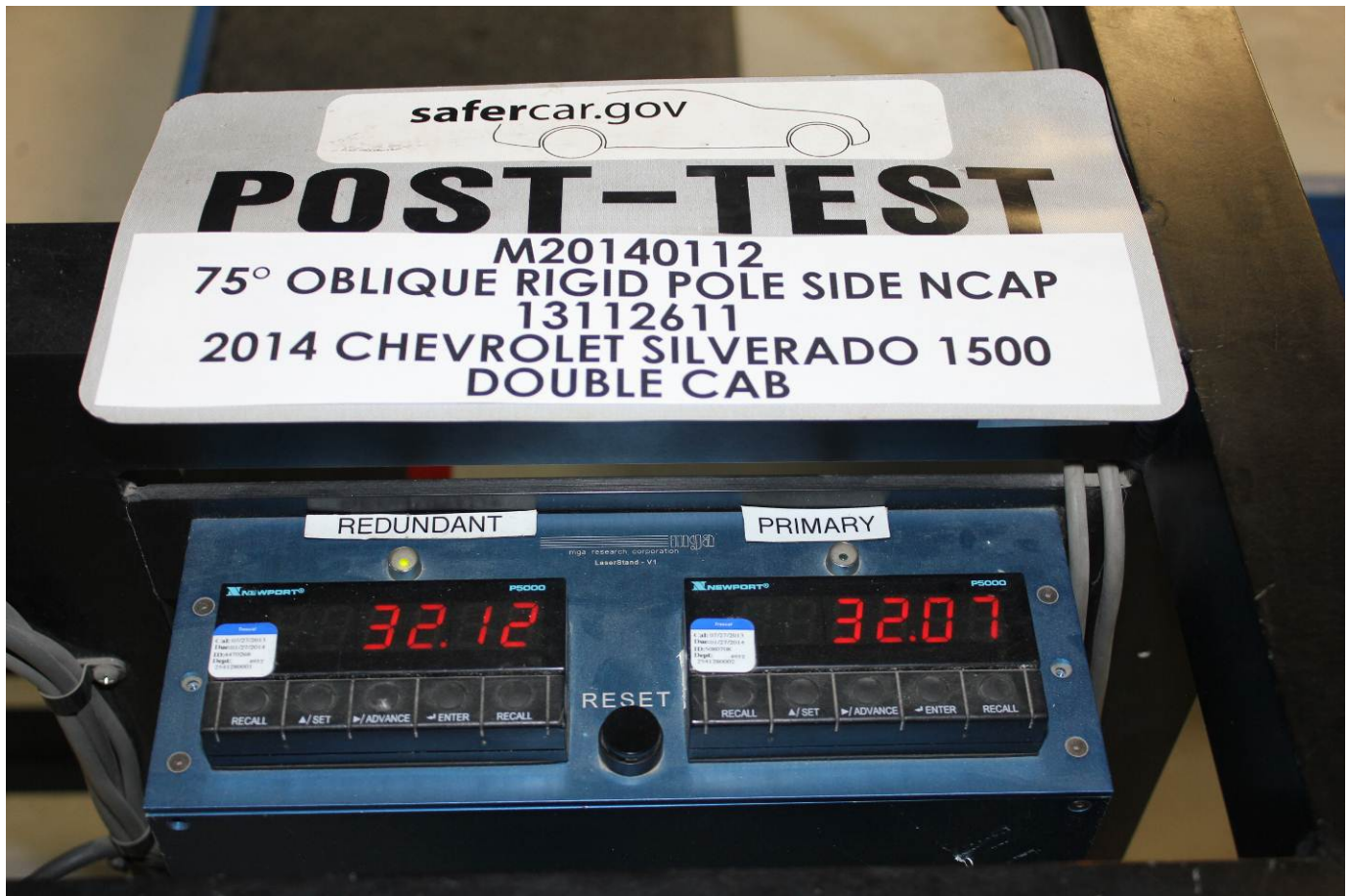
Post-Test Primary and Redundant Speed Trap Read-Out
