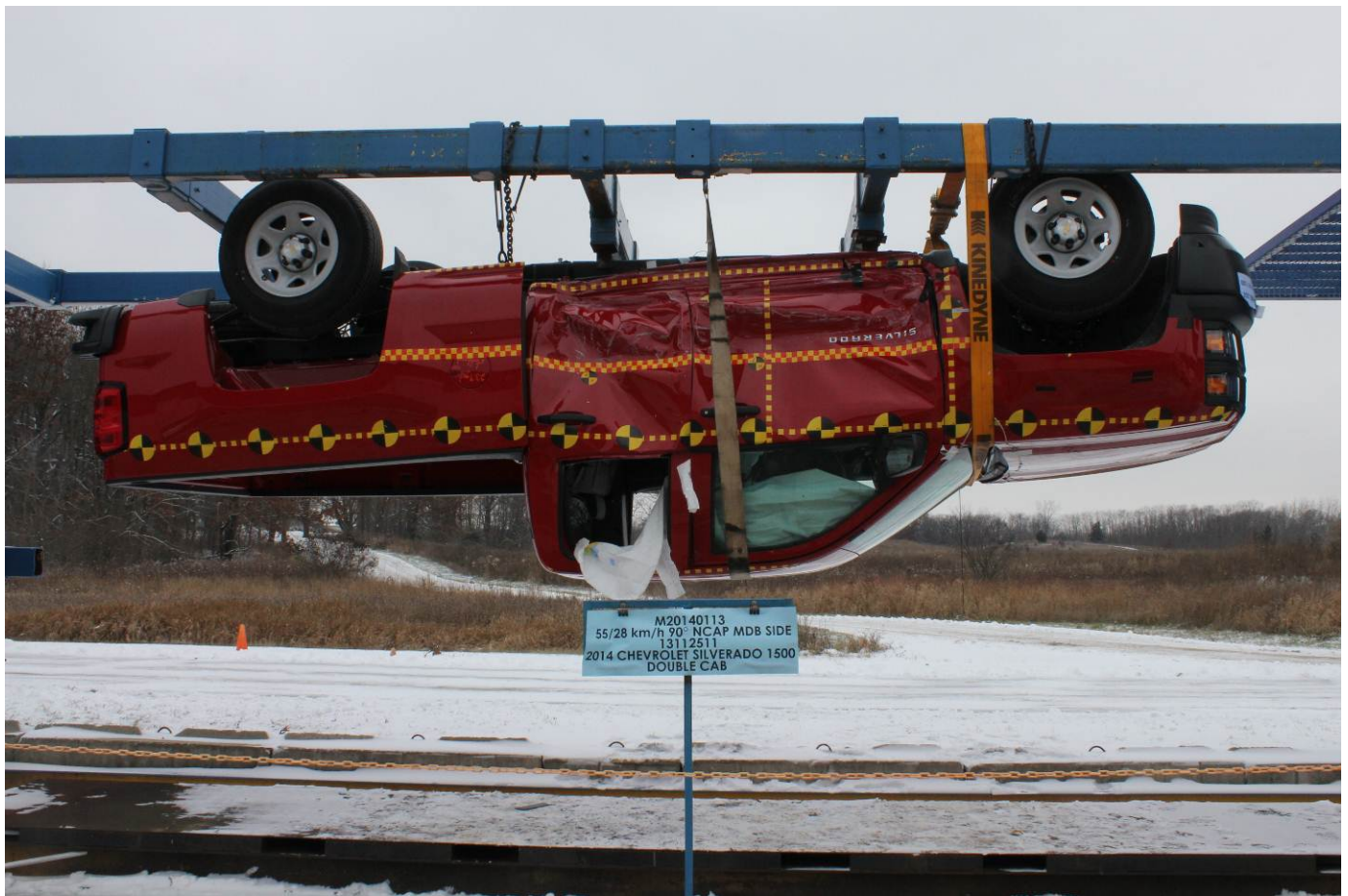
FMVSS No. 301 Static Rollover 180 Degrees
