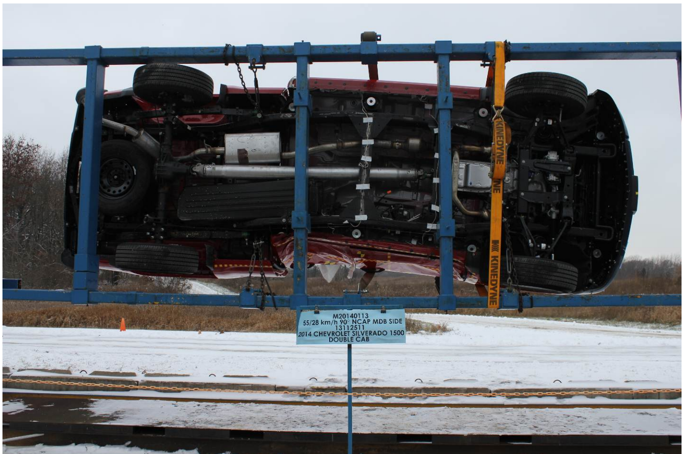
FMVSS No. 301 Static Rollover 90 Degrees
