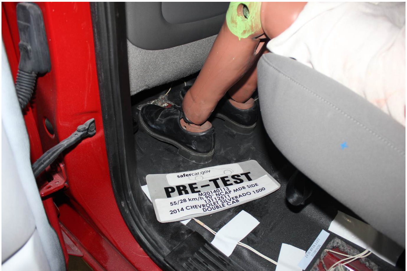
Pre-Test Placement of Rear Passenger Dummy's Feet
