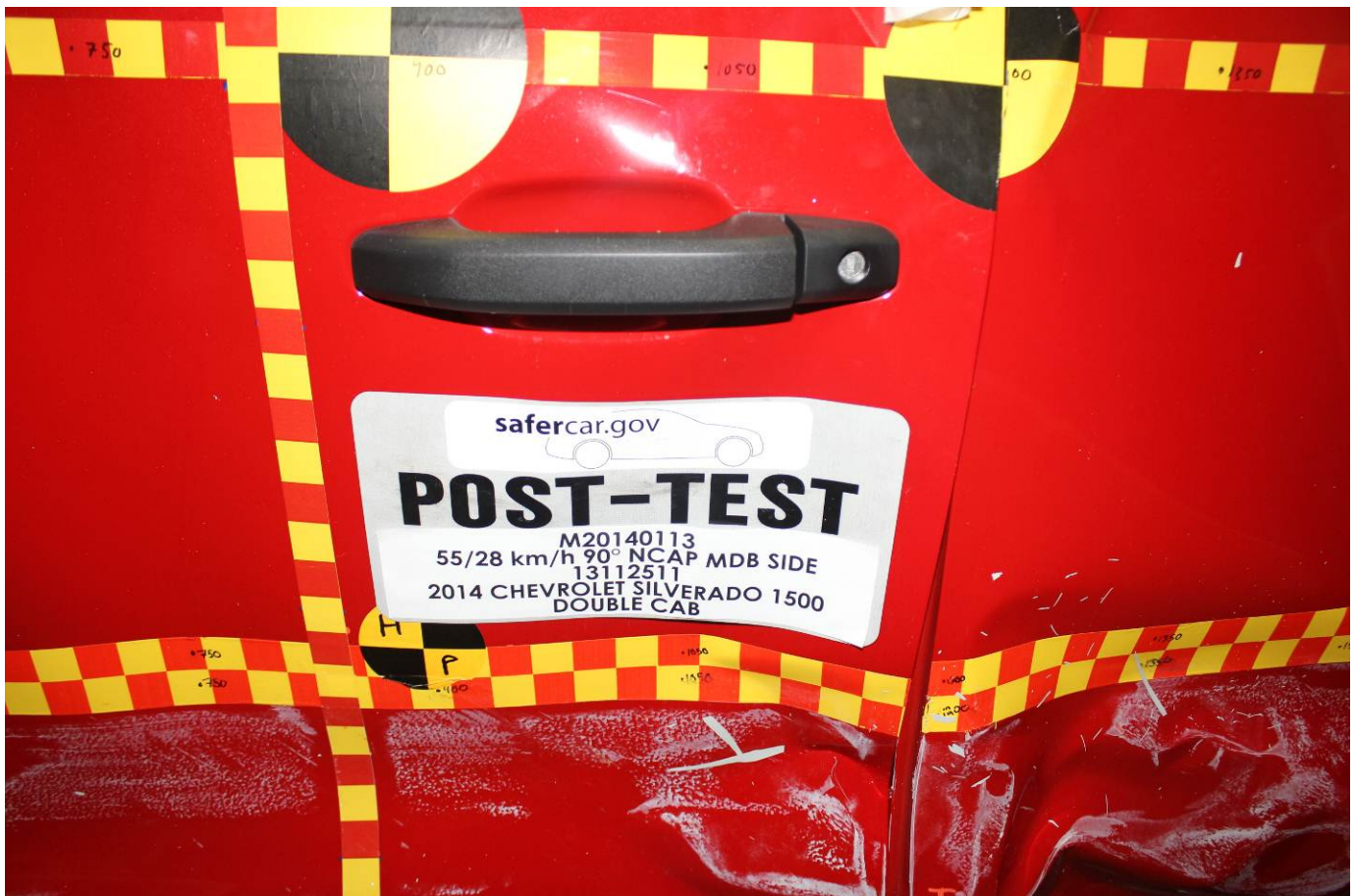
Post-Test Left Front Door Latch Close-Up
