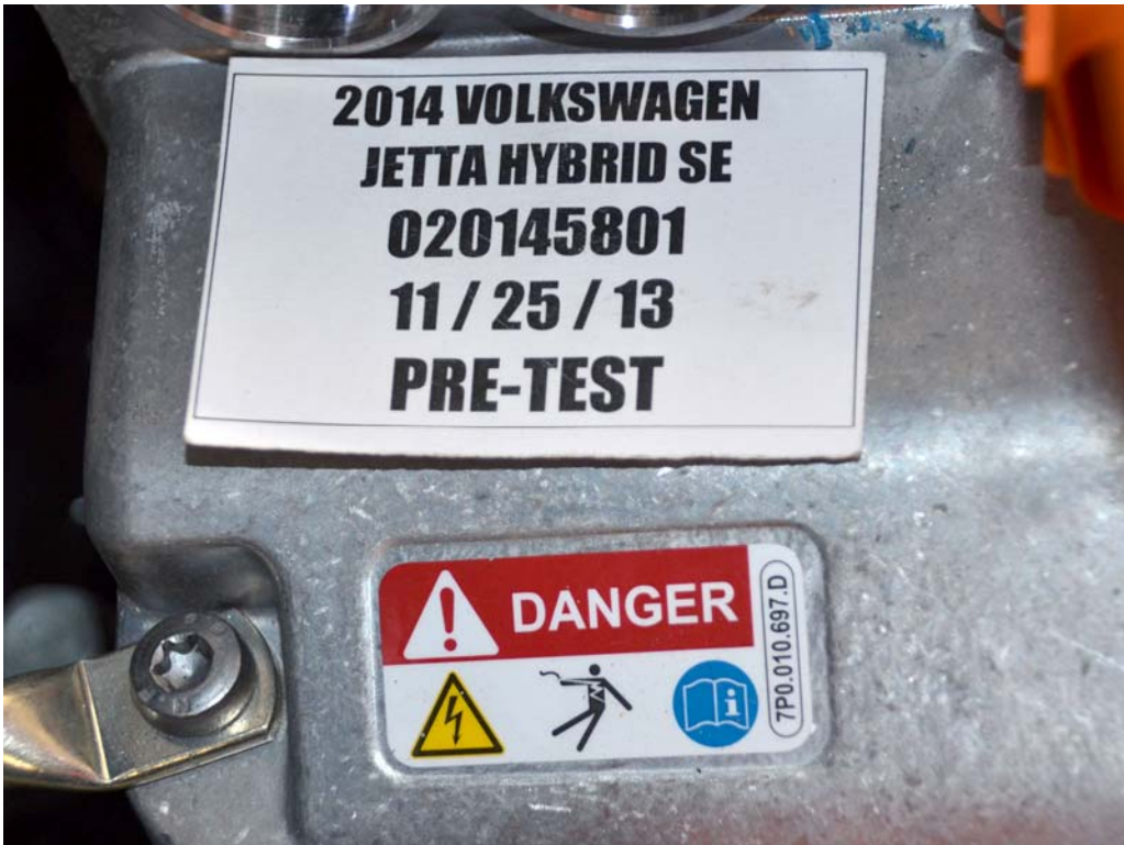
FIGURE 2a. Power Inverter Warning Label
