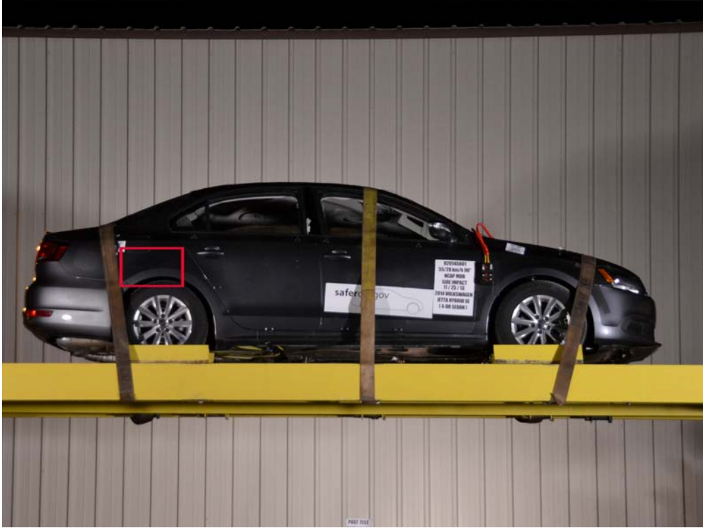
FIGURE 32. FMVSS No. 305 Static Rollover at 360°
