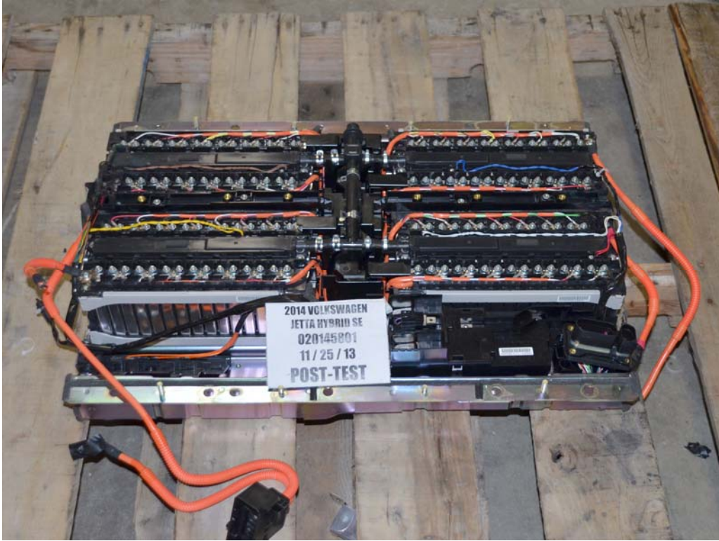
FIGURE 15. Post-Impact View of Propulsion Battery Module(s)
