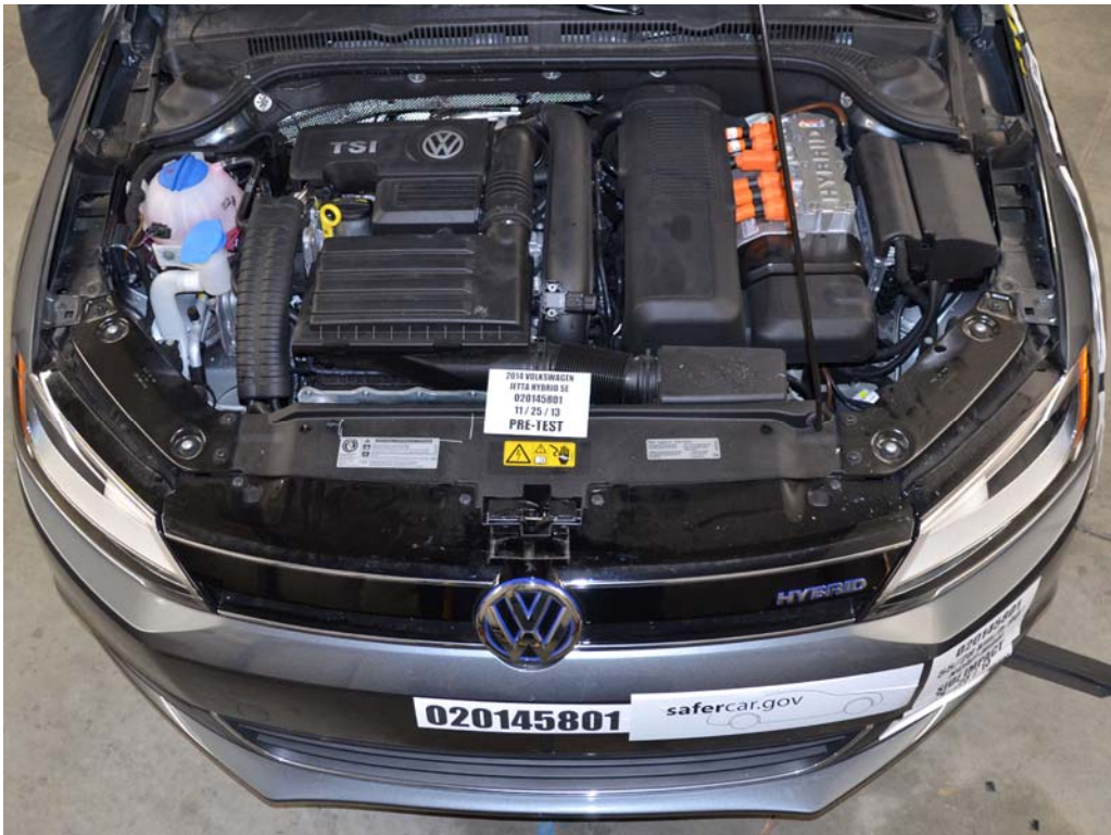
FIGURE 16. Pre-Impact View of Electric Propulsion Drive
