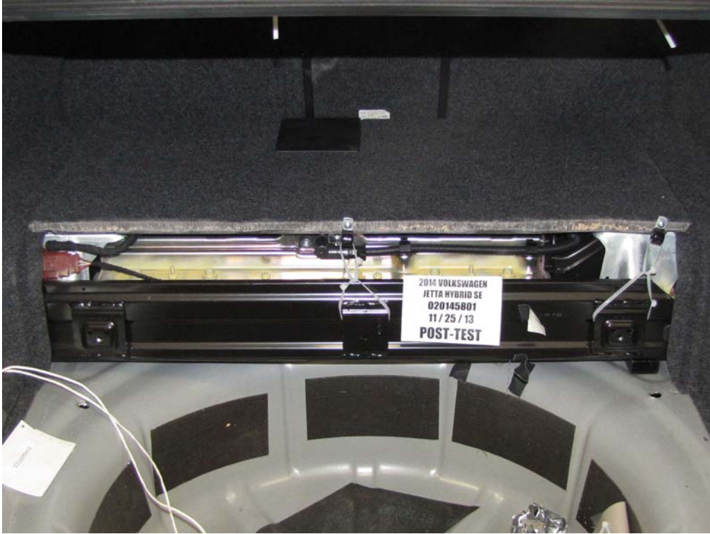
FIGURE 11. Post-Impact Rear View of Propulsion Battery
