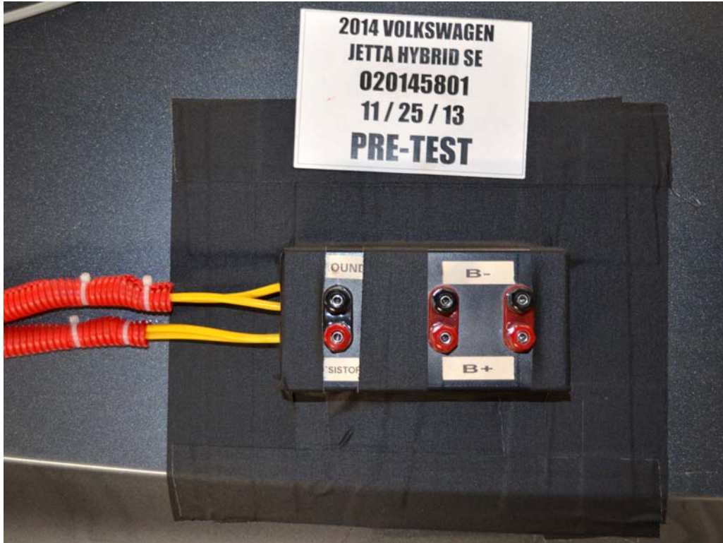
FIGURE 24. Pre-Impact View of Installed Test Interface Port
