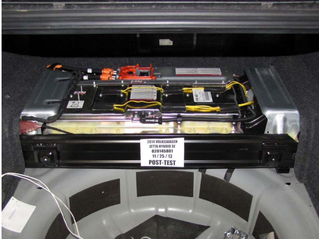
FIGURE 13a. Post-Impact View of Propulsion Battery Box(s) or Container(s) which Holds Individual Battery Modules
