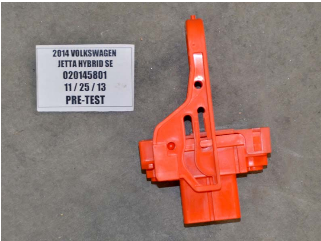
FIGURE 7. Manual High Voltage Service Disconnect Removed
