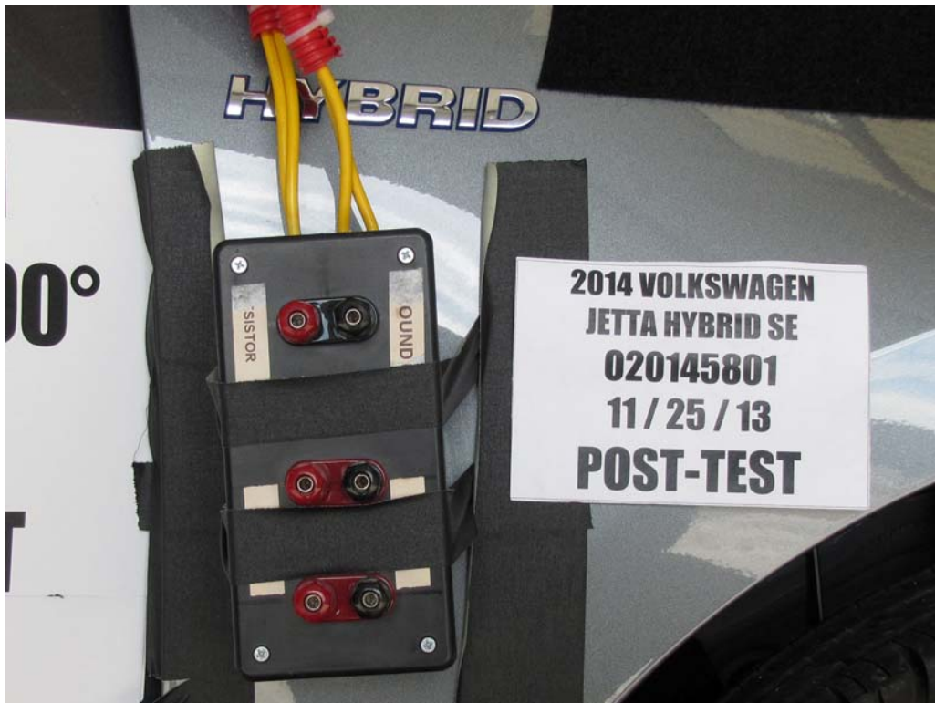
FIGURE 25. Post-Impact View of Installed Test Interface Port
