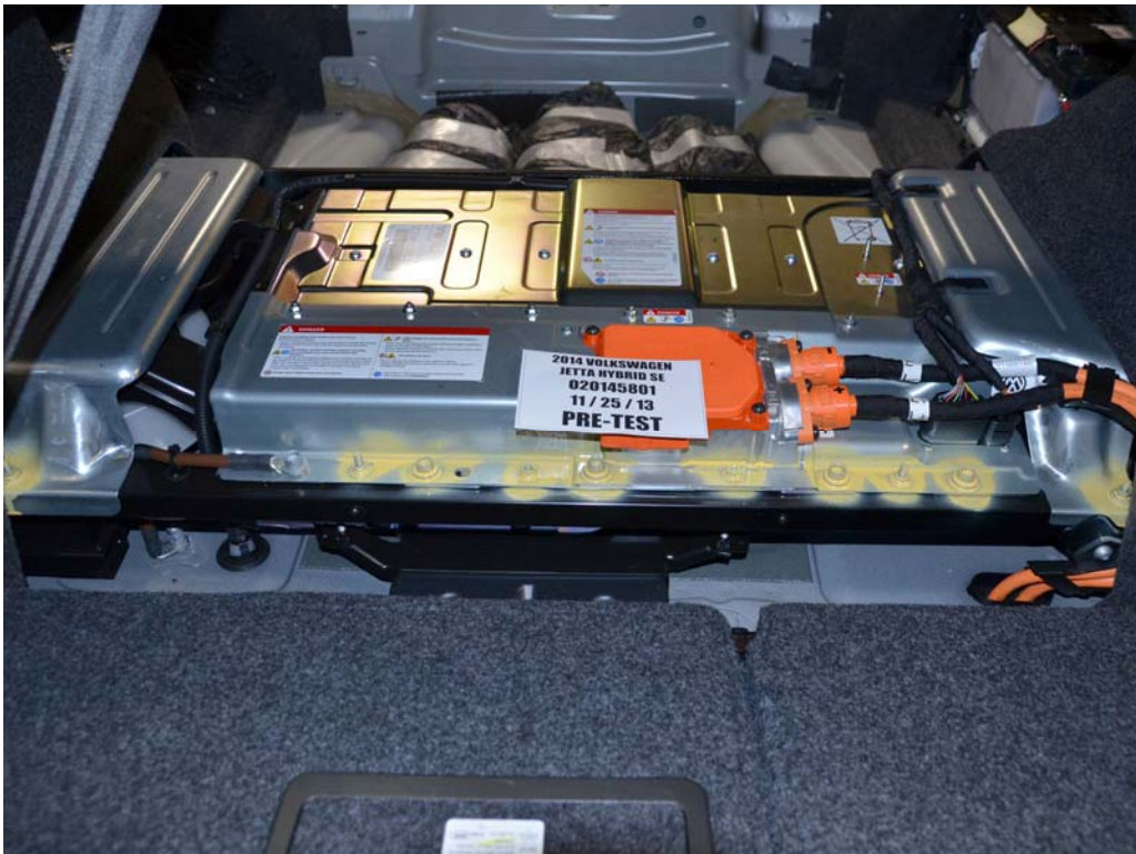
FIGURE 12. Pre-Impact View of Propulsion Battery Box(s) or Container(s) which Holds Individual Battery Modules
