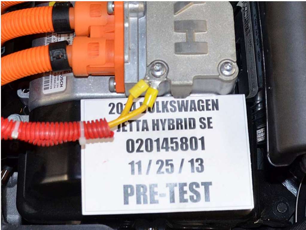
FIGURE 21. Pre-Impact View of Ground Lead Attached
