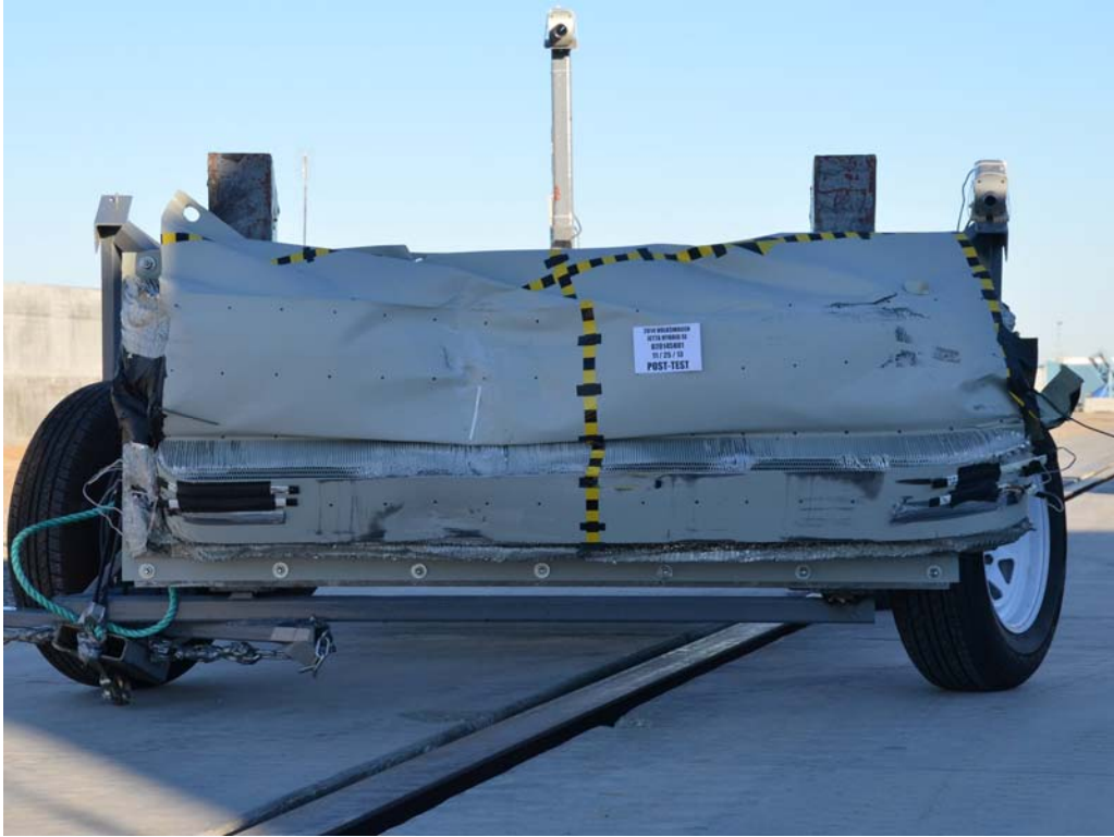
FIGURE 85. Post-Test Front View of MDB Impactor Face
