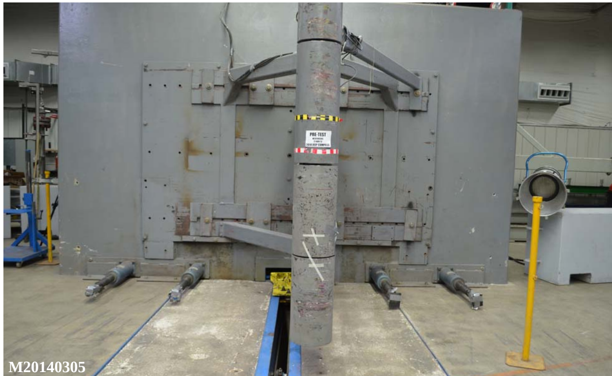
Figure 057: Pre-Test Pole Barrier Front View
