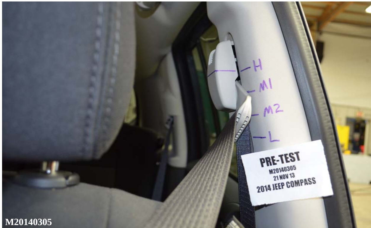
Figure 033: Pre-Test View of Belt Anchorage for Dummy
