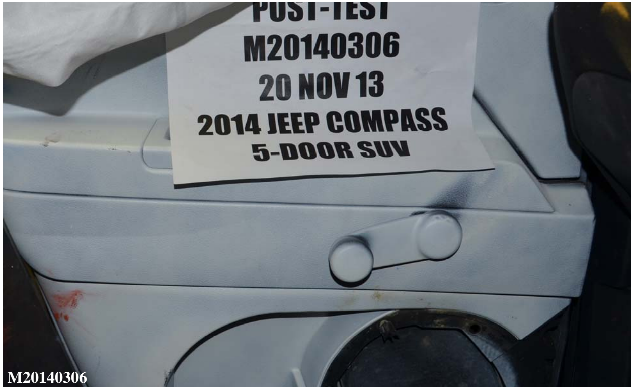
Figure A-81: Post-Test Rear Passenger Dummy Close-Up Knee Contact View
