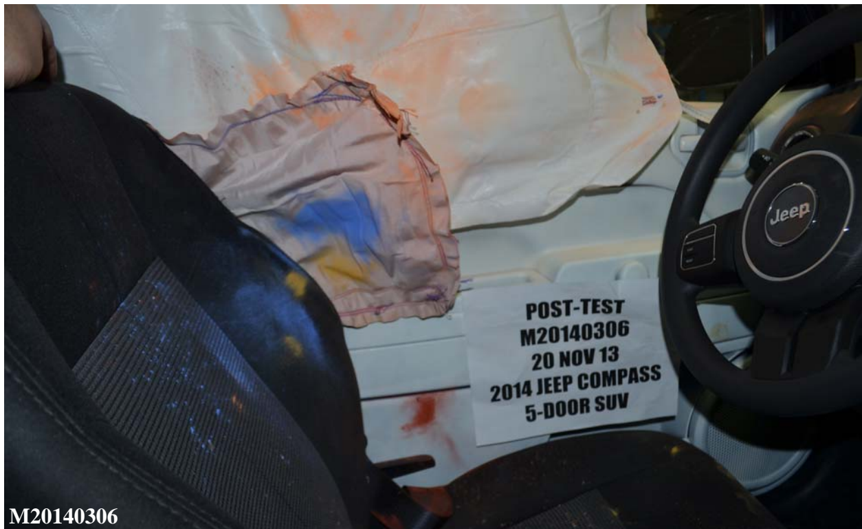
Figure A-50: Post-Test Driver Dummy Close-Up Torso Contact with Vehicle Interior View
