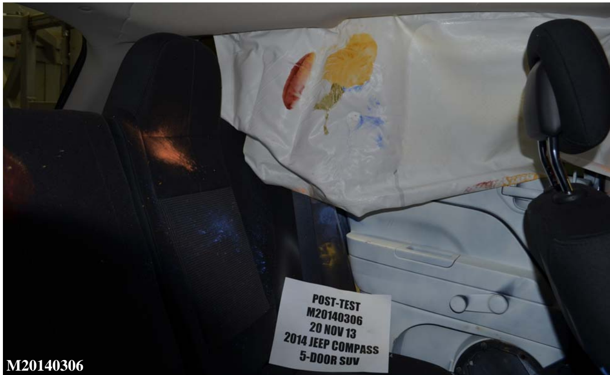
Figure A-74: Post-Test Rear Passenger Inner Door Panel View Showing Dummy Contact Locations
