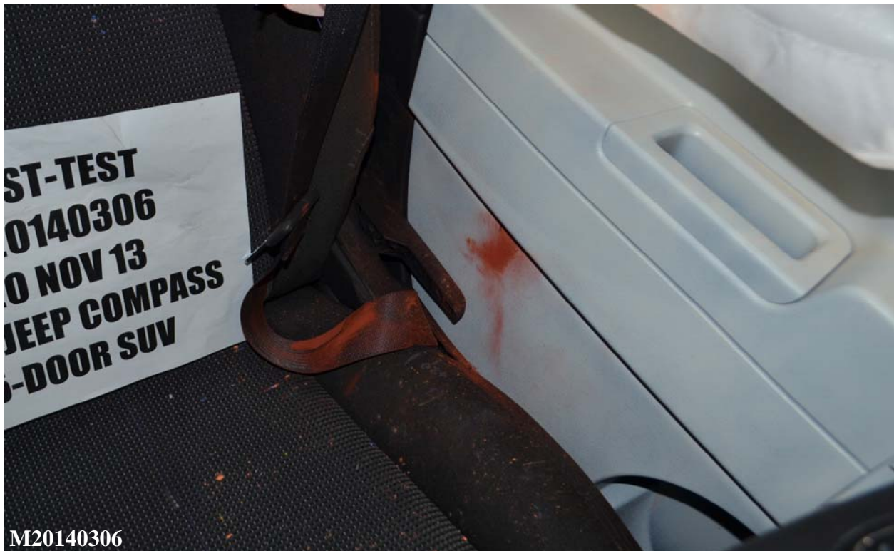
Figure A-52: Post-Test Driver Dummy Close-Up Pelvis Contact With Vehicle Interior View
