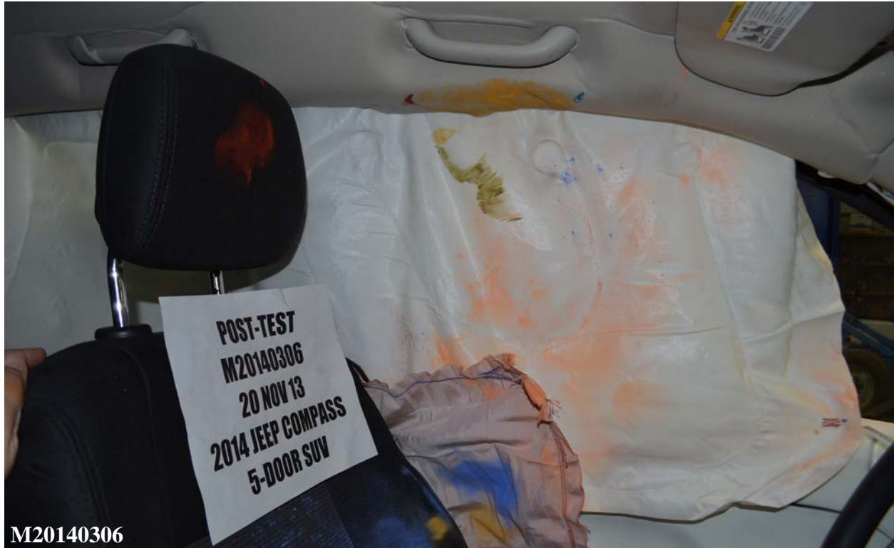
Figure A-49: Post-Test Driver Dummy Close-Up Head Contact with Side Airbag View
