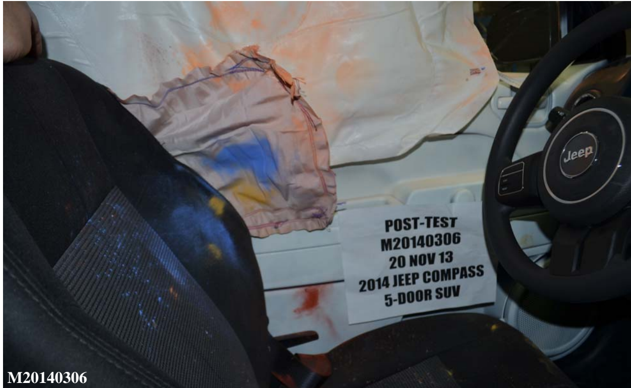
Figure A-51: Post-Test Driver Dummy Close-Up Torso Contact with Side Air Bag View
