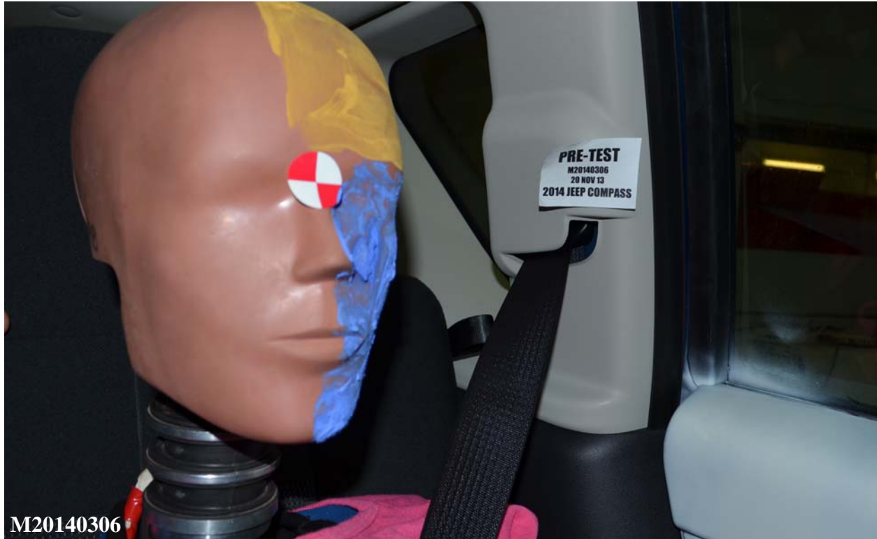
Figure A-65: Pre-Test View of Belt Anchorage for Rear Passenger Dummy
