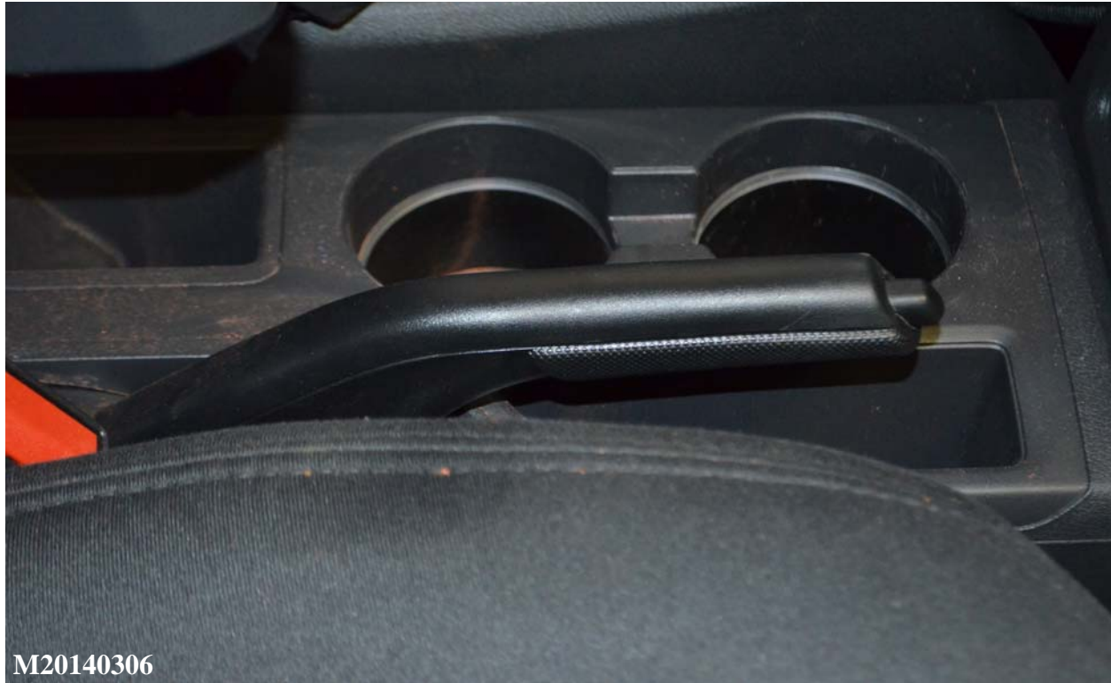
Figure A-37: View of Disengaged Parking Brake
