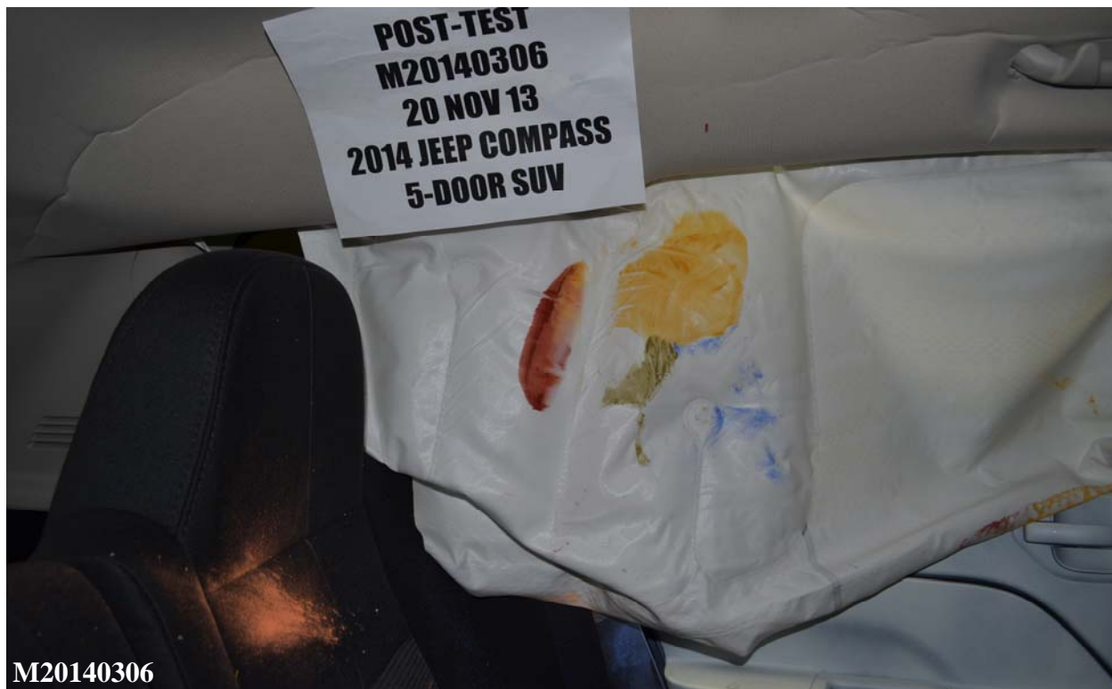
Figure A-76: Post-Test Rear Passenger Dummy Close-Up Head Contact with Side Airbag View
