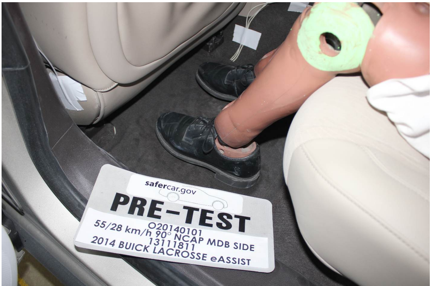
Pre-Test Placement of Rear Passenger Dummy's Feet
