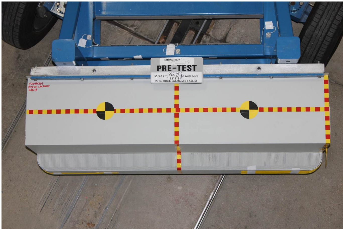
Pre-Test Top View of MDB Impactor Face
