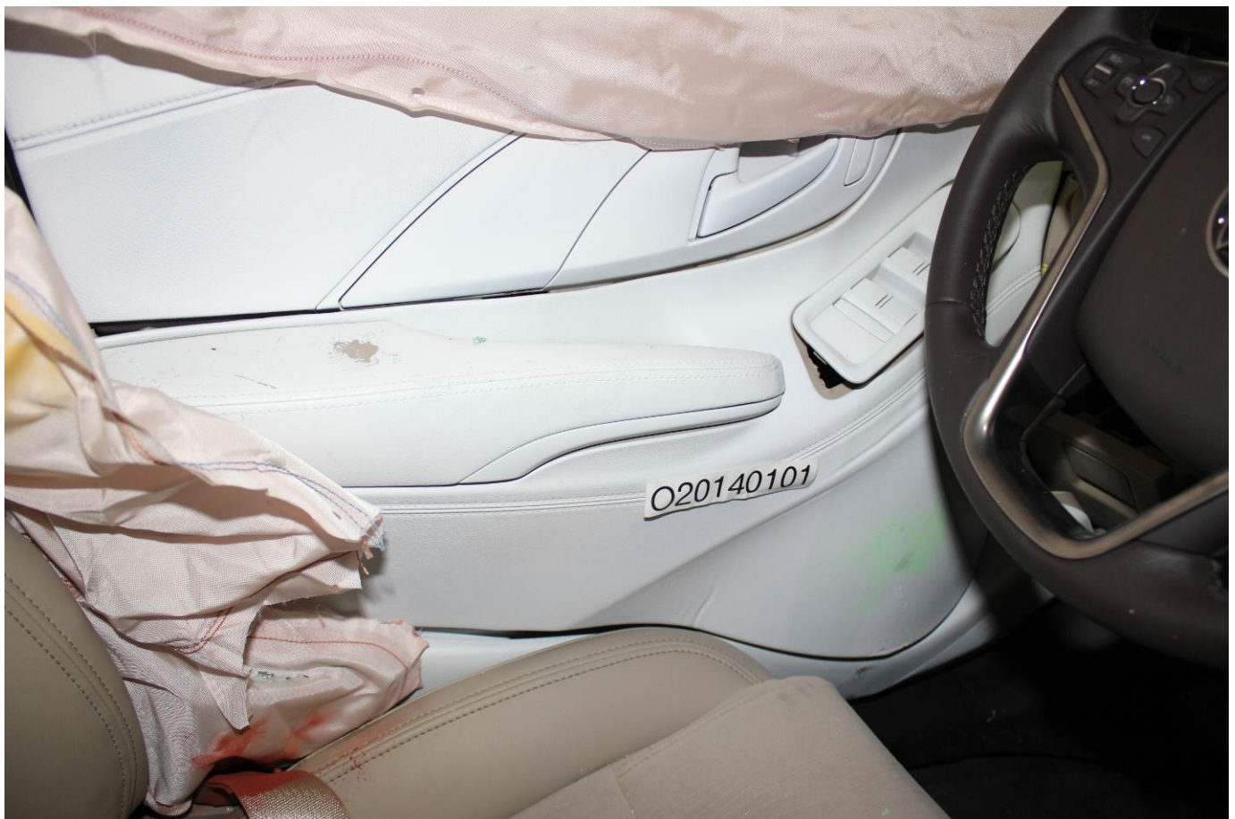
Post-Test Driver Dummy Close-up Knee Contact View
