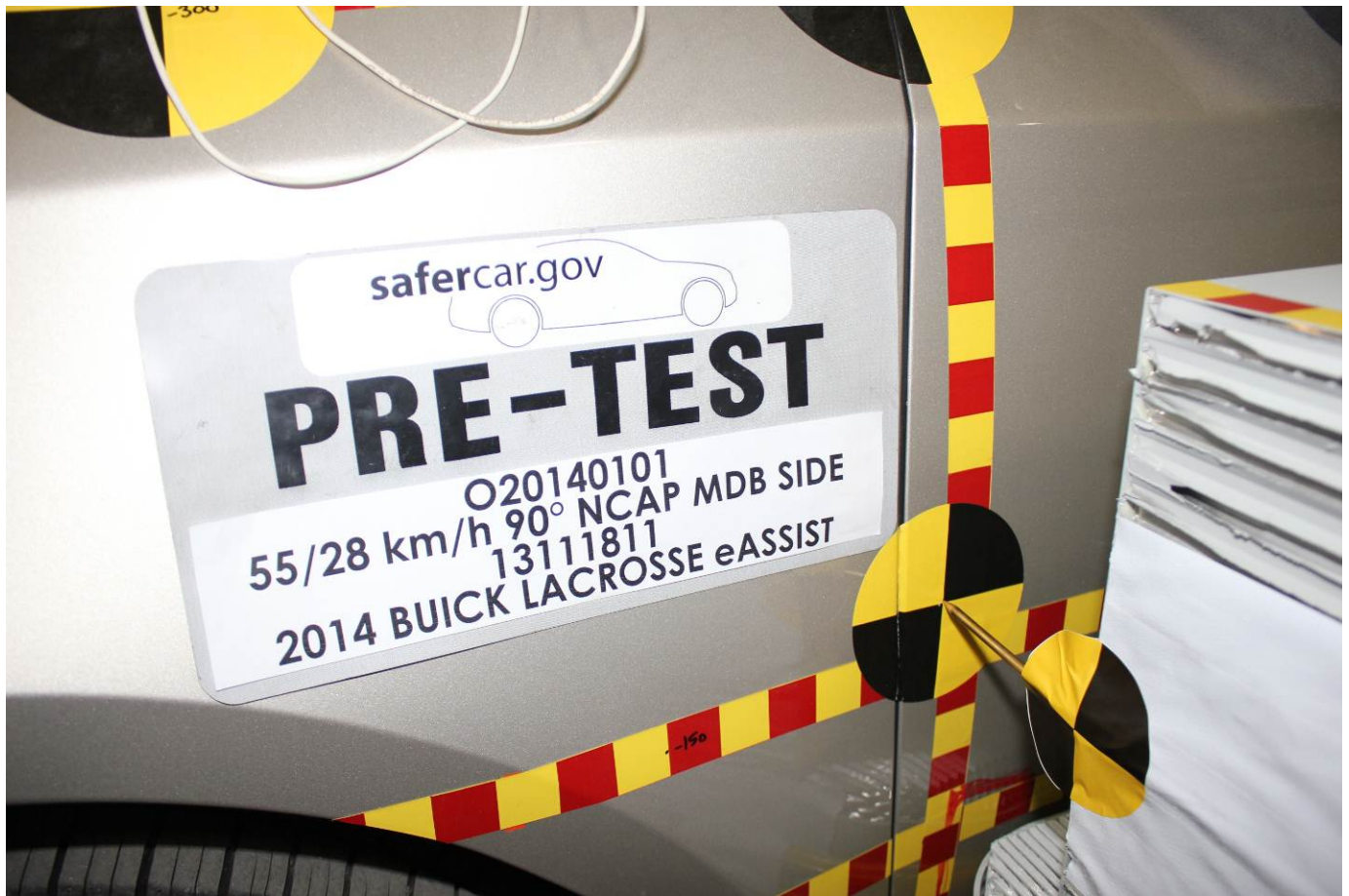
Pre-Test Close-Up View of Impact Point Target
