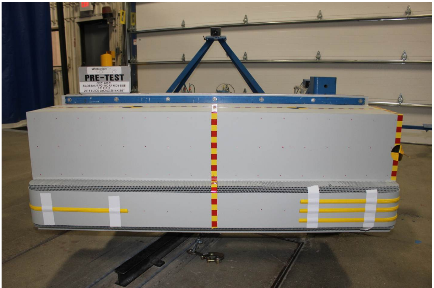
Pre-Test Front View of MDB Impactor Face
