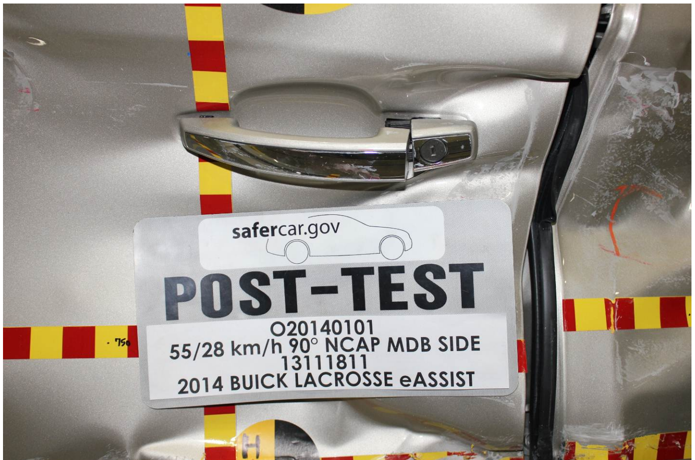
Post-Test Left Front Door Latch Close-Up
