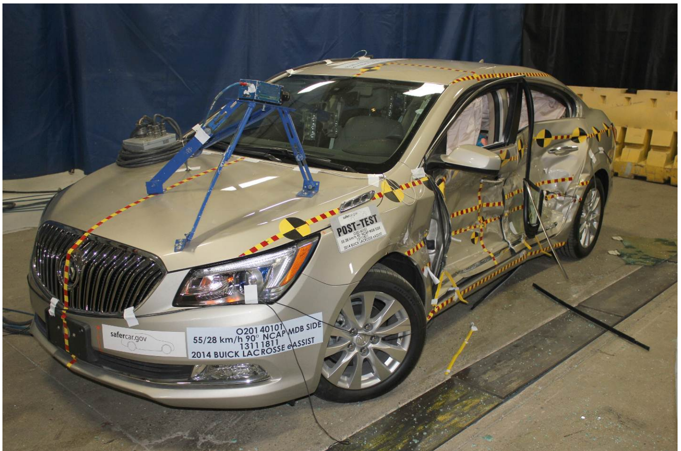
Post-Test Left Front Three-Quarter View of Test Vehicle
