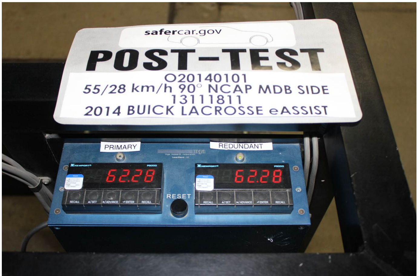
Post-Test Primary and Redundant Speed Trap Read-Out
