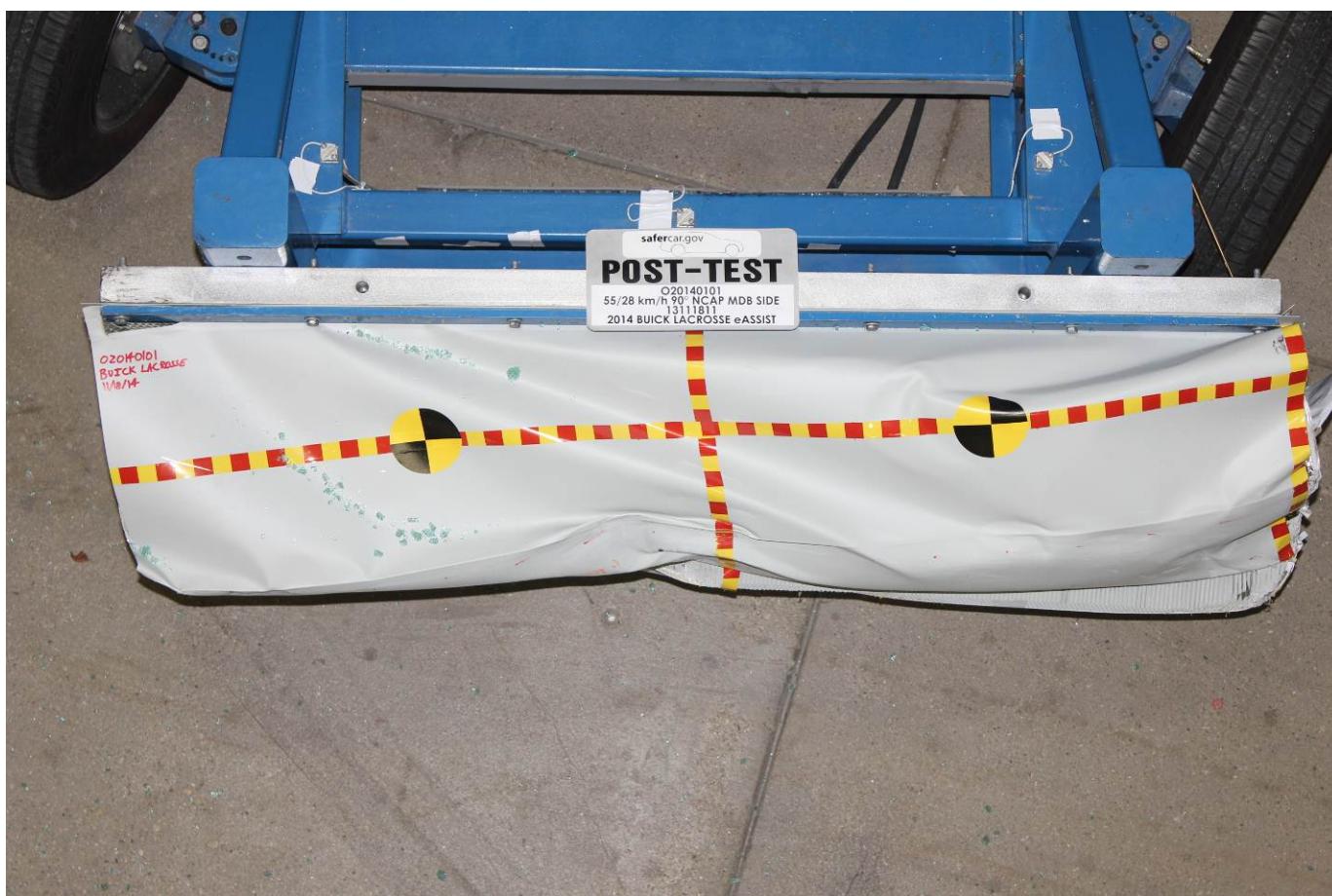
Post-Test Top View of MDB Impactor Face
