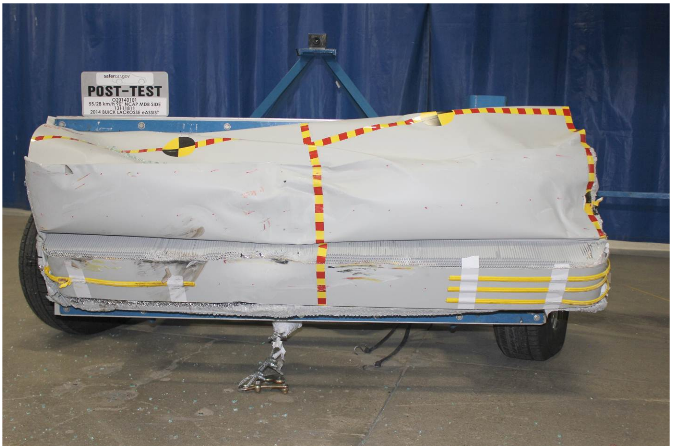
Post-Test Front View of MDB Impactor Face
