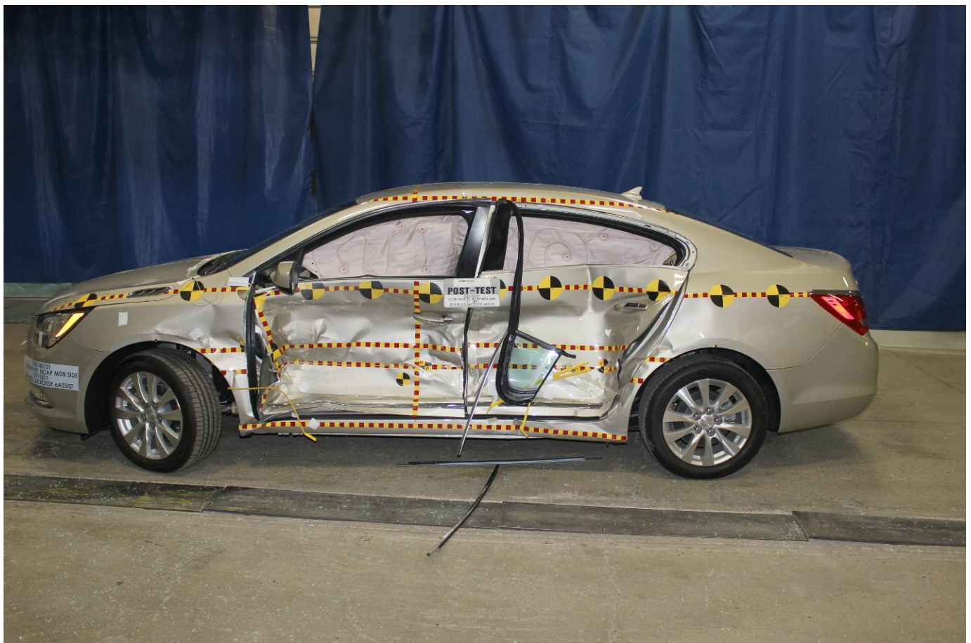
Post-Test Left Side View of Test Vehicle
