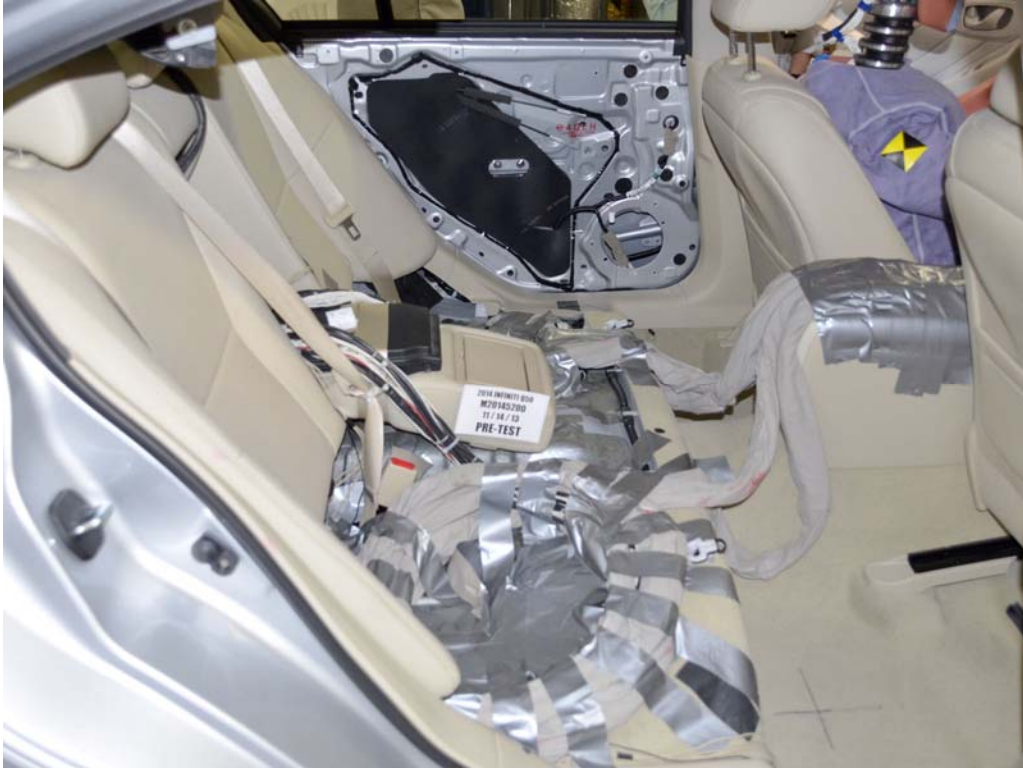
FIGURE 27. Pre-Test Dummy Cable Routing
