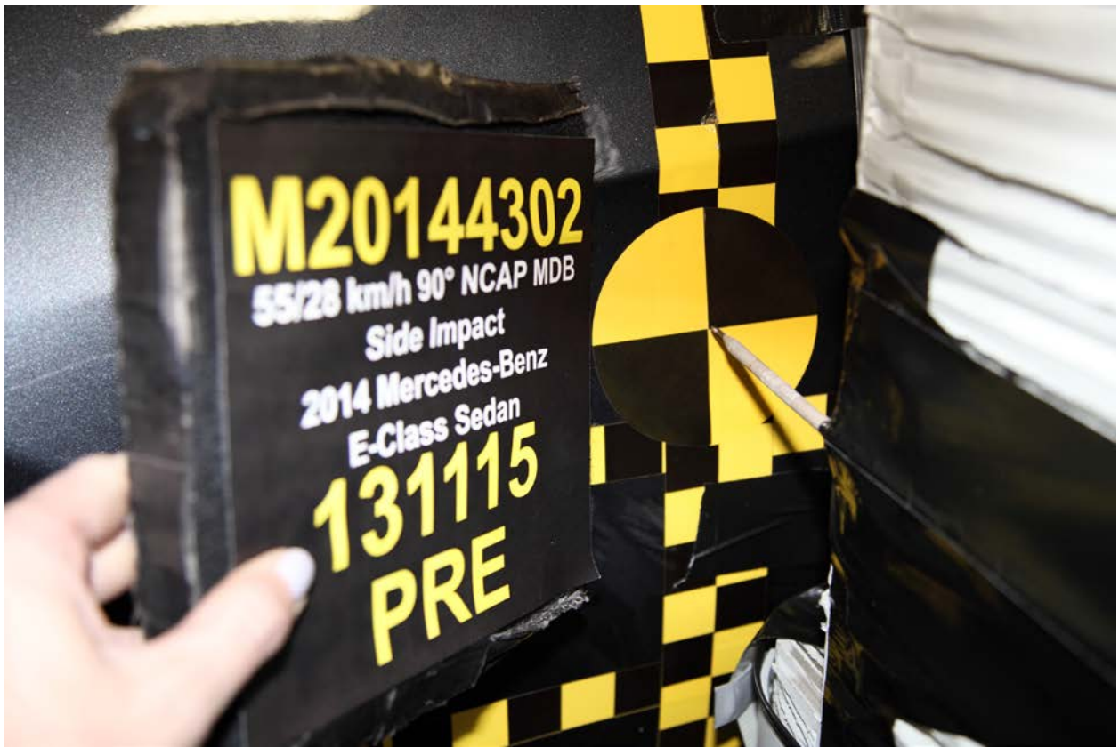
019 Pre-Test Close-up View of Impact Point Target
