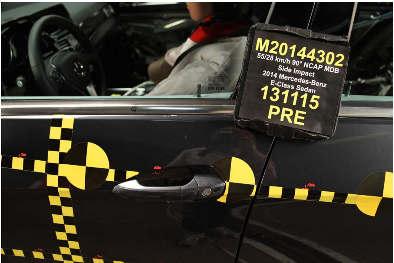
021 Pre-Test Left Front Door Latch Close-up
