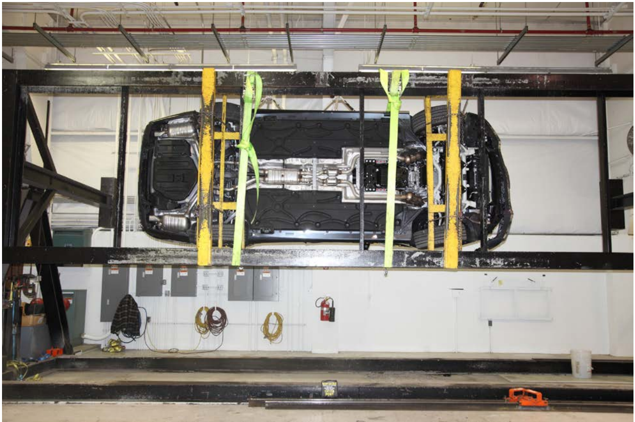
099 FMVSS No. 301 Static Rollover 270 Degrees
