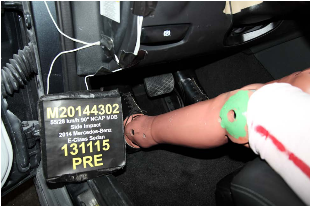
034 Pre-Test Placement of Driver Dummy Feet
