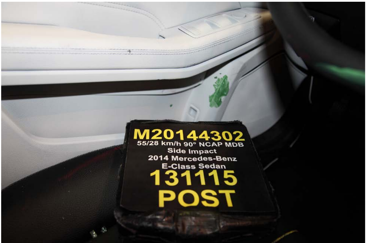
054 Post-Test Driver Dummy Close-Up Knee Contact View
