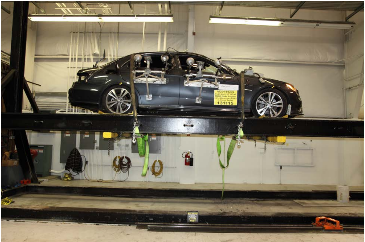
096 FMVSS No. 301 Static Rollover 0 Degrees
