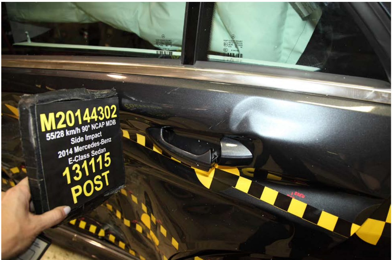
024 Post-Test Left Rear Door Latch Close-up
