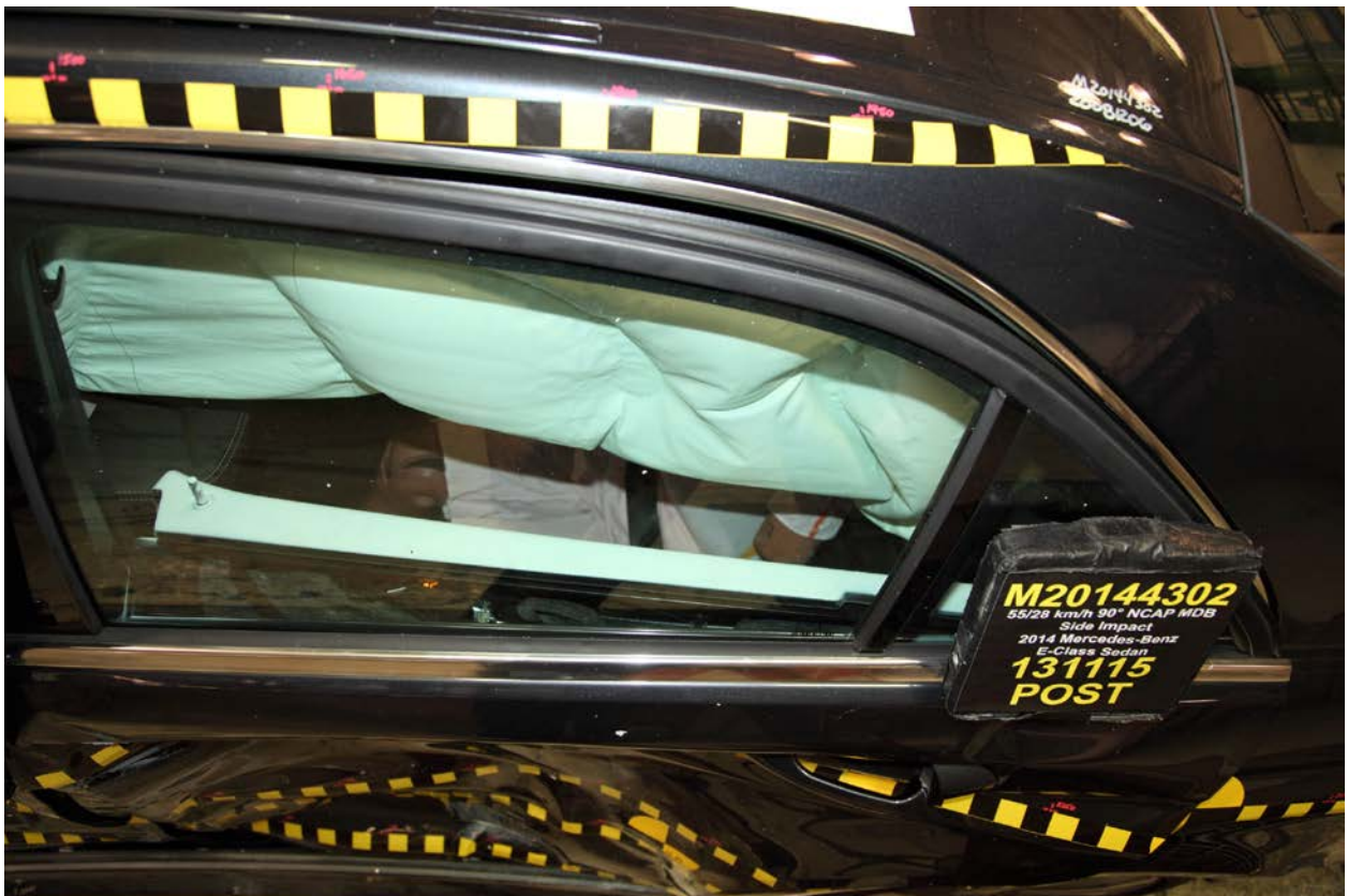
070 Post-Test Passenger Dummy and Door Clearance View
