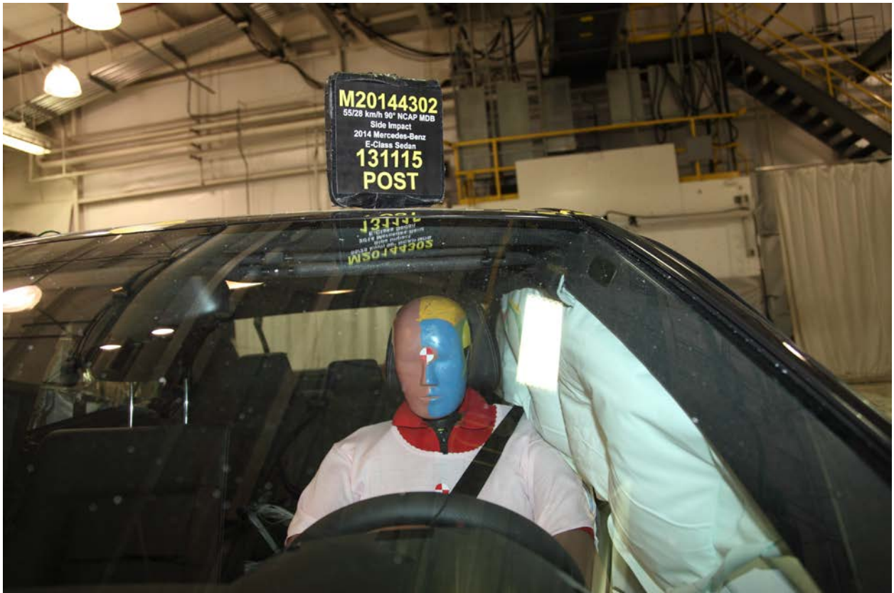
026 Post-Test Front Close-up View of Driver Dummy
