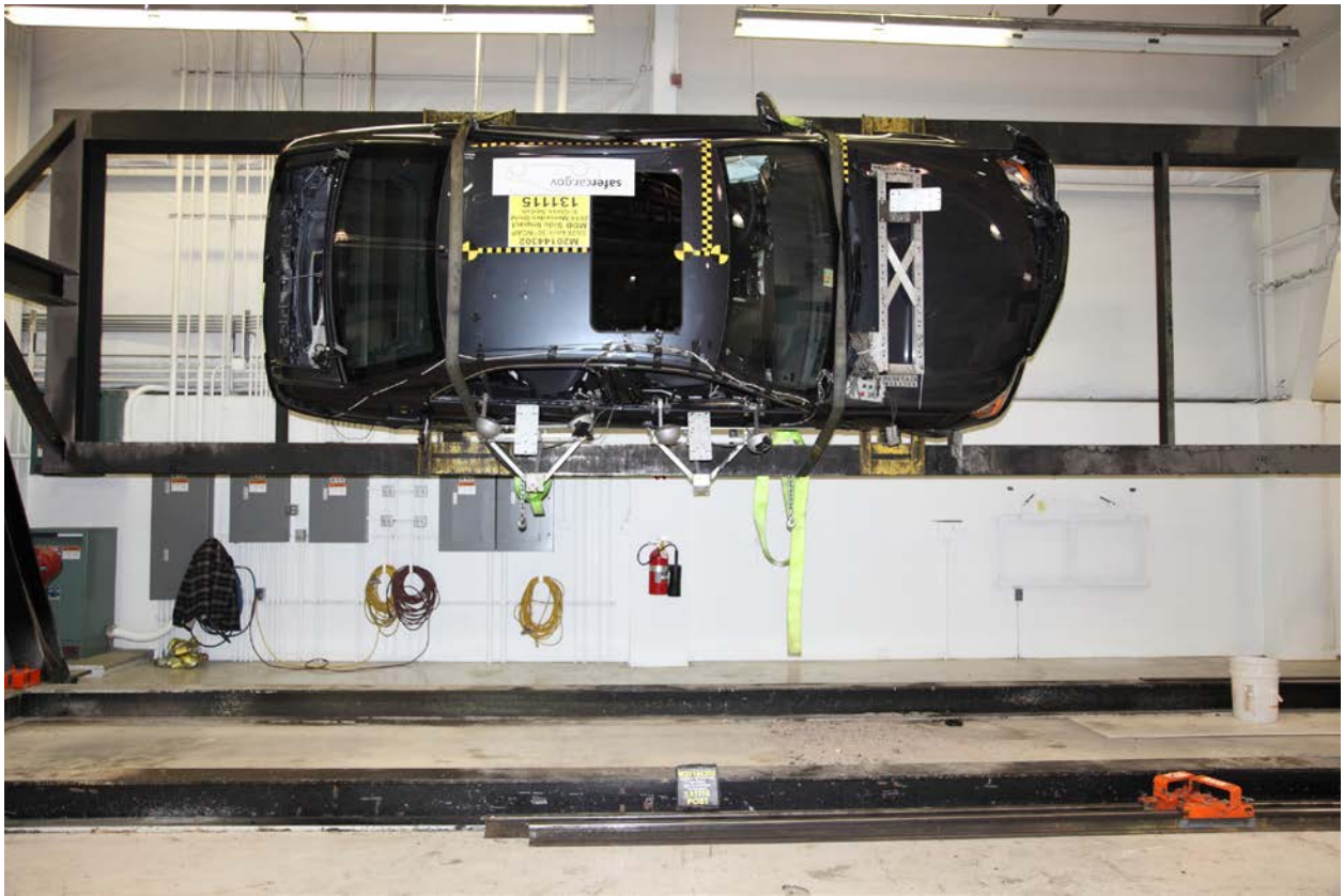
097 FMVSS No. 301 Static Rollover 90 Degrees
