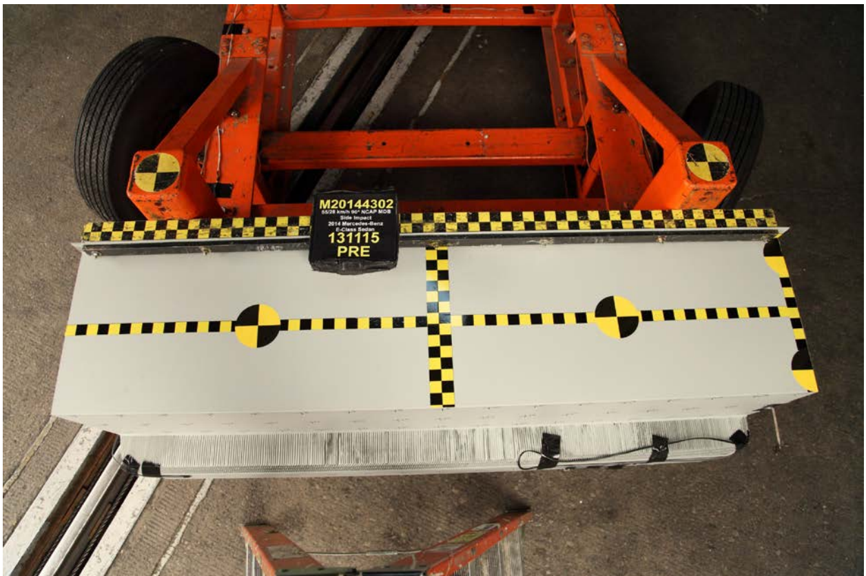
086 Pre-Test Top View of MDB Impactor Face
