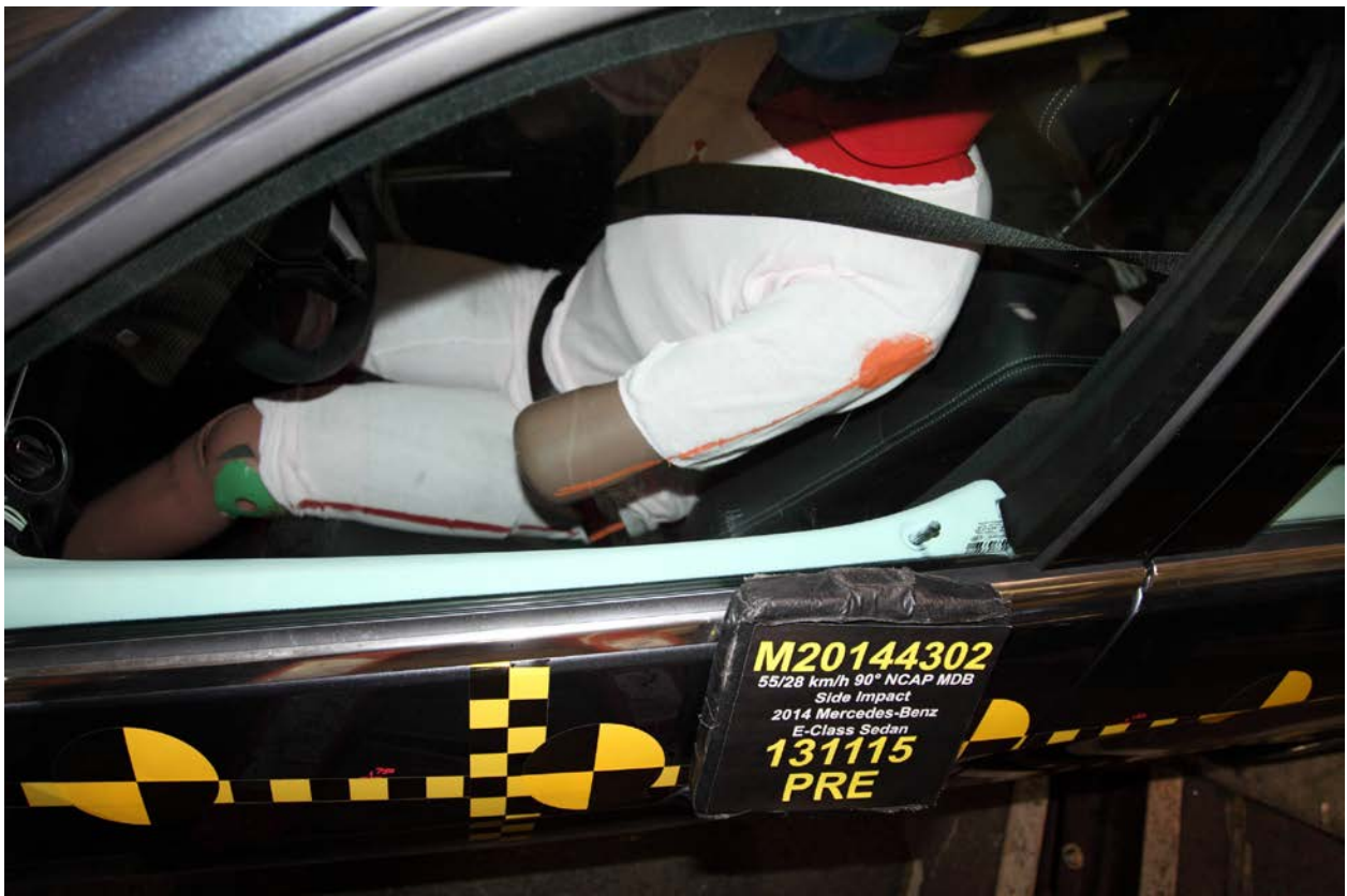
042 Pre-Test Driver Dummy and Door Clearance View
