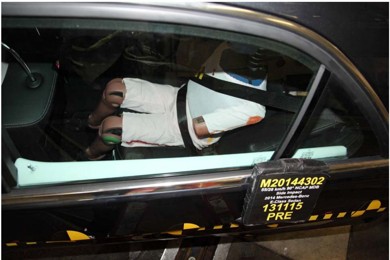
069 Pre-Test Passenger Dummy and Door Clearance View
