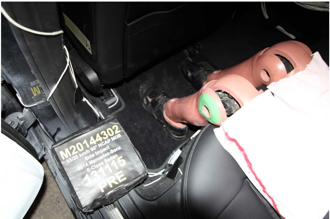
064 Pre-Test Placement of Rear Passenger Dummy Feet
