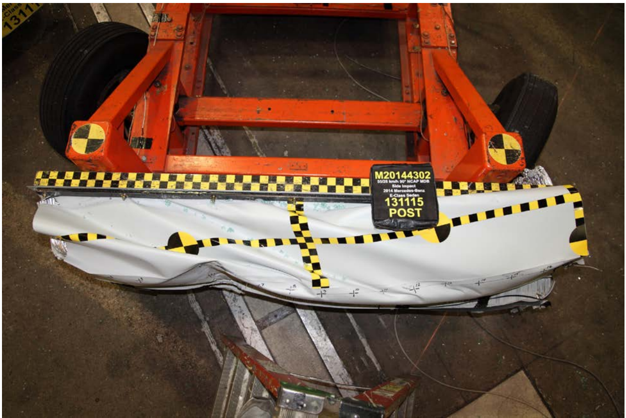
087 Post-Test Top View of MDB Impactor Face
