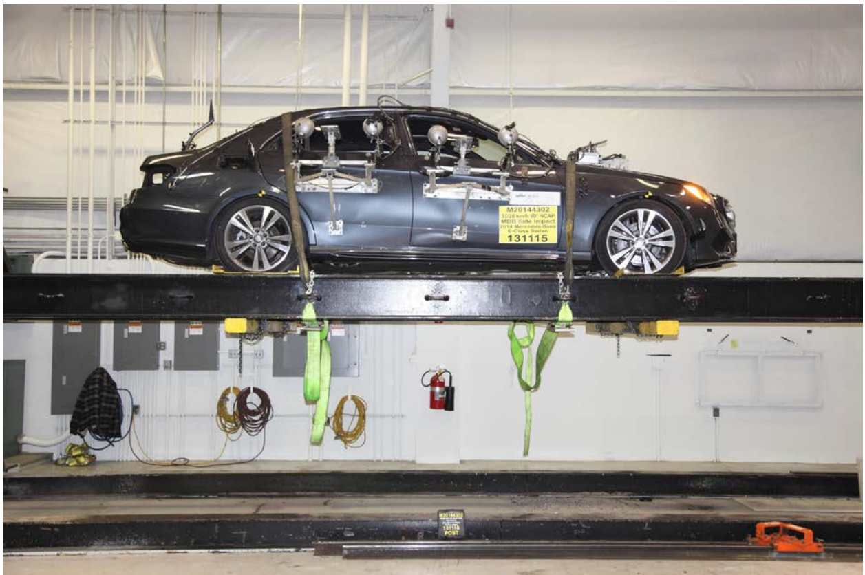
100 FMVSS No. 301 Static Rollover 360 Degrees
