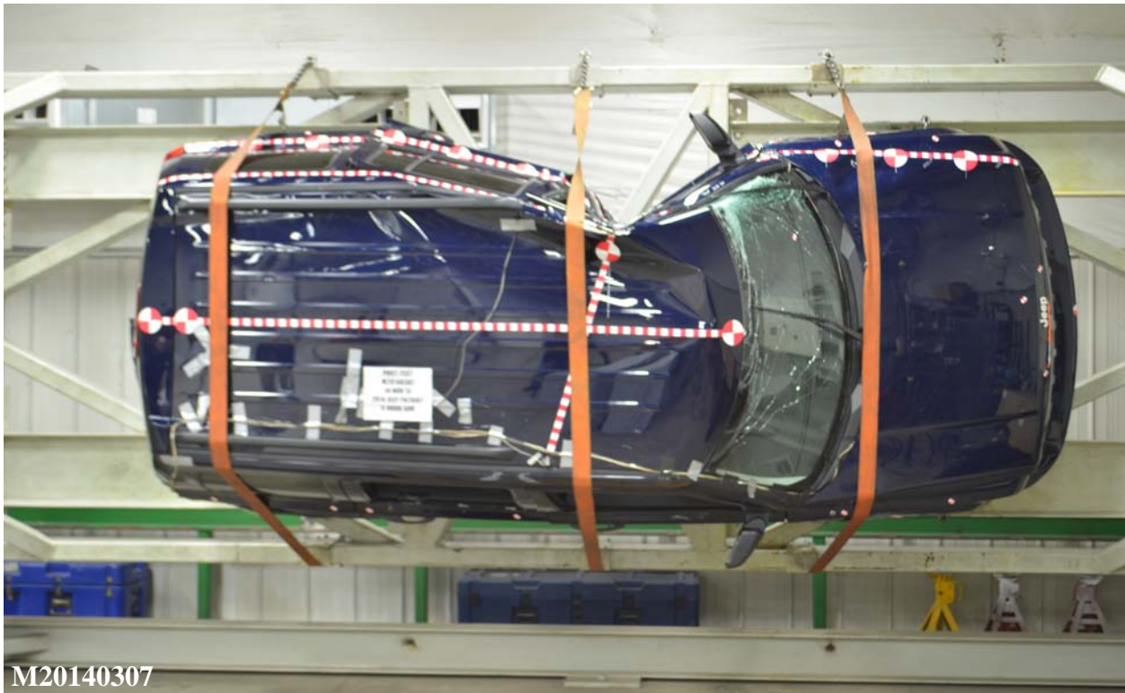
Figure 066: FMVSS No. 301 Static Rollover 270 Degrees
