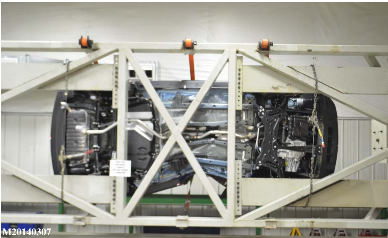
Figure 064: FMVSS No. 301 Static Rollover 90 Degrees
