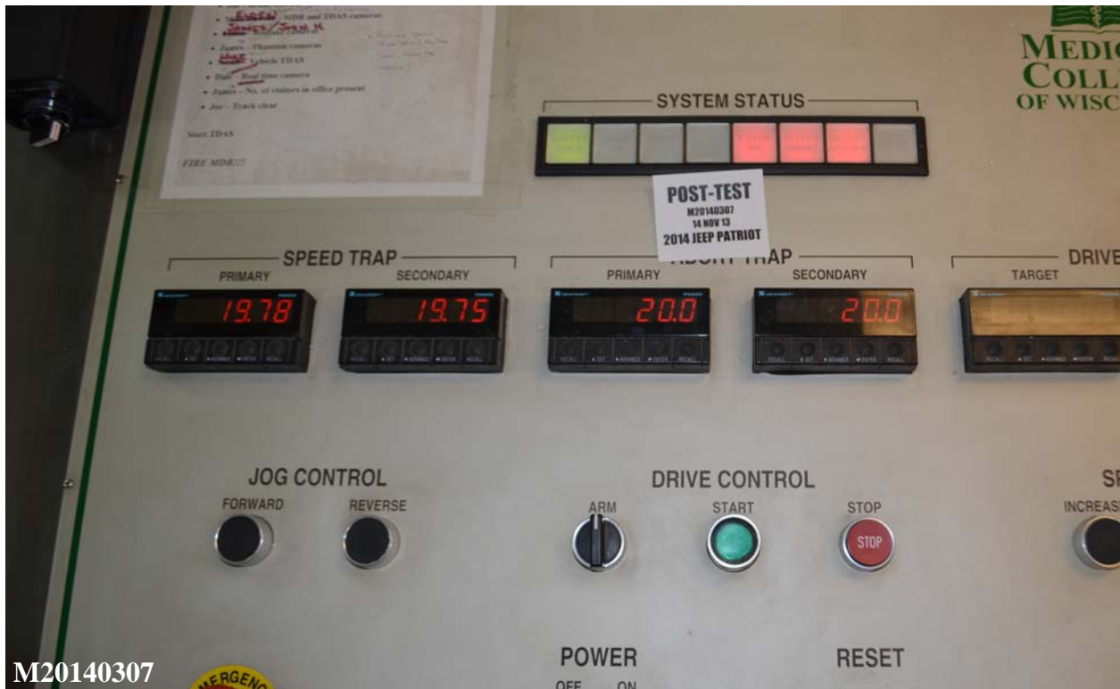
Figure 062: Post-Test Primary and Redundant Speed Trap Read-Out
