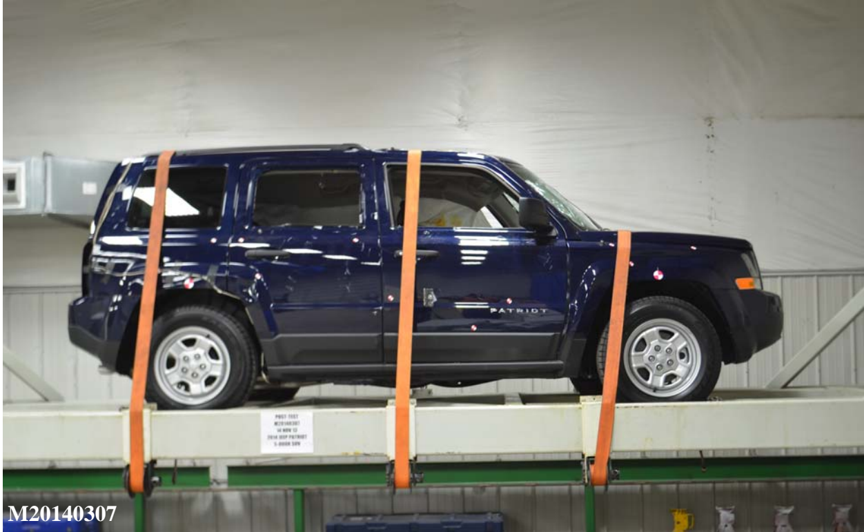
Figure 067: FMVSS No. 301 Static Rollover 360 Degrees
