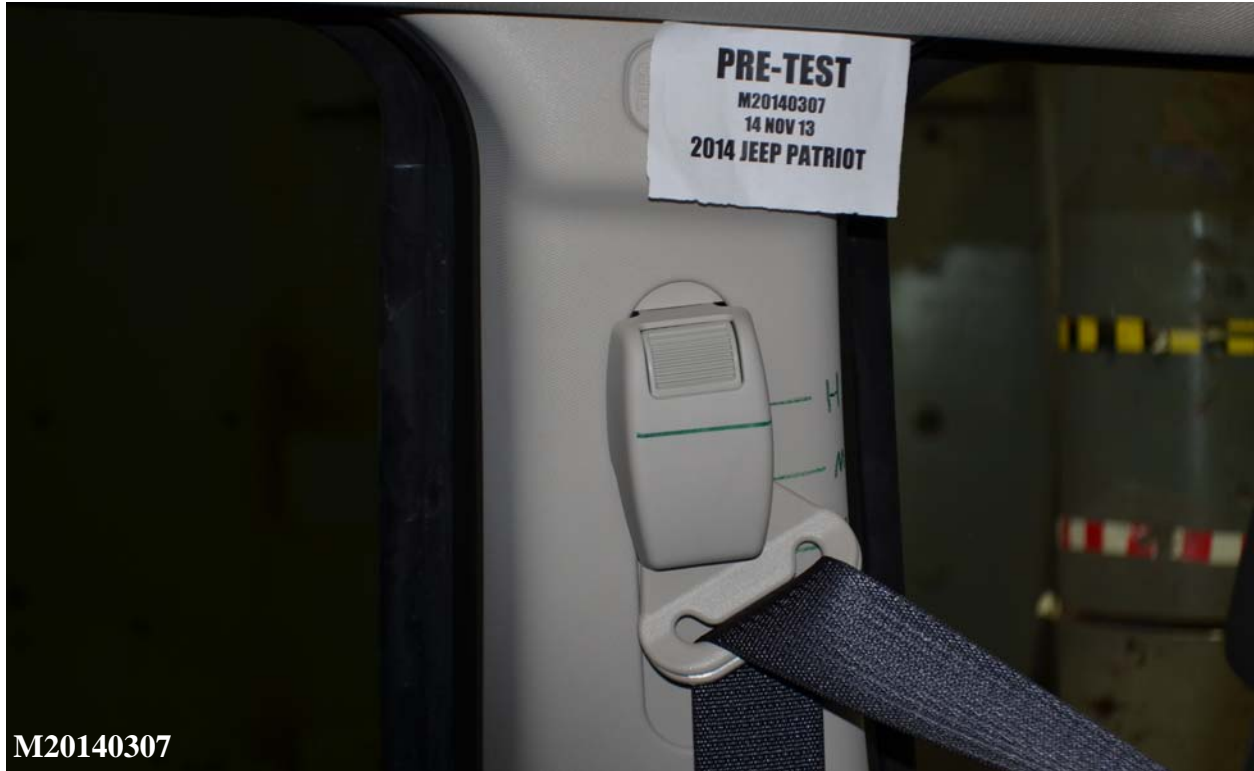
Figure 033: Pre-Test View of Belt Anchorage for Dummy
