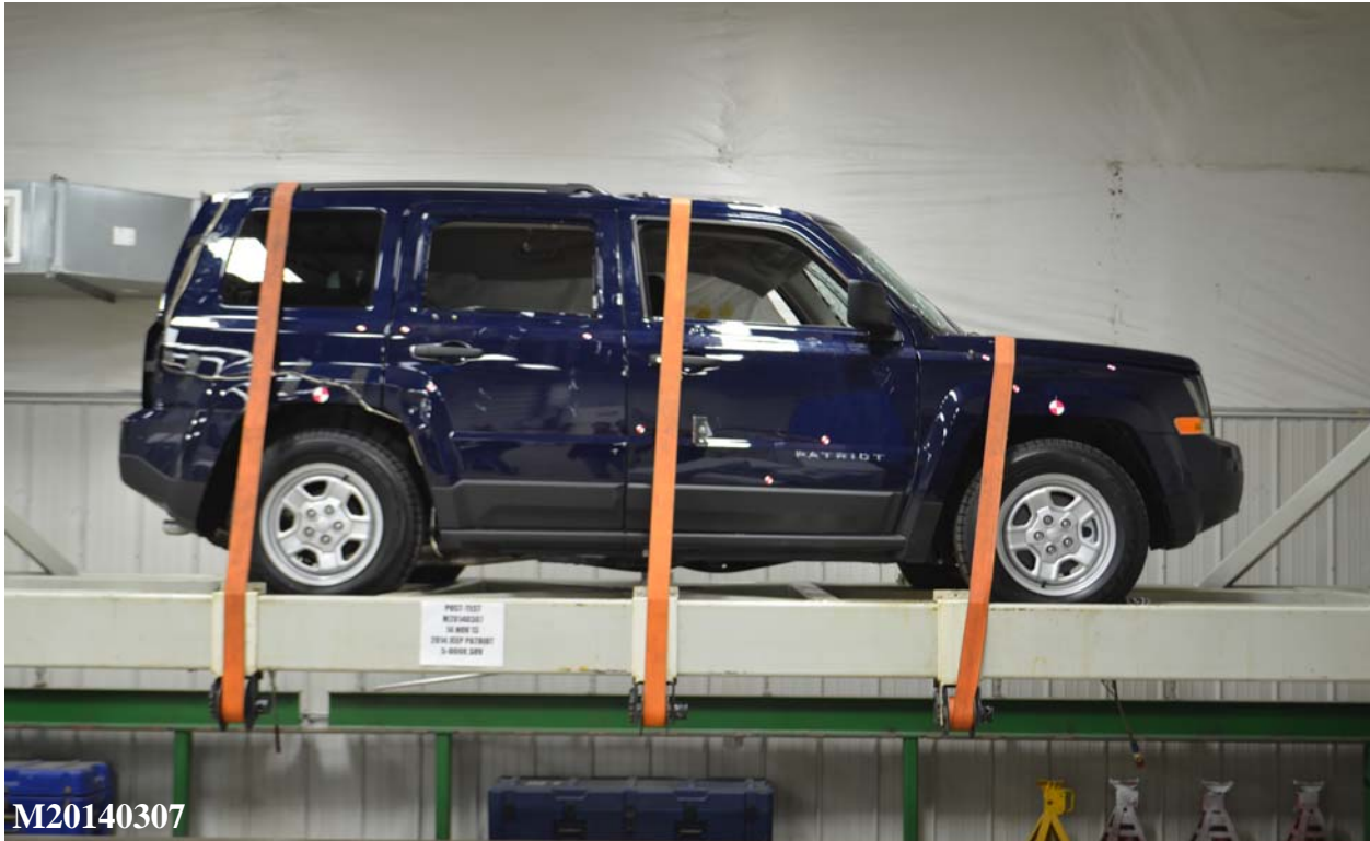
Figure 063: FMVSS No. 301 Static Rollover 0 Degrees
