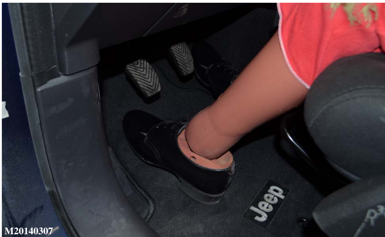
Figure 032: Pre-Test Placement of Dummy's Feet
