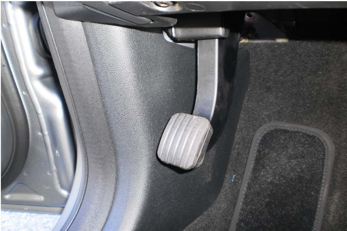
035 Pre-Test View of Disengaged Parking Brake
