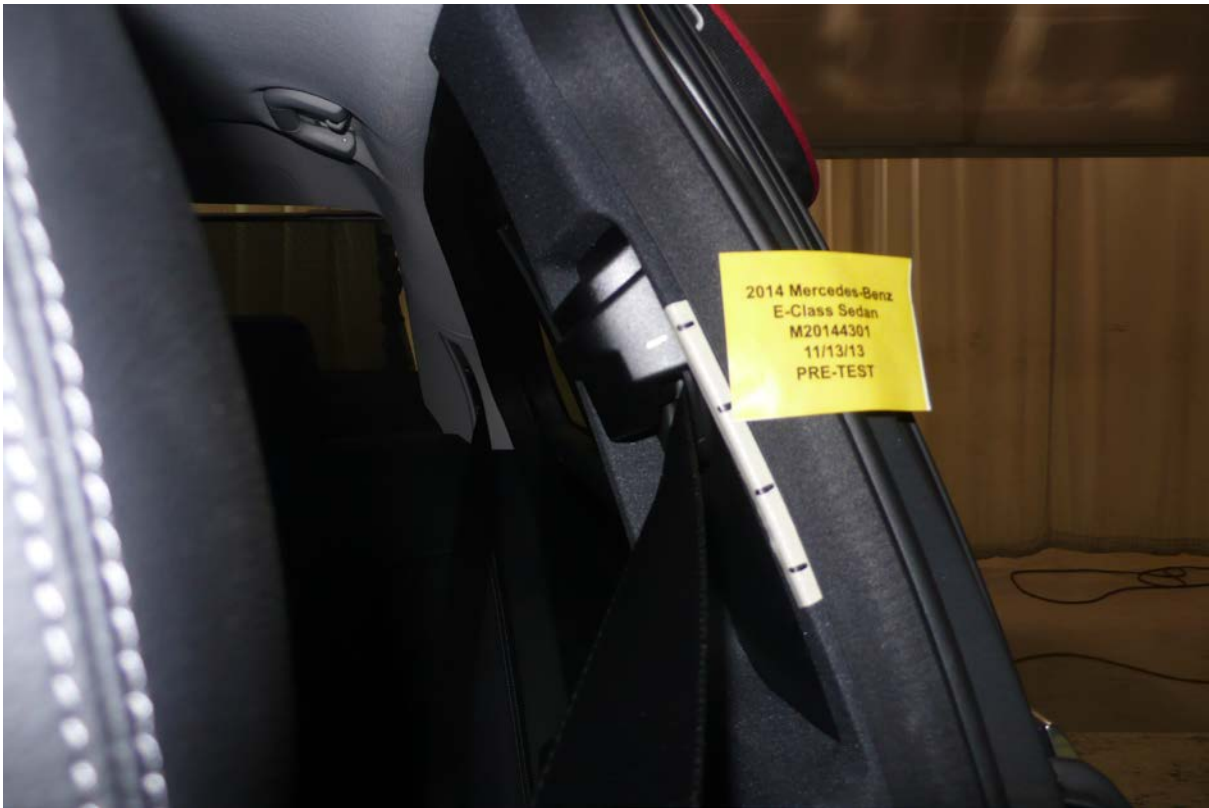
033 Pre-Test View of Belt Anchorage for Dummy
