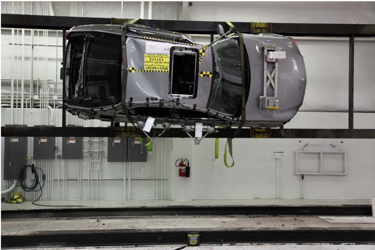
064 FMVSS No. 301 Static Rollover 90 Degrees
