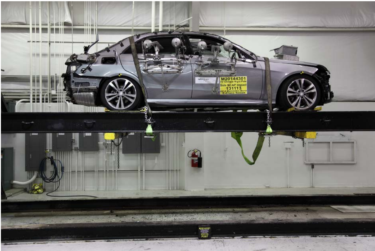
067 FMVSS No. 301 Static Rollover 360 Degrees
