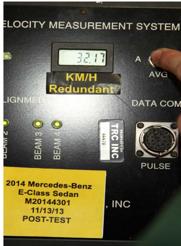
062 Post-Test Primary and Redundant Speed Trap Read-Out
