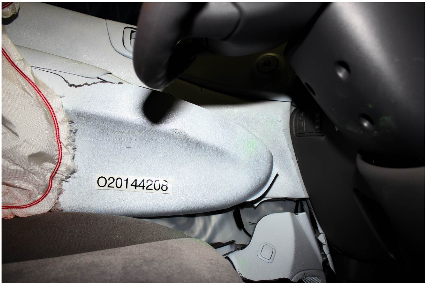
Post-Test Driver Dummy Close-up Knee Contact View
