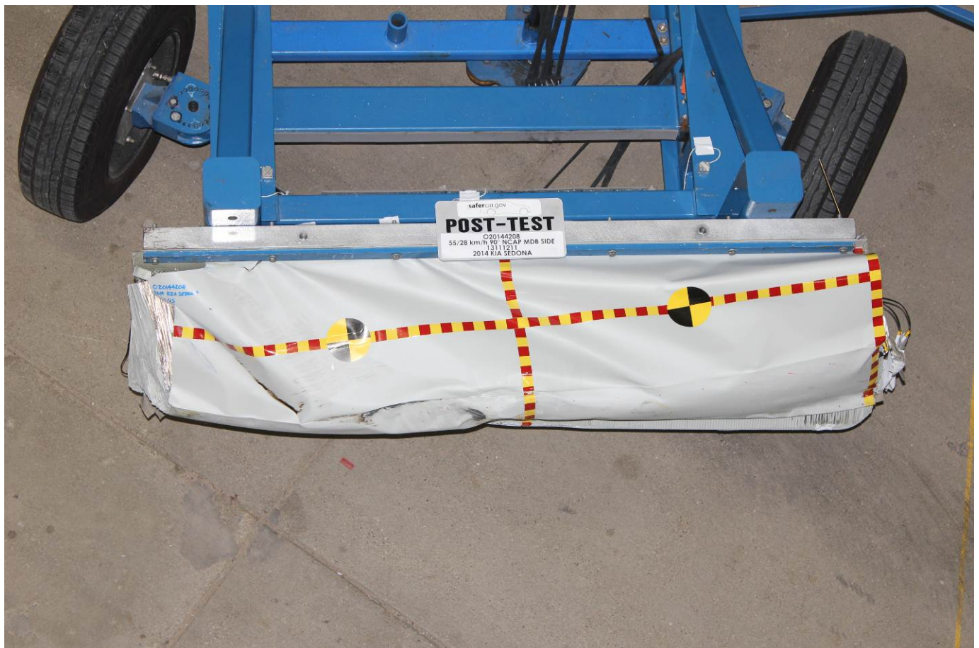
Post-Test Top View of MDB Impactor Face
