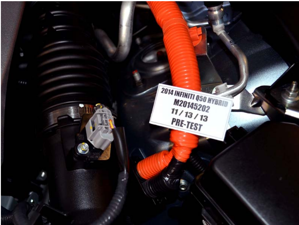
FIGURE 18c. Pre-Impact View of High Voltage Interconnects
