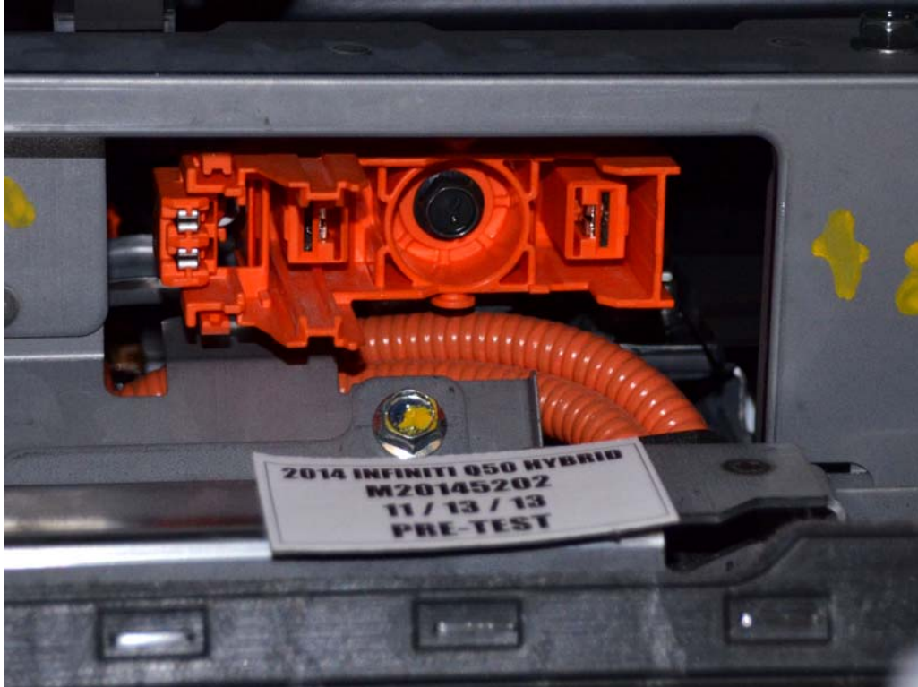
FIGURE 8. Manual High Voltage Service Disconnect Removed
