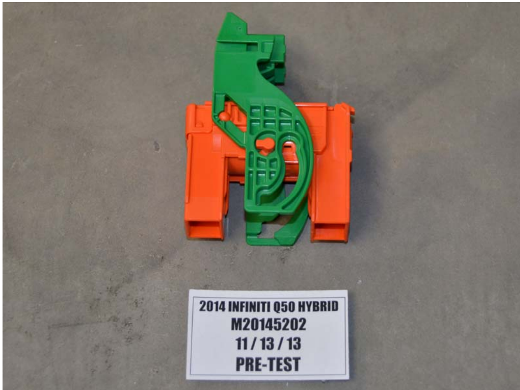
FIGURE 7. Manual High Voltage Service Disconnect Removed
