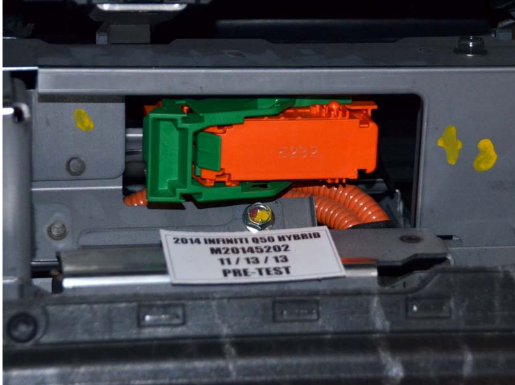
FIGURE 6. Manual High Voltage Service Disconnect in Place
