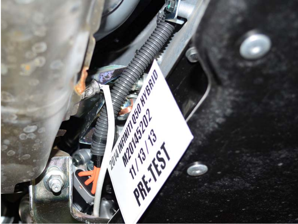
FIGURE 18b. Pre-Impact View of High Voltage Interconnects
