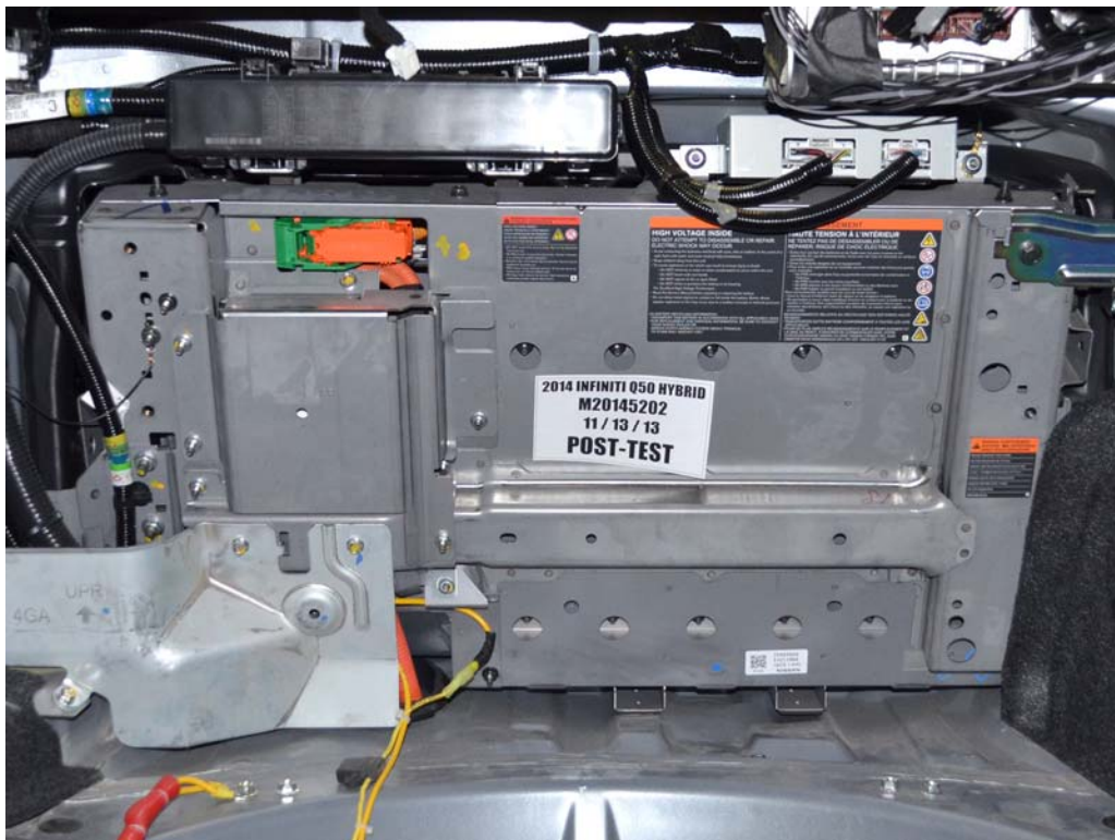
FIGURE 11. Post-Impact Rear View of Propulsion Battery
