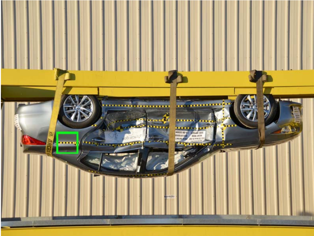
FIGURE 30. FMVSS No. 305 Static Rollover at 180°
