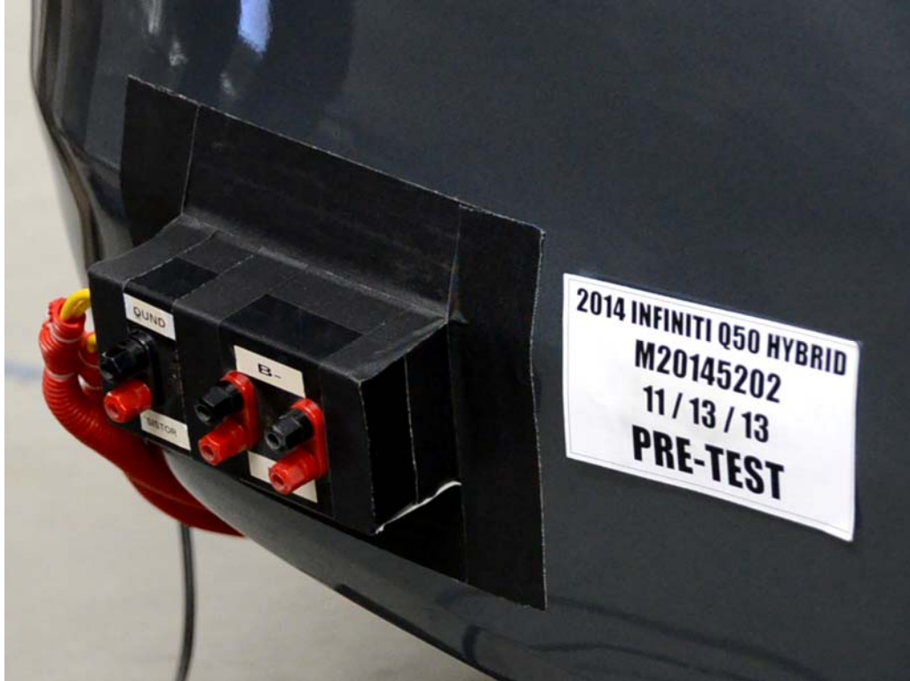
FIGURE 24. Pre-Impact View of Installed Test Interface Port
