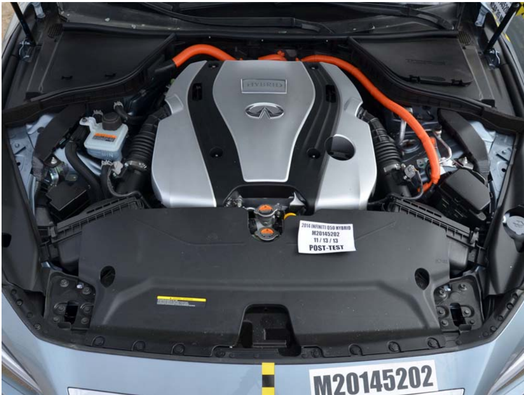
FIGURE 17. Post-Impact View of Electric Propulsion Drive
