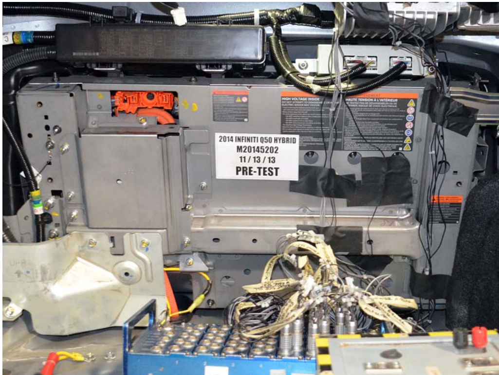
FIGURE 9. Pre-Impact View of Propulsion Battery
