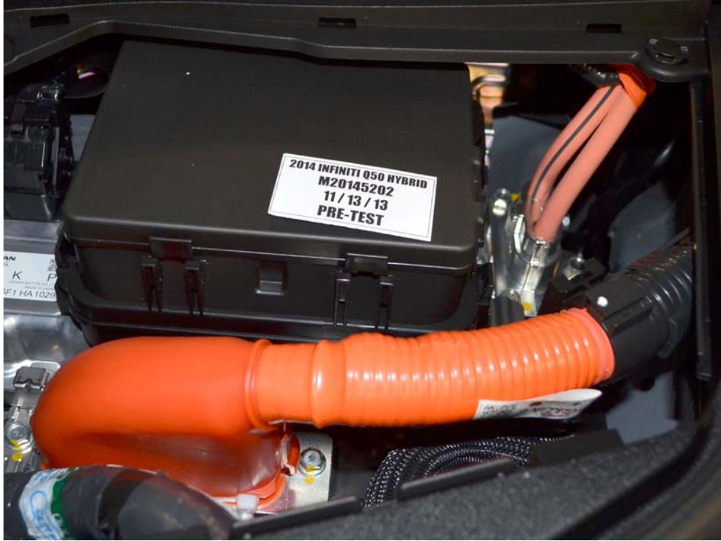
FIGURE 18d. Pre-Impact View of High Voltage Interconnects
