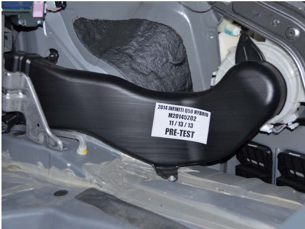
FIGURE 19. Pre-Impact View of Propulsion Battery Venting System
