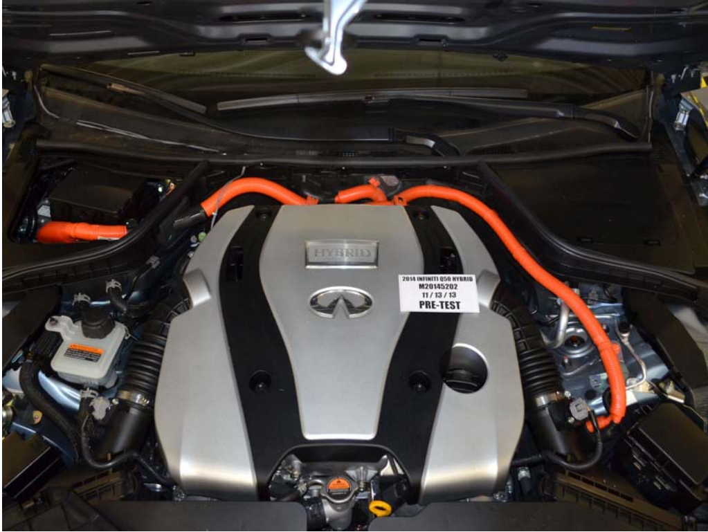
FIGURE 16. Pre-Impact View of Electric Propulsion Drive
