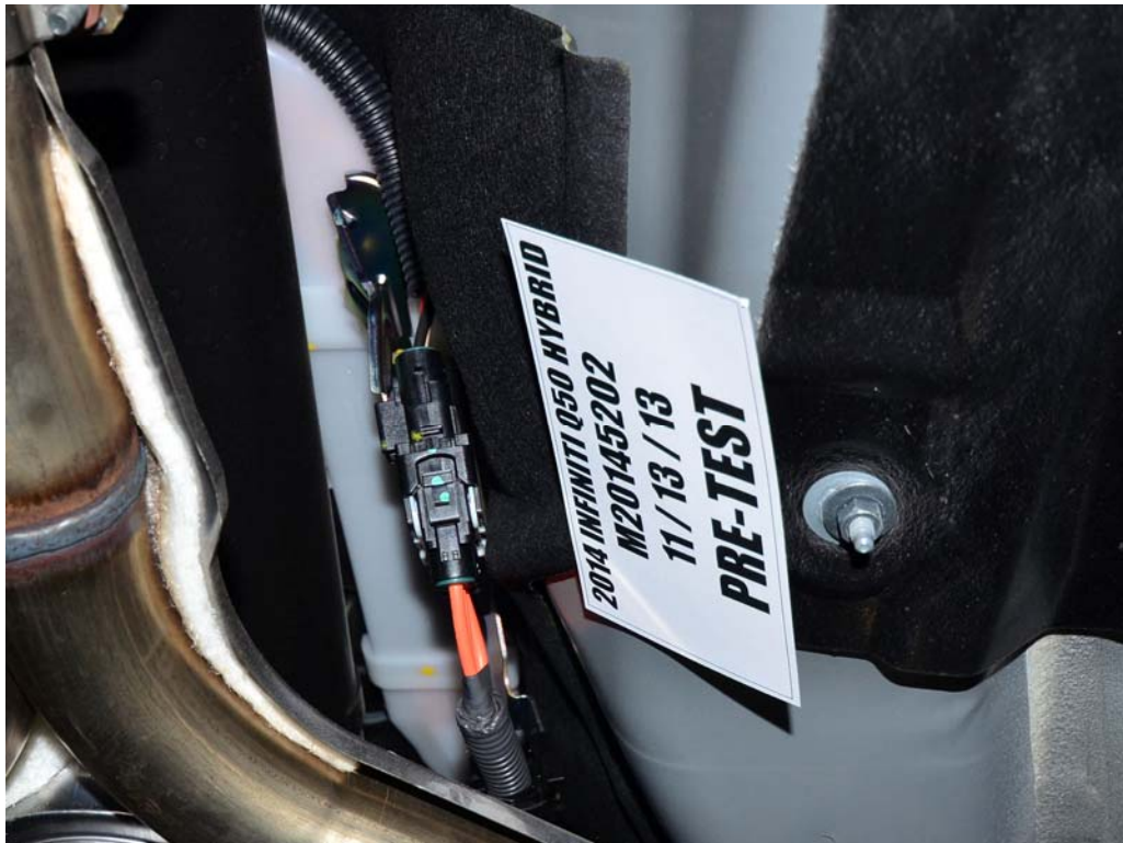
FIGURE 18a. Pre-Impact View of High Voltage Interconnects
