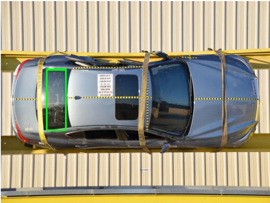
FIGURE 29. FMVSS No. 305 Static Rollover at 90°
